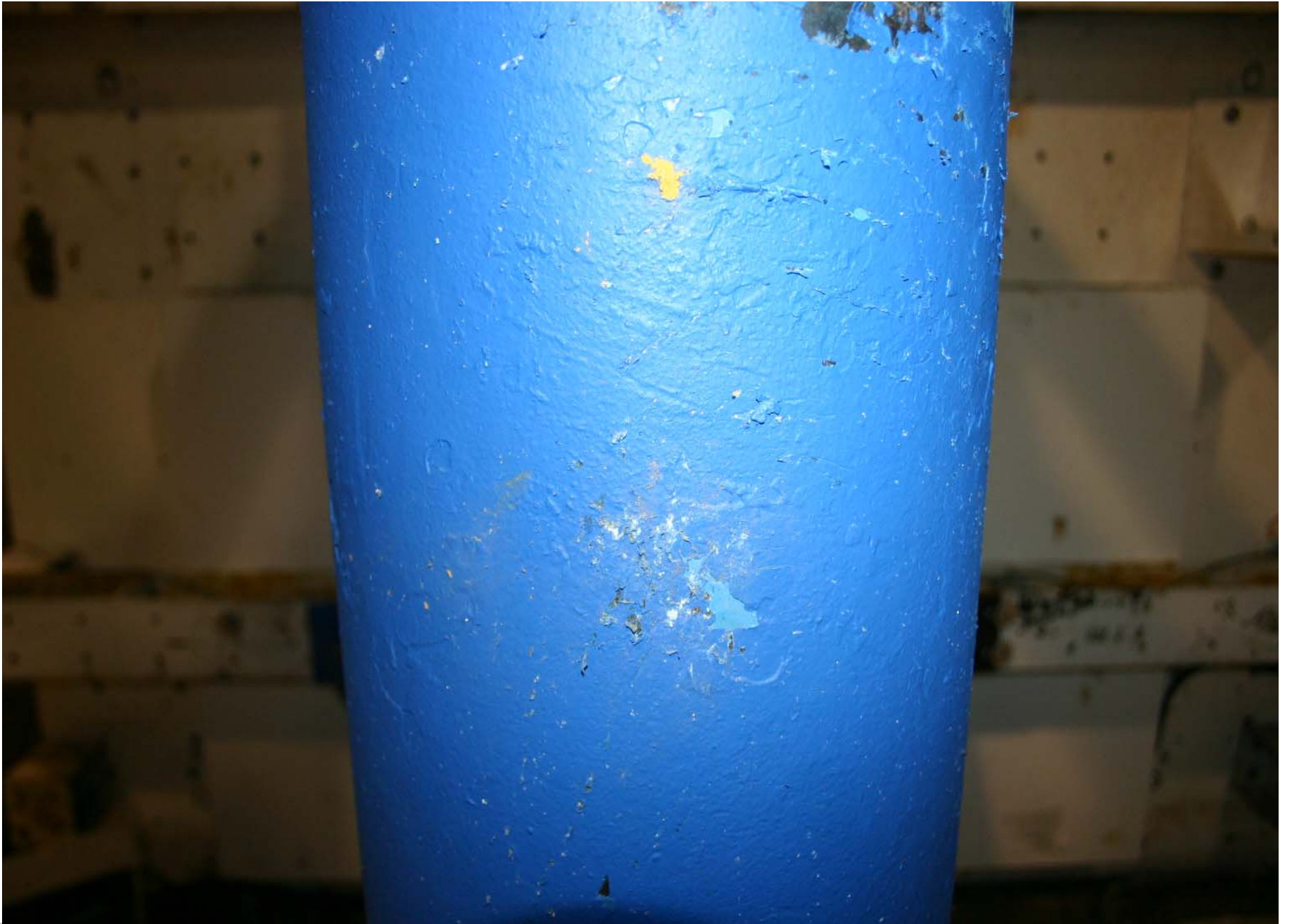
Post-Test Driver Dummy Head Contact with Pole
