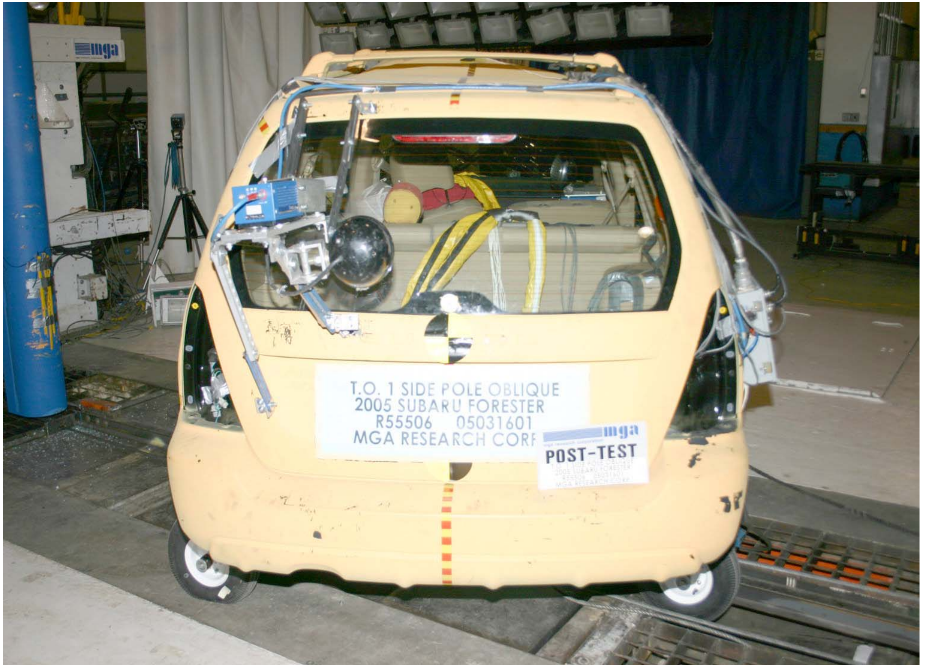
Post-Test Rear View of Test Vehicle
