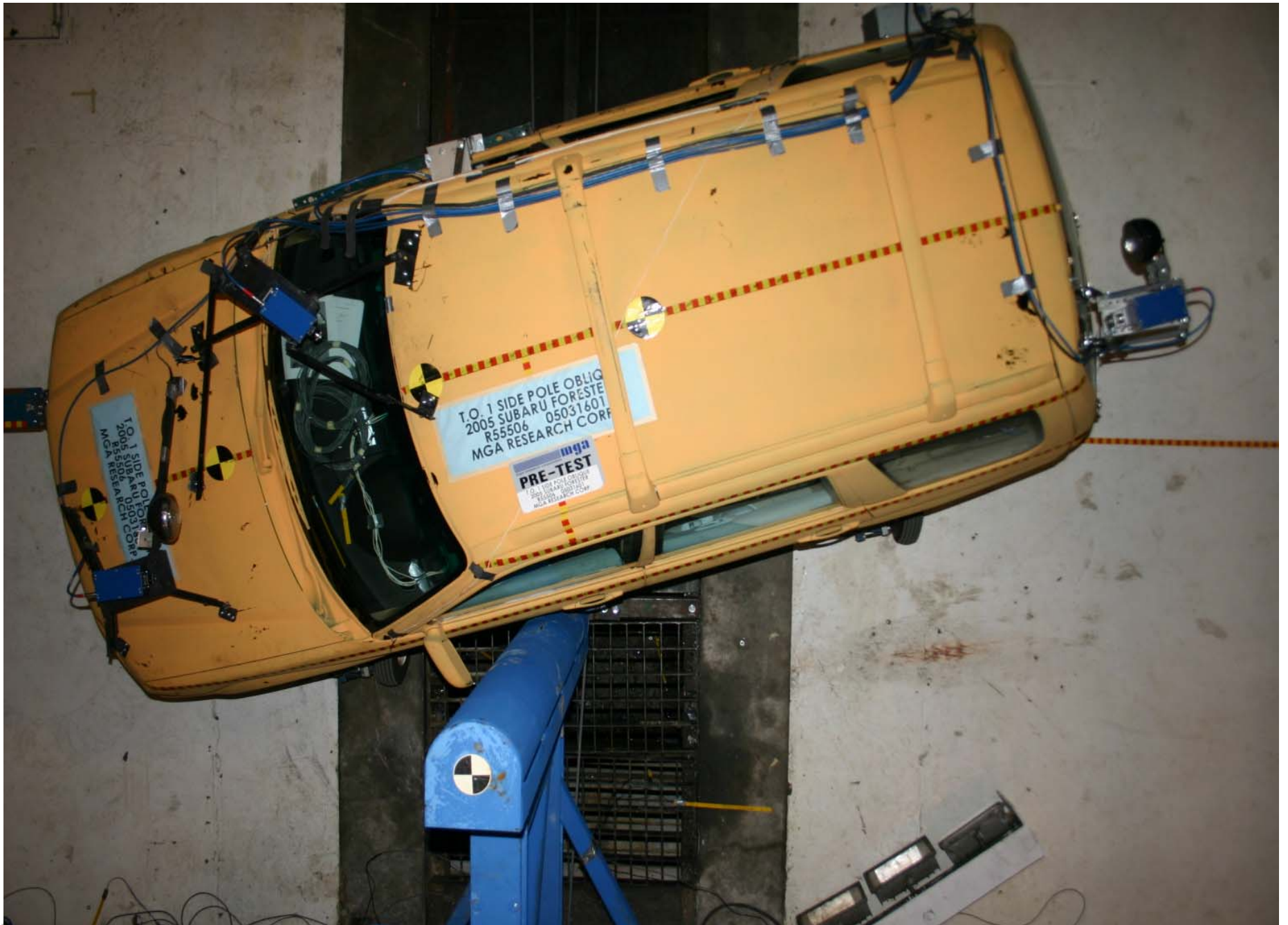
Pre-Test Vehicle Overhead View Positioned Against Pole
