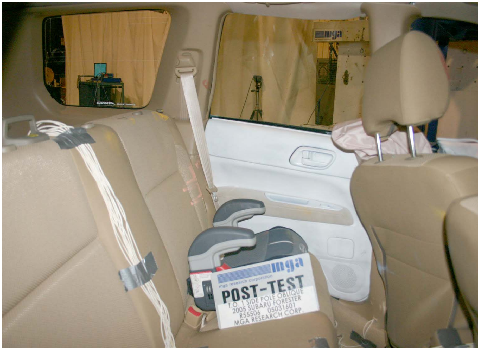
Post-Test LRP Child Dummy Contact
