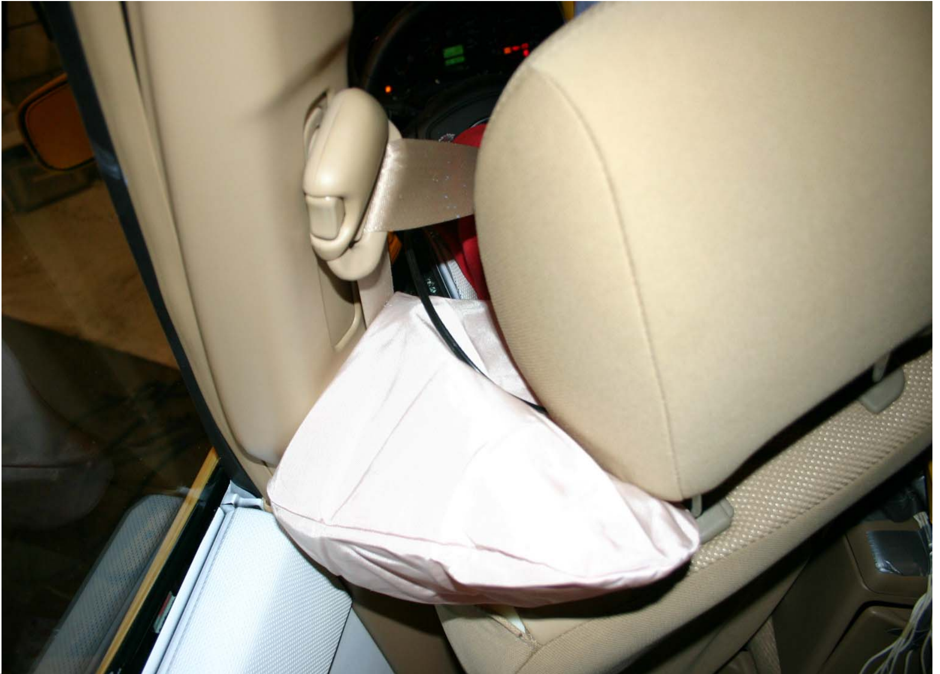
Post-Test Combination Airbag
