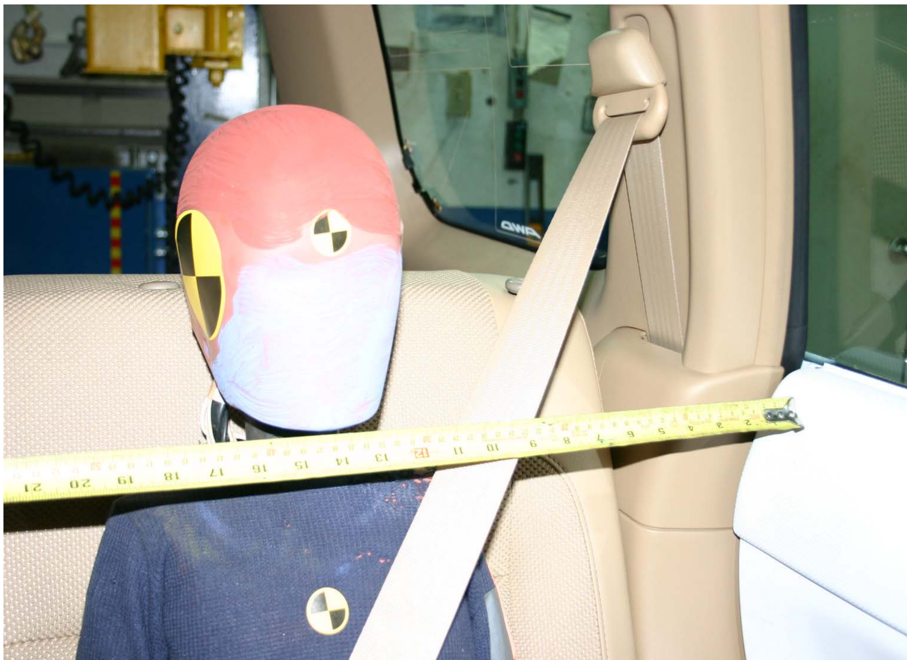
Pre-Test LRP Child Dummy Lateral Clearance Measurements
