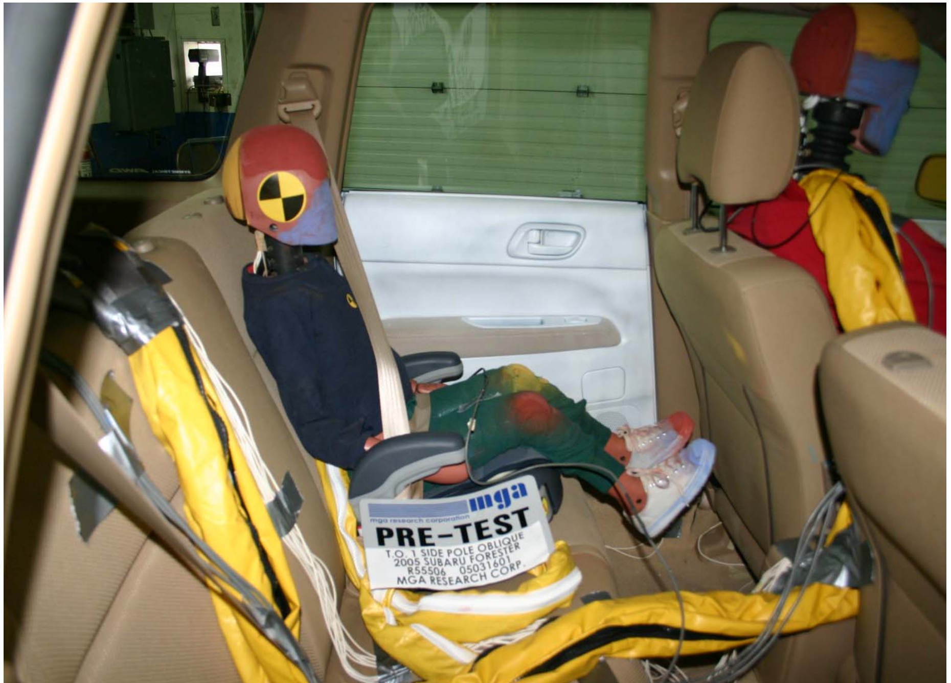
Pre-Test LRP Child Dummy Right Side View
