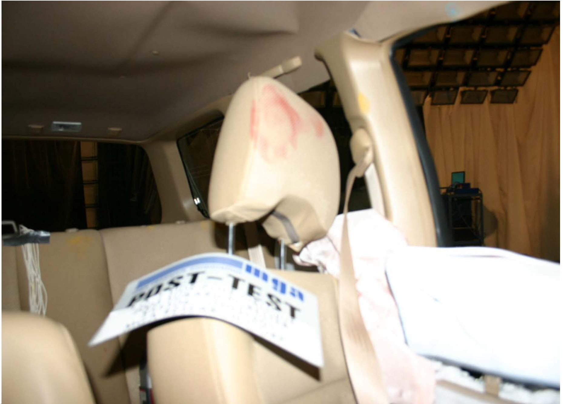
Post-Test Driver Dummy Head Contact
