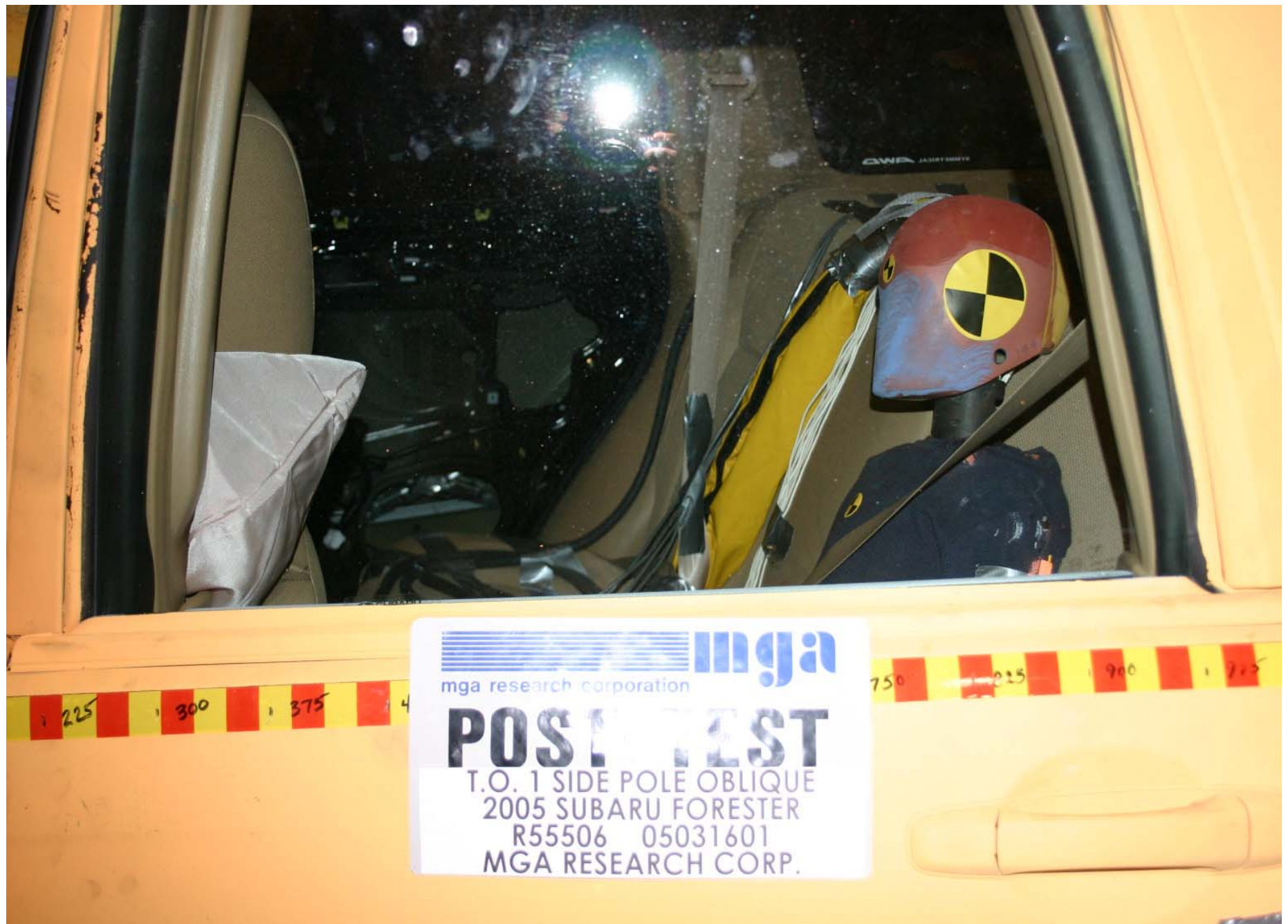
Post-Test LRP Child Dummy Left Side View
