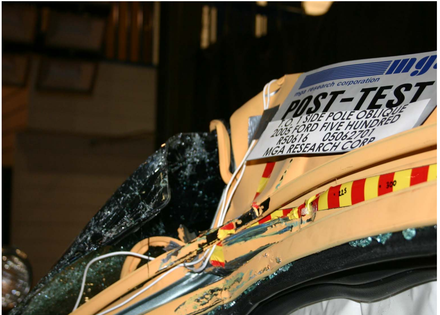
Post-Test Windshield Retention
