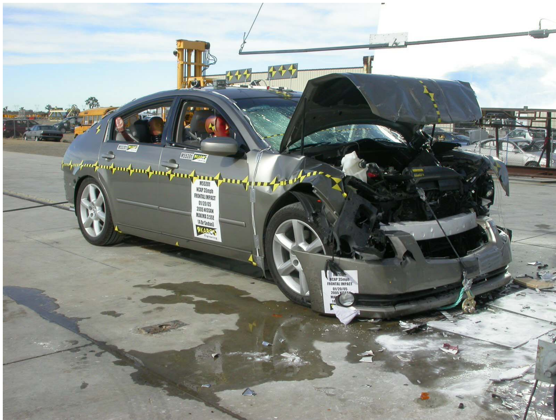
Figure A-3: Post-Test Right Front \frac{3}{4} View of Frontal NCAP Test
