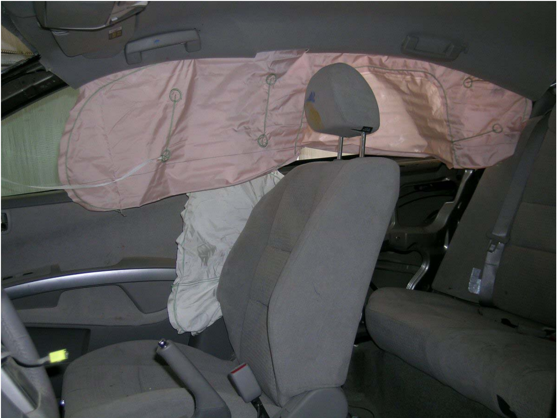
Figure A-9: Post-Test Airbags, Left Side View
