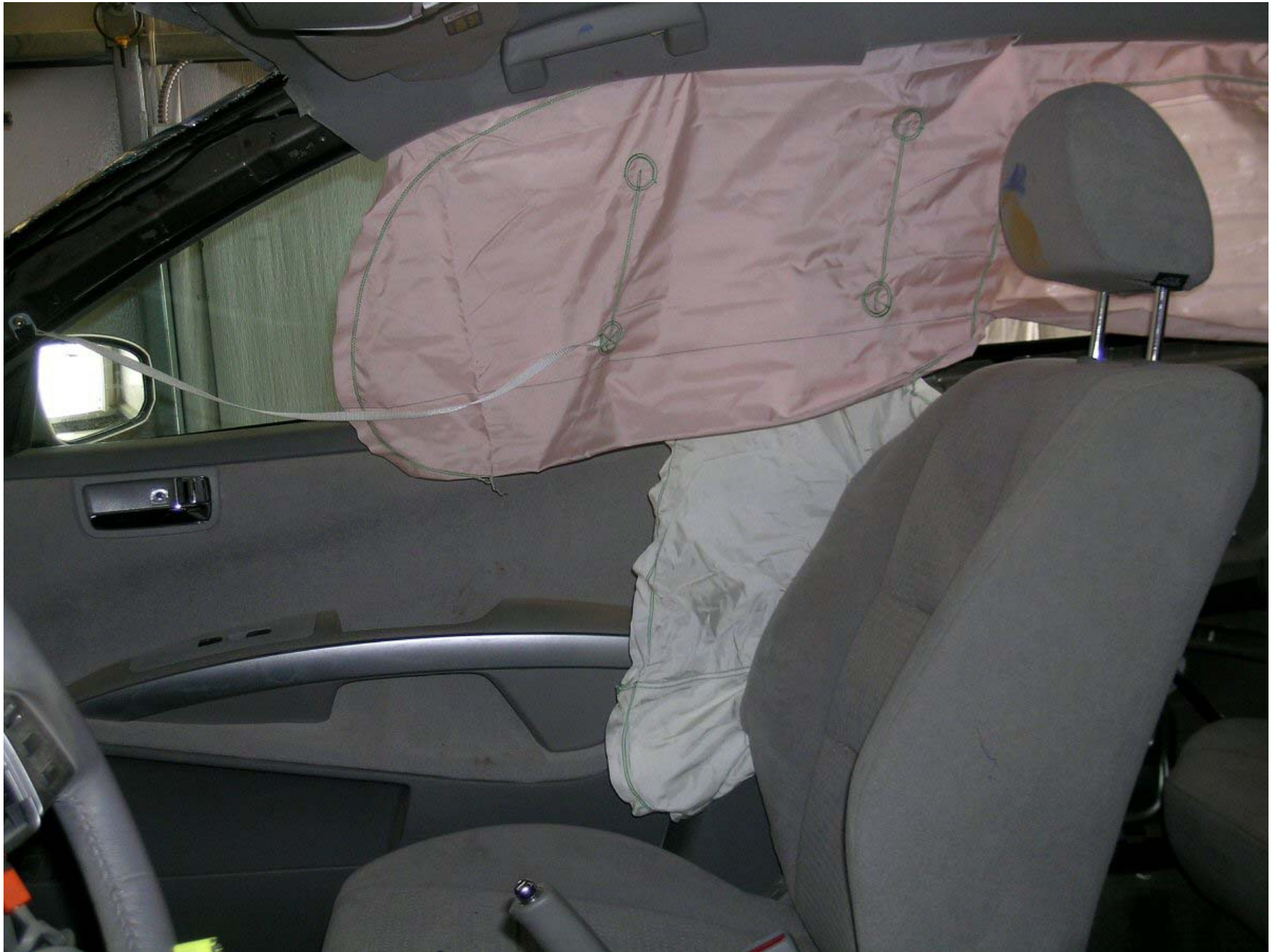
Figure A-10: Post-Test Airbags, Left Side Close-up View
