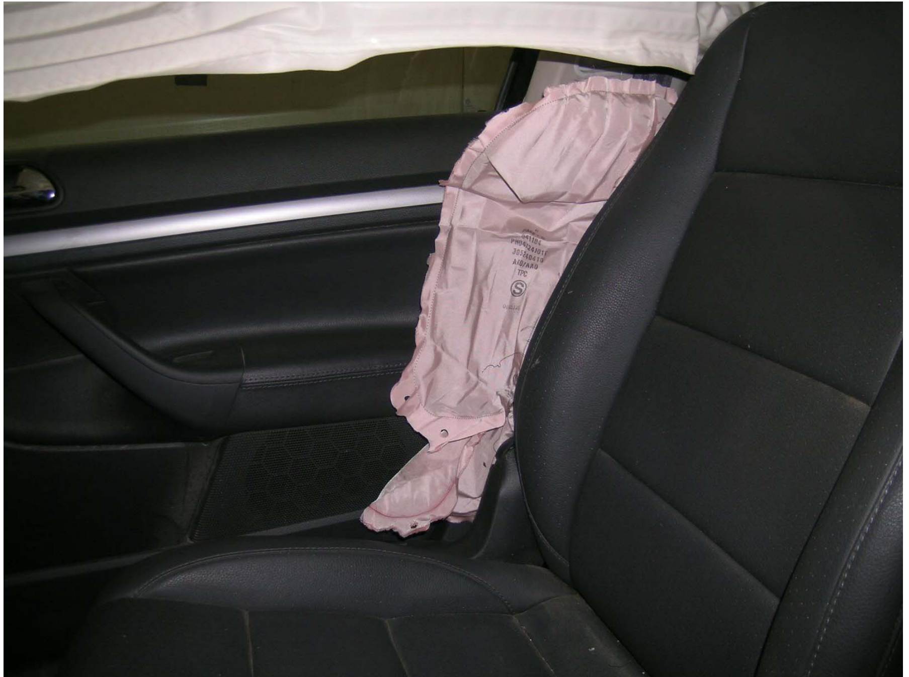
Figure A-10: Post-Test Side Airbag, Left Side Close-up View
