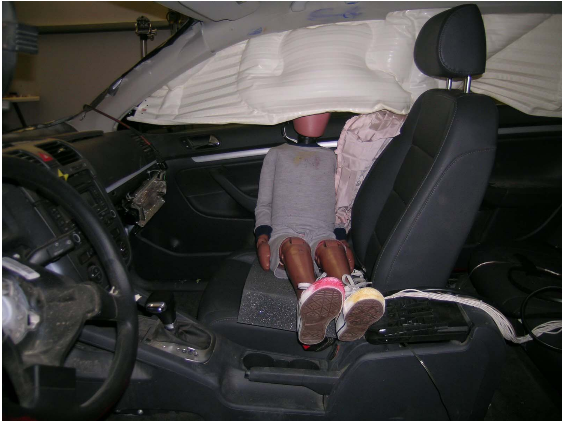
Figure A-8: Post-Test Dummy Position and Airbags, Left Side View
