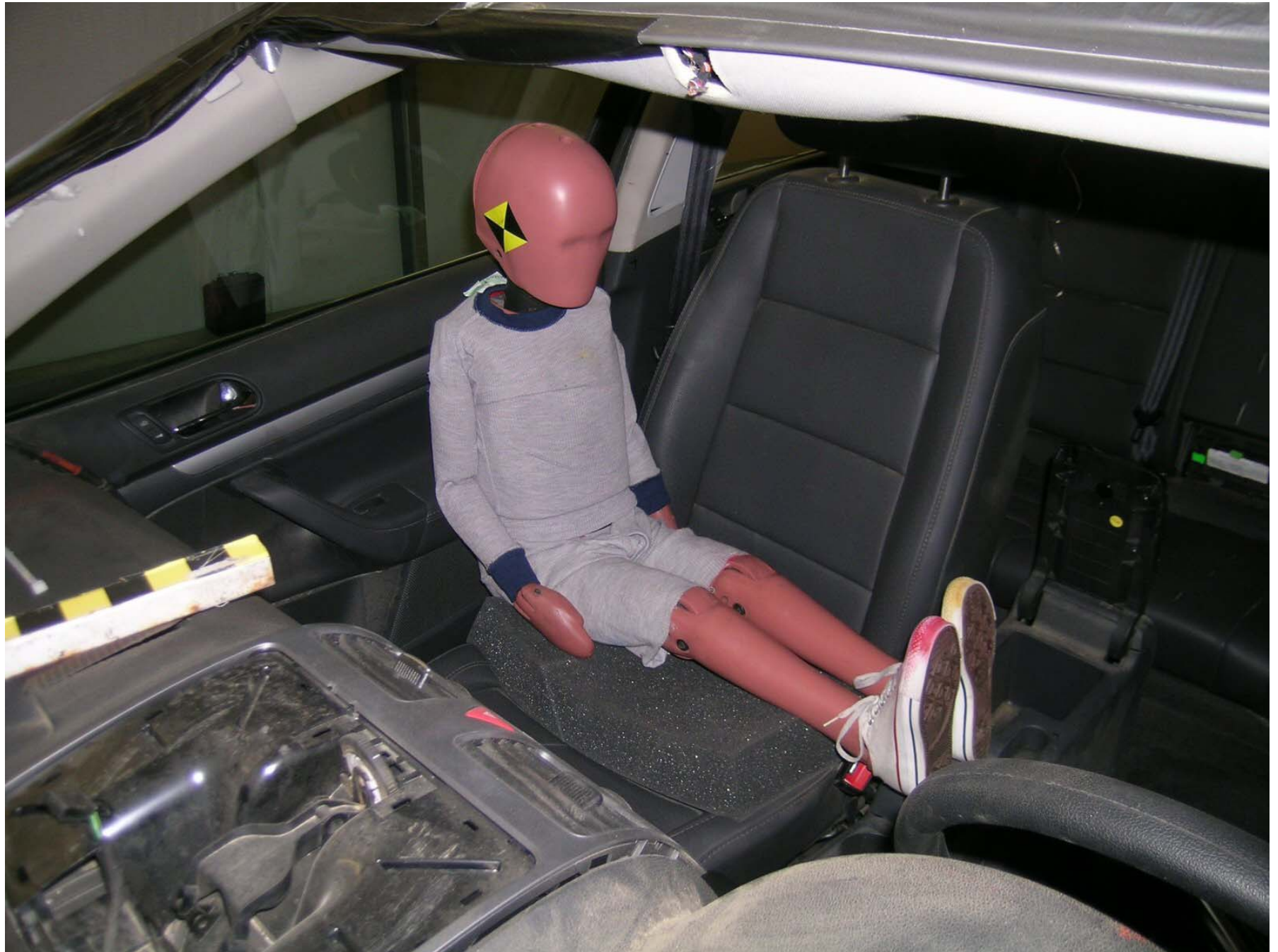
Figure A-6: Pre-Test Dummy Position, \frac{3}{4} View
