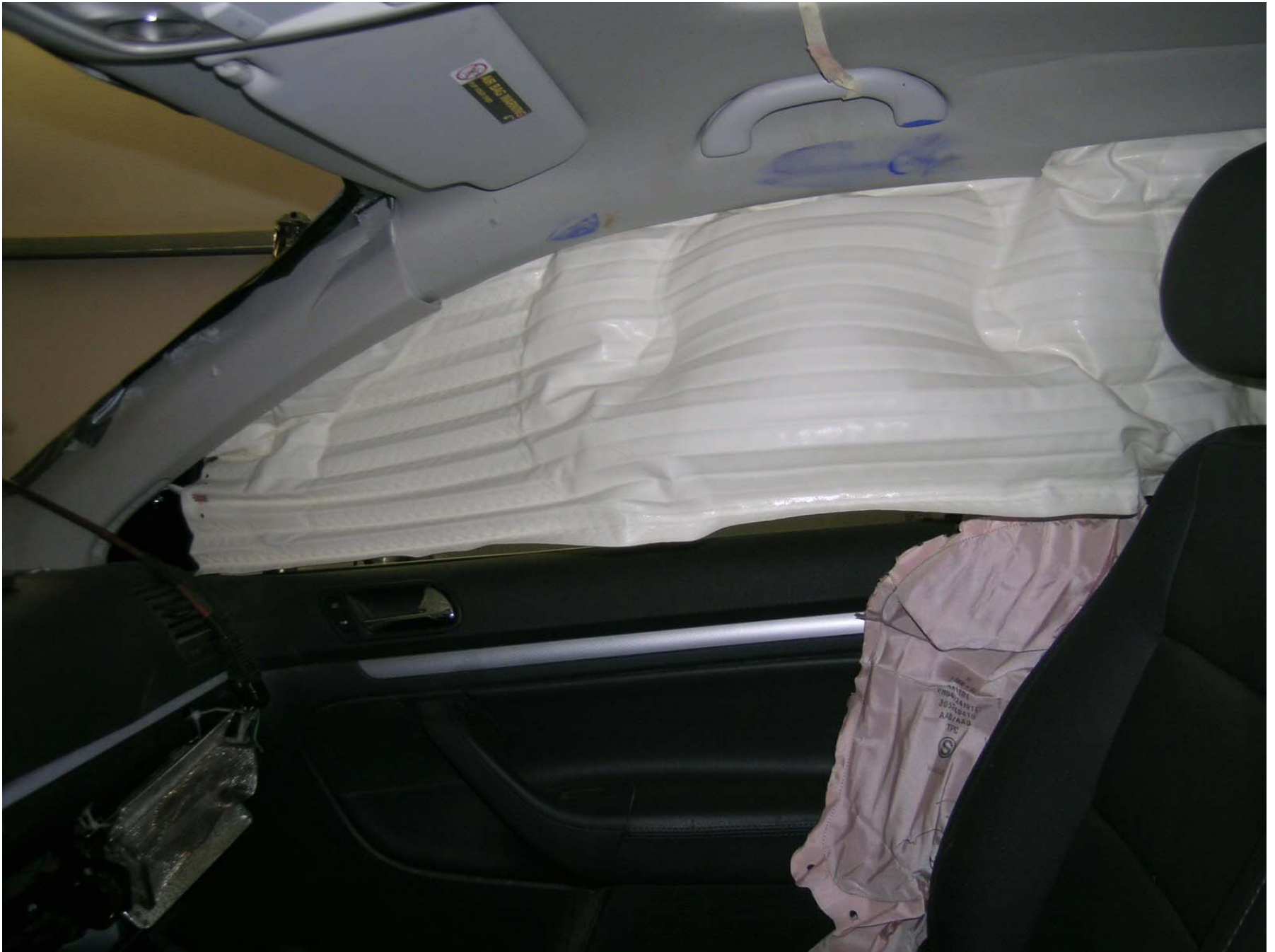
Figure A-9: Post-Test Airbags, Left Side View
