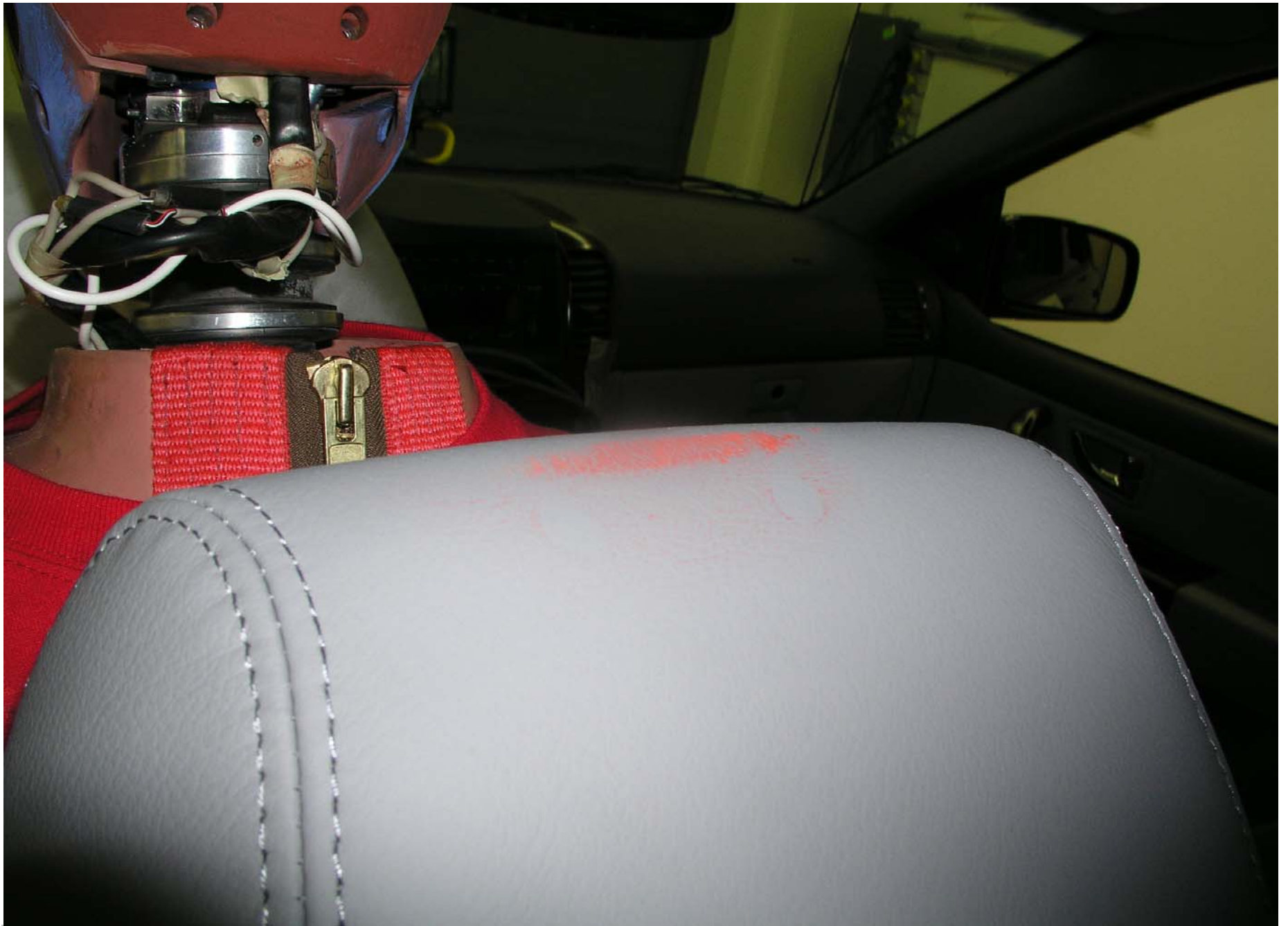
Post-Test 5th Fem. P2 Driver Dummy Head Contact View (headrest)
