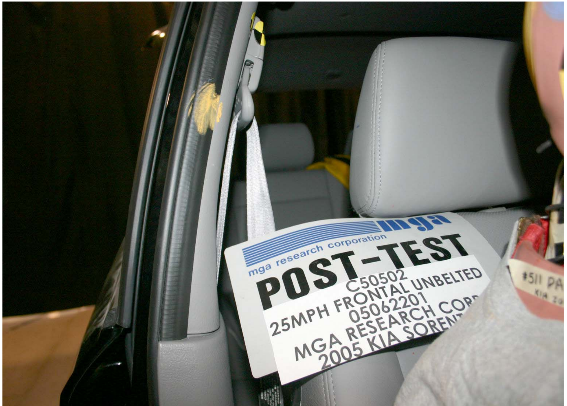
Post-Test Passenger Dummy Head Contact (B-Pillar )
