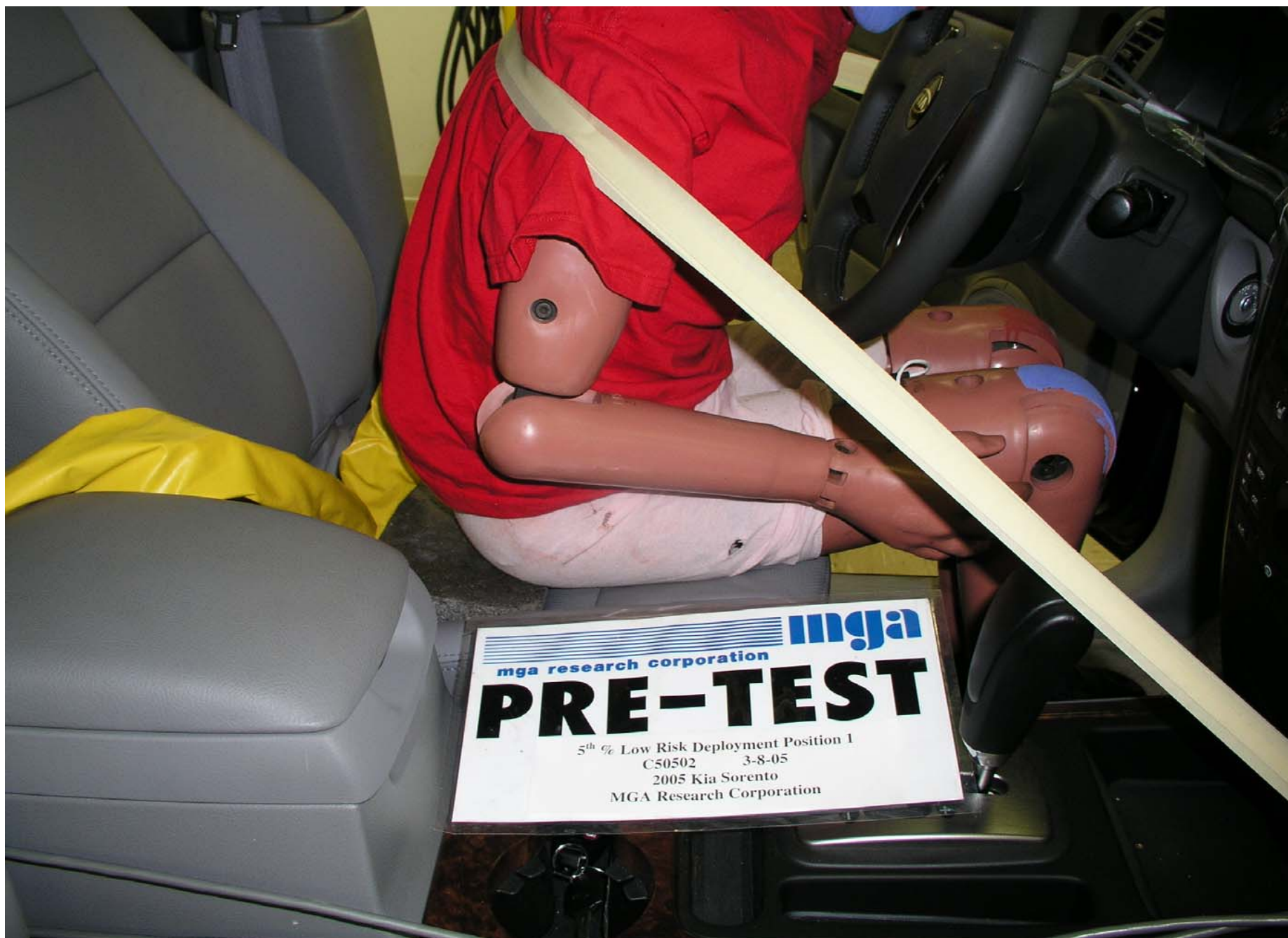
Pre-Test 5th Fem. P1 Driver Dummy Right Side Mid Position View
