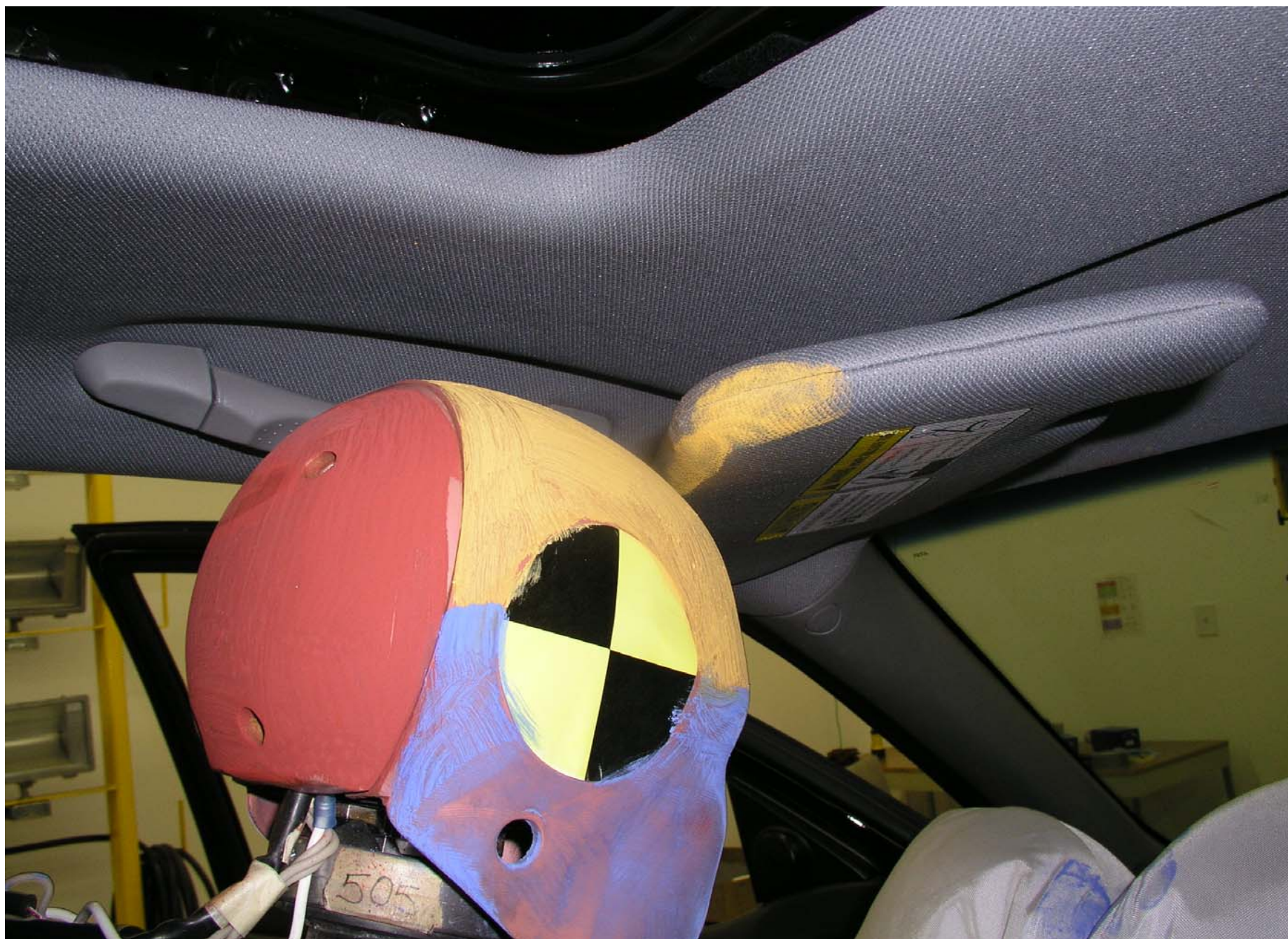
Post-Test 5th Fem. P2 Driver Dummy Head Contact View (visor)
