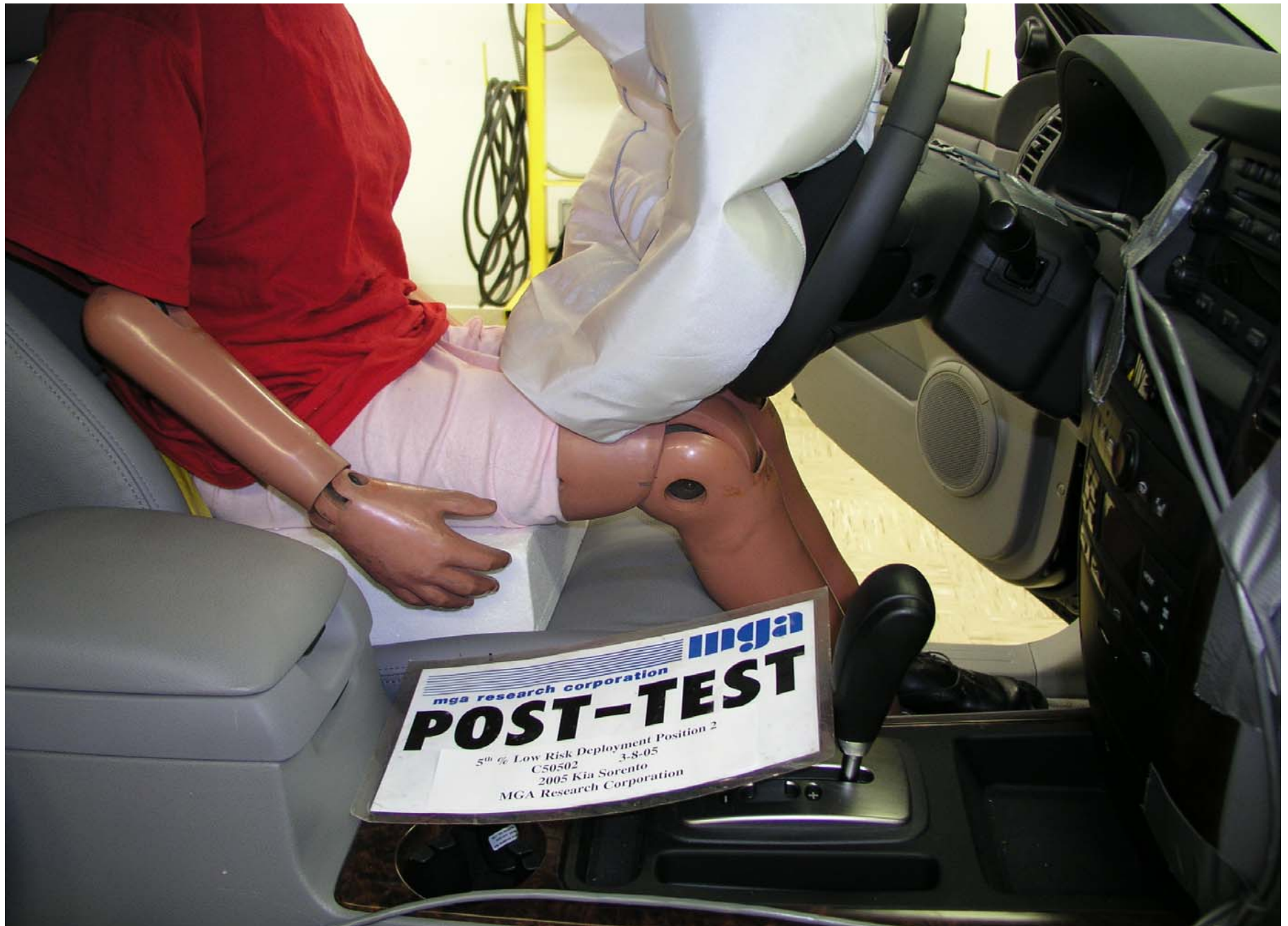
Post-Test 5th Fem. P2 Driver Dummy Right Side Knee Position View
