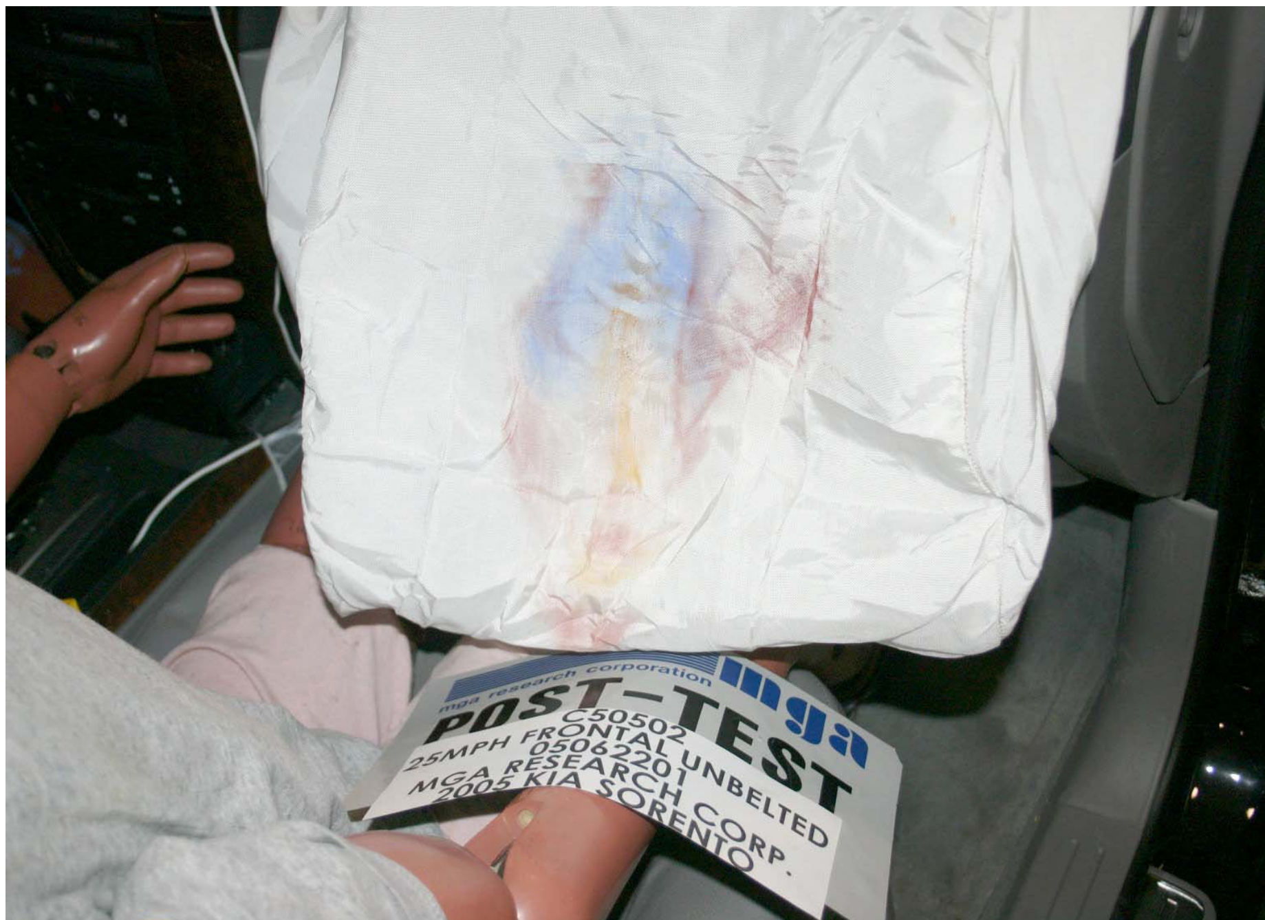
Post-Test Passenger Dummy Airbag Contact
