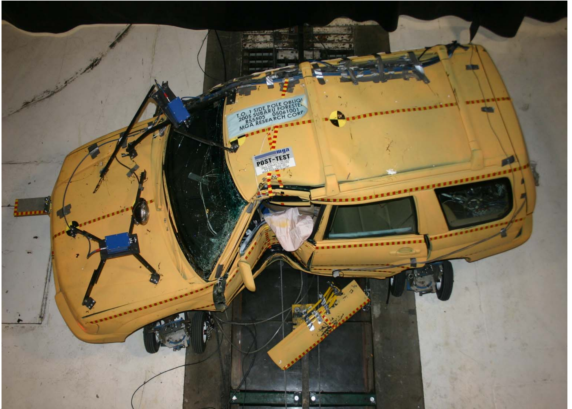
Post-Test Vehicle Overhead View
