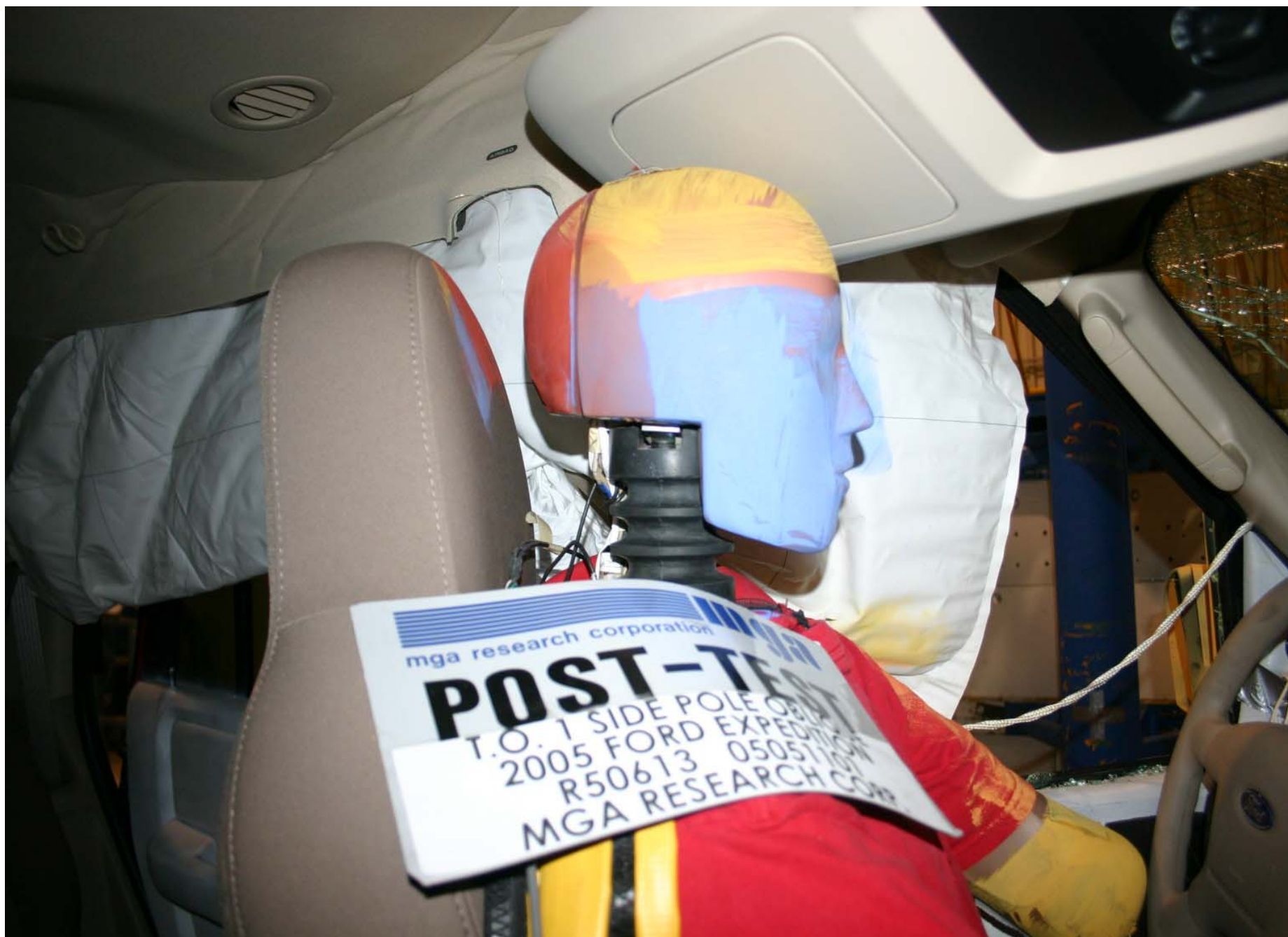
Post-Test Driver Dummy Head Contact
