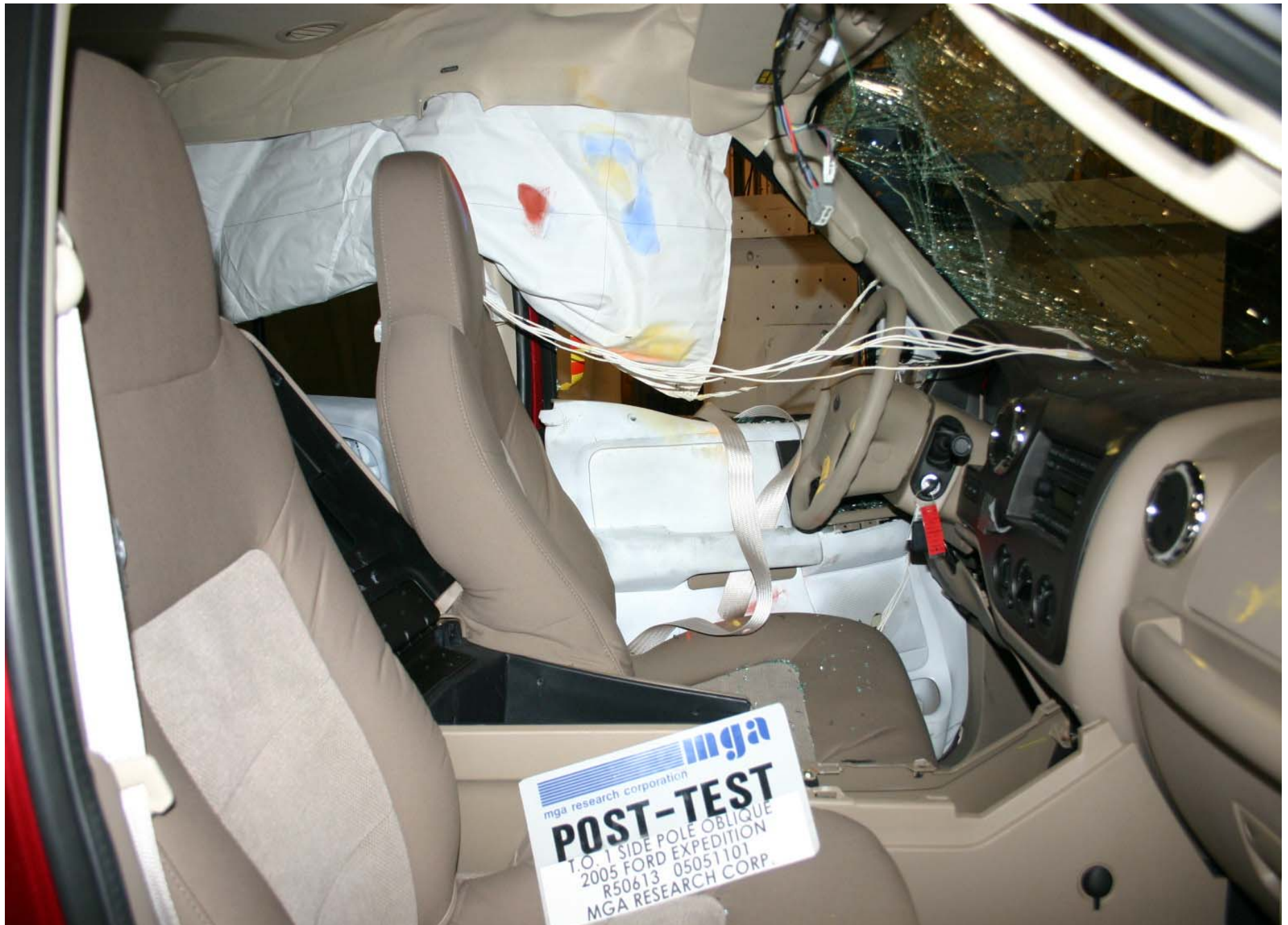
Post-Test Driver Dummy Contact
