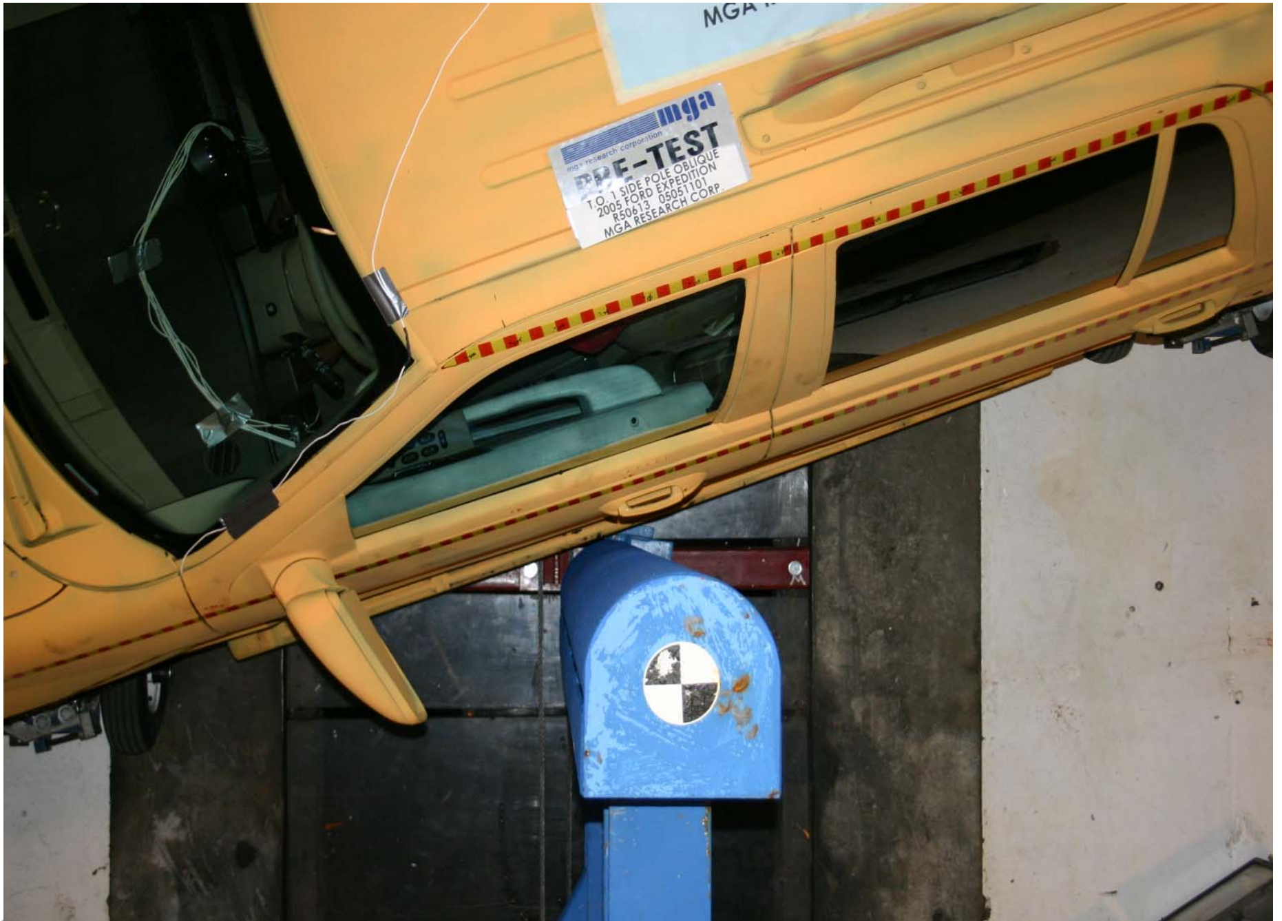
Pre-Test Vehicle Overhead View Positioned Against Pole
