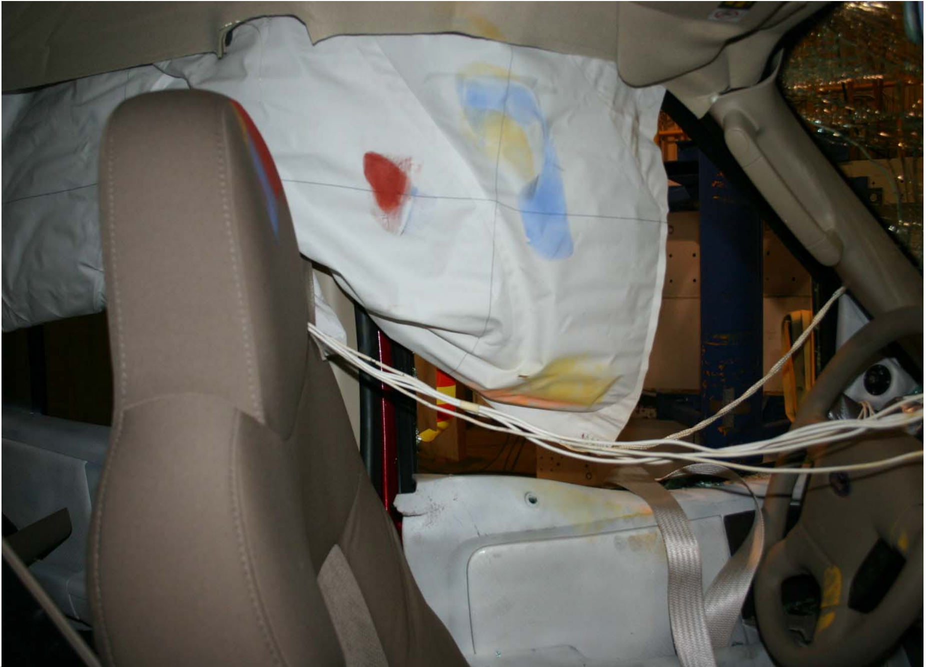
Post-Test Driver Dummy Head Contact
