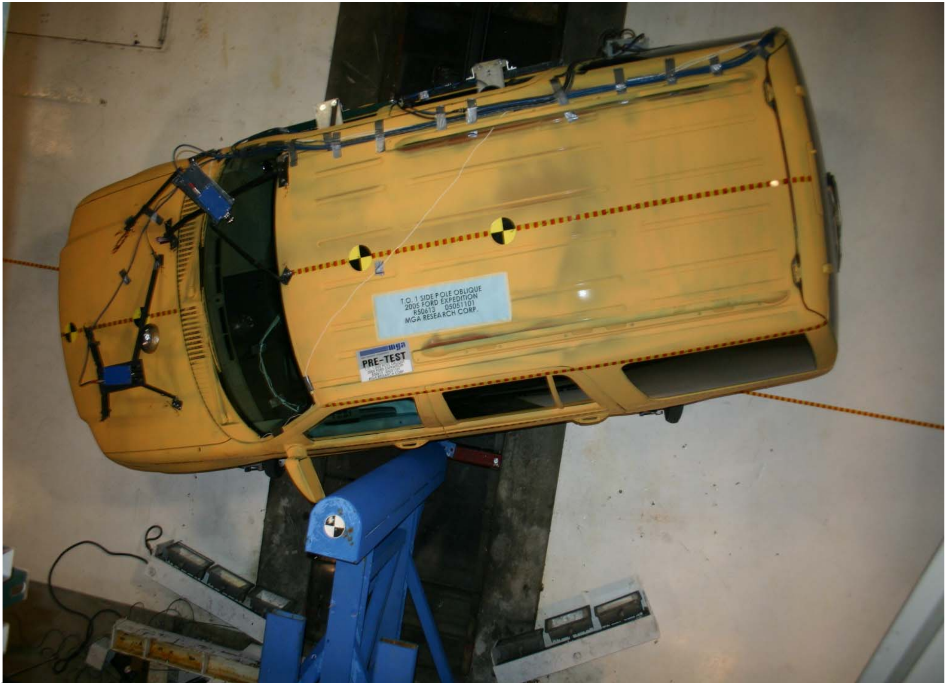
Pre-Test Vehicle Overhead View Positioned Against Pole
