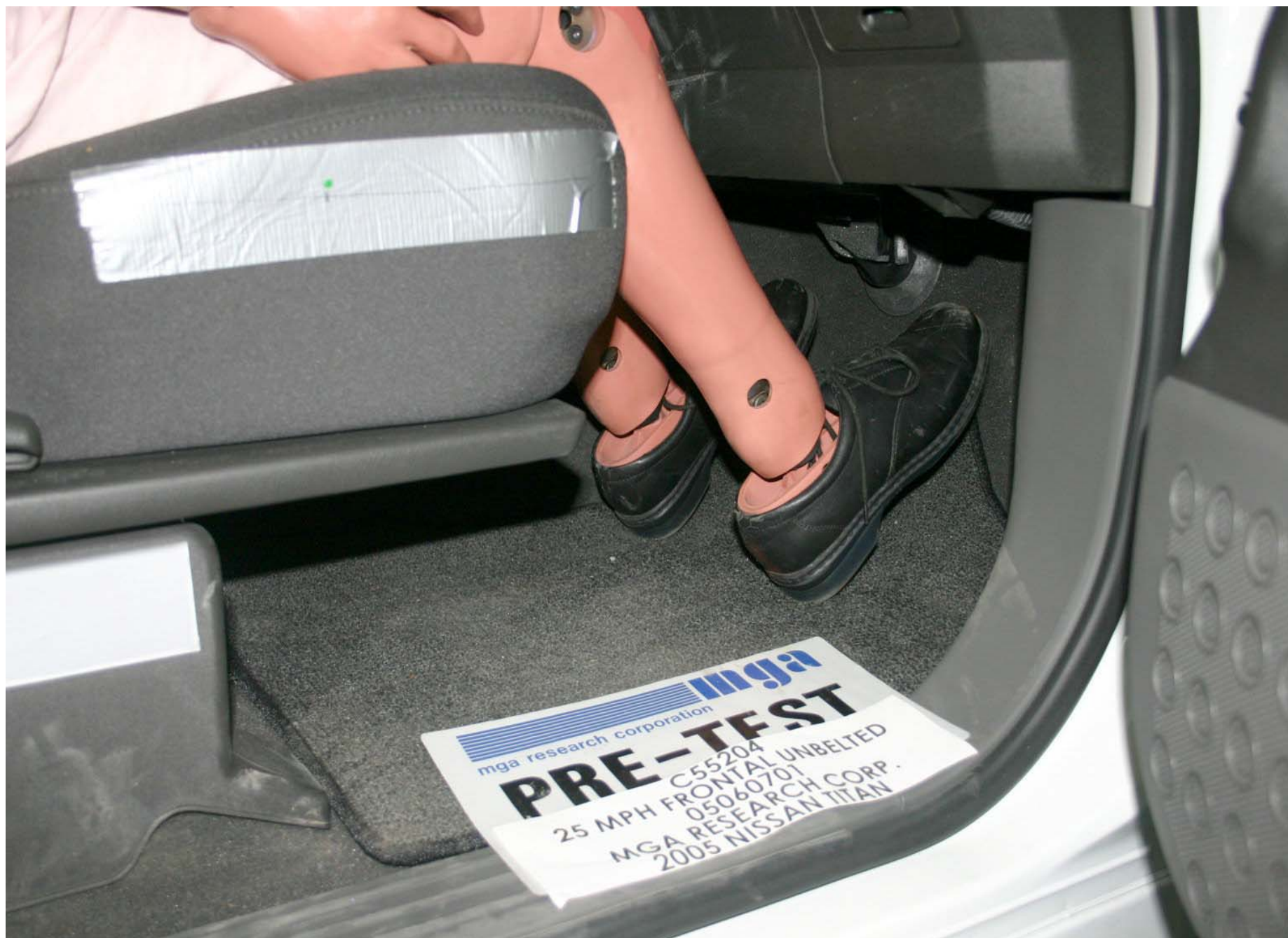
Pre-Test Passenger Dummy Feet Position
