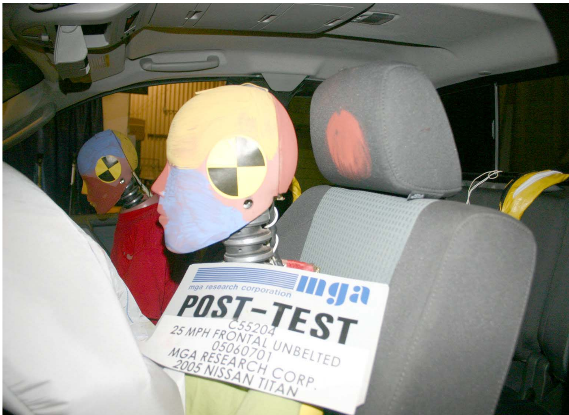
Post-Test Driver Dummy Head Contact (headrest)
