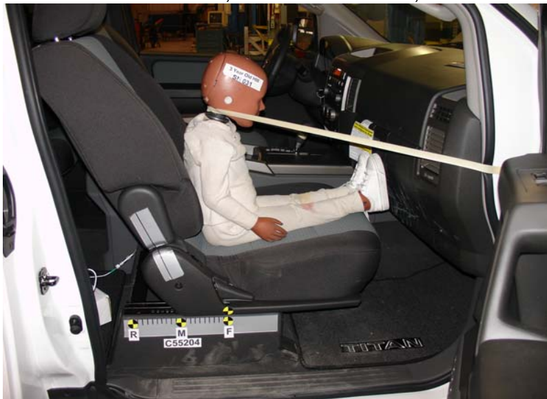
3-Year-Old Unbelted, Forward Seat Track, Position 3
