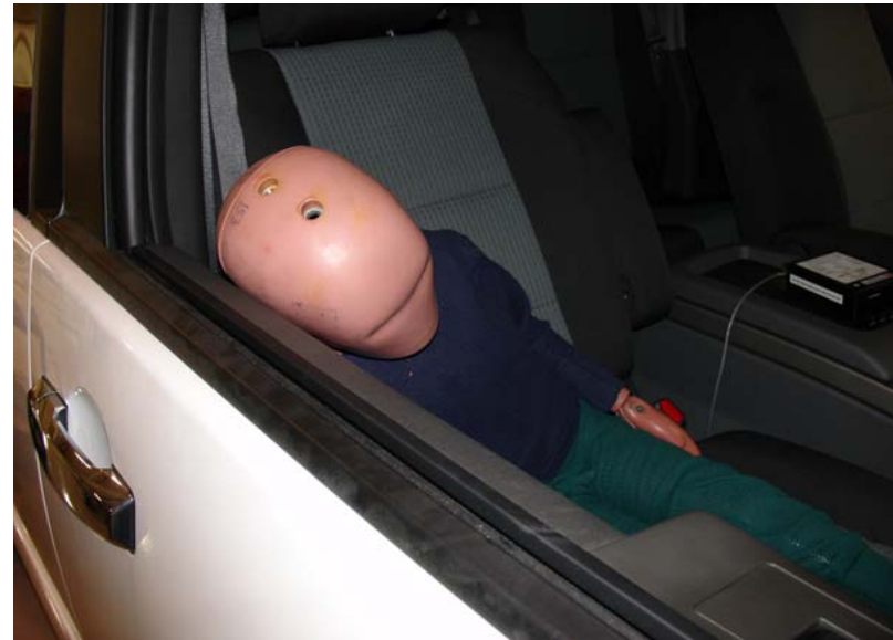
6-Year-Old Unbelted, Rearward Seat Track, Position 4
