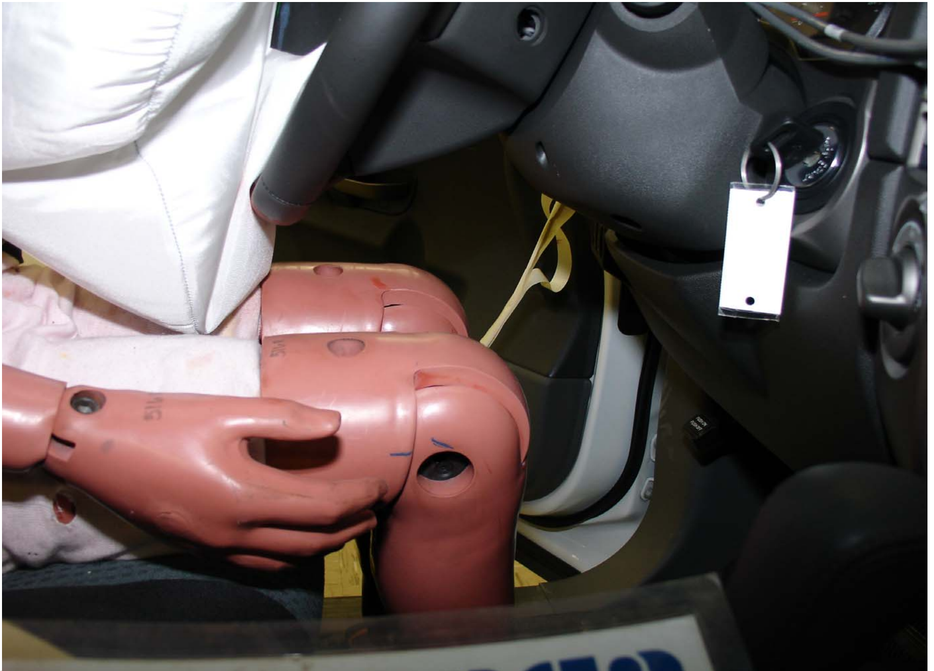
Post-Test 5th Fem. P1 Driver Dummy Right Side Knee Position View
