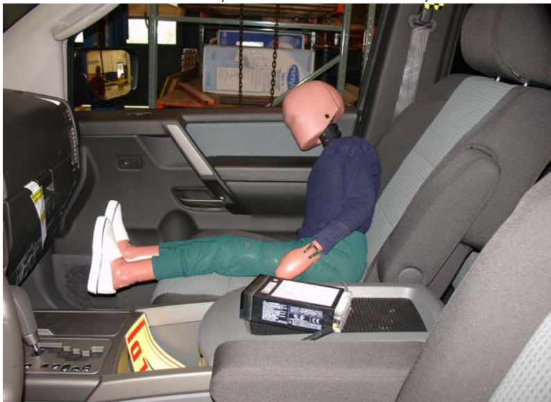
6-Year-Old Unbelted, Rearward Seat Track, Position 4, View 2
