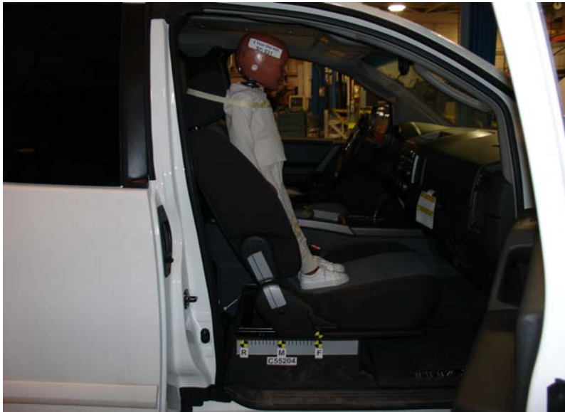
3-Year-Old Unbelted, Forward Seat Track, Position 5
