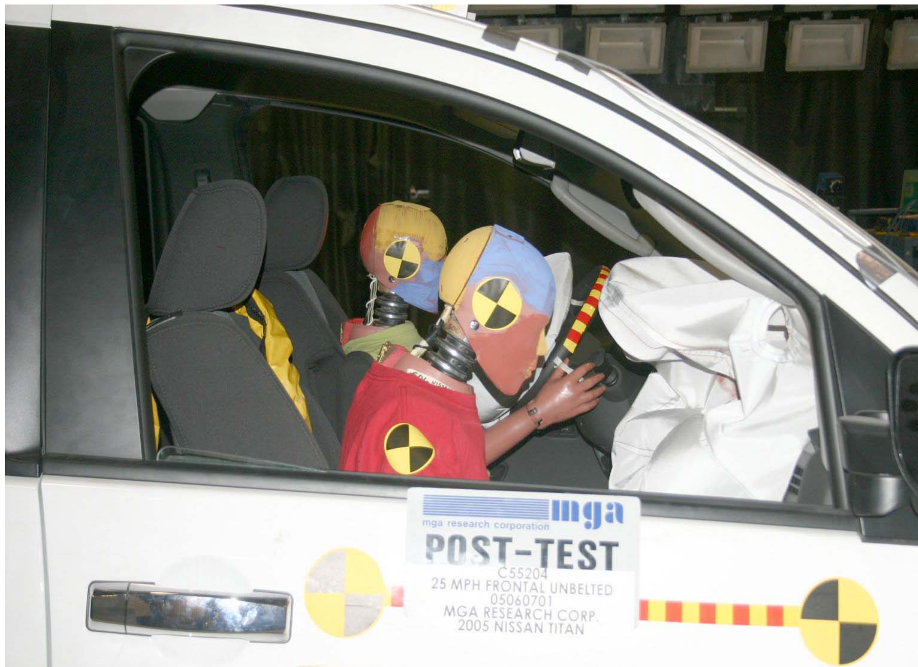
Post-Test Passenger Dummy Position Right Side View
