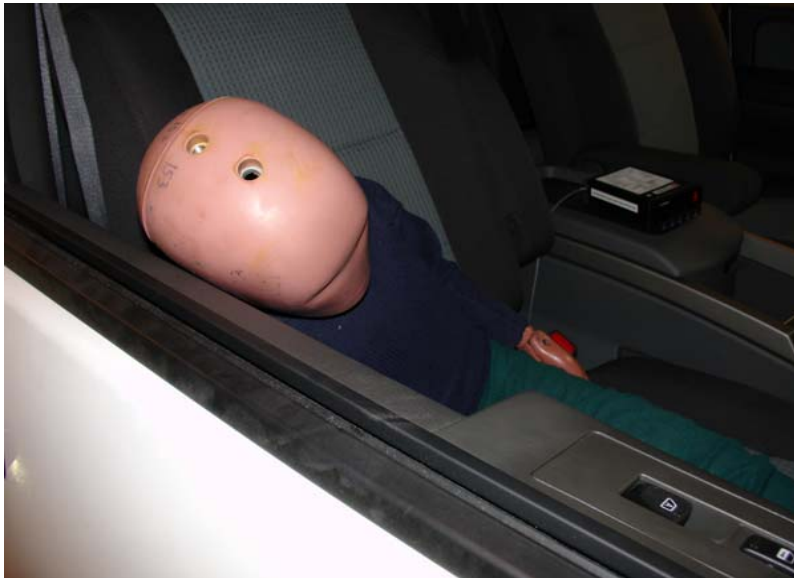
6-Year-Old Unbelted, Middle Seat Track, Position 4
