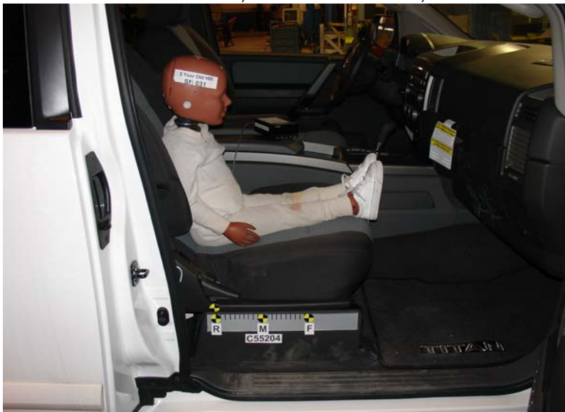
3-Year-Old Unbelted, Rearward Seat Track, Position 1
