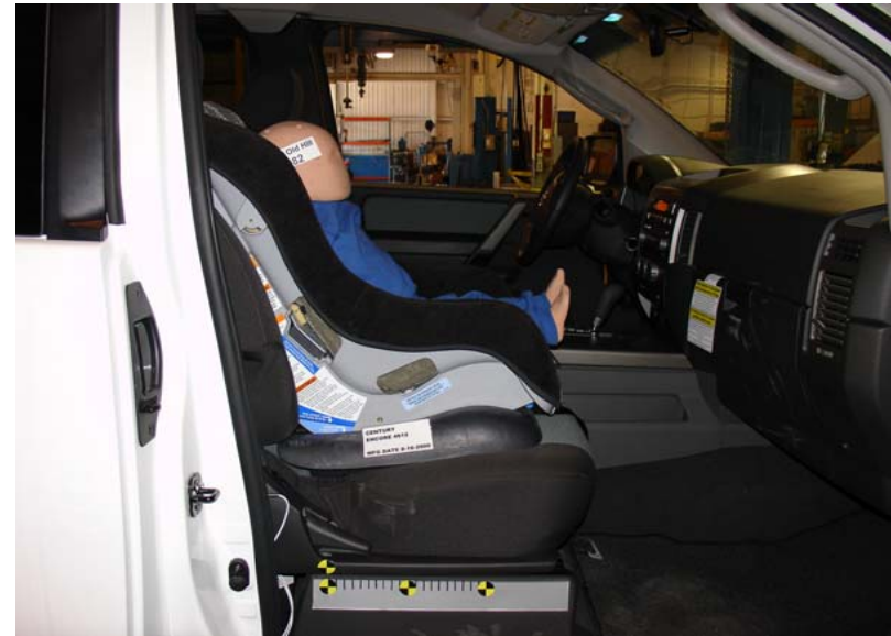
Century Encore Fwd Facing Unbelted, Rearward Seat Track
