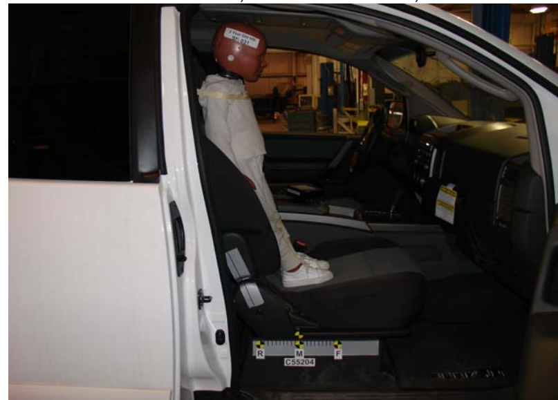
3-Year-Old Unbelted, Middle Seat Track, Position 5
