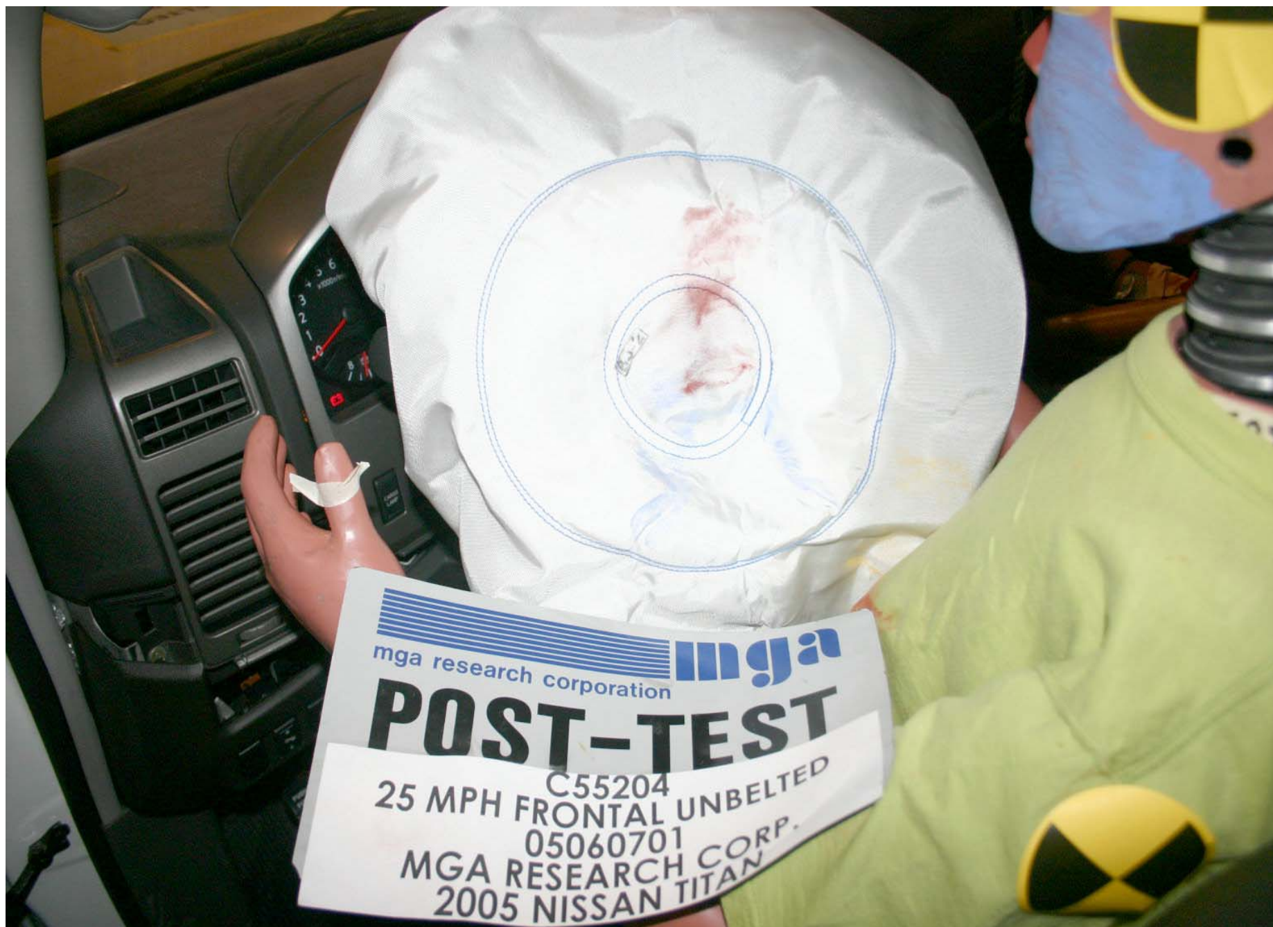
Post-Test Driver Dummy Airbag Contact
