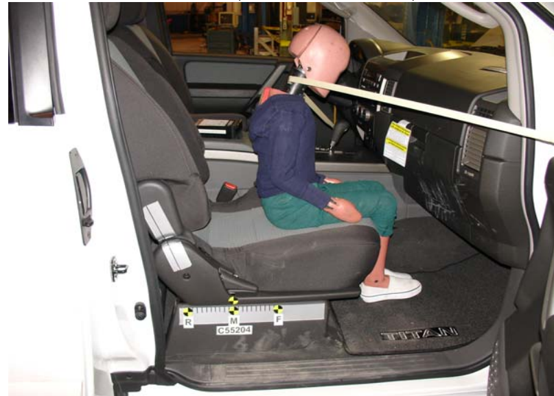
6-Year-Old Unbelted, Middle Seat Track, Position 3
