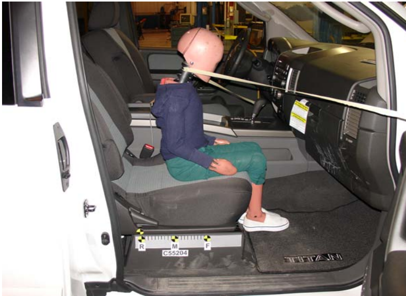
6-Year-Old Unbelted, Rearward Seat Track, Position 3
