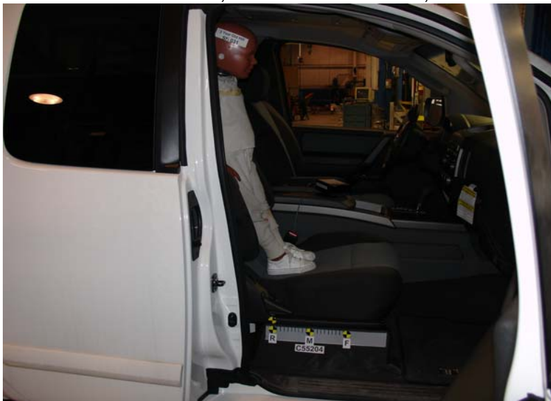
3-Year-Old Unbelted, Rearward Seat Track, Position 5
