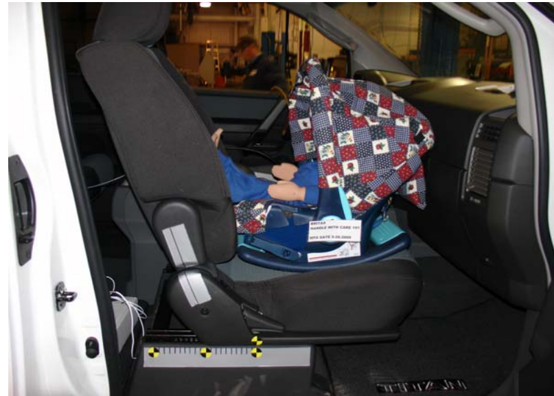
Britax Handle With Care 191 Unbelted, Forward Seat Track, Handle Up
