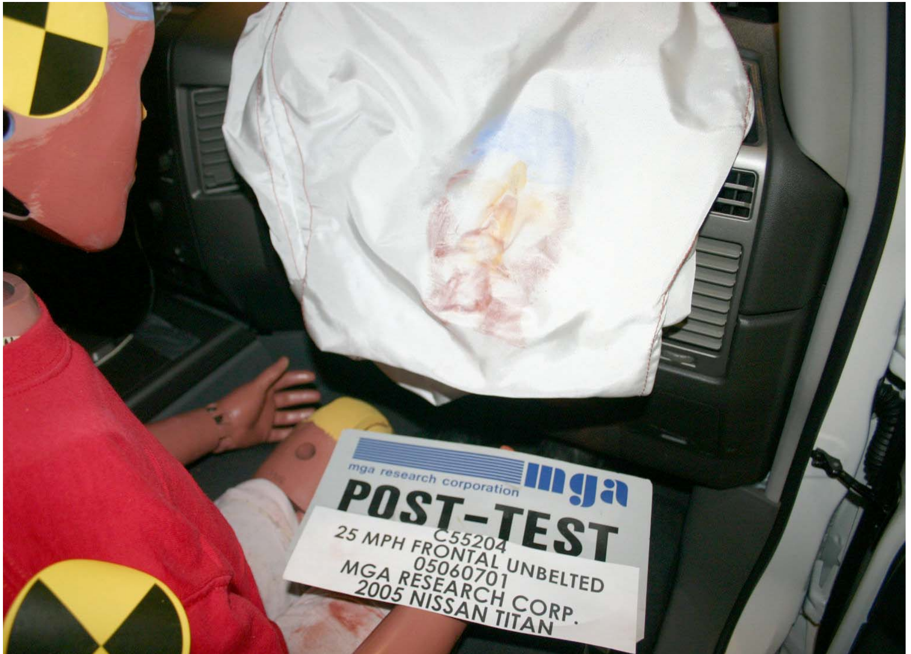
Post-Test Passenger Dummy Airbag Contact
