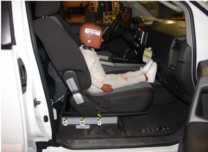
3-Year-Old Unbelted, Forward Seat Track, Position 1
