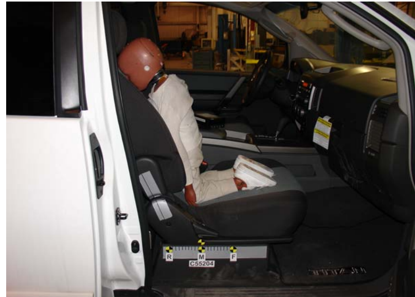
3-Year-Old Unbelted, Middle Seat Track, Position 7
