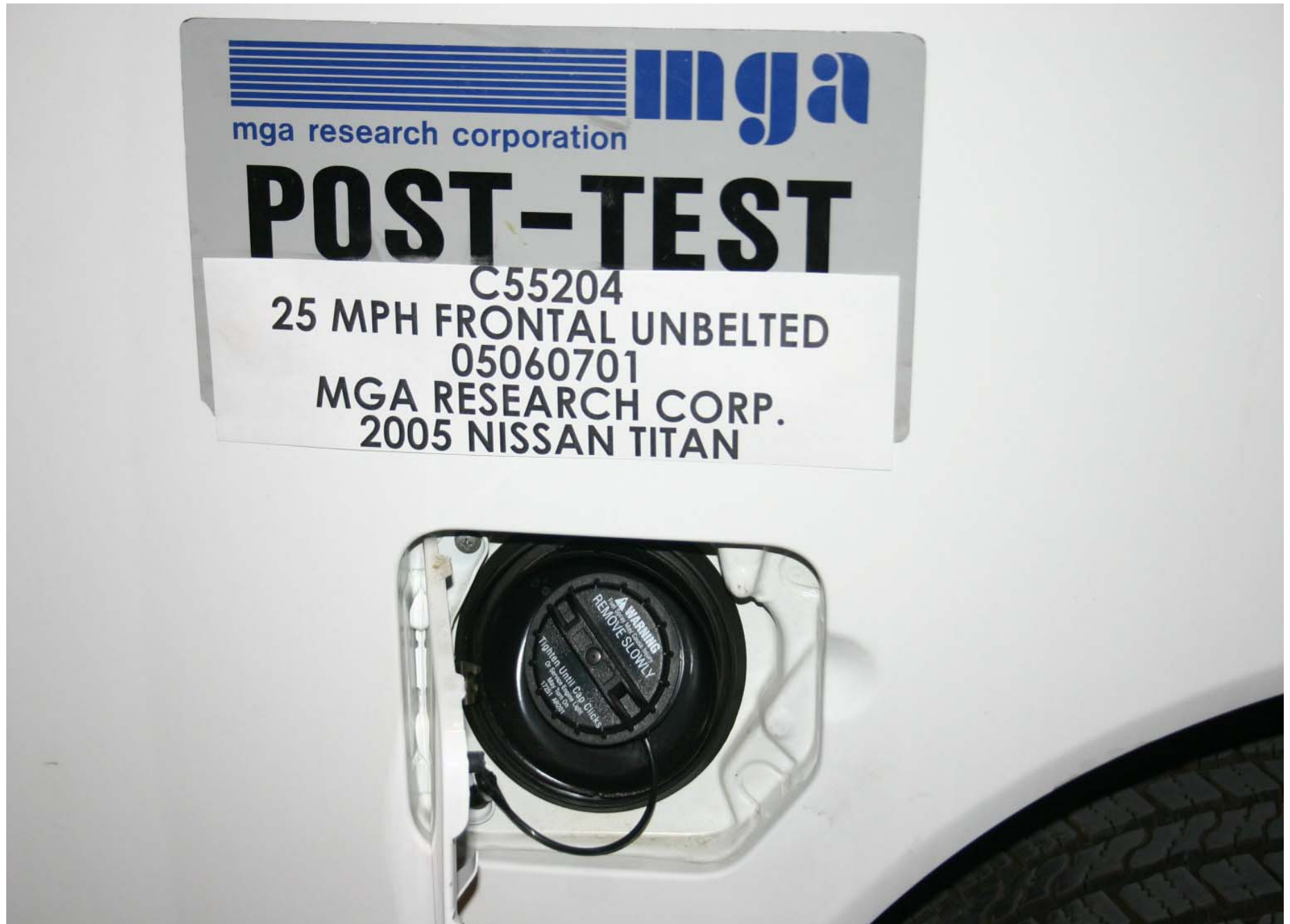
Post-Test Fuel Filler Cap View
