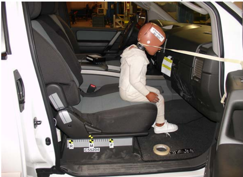
3-Year-Old Unbelted, Middle Seat Track, Position 4
