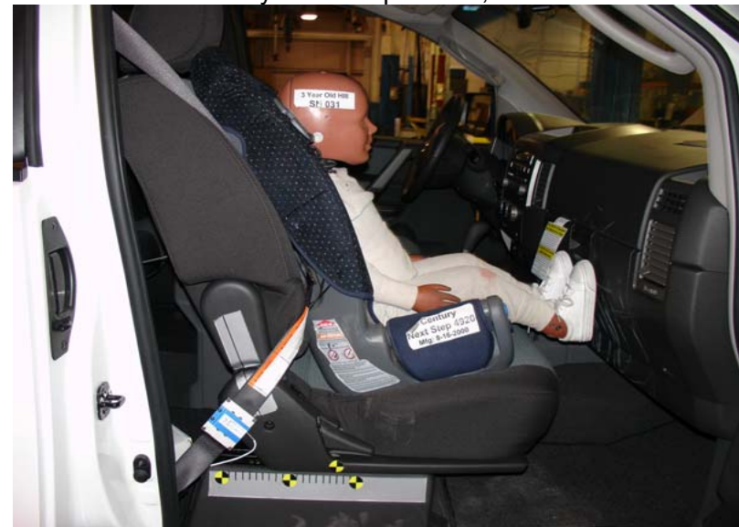
3-Year-Old Century Next Step Cinched With Harness, Forward Seat Track
