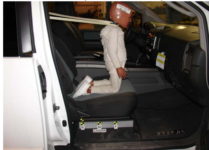
3-Year-Old Unbelted, Rearward Seat Track, Position 6
