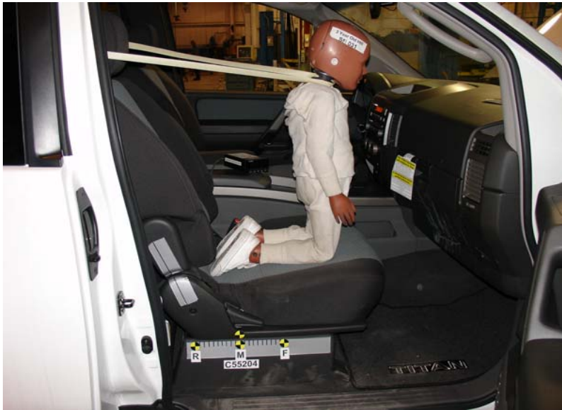
3-Year-Old Unbelted, Middle Seat Track, Position 6
