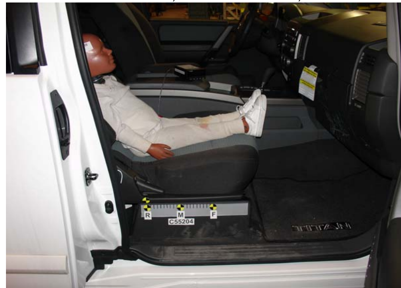
3-Year-Old Unbelted, Rearward Seat Track, Position 2
