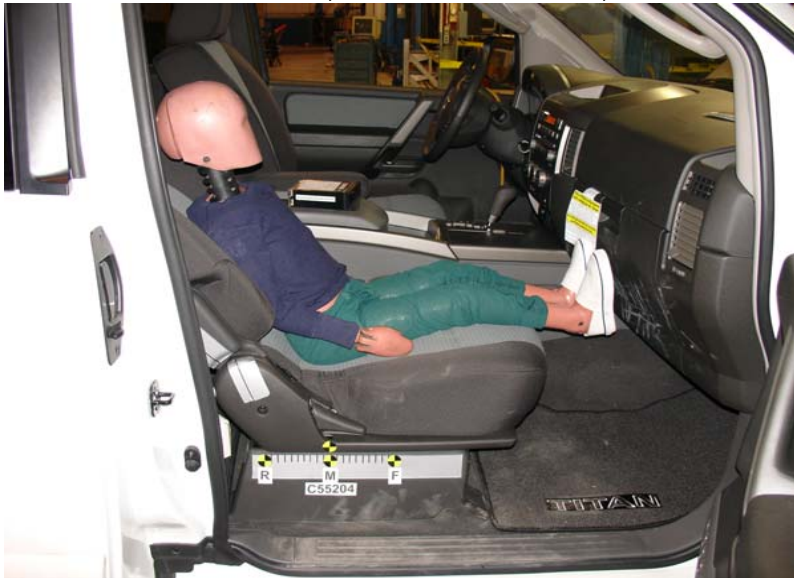
6-Year-Old Unbelted, Middle Seat Track, Position 2
