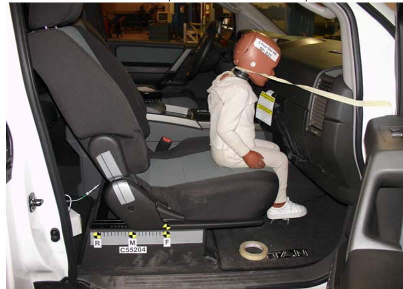
3-Year-Old Unbelted, Forward Seat Track, Position 4
