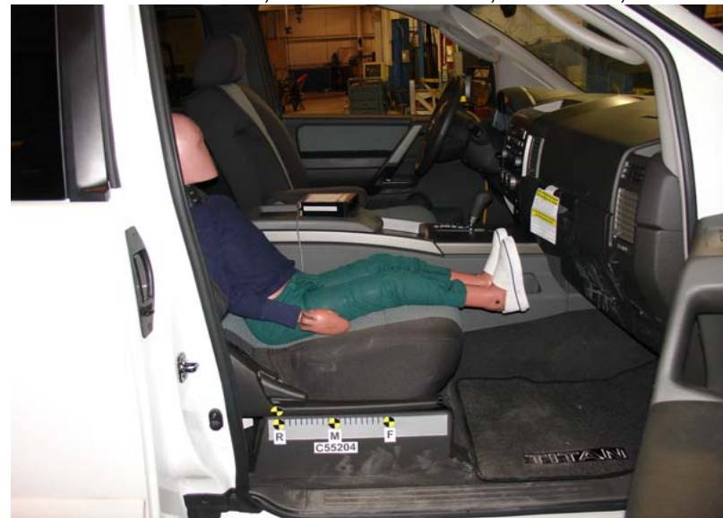
6-Year-Old Unbelted, Rearward Seat Track, Position 2
