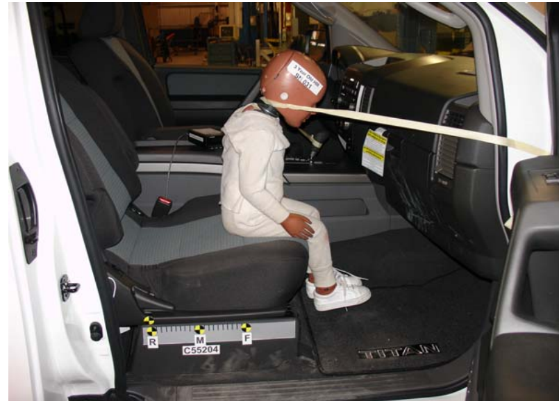
3-Year-Old Unbelted, Rearward Seat Track, Position 4
