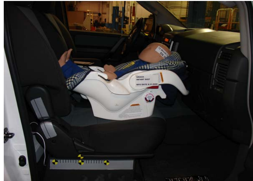
Graco Infant W/O Base Unbelted, Middle Seat Track, Handle Down
