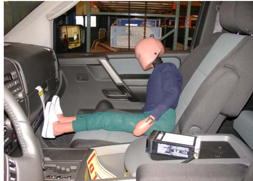
6-Year-Old Unbelted, Middle Seat Track, Position 4, View 2
