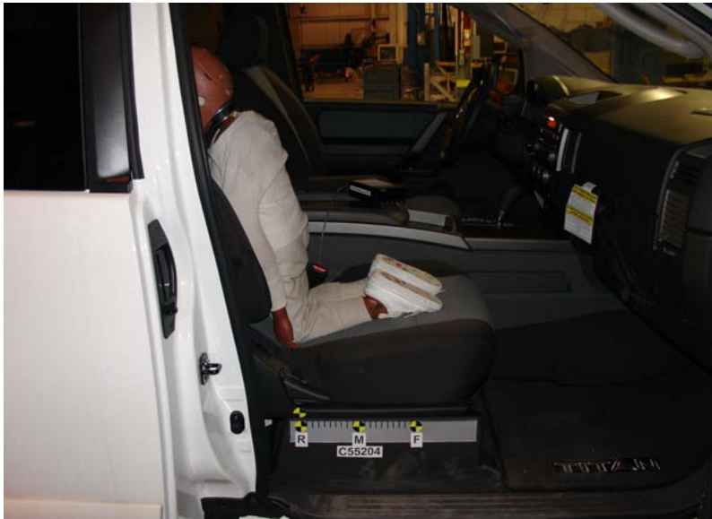
3-Year-Old Unbelted, Rearward Seat Track, Position 7
