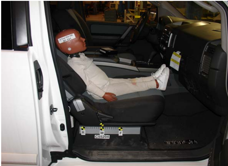
3-Year-Old Unbelted, Middle Seat Track, Position 2
