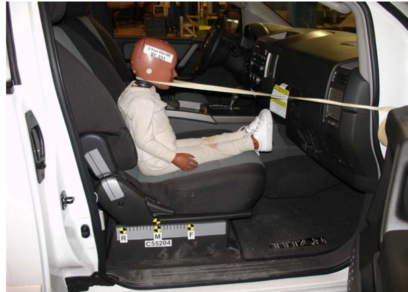
3-Year-Old Unbelted, Middle Seat Track, Position 3
