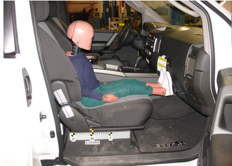
6-Year-Old Unbelted, Middle Seat Track, Position 1
