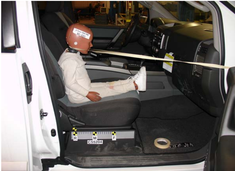
3-Year-Old Unbelted, Rearward Seat Track, Position 3
