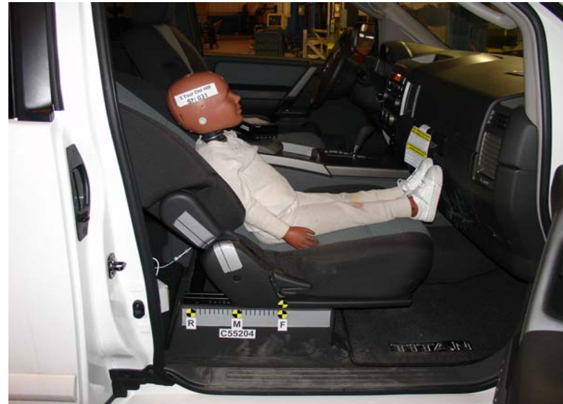
3-Year-Old Unbelted, Forward Seat Track, Position 2
