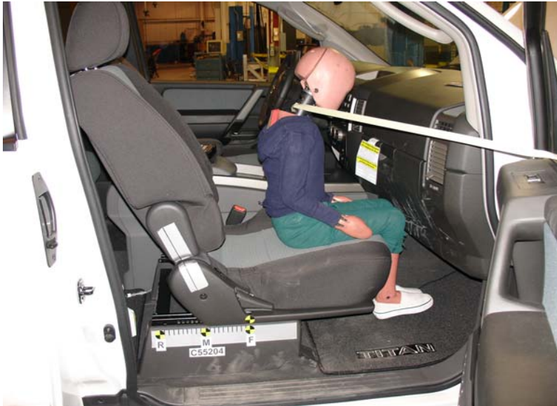
6-Year-Old Unbelted, Forward Seat Track, Position 3
