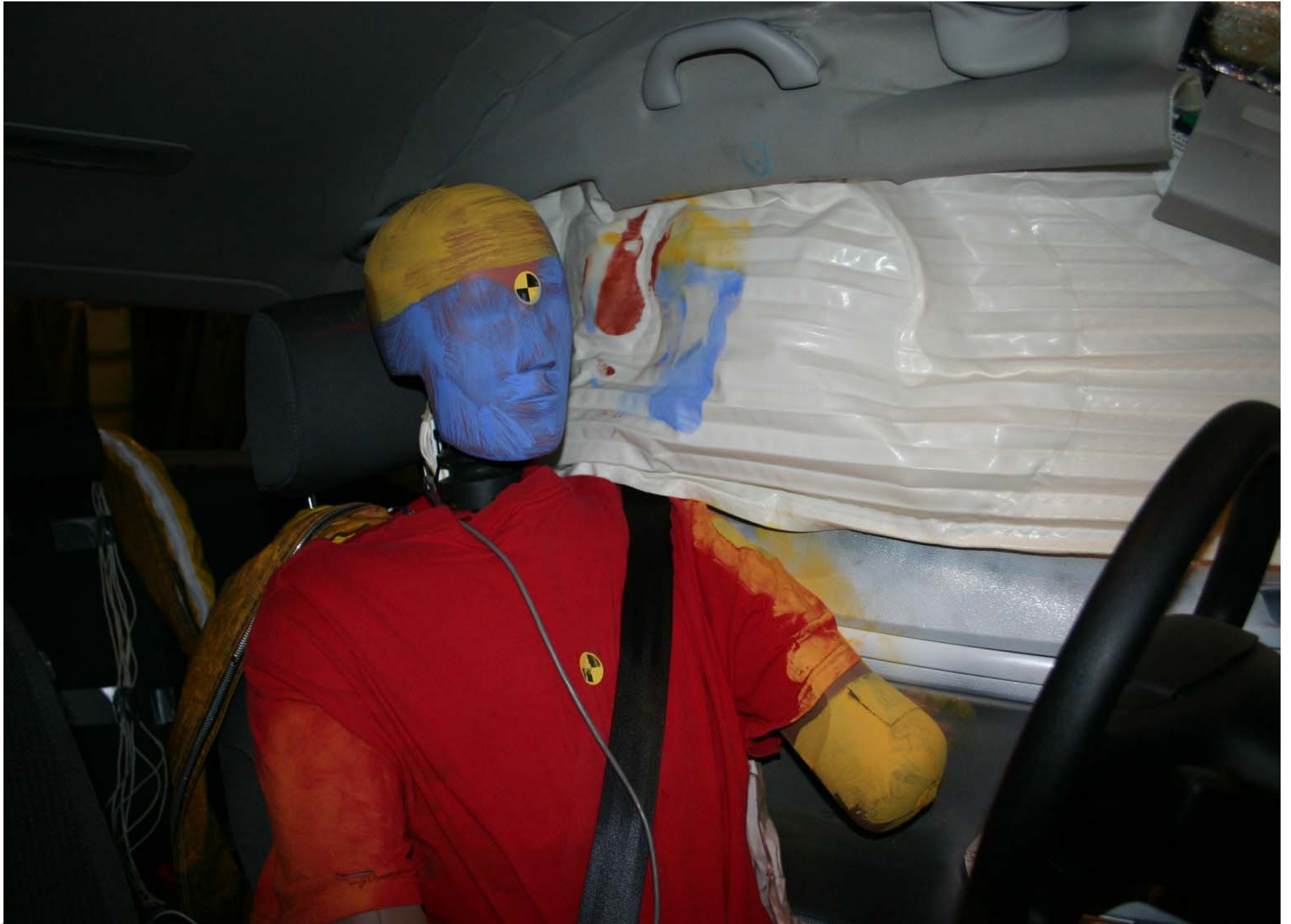
Post-Test Driver Dummy Head Contact
