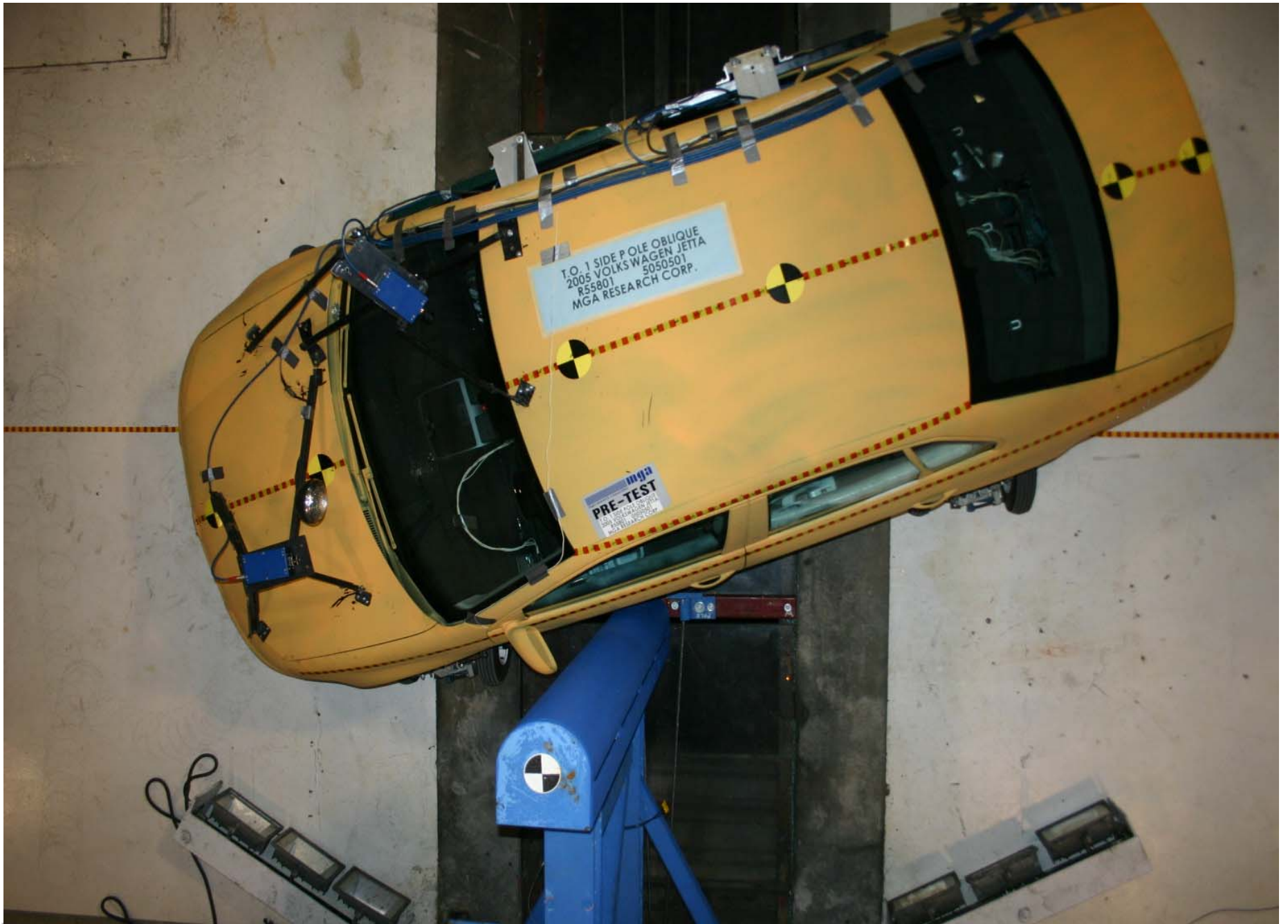
Pre-Test Vehicle Overhead View Positioned Against Pole
