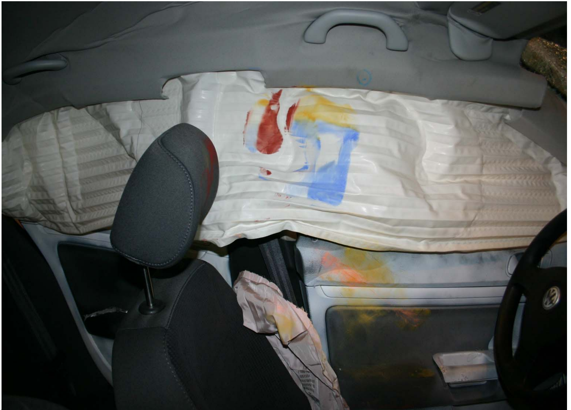
Post-Test Driver Dummy Head Contact
