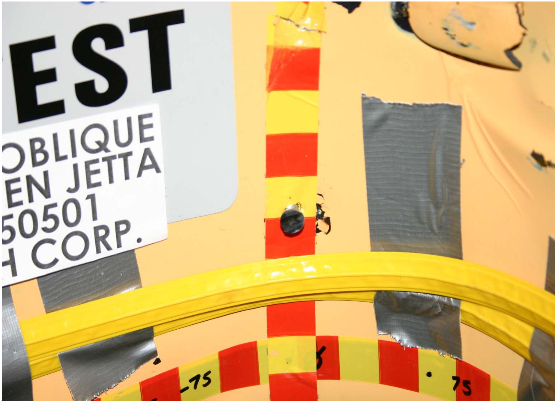
Post-Test Impact Point on Vehicle
