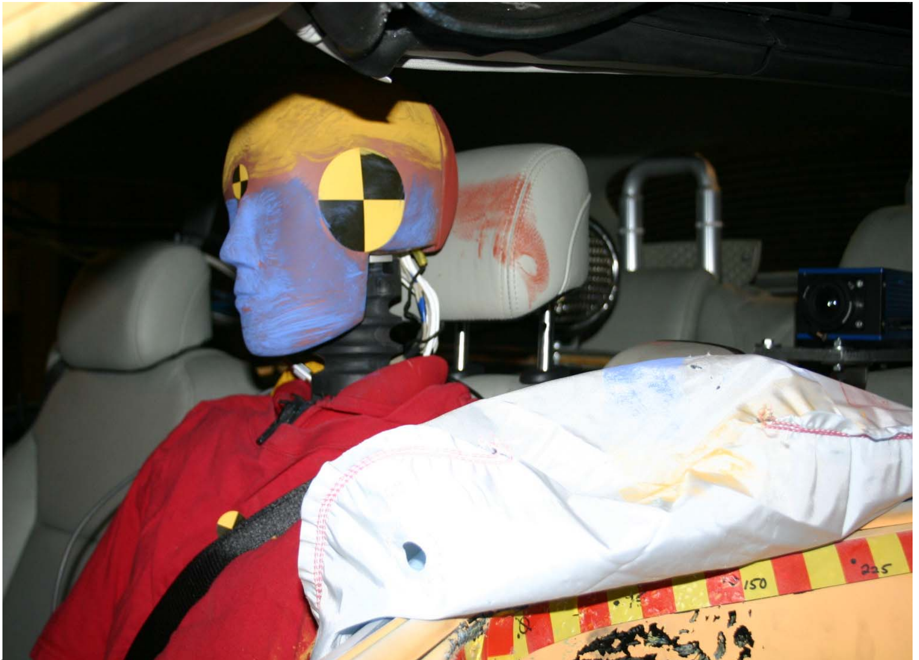
Post-Test Driver Dummy Head Contact
