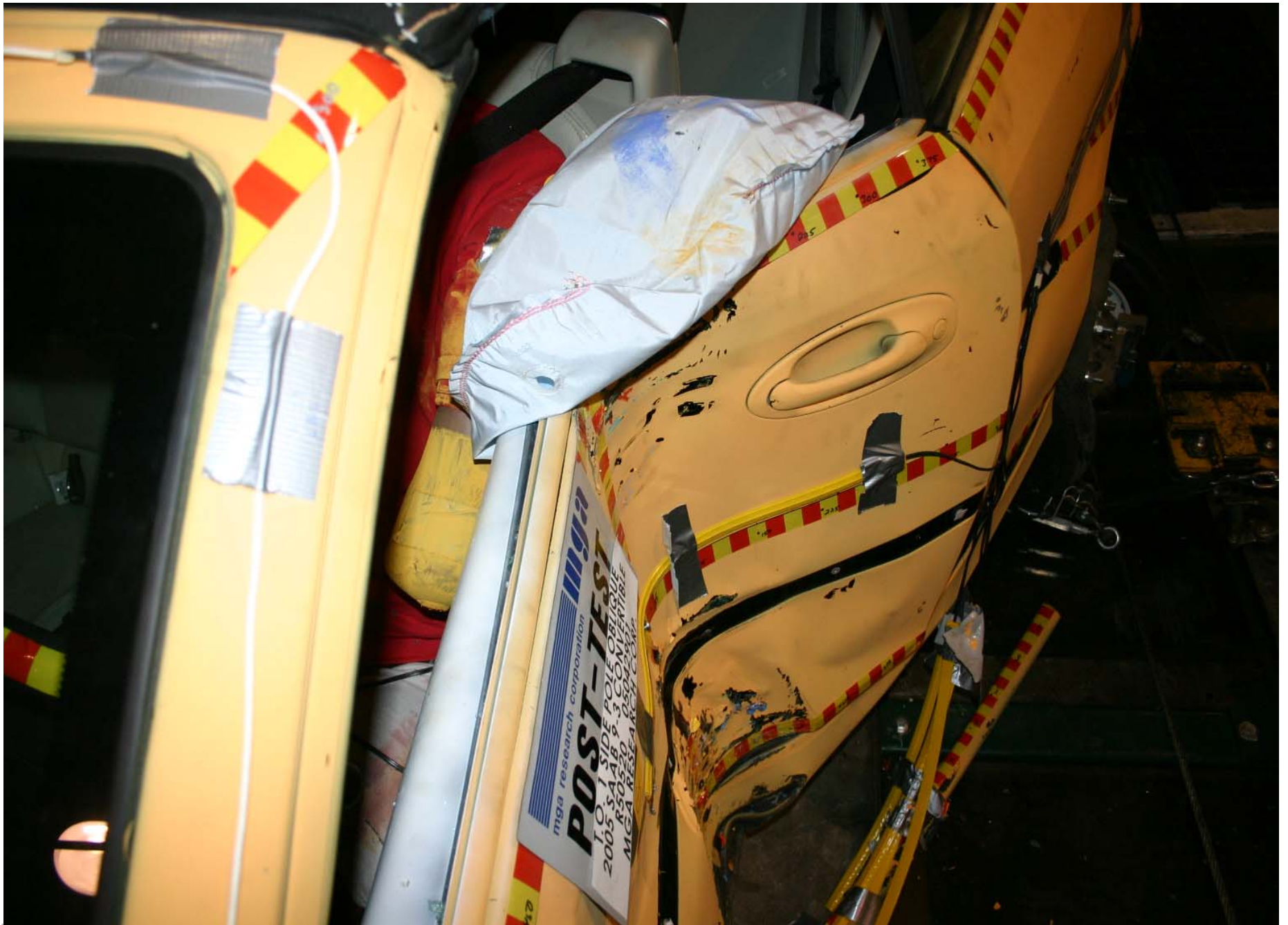
Post-Test Driver Shoulder and Door Top View
