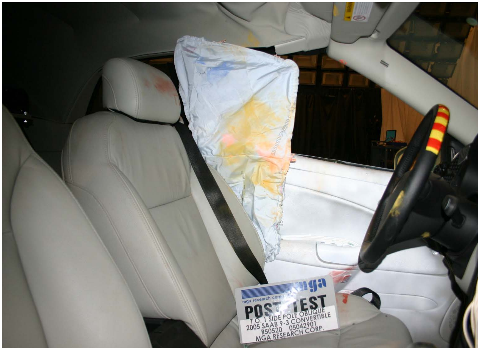
Post-Test Driver Dummy Contact
