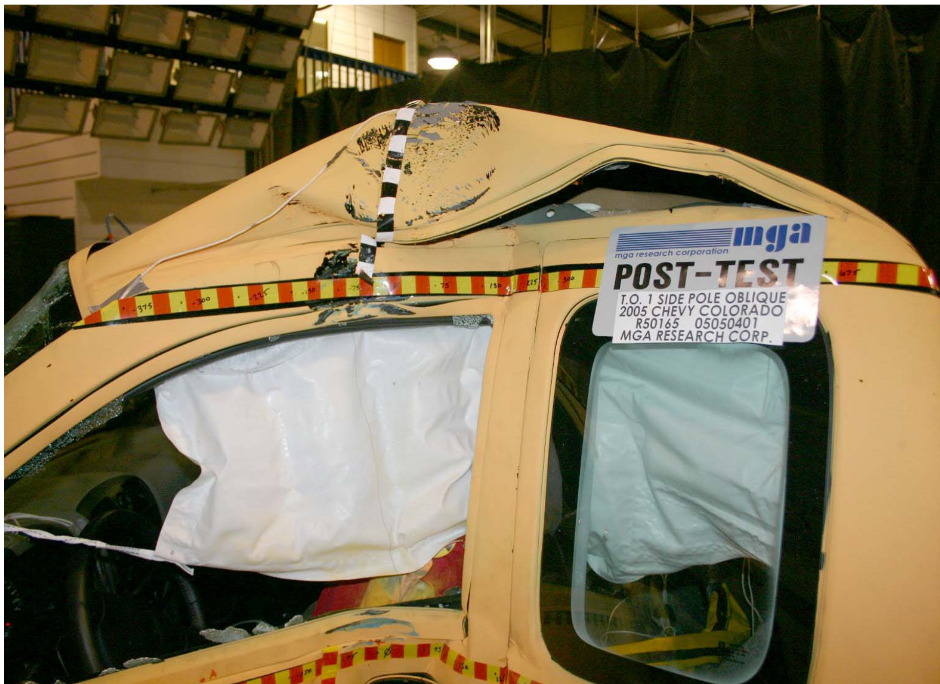
Post-Test Roof Separation View
