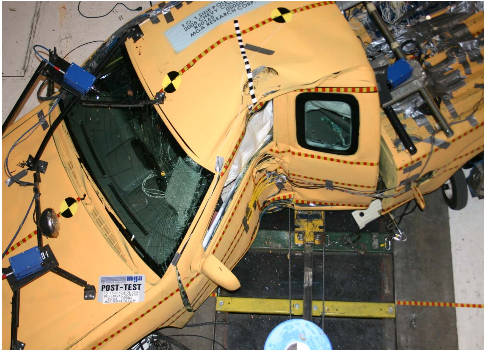
Post-Test Pole and Vehicle Overhead View (Close-Up)
