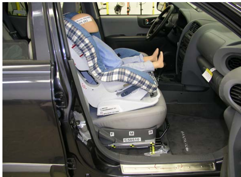
Britax Roundabout 161 Fwd Facing Unbelted, Rearward Seat Track
