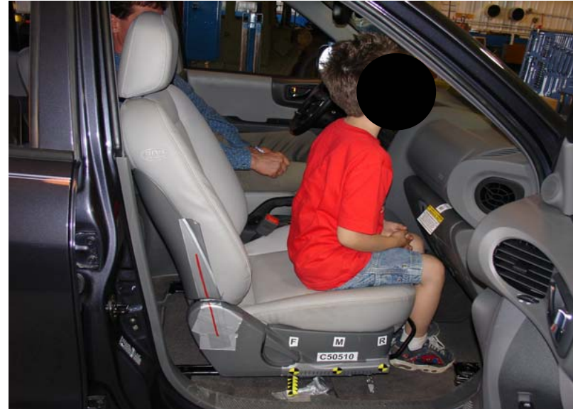
6-Year-Old Unbelted, Forward Seat Track, Position 4, Human Subject 06
