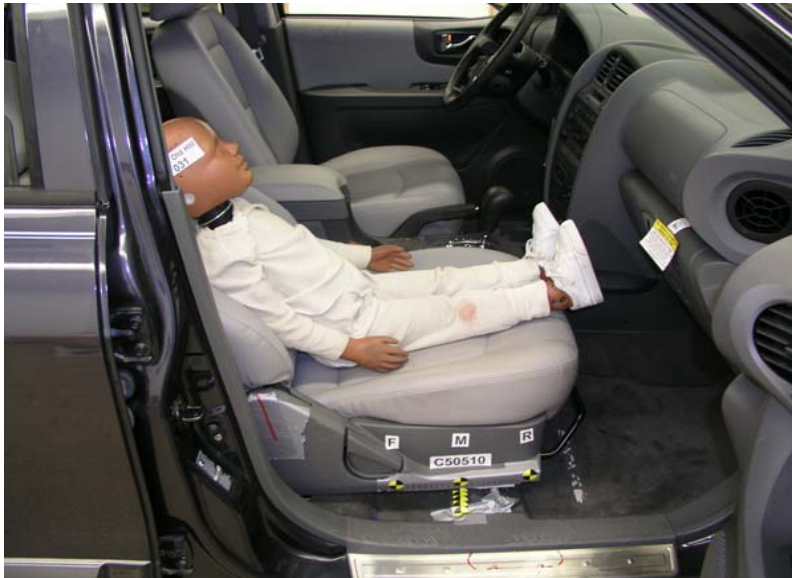
3-Year-Old Unbelted, Middle Seat Track, Position 2
