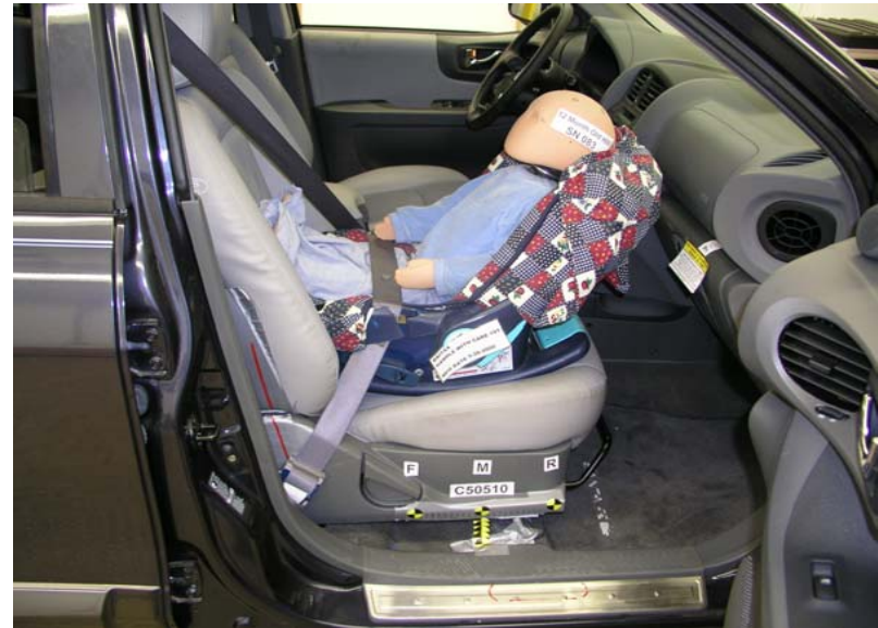
Britax Handle With Care 191 With Belt, Middle Seat Track, Handle Down
