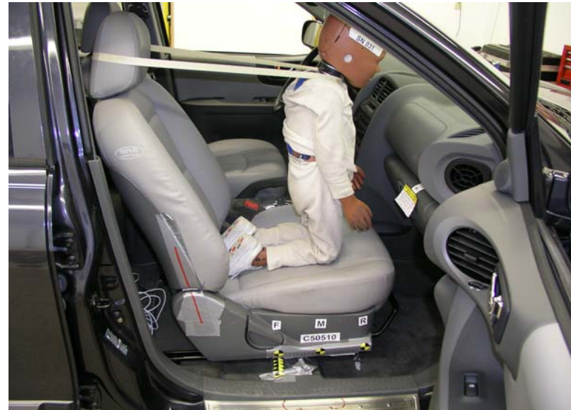
3-Year-Old Unbelted, Forward Seat Track, Position 6
