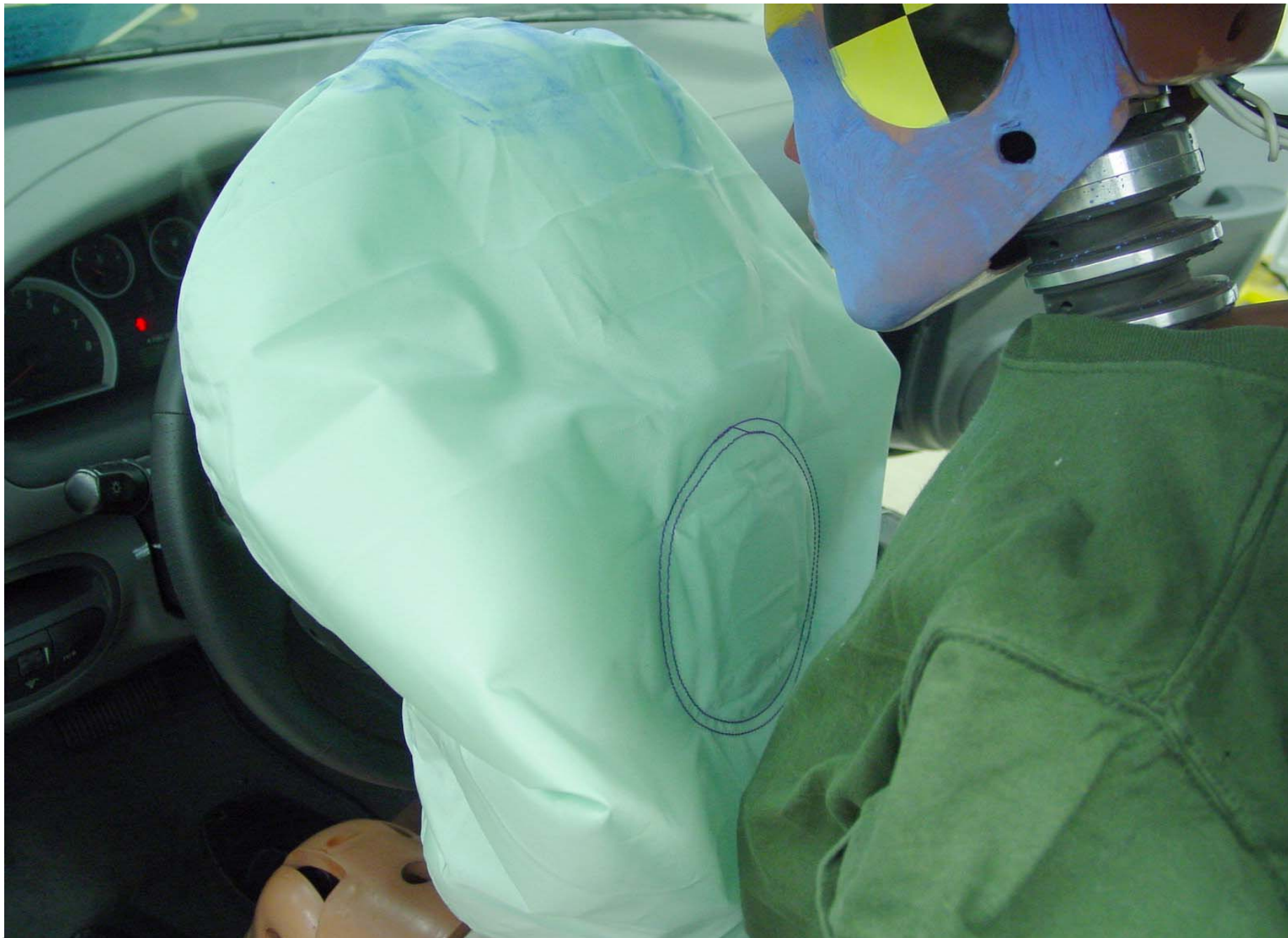
Post-Test 5th Fem. P2 Driver Dummy Airbag Left View
