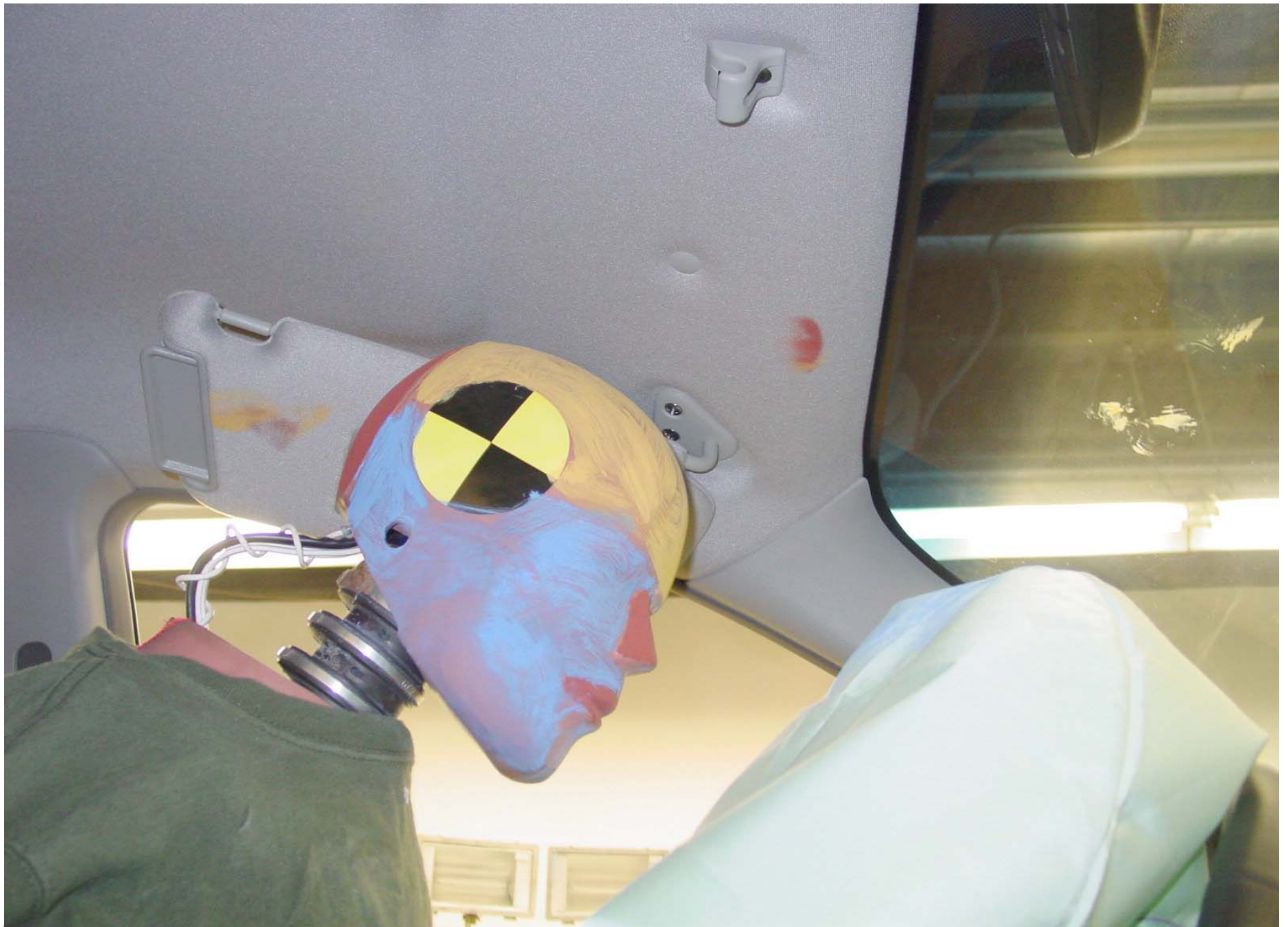
Post-Test 5th Fem. P2 Driver Dummy Right Side Head Position View
