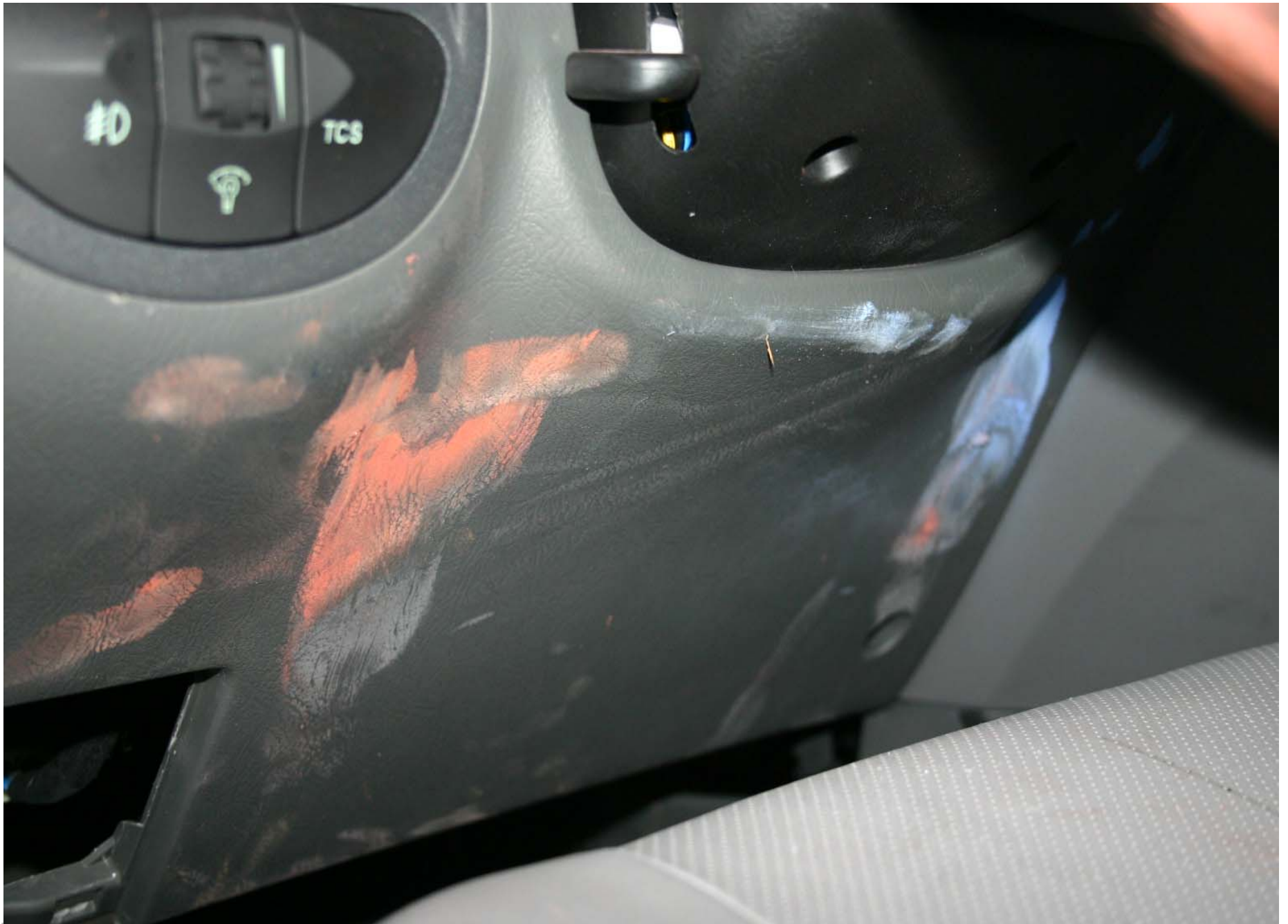
Post-Test Driver Dummy Knee Contact
