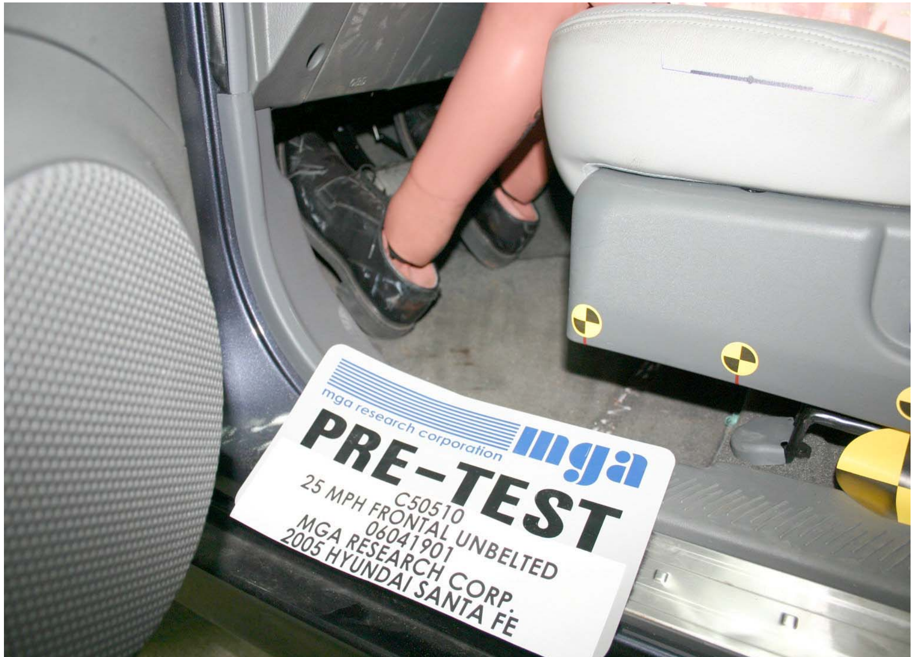
Pre-Test Driver Dummy Feet Position
