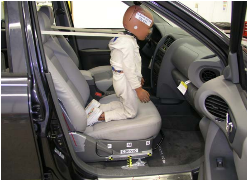
3-Year-Old Unbelted, Middle Seat Track, Position 6
