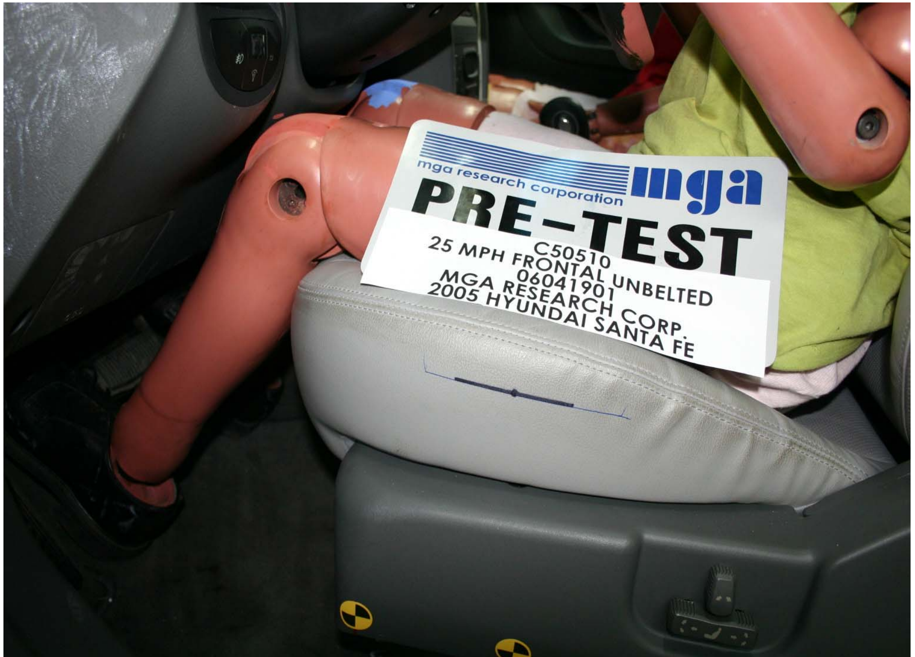
Pre-Test Driver Side Knee Bolster View
