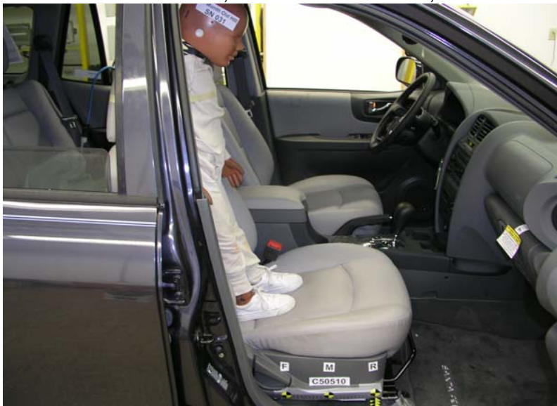
3-Year-Old Unbelted, Rearward Seat Track, Position 5
