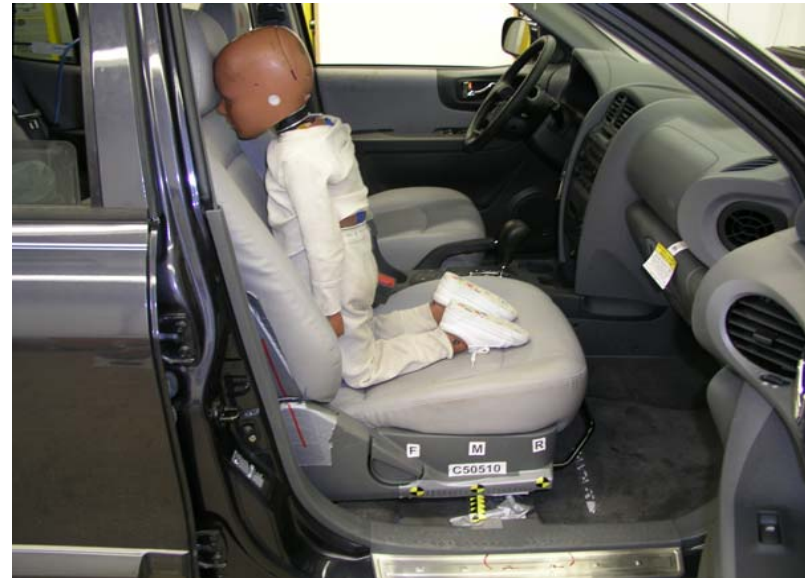
3-Year-Old Unbelted, Middle Seat Track, Position 7
