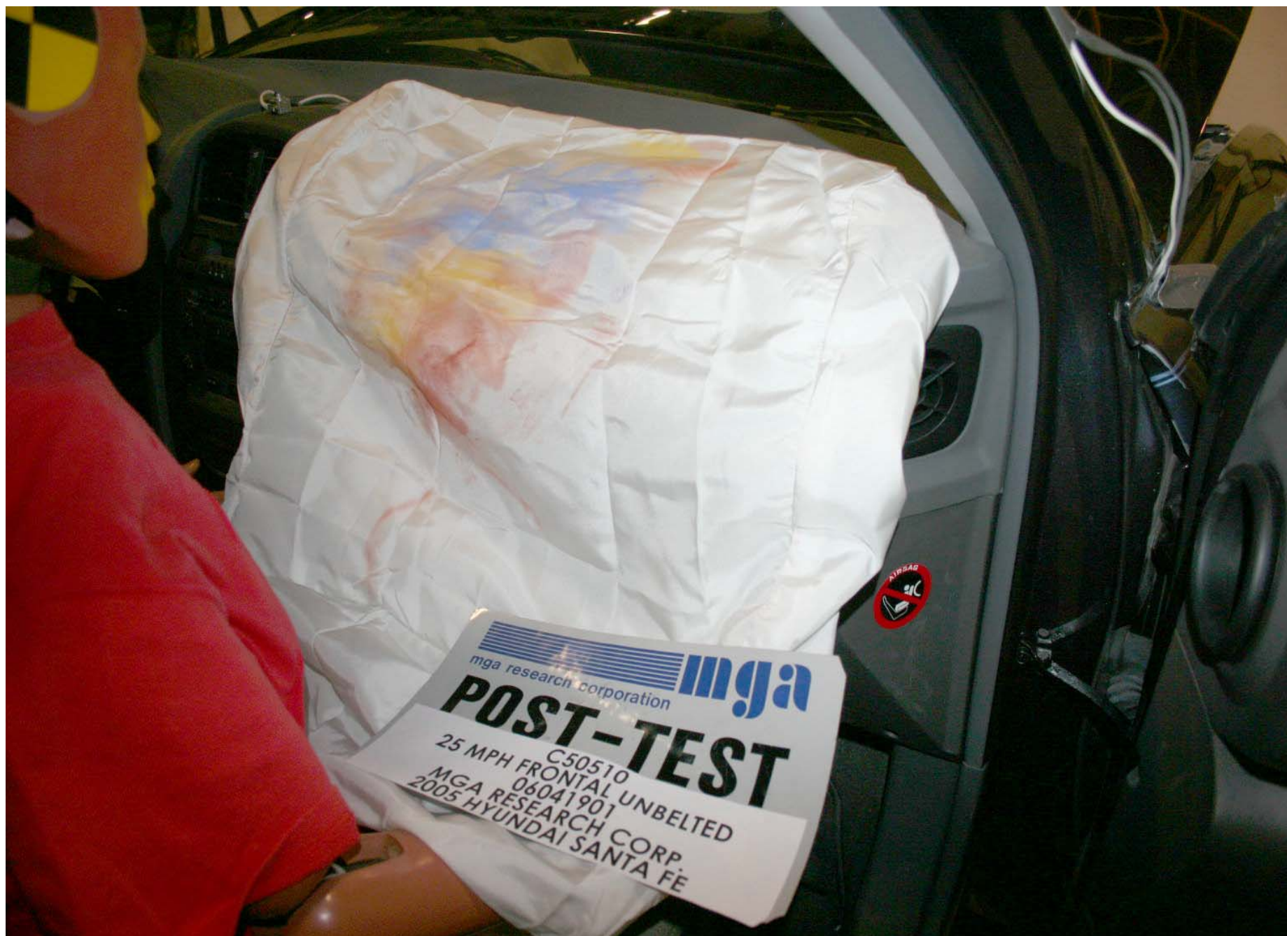
Post-Test Passenger Dummy Airbag Contact
