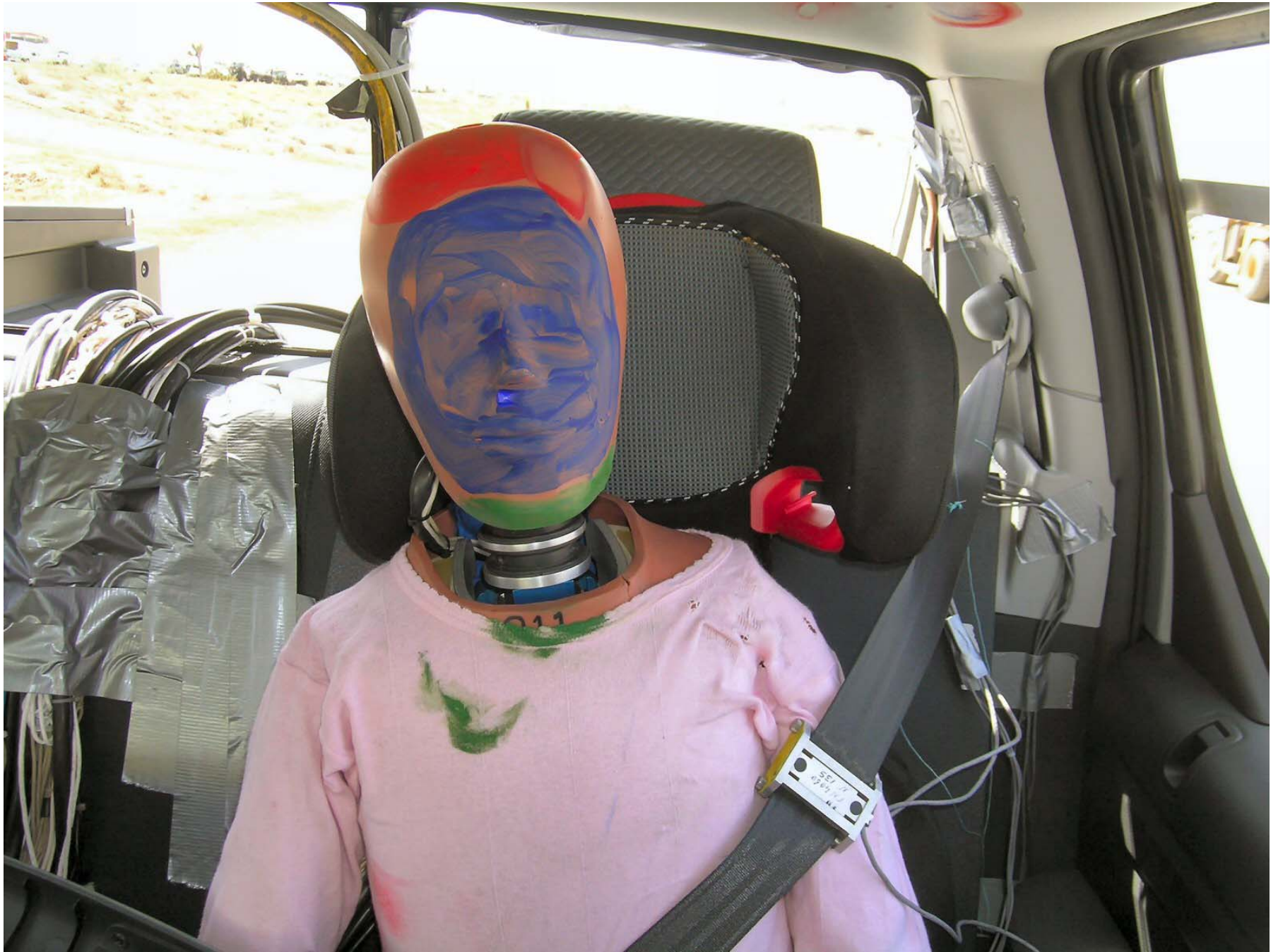
Figure F2-29: Post-Test Position 4 Front View (Head Position)
