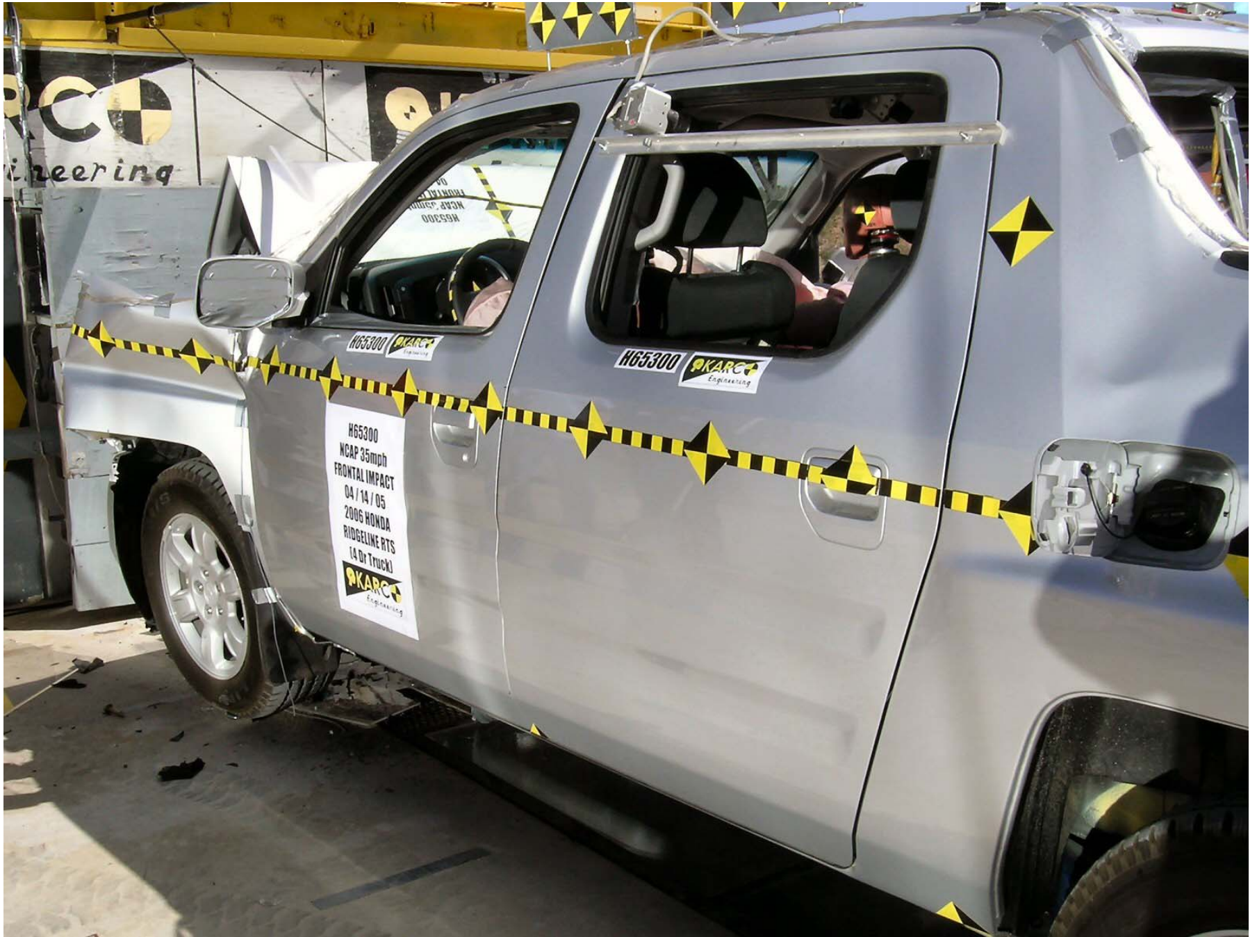
Figure A-16: Post-Test Left Side ¾ View of Doors After Impact
