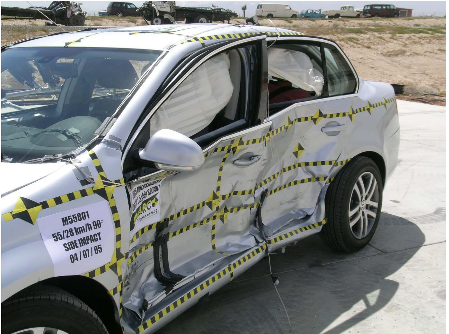
Figure A-28: Post-Test Front ¾ View of Left Side Doors
