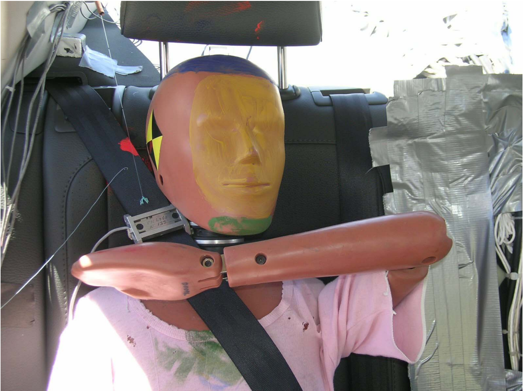
Figure F2-2: Post-Test Position 3 Front View (Head Position)
