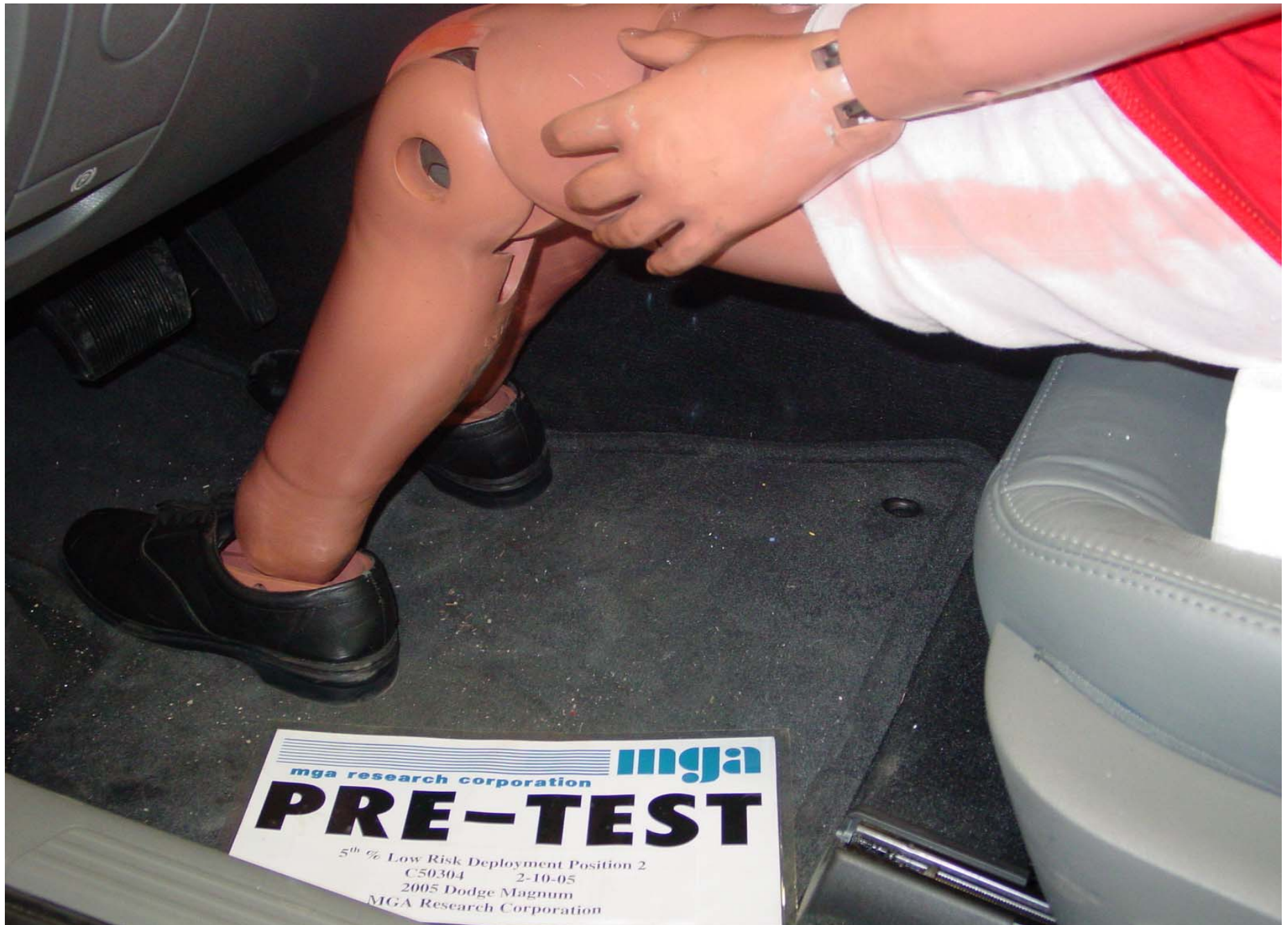
Pre-Test 5th Fem. P2 Driver Dummy Left Side Knee Position View
