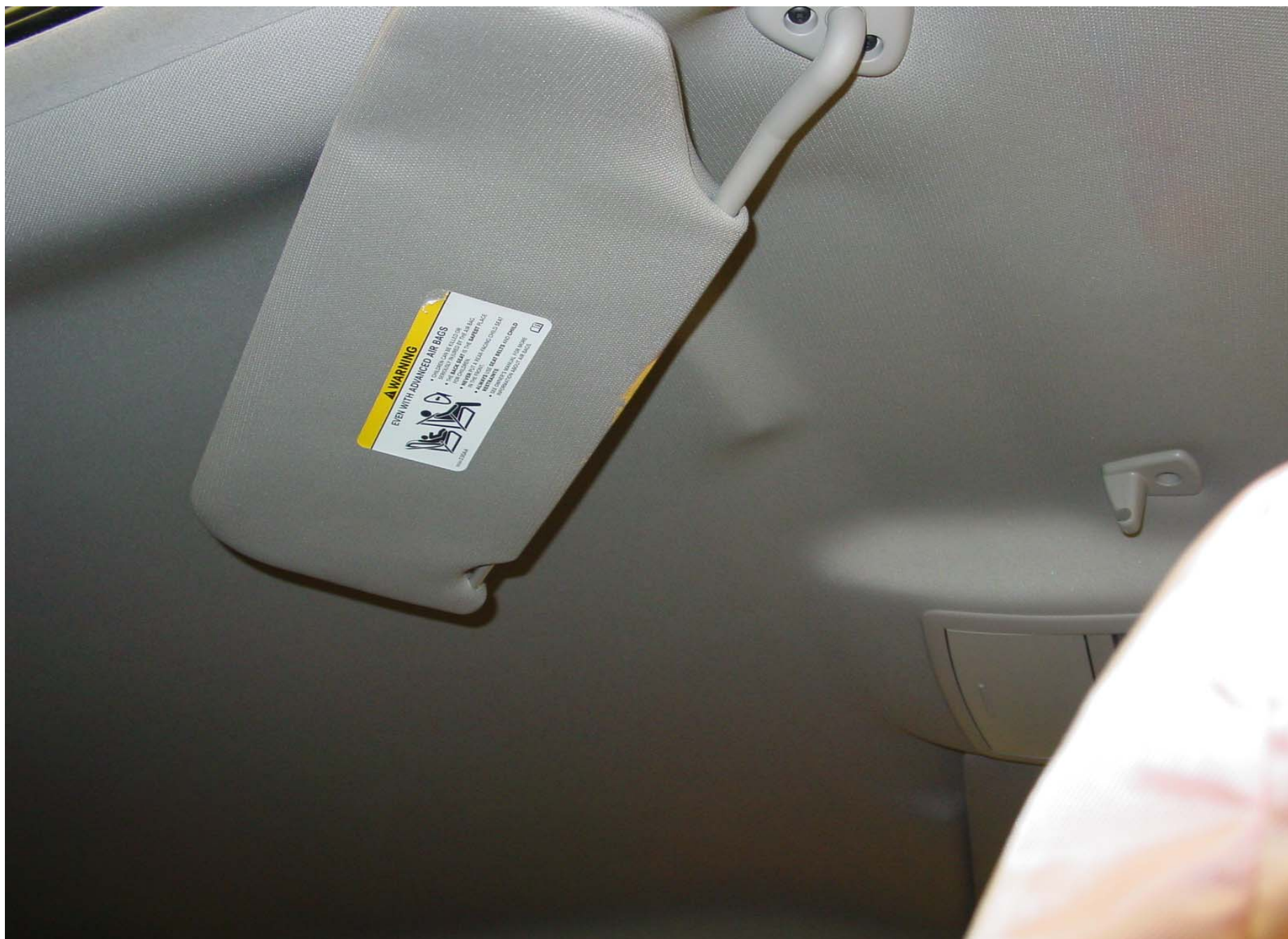
Post-Test 6YO P1 Passenger Dummy Head Contact View (Visor)
