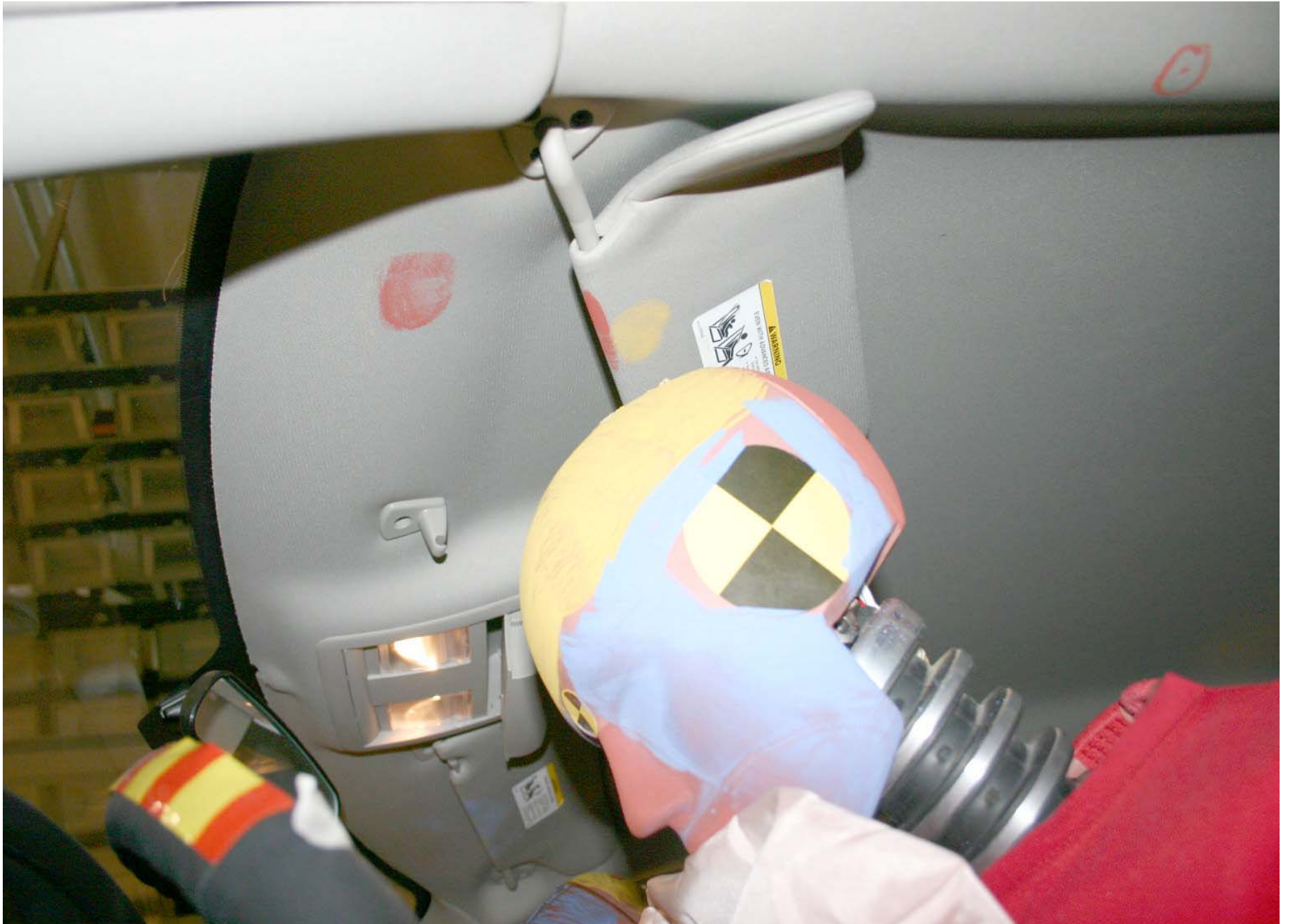
Post-Test Driver Dummy Head Contact (visor)
