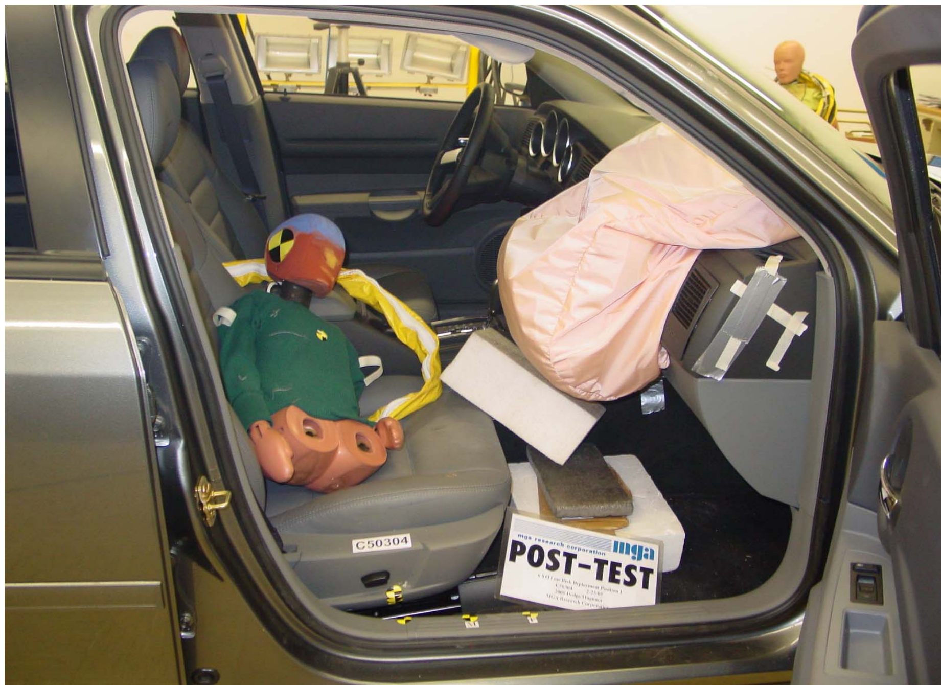
Post-Test 6YO P1 Passenger Dummy Right Side View (Door Open)
