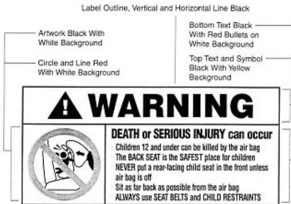
Figure 6a. Sun Visor Label Visible When Visor is in Down Position.
