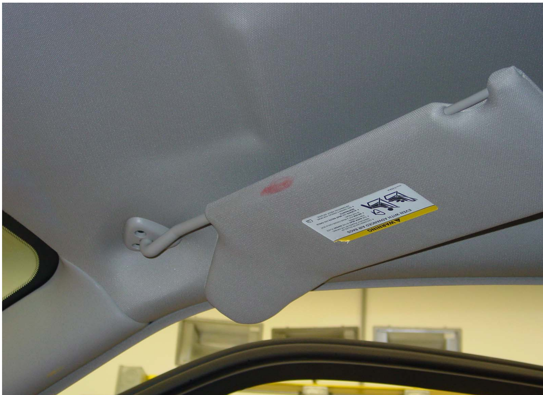
Post-Test 3YO P1 Passenger Dummy Head Contact View (Visor)
