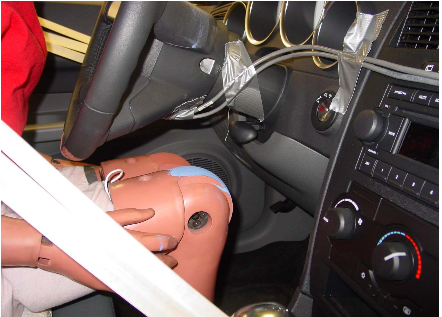
Pre-Test 5th Fem. P1 Driver Dummy Right Side Knee Position View
