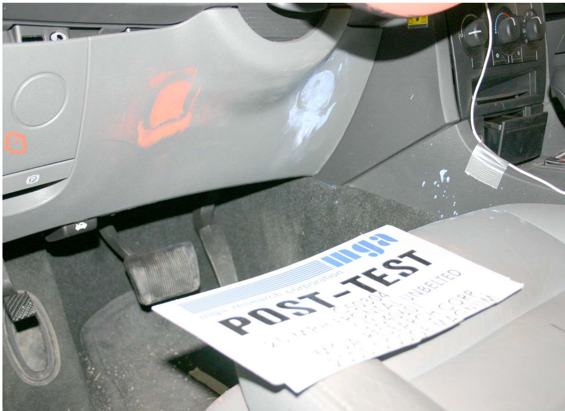
Post-Test Driver Knee Contact
