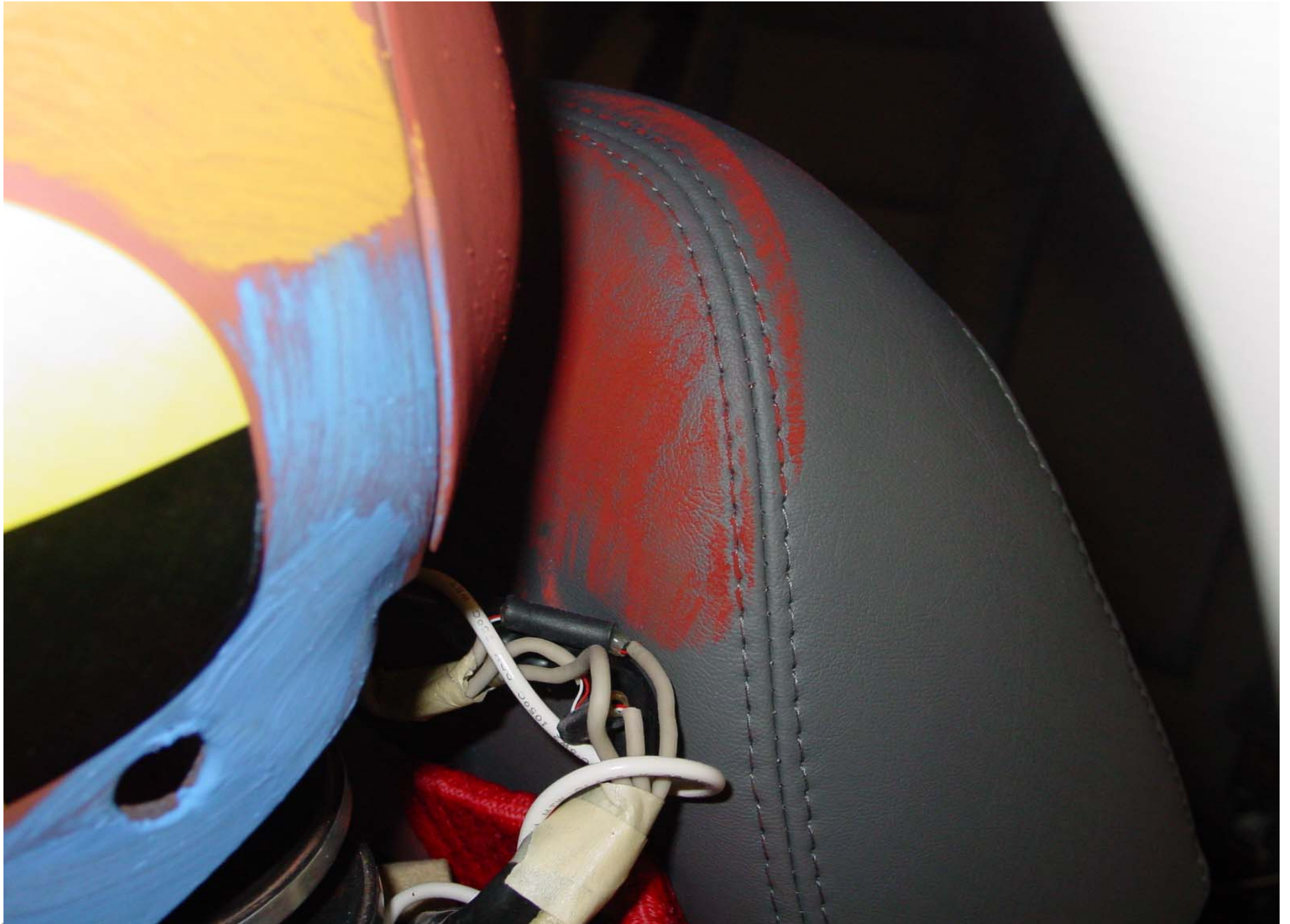
Post-Test 5th Fem. P2 Driver Dummy Head Contact View
