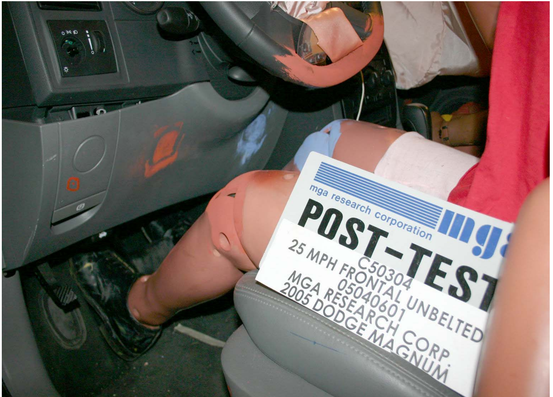
Post-Test Driver Side Knee Bolster View
