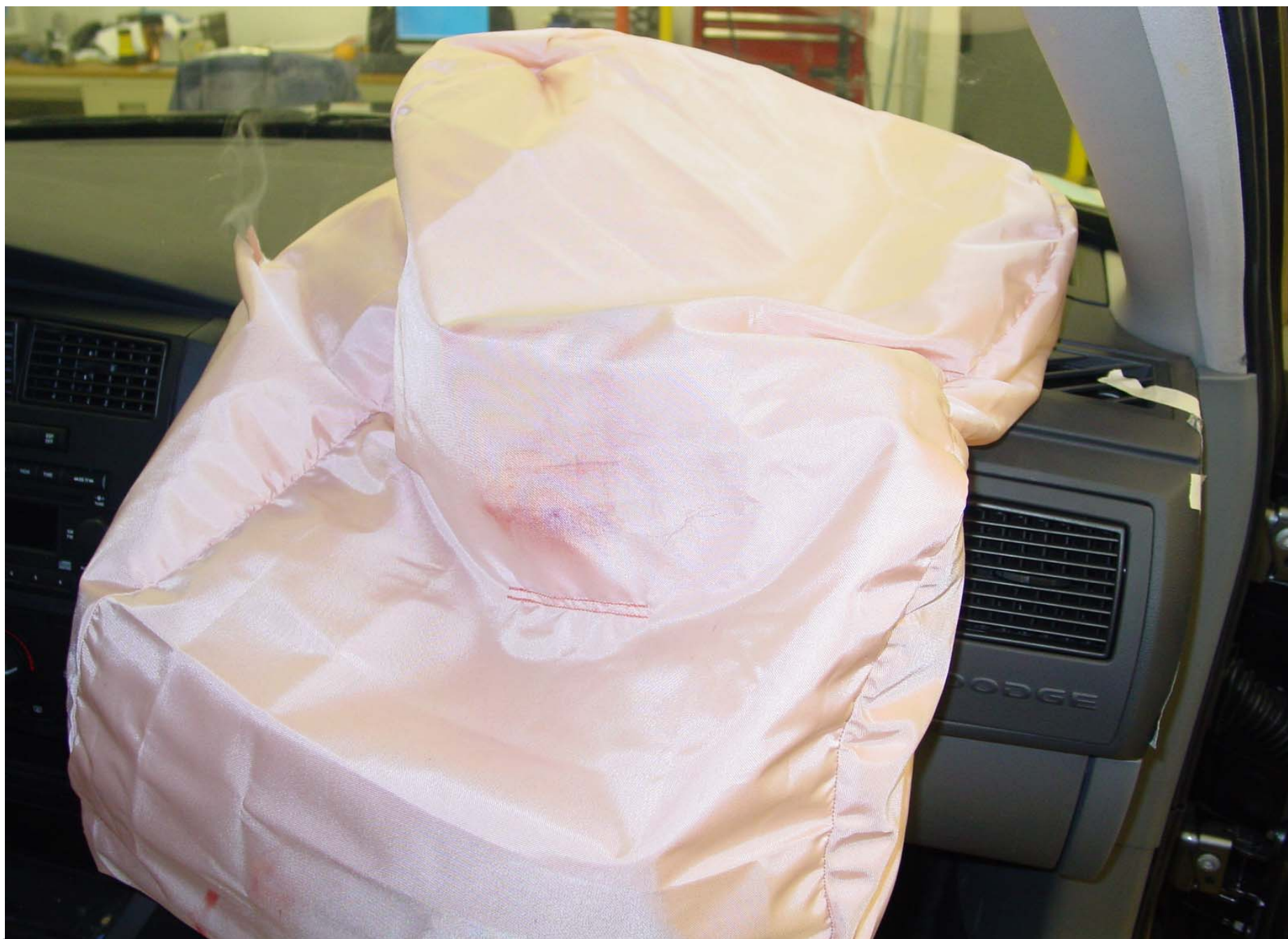
Post-Test 6YO P1 Passenger Dummy Airbag Contact View
