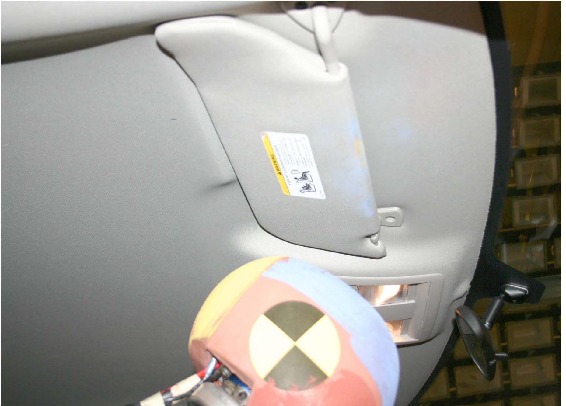
Post-Test Passenger Dummy Head Contact
