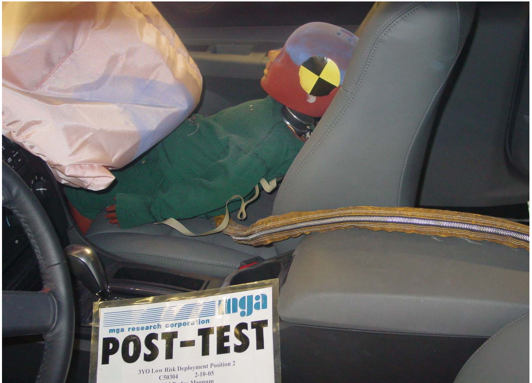
Post-Test 3YO P2 Passenger Dummy Left Side View (Door Open)
