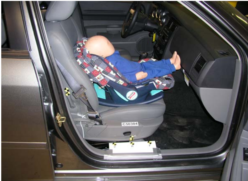
Britax Handle With Care 191 Fwd Facing Unbelted, Middle Seat Track, Handle Down
