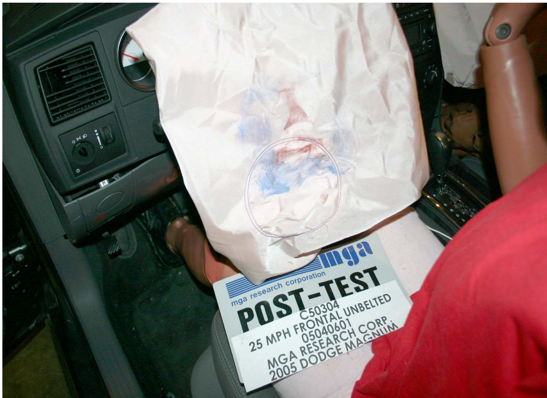
Post-Test Driver Dummy Airbag Contact
