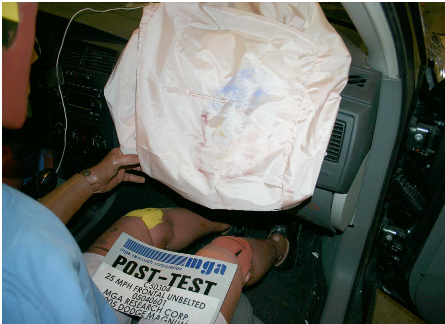
Post-Test Passenger Dummy Airbag Contact
