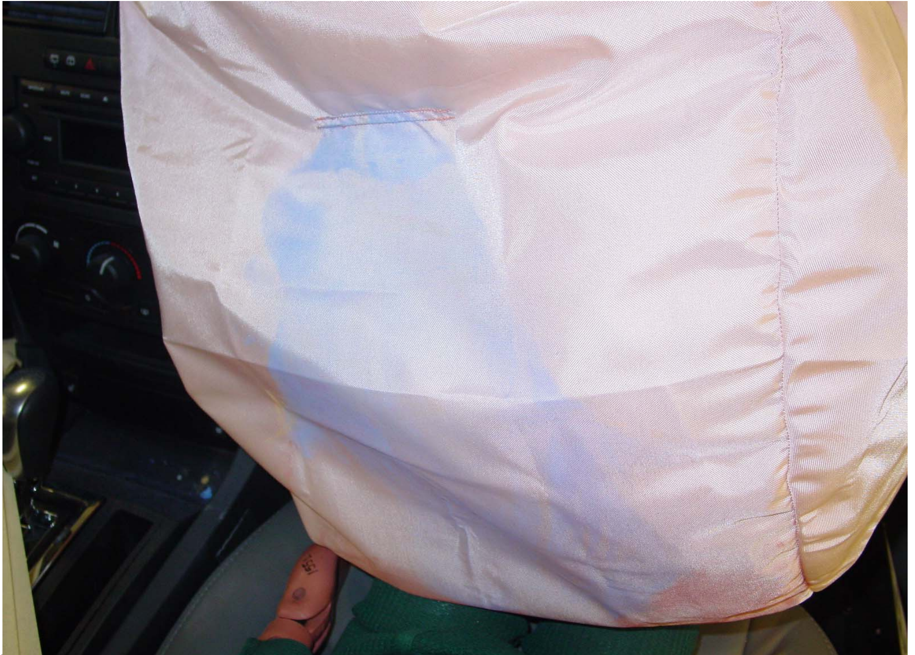
Post-Test 6YO P2 Passenger Dummy Airbag Contact View
