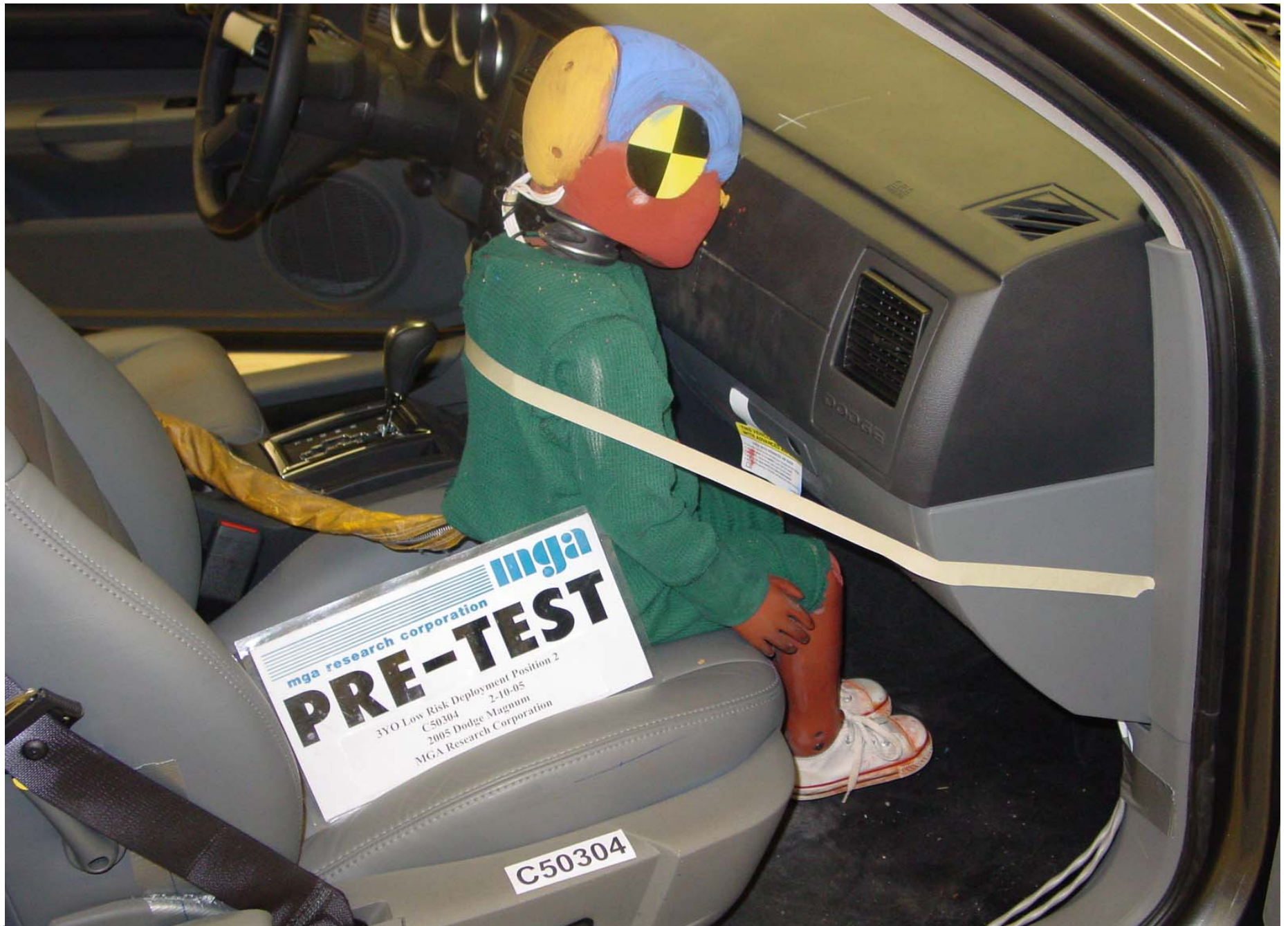
Pre-Test 3YO P2 Passenger Dummy Right Side View (Door Open)
