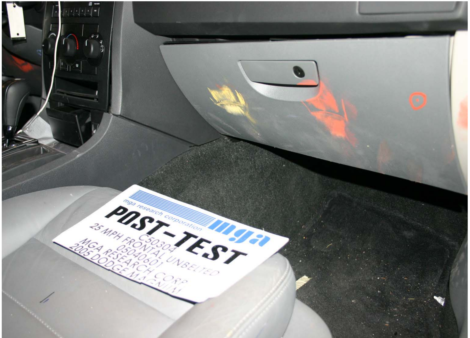
Post-Test Passenger Dummy Knee Contact
