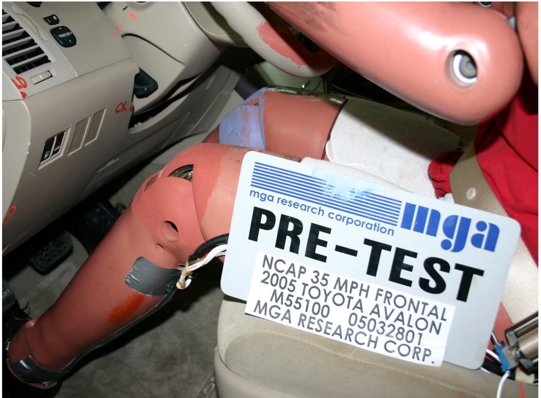
Pre-Test Driver Side Knee Bolster View
