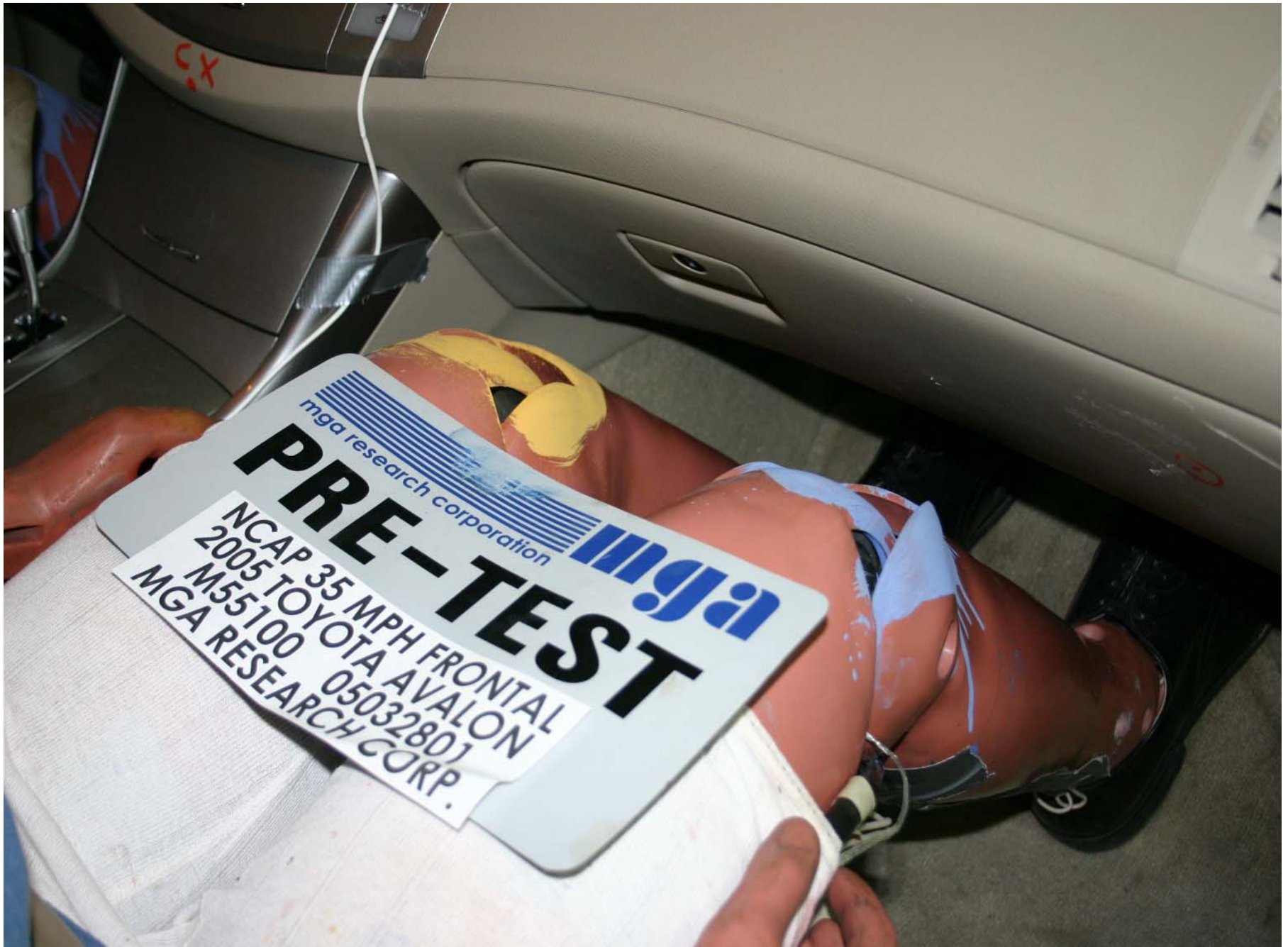
Pre-Test Passenger Side Knee Bolster View
