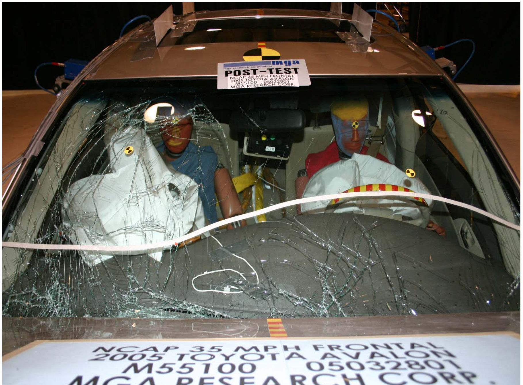
Post-Test Windshield View
