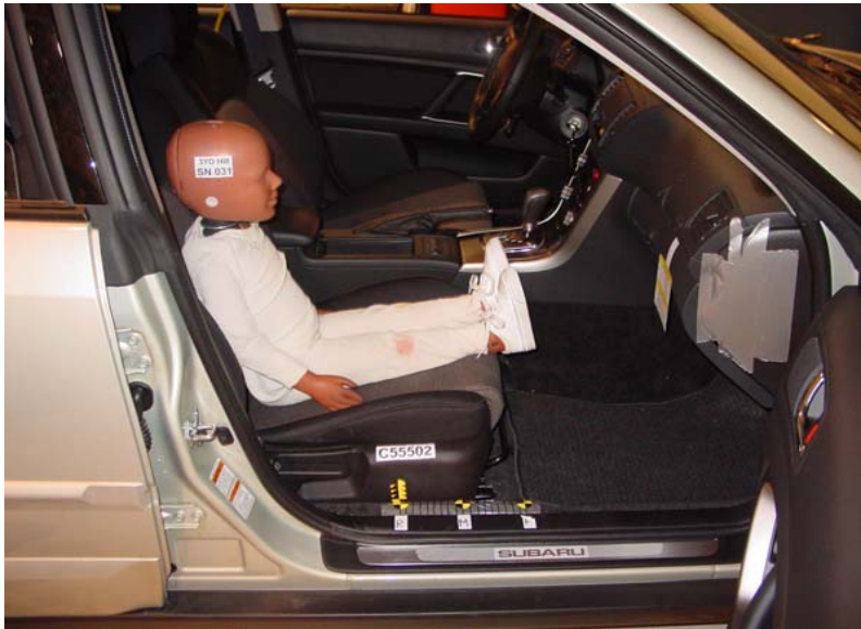
3-Year-Old Unbelted, Rearward Seat Track, Position 1
