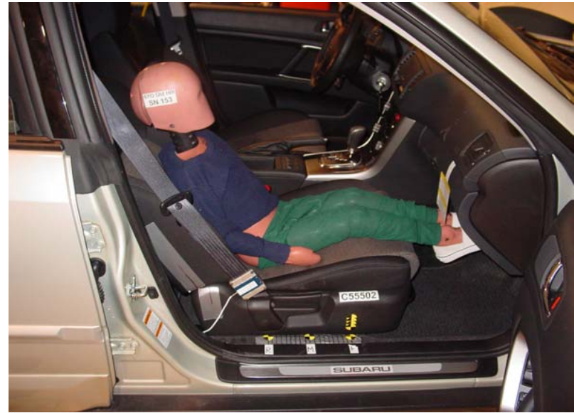
6-Year-Old Unbelted, Forward Seat Track, Position 2
