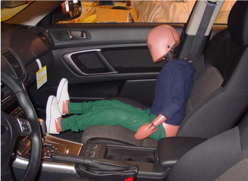
6-Year-Old Unbelted, Rearward Seat Track, Position 4, View 2
