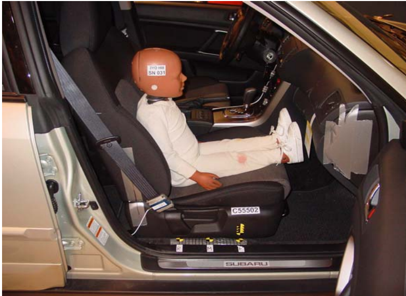
3-Year-Old Unbelted, Forward Seat Track, Position 1
