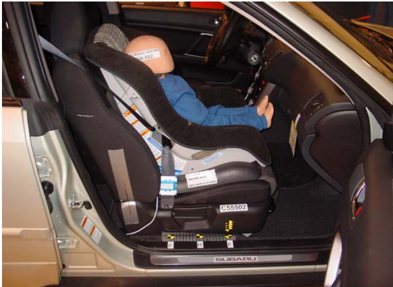
Century Encore Fwd Facing With Belt, Forward Seat Track
