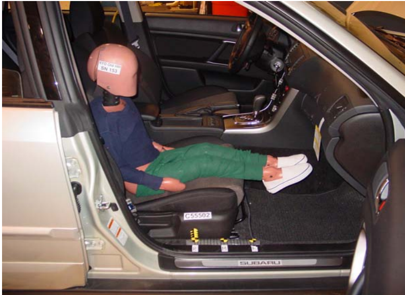
6-Year-Old Unbelted, Rearward Seat Track, Position 1
