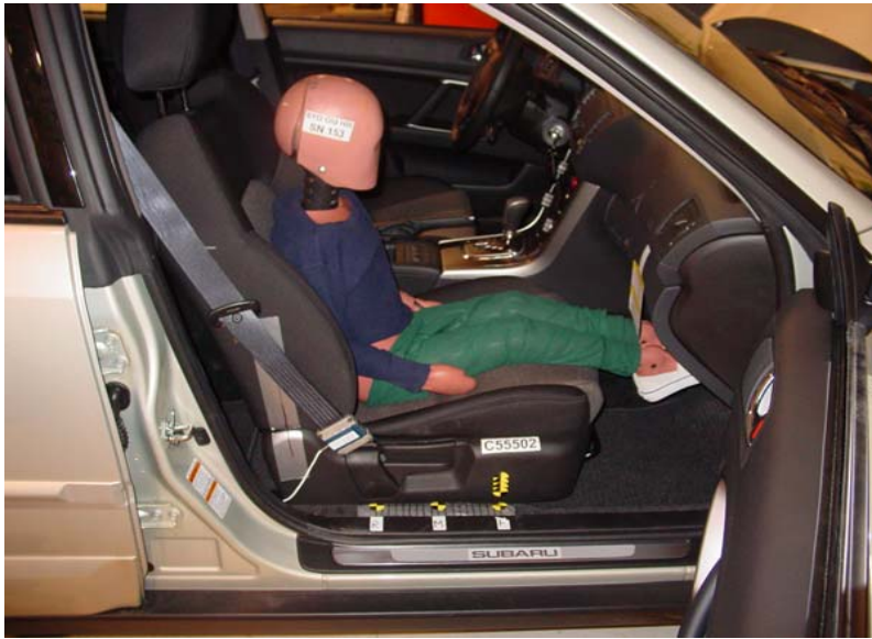
6-Year-Old Unbelted, Forward Seat Track, Position 1
