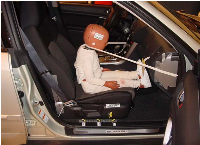
3-Year-Old Unbelted, Forward Seat Track, Position 3
