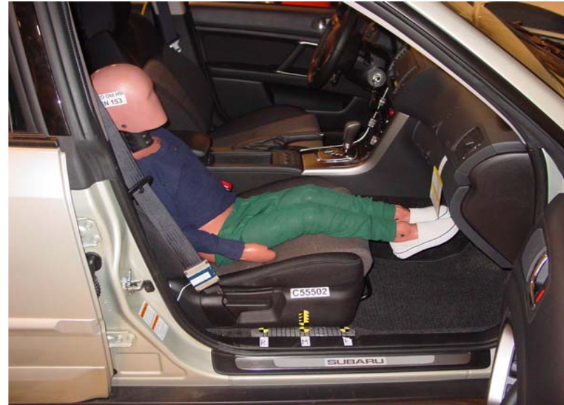
6-Year-Old Unbelted, Middle Seat Track, Position 2
