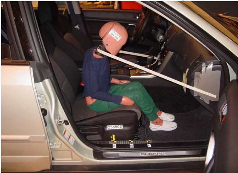
6-Year-Old Unbelted, Rearward Seat Track, Position 3
