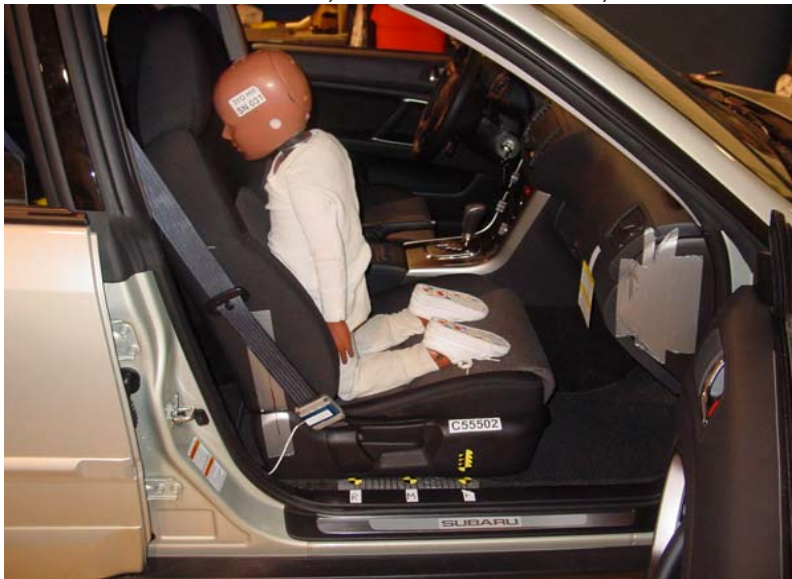
3-Year-Old Unbelted, Forward Seat Track, Position 7
