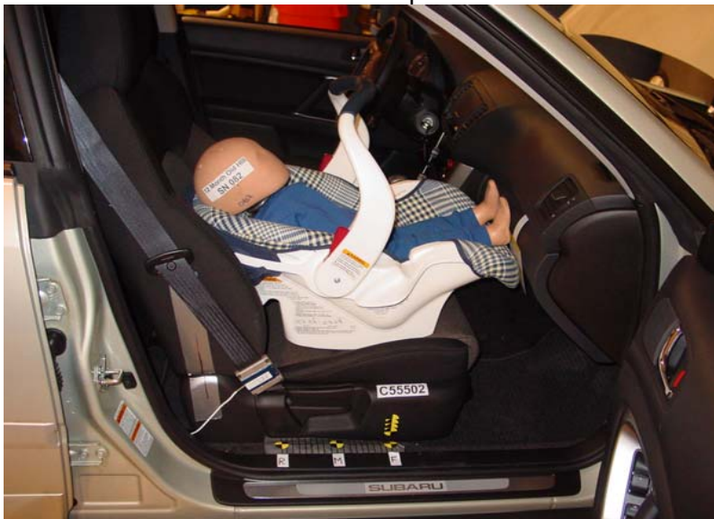
Graco Infant W/O Base Fwd Facing Unbelted, Forward Seat Track, Handle Up
