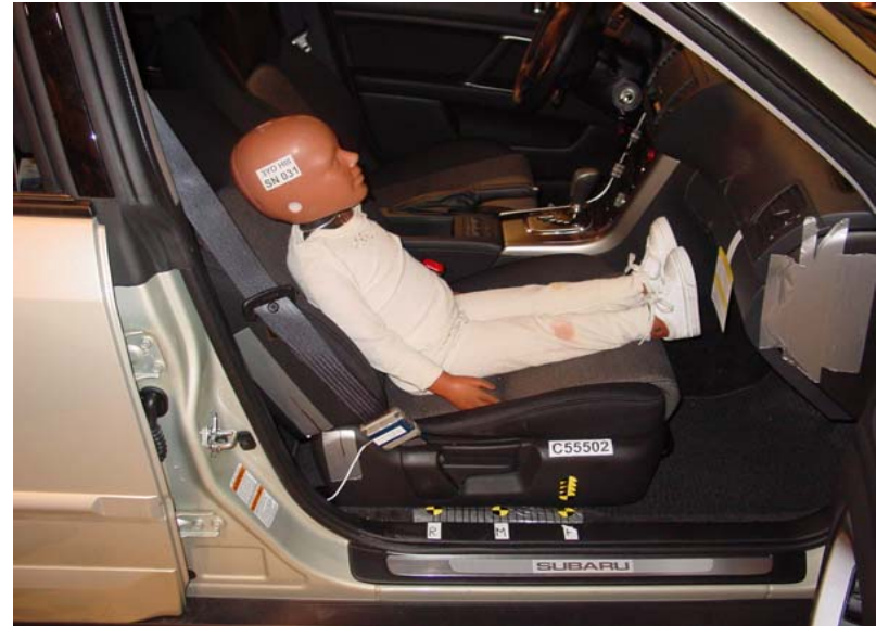
3-Year-Old Unbelted, Forward Seat Track, Position 2
