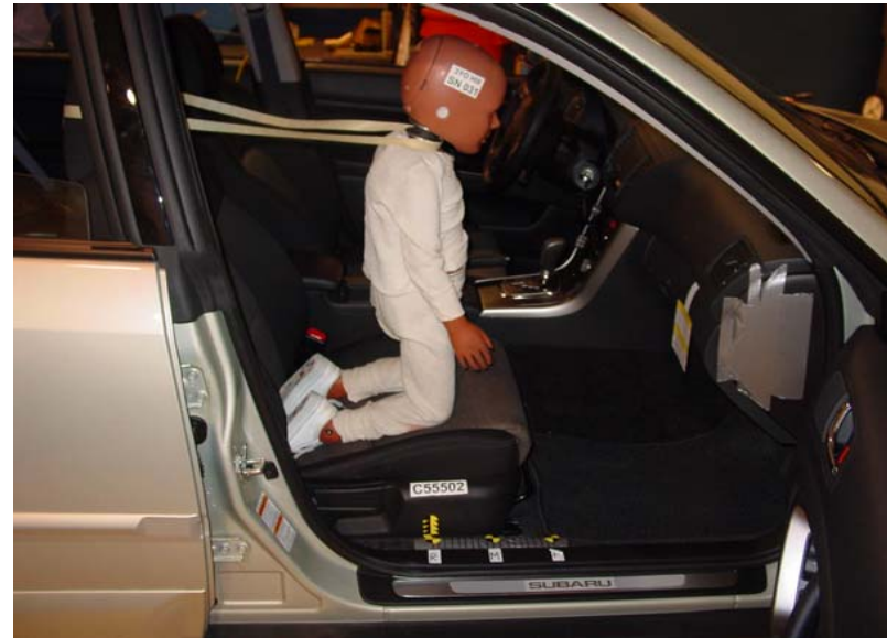
3-Year-Old Unbelted, Rearward Seat Track, Position 6
