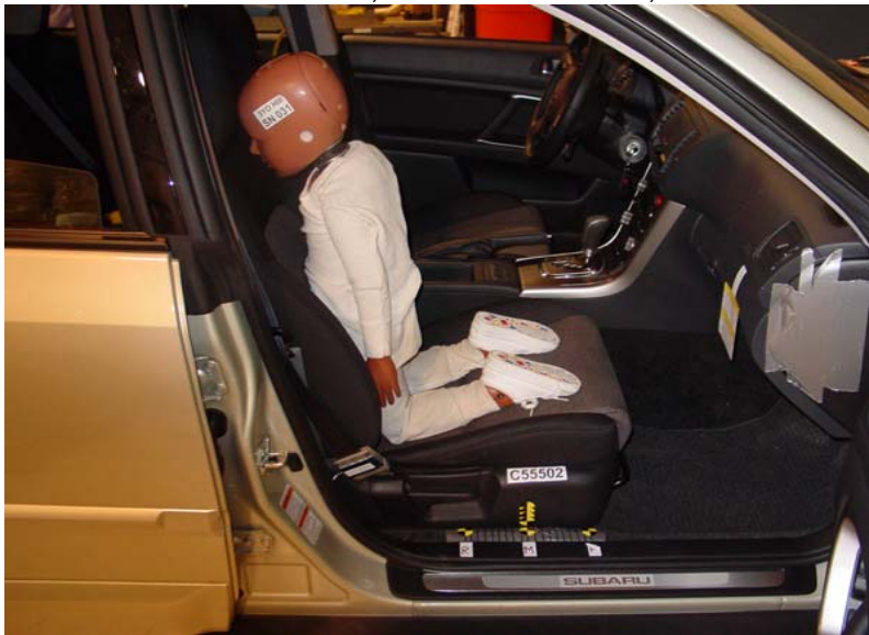
3-Year-Old Unbelted, Middle Seat Track, Position 7
