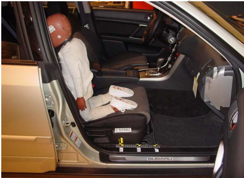
3-Year-Old Unbelted, Rearward Seat Track, Position 7
