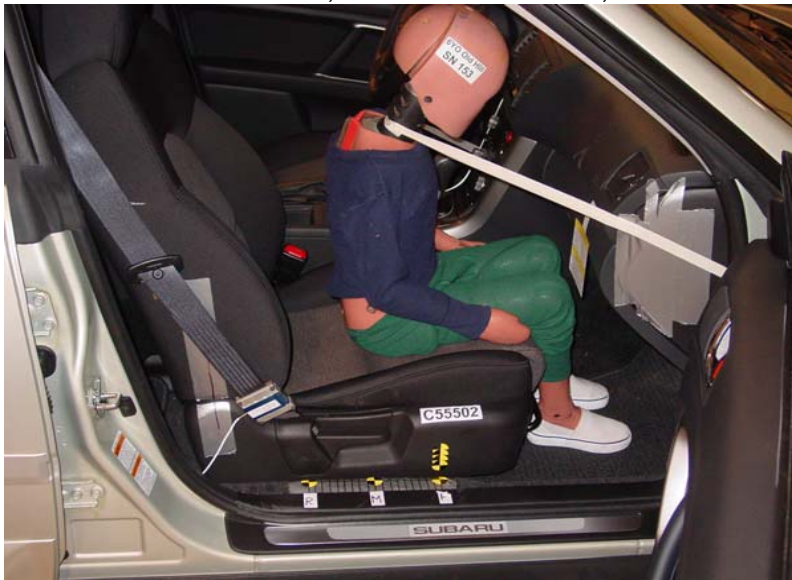
6-Year-Old Unbelted, Forward Seat Track, Position 3
