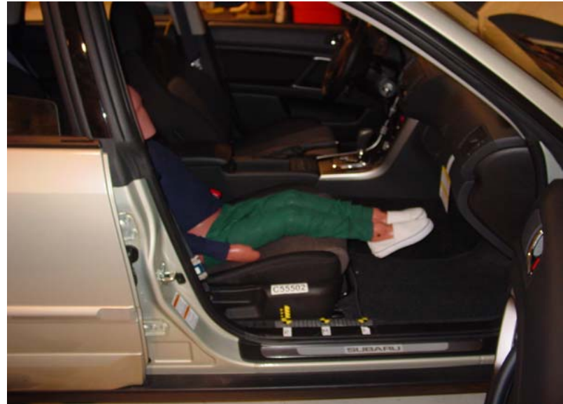
6-Year-Old Unbelted, Rearward Seat Track, Position 2
