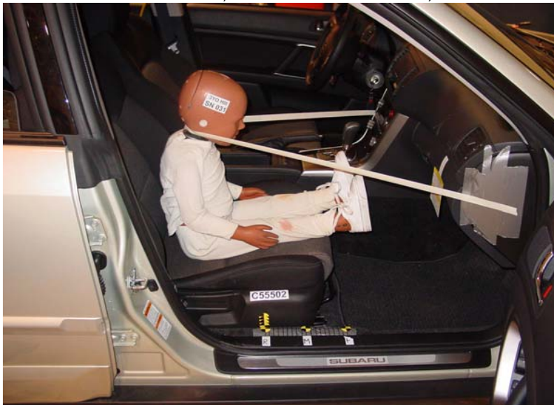
3-Year-Old Unbelted, Rearward Seat Track, Position 3
