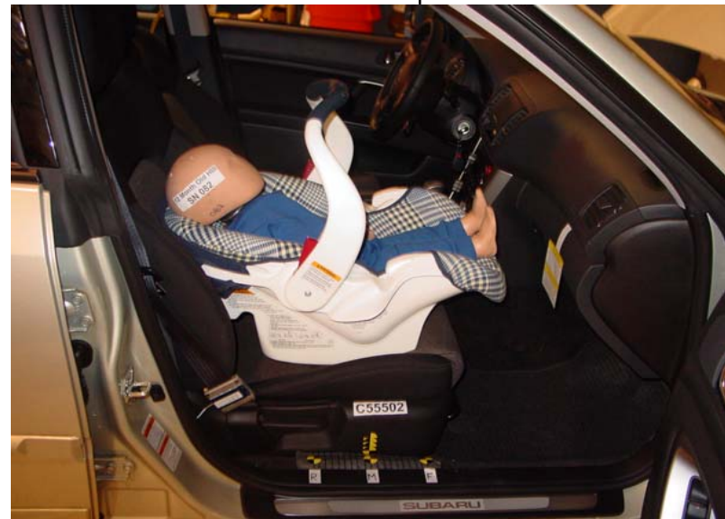
Graco Infant W/O Base Fwd Facing Unbelted, Middle Seat Track, Handle Up
