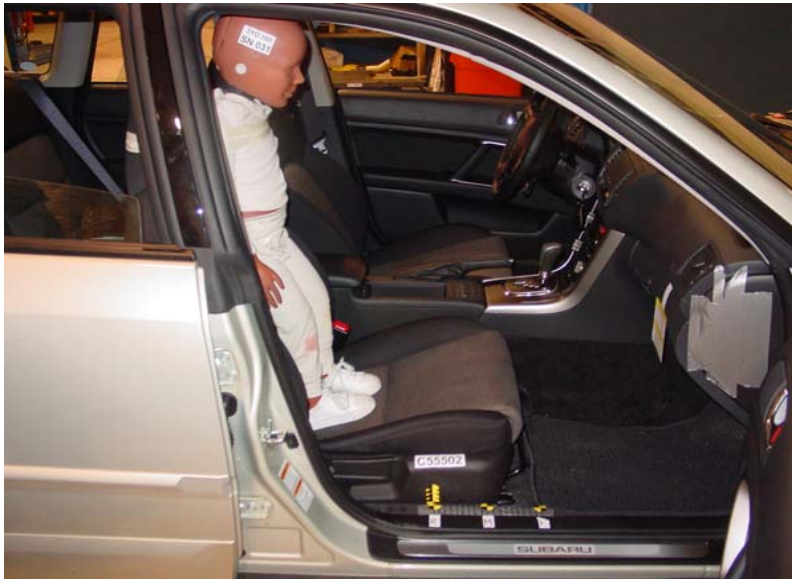
3-Year-Old Unbelted, Rearward Seat Track, Position 5
