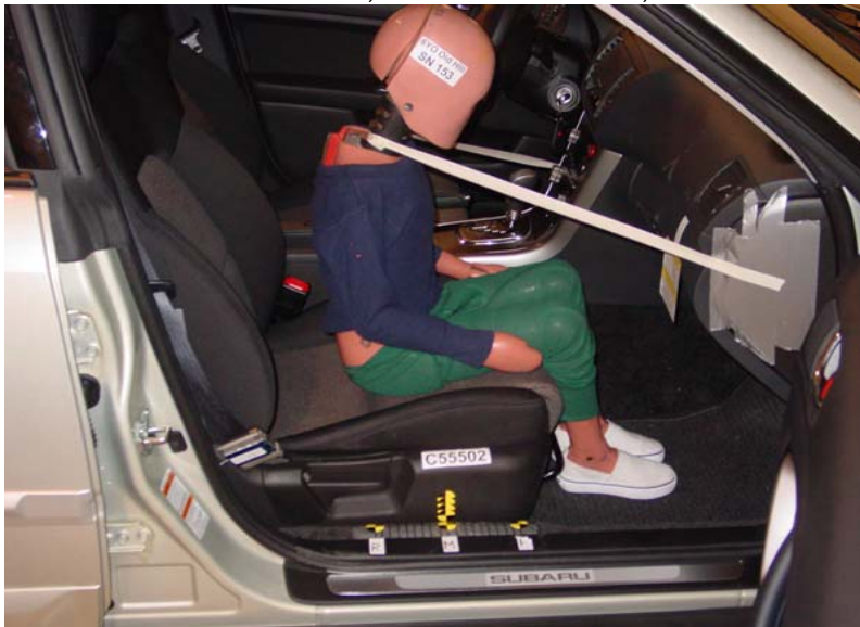
6-Year-Old Unbelted, Middle Seat Track, Position 3
