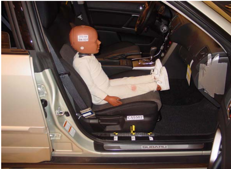
3-Year-Old Unbelted, Middle Seat Track, Position 1
