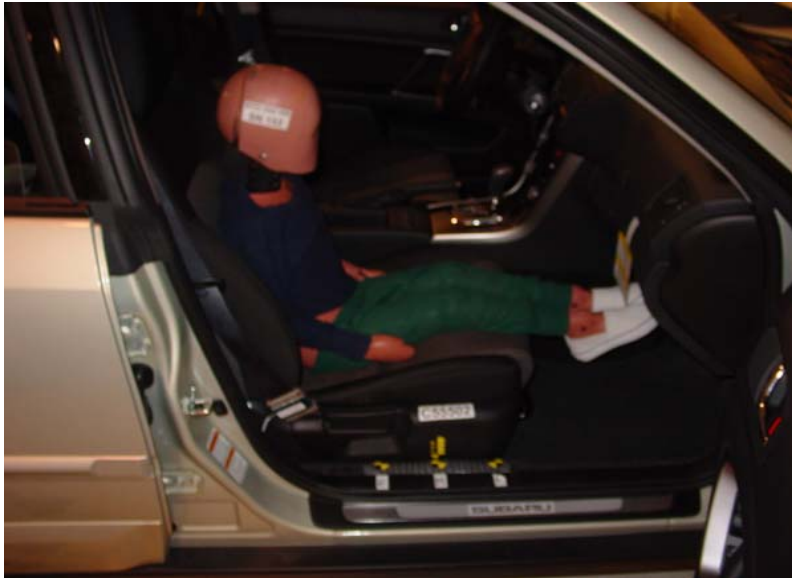
6-Year-Old Unbelted, Middle Seat Track, Position 1
