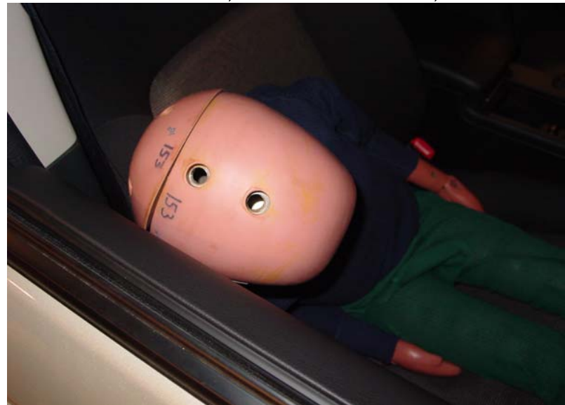
6-Year-Old Unbelted, Rearward Seat Track, Position 4
