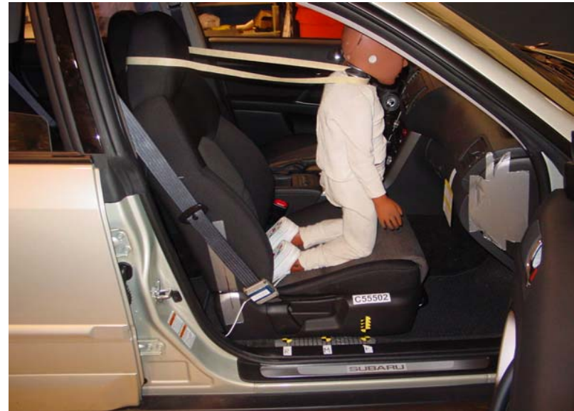
3-Year-Old Unbelted, Forward Seat Track, Position 6
