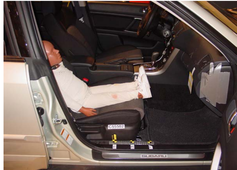
3-Year-Old Unbelted, Rearward Seat Track, Position 2
