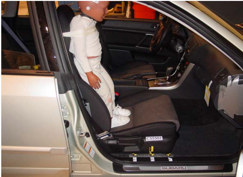
3-Year-Old Unbelted, Middle Seat Track, Position 5
