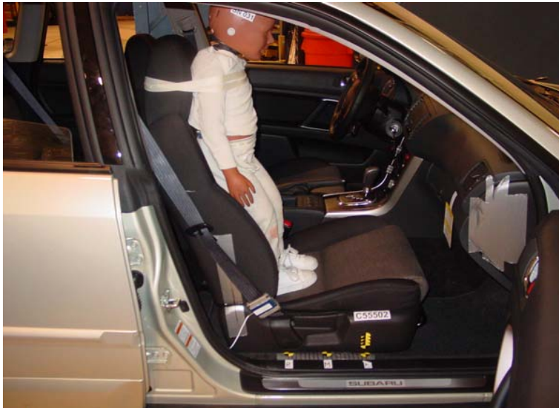
3-Year-Old Unbelted, Forward Seat Track, Position 5
