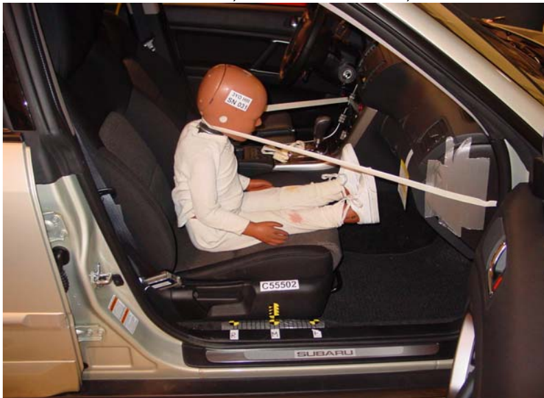
3-Year-Old Unbelted, Middle Seat Track, Position 3
