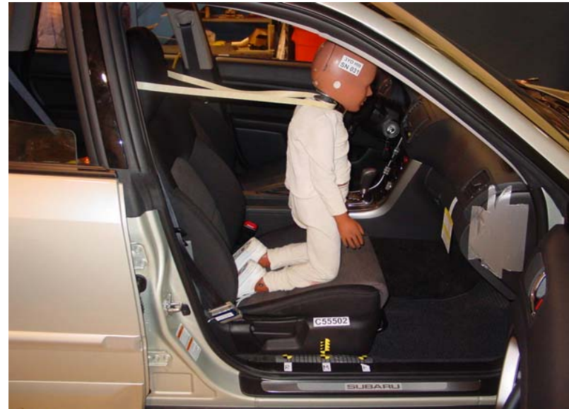
3-Year-Old Unbelted, Middle Seat Track, Position 6
