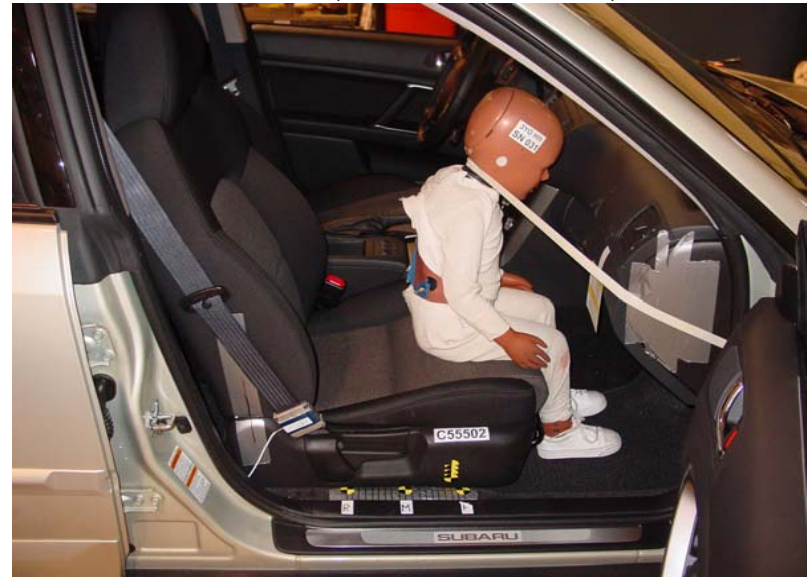
3-Year-Old Unbelted, Forward Seat Track, Position 4
