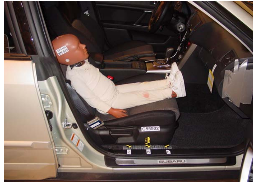
3-Year-Old Unbelted, Middle Seat Track, Position 2
