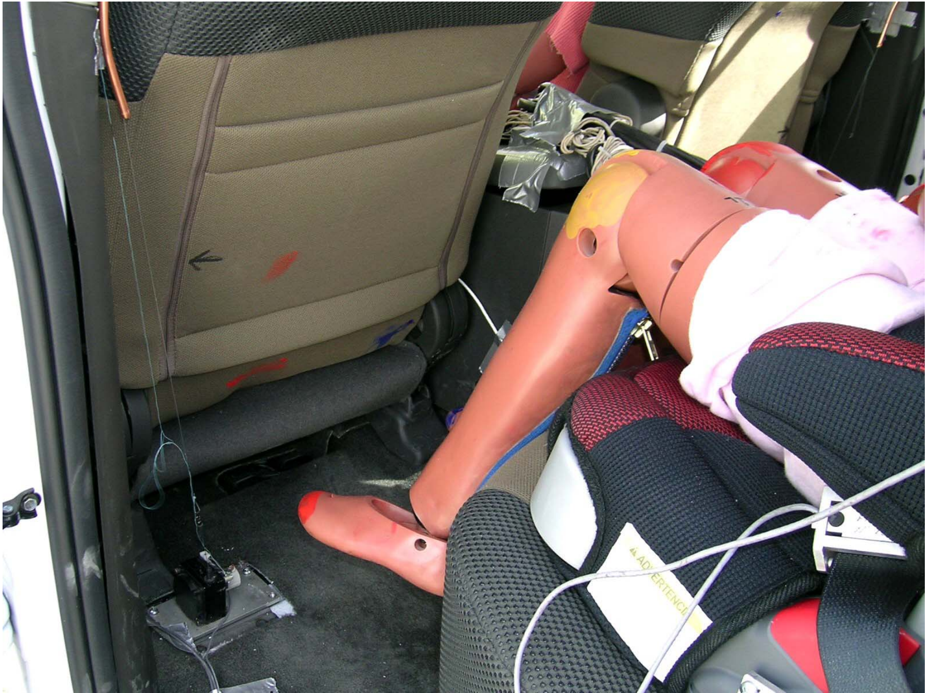
Figure F2-27: Post-Test Position 4 Dummy Feet Contacts
