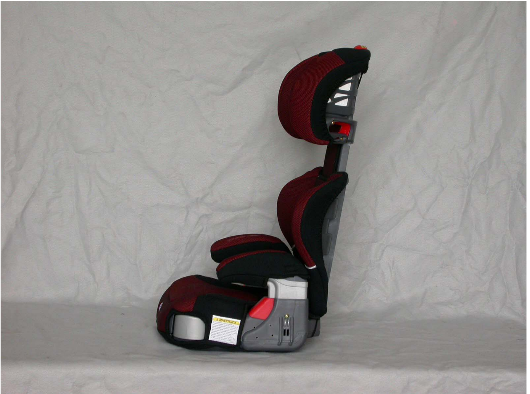
Figure F2-16: Post-Test Left Side View of Position 4 CRS
