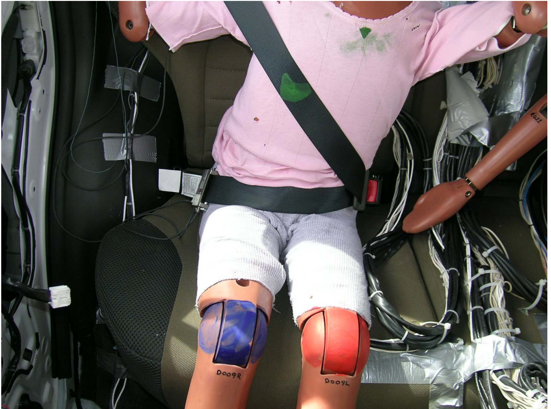
Figure F2-4: Post-Test Position 3 Front View (Seat Belt Position)
