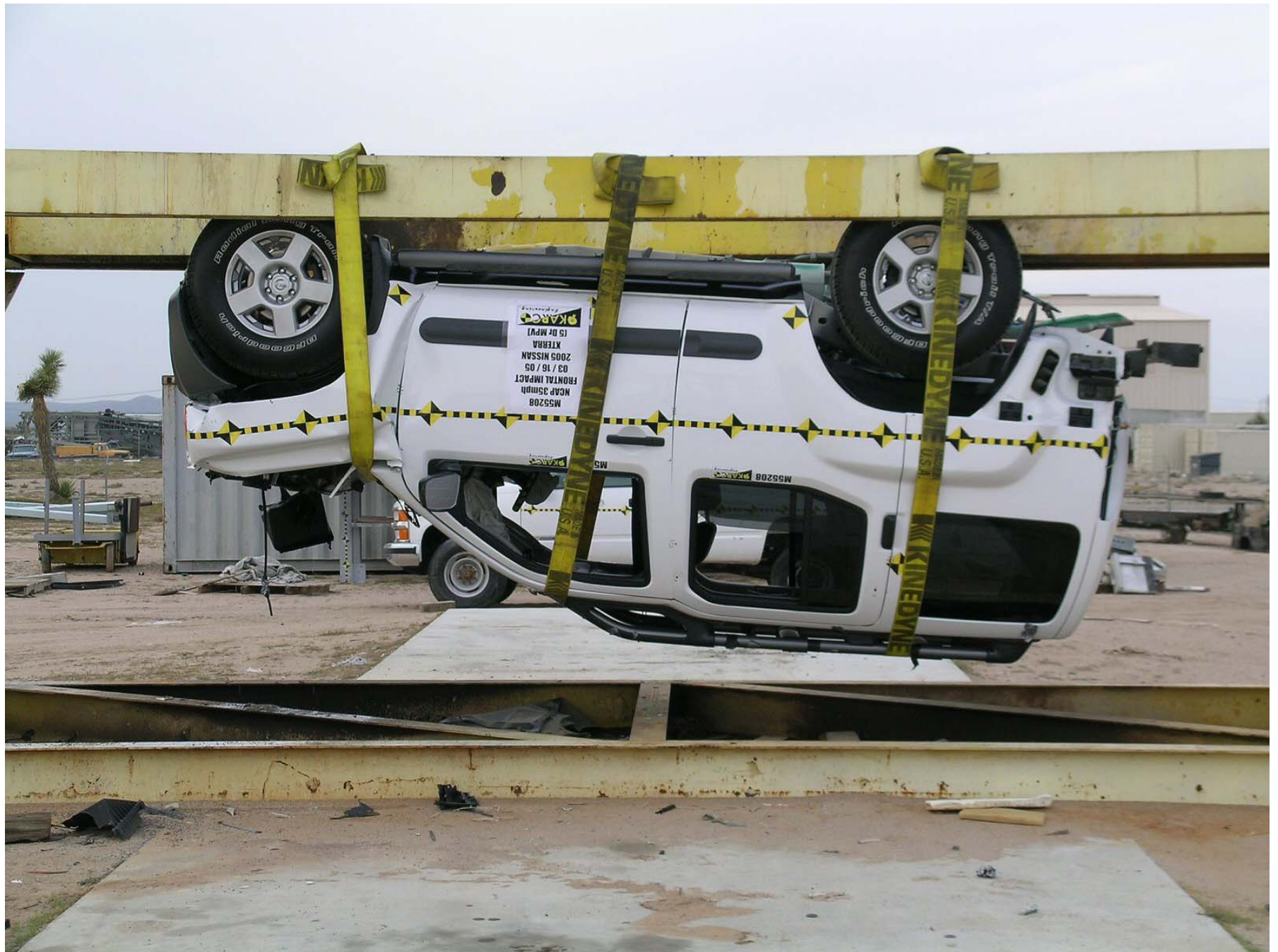
Figure A-60: Vehicle on Rollover Device (180°)
