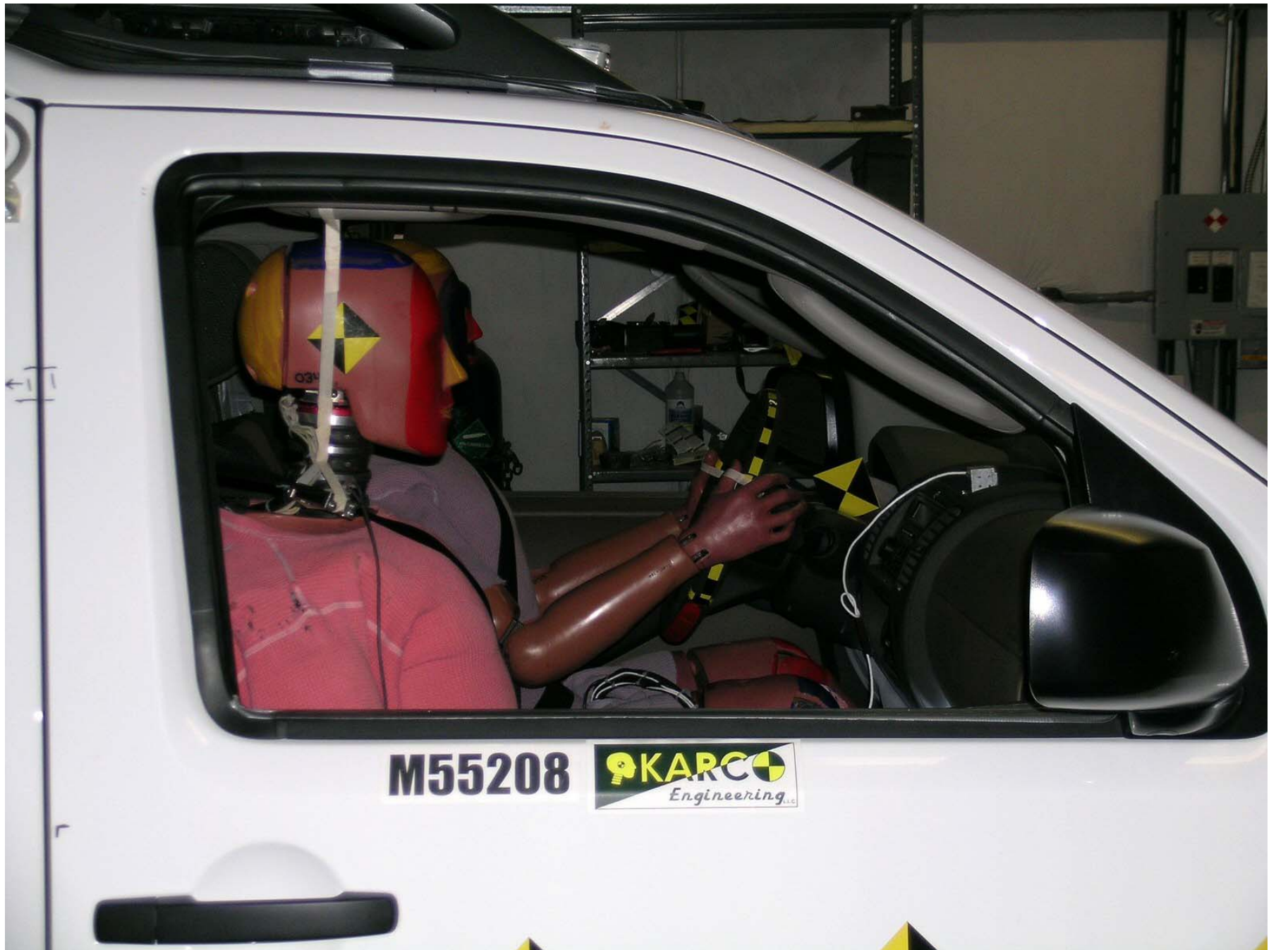
Figure A-46: Pre-Test Passenger Dummy (Through Window)
