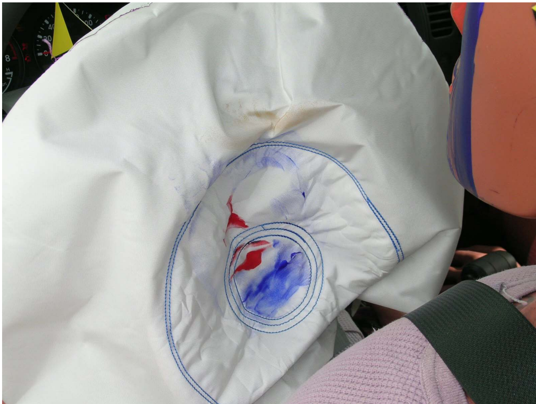
Figure A-43: Post-Test Driver Dummy Airbag Contact
