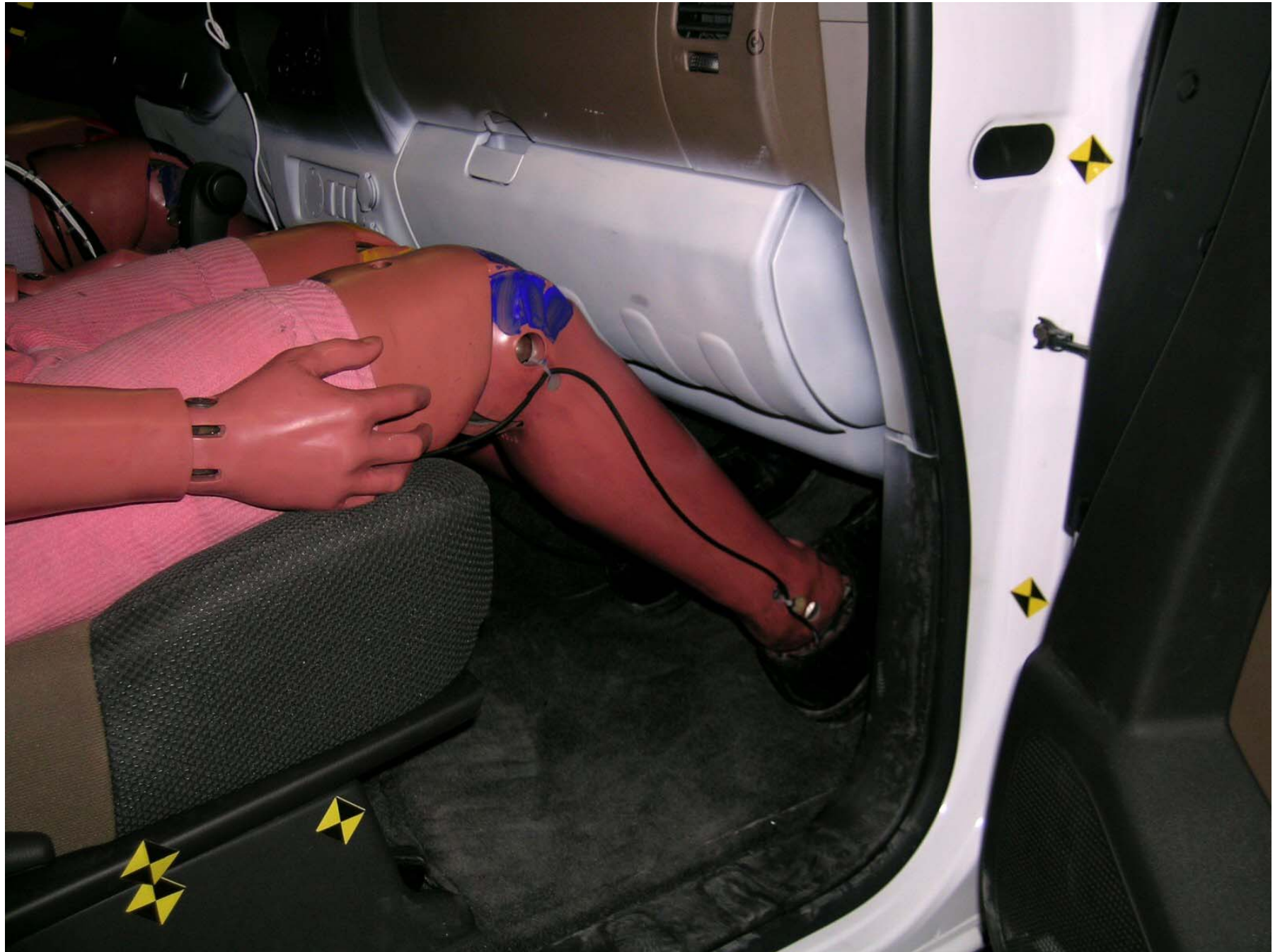
Figure A-50: Pre-Test Passenger Dummy Feet
