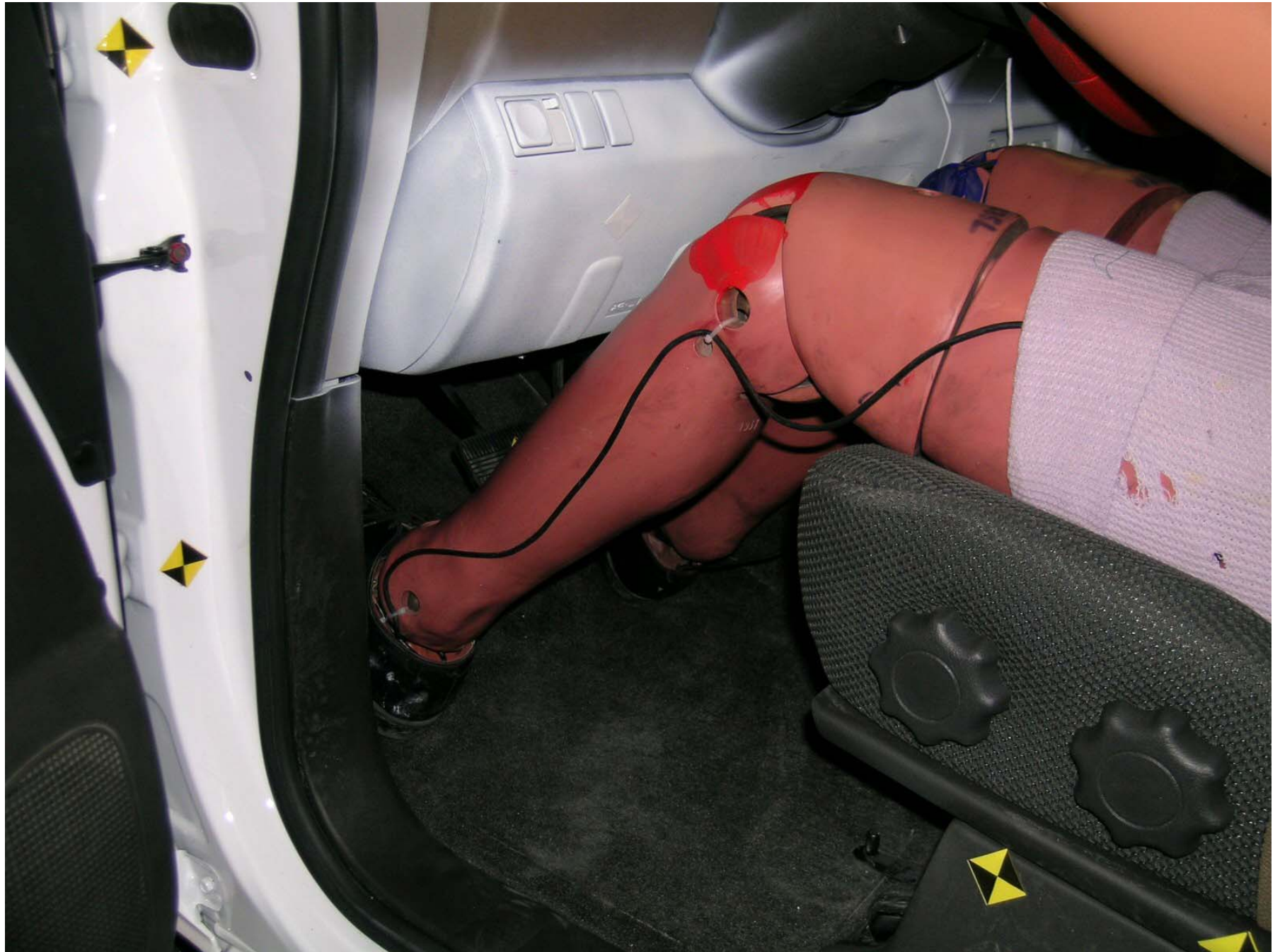
Figure A-36: Pre-Test Driver Dummy Feet
