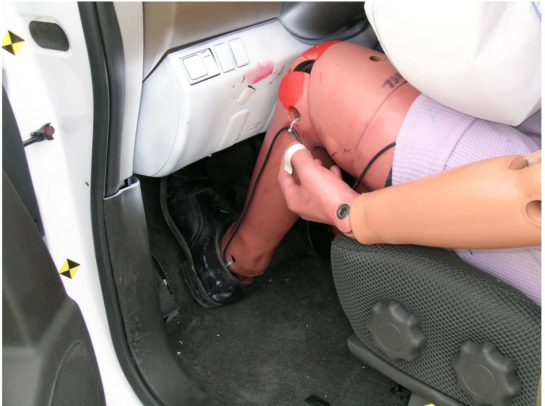
Figure A-37: Post-Test Driver Dummy Feet
