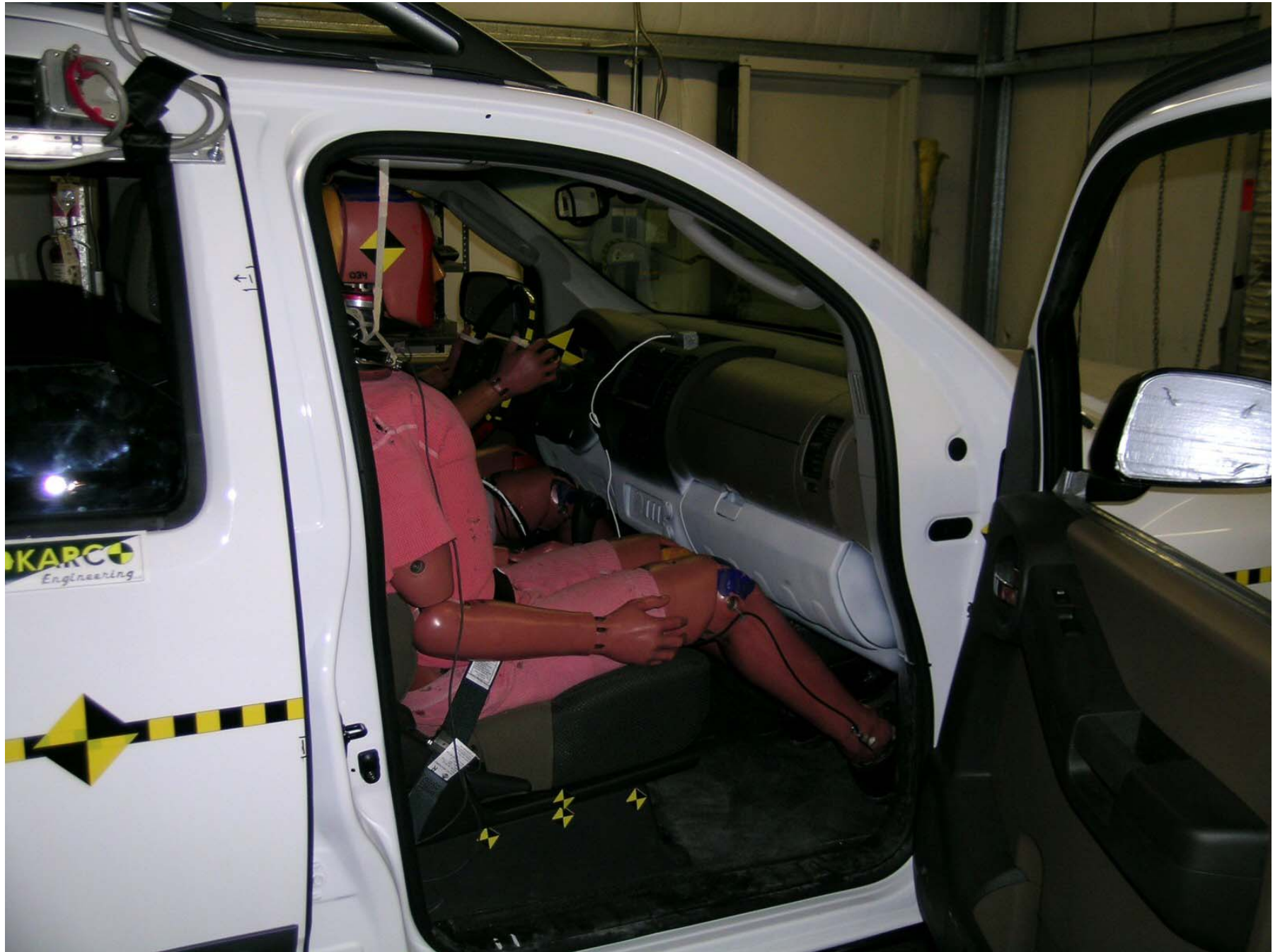
Figure A-48: Pre-Test Passenger Dummy (Door Open)
