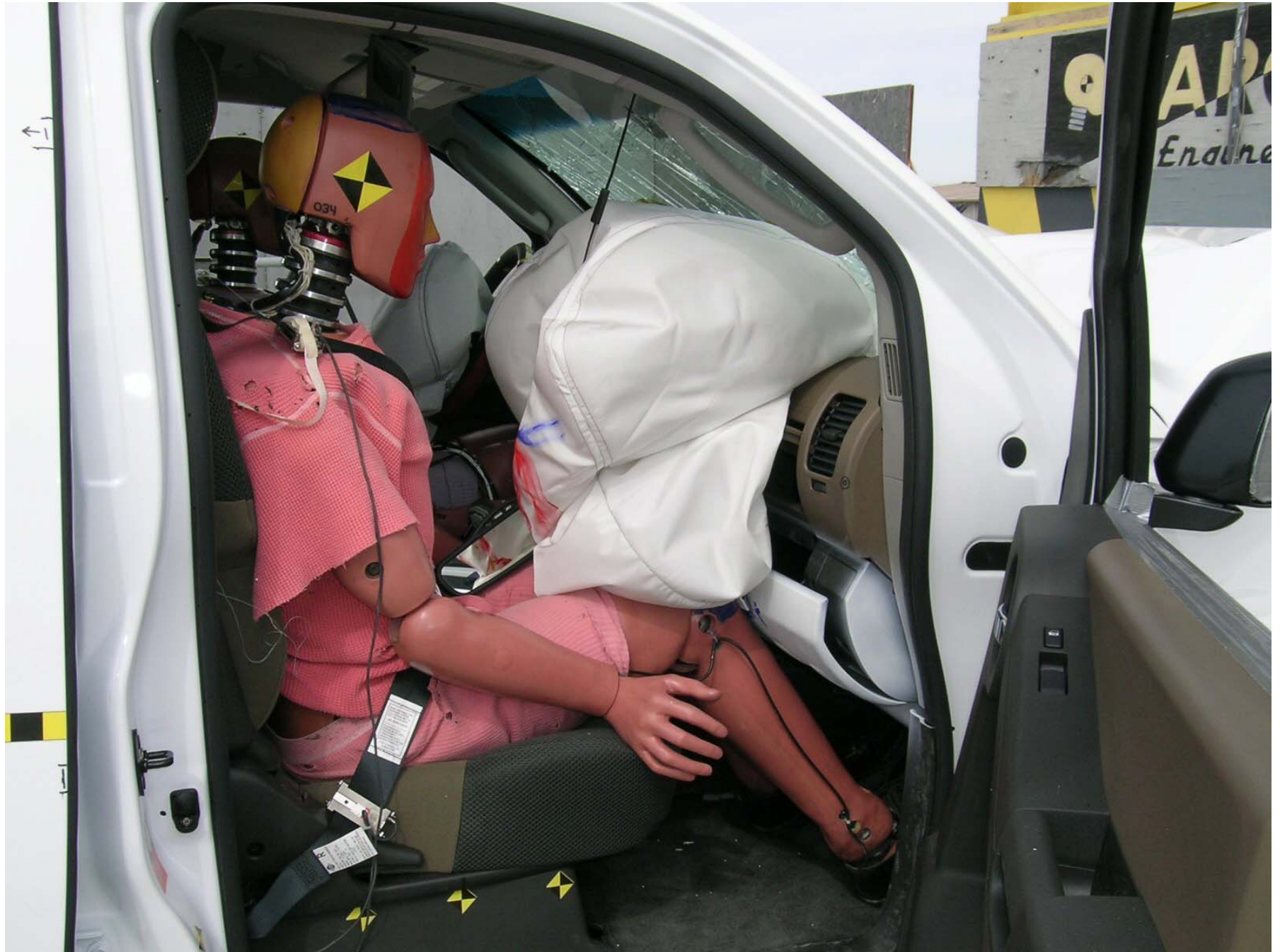
Figure A-49: Post-Test Passenger Dummy (Door Open)
