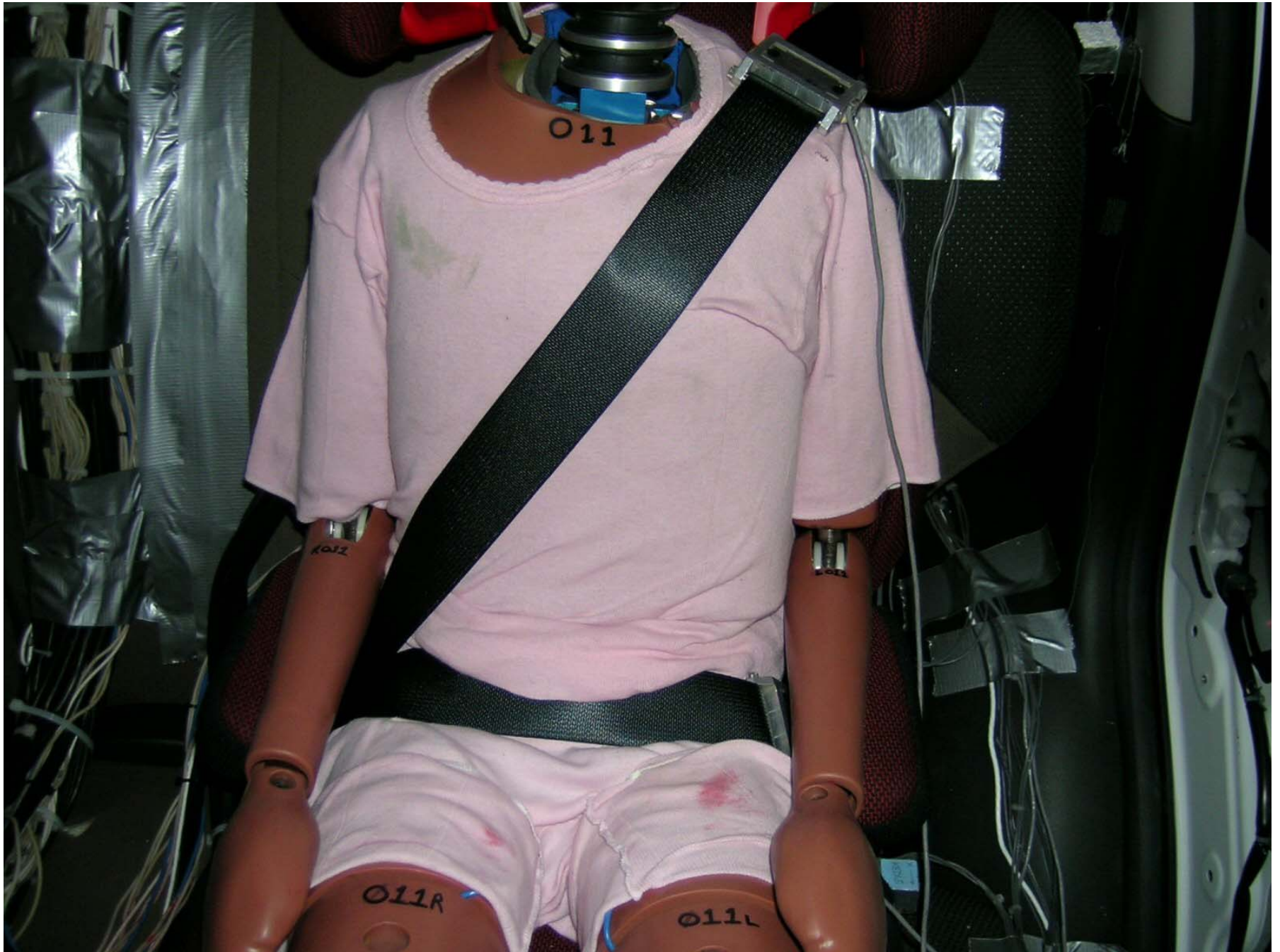
Figure F2-21: Pre-Test Position 4 Front View (Seat Belt Position)
