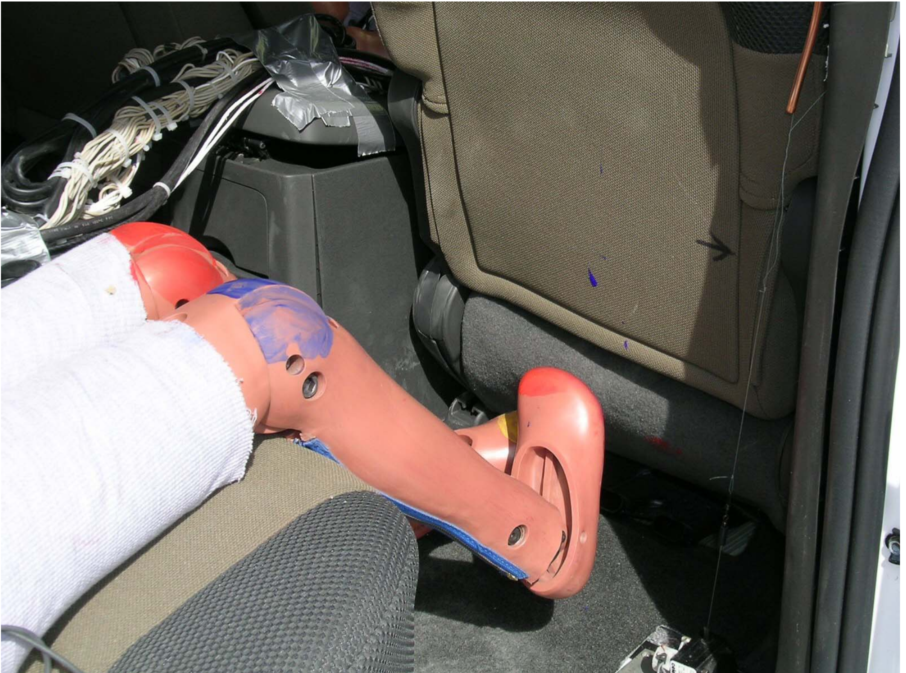
Figure F2-9: Post-Test Position 3 Dummy Feet
