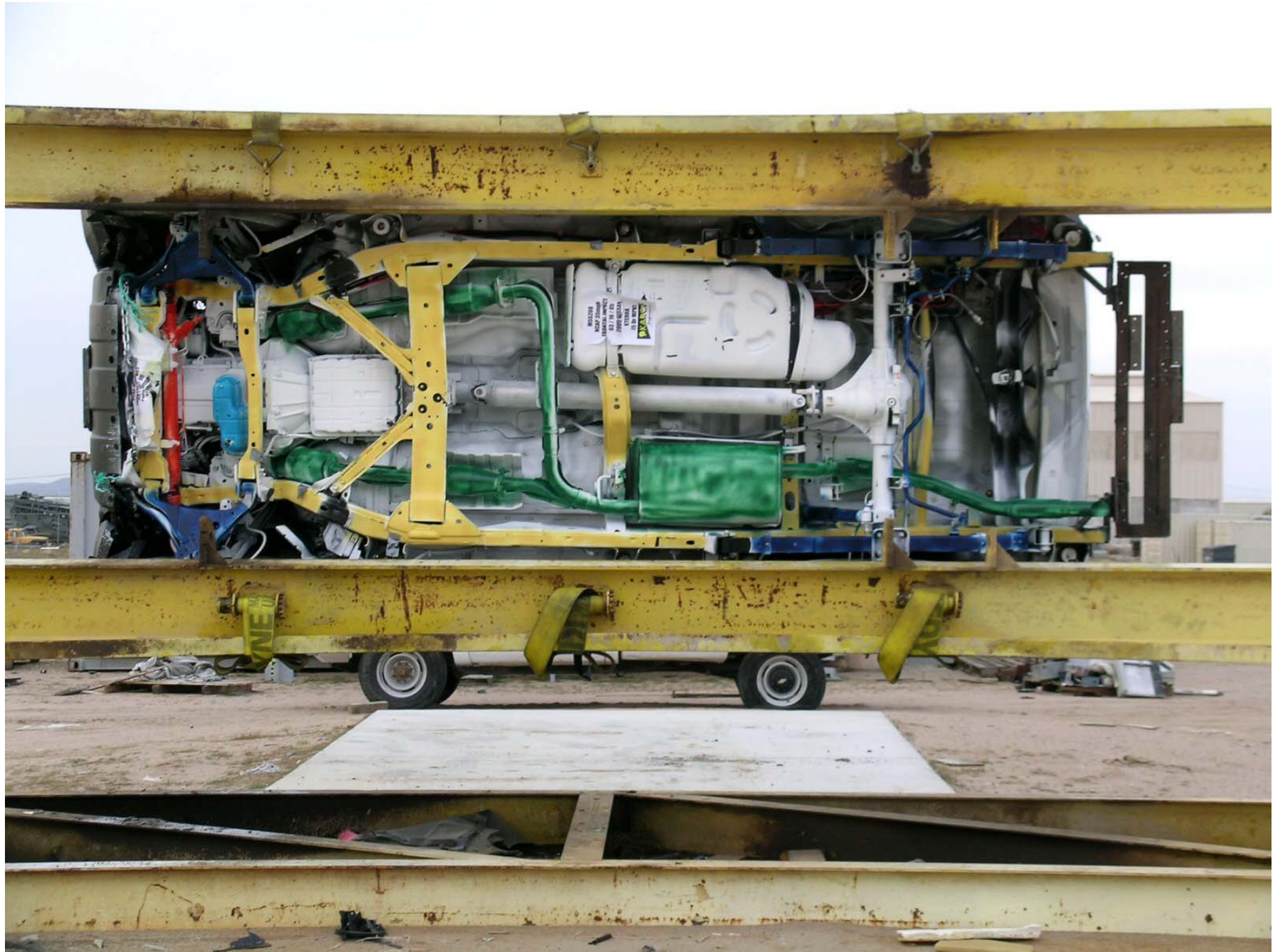
Figure A-61: Vehicle on Rollover Device (270°)
