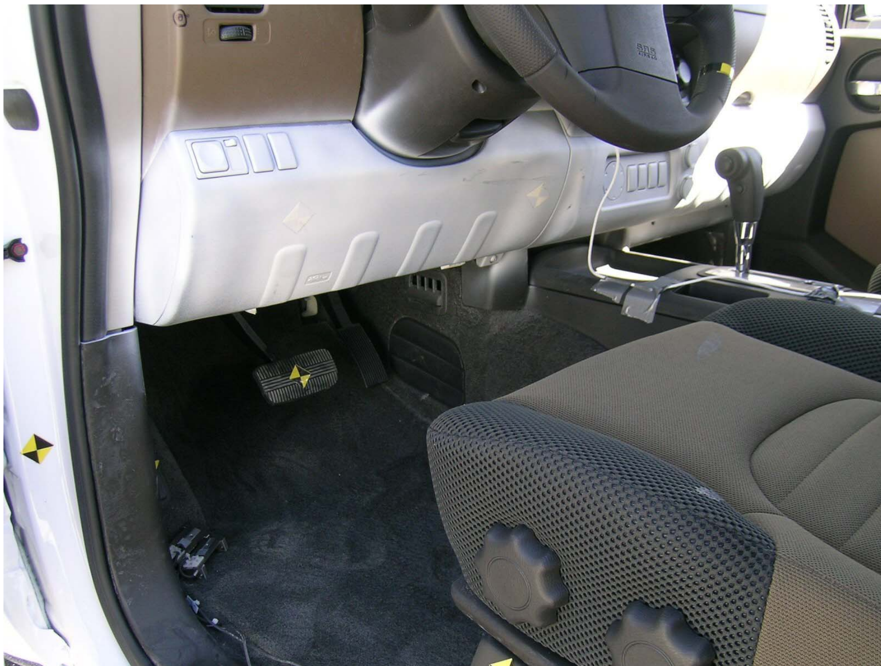
Figure A-38: Pre-Test Driver Side Knee Bolster
