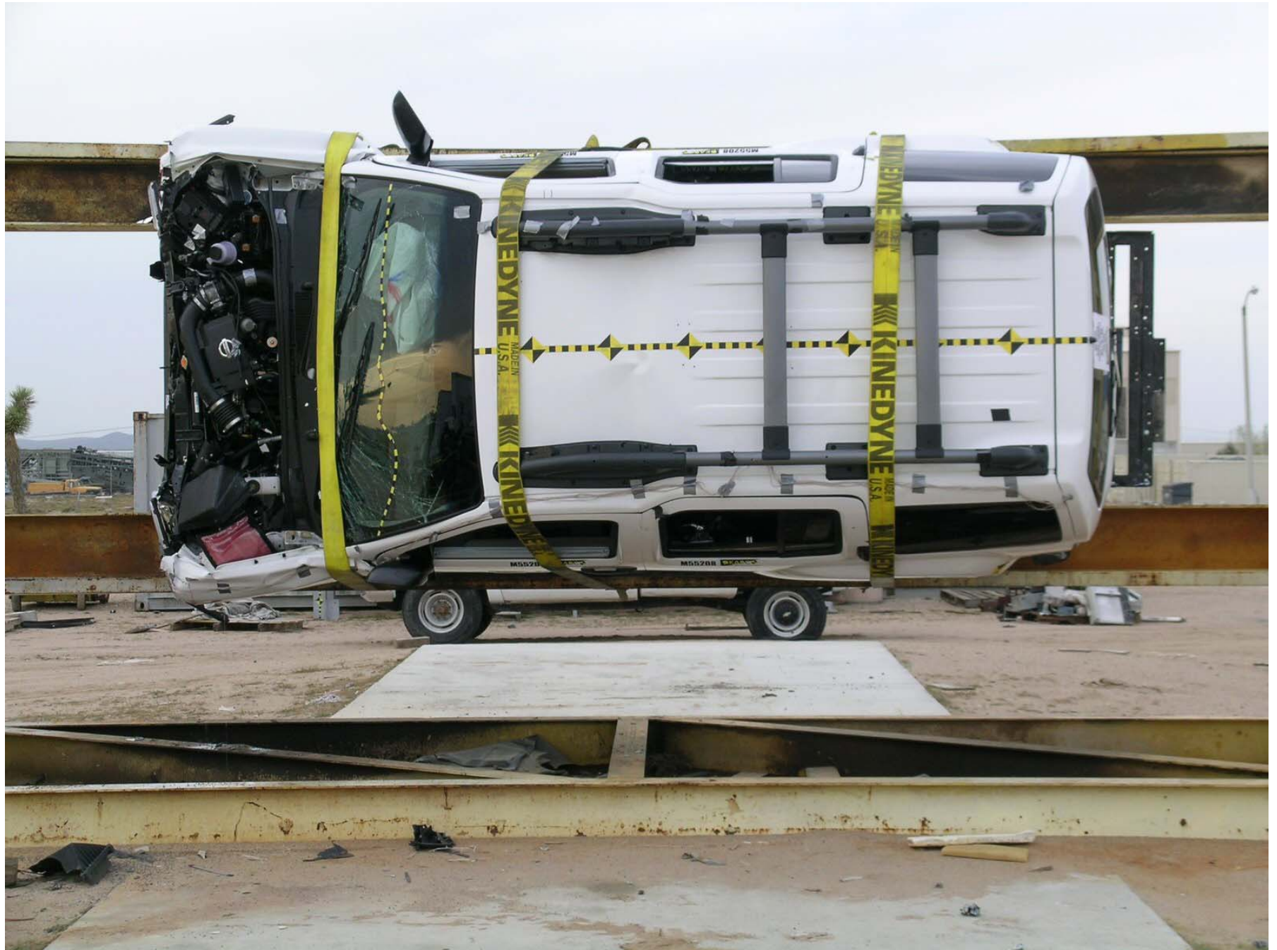
Figure A-59: Vehicle on Rollover Device (90°)
