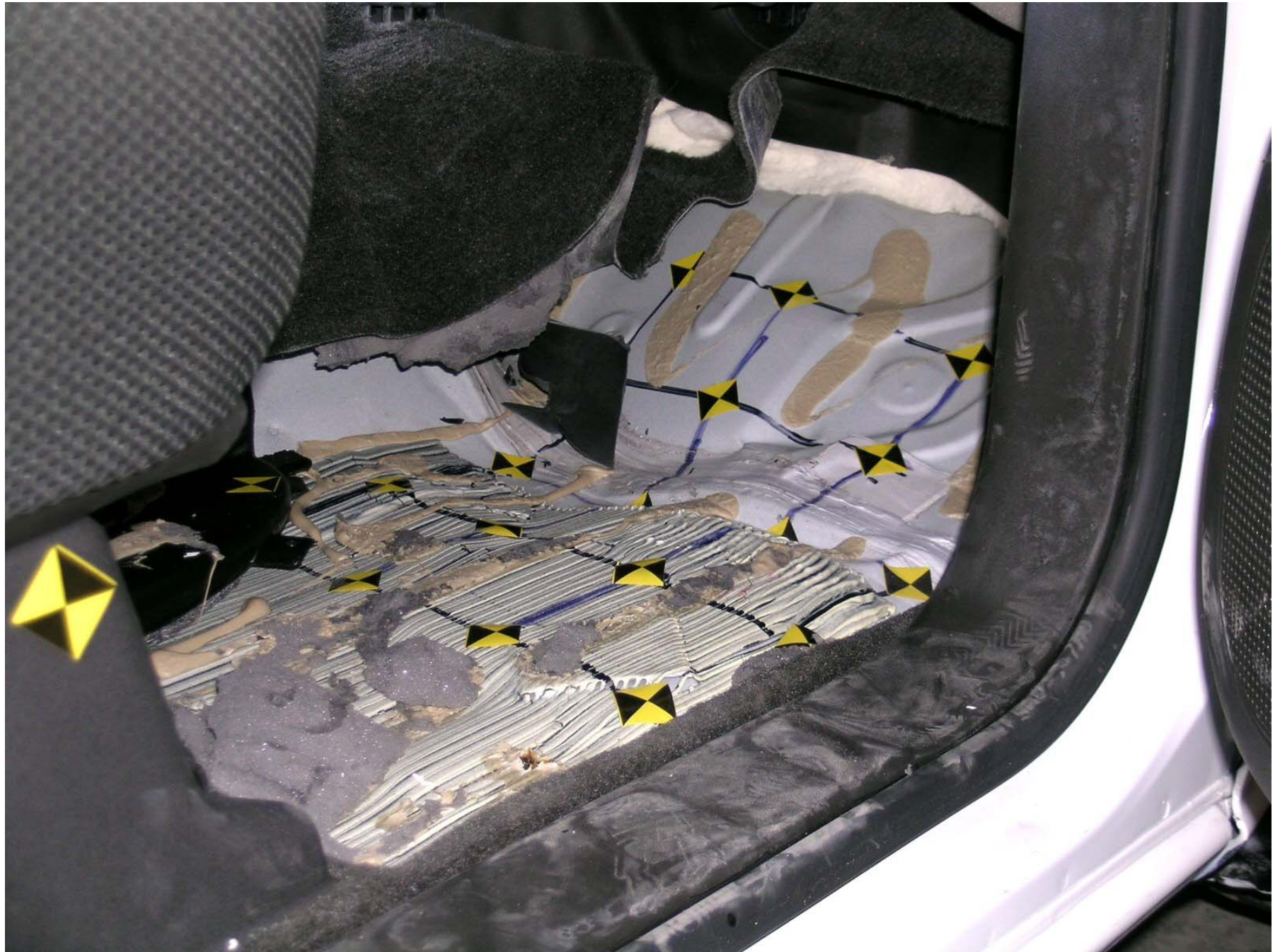
Figure A-55: Post-Test Passenger Side Floor Pan
