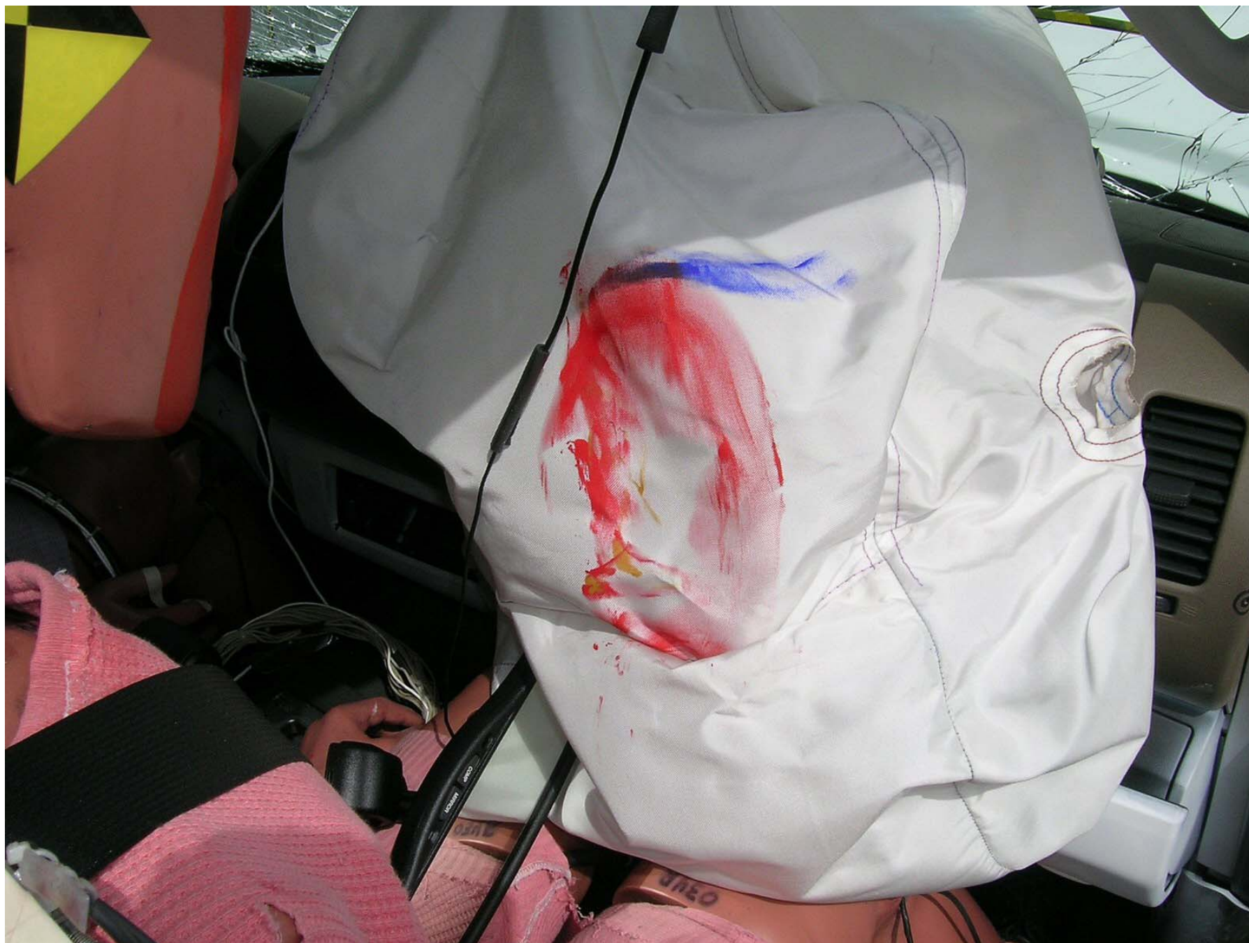
Figure A-57: Post-Test Passenger Dummy Airbag Contact
