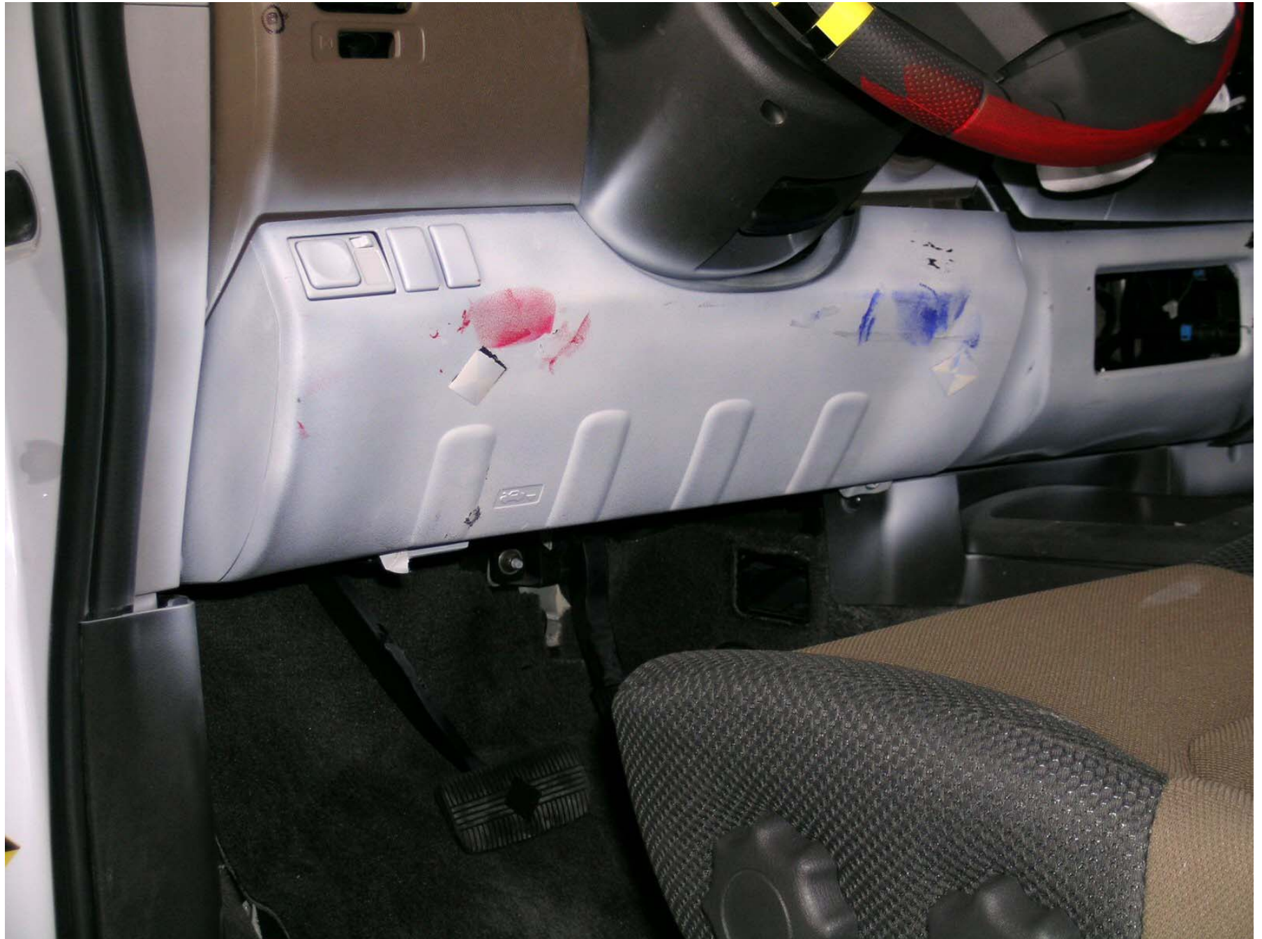
Figure A-39: Post-Test Driver Side Knee Bolster
