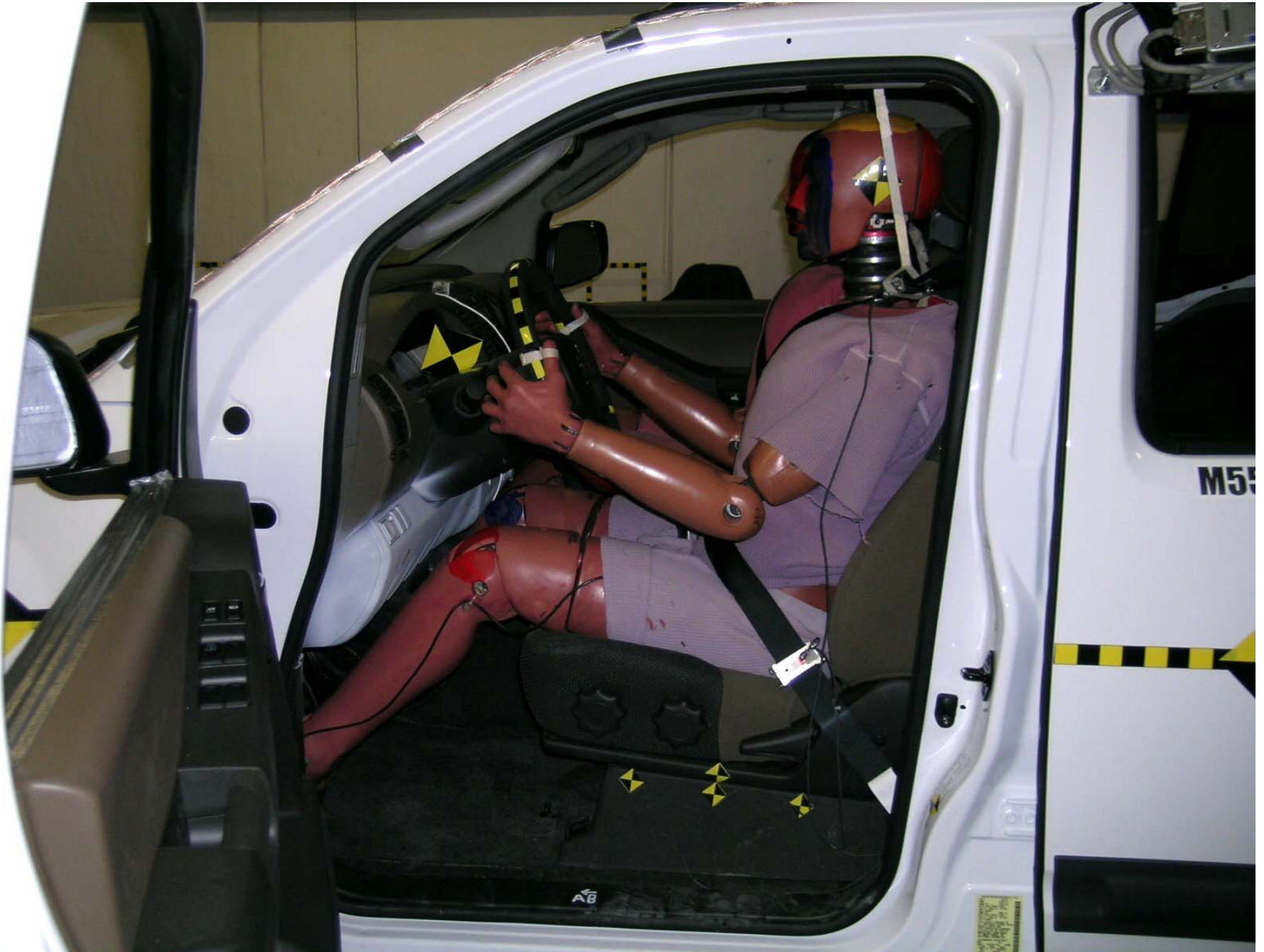
Figure A-34: Pre-Test Driver Dummy (Door Open)
