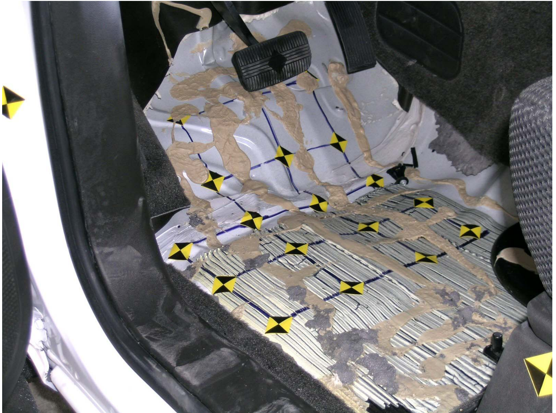
Figure A-41: Post-Test Driver Side Floor Pan
