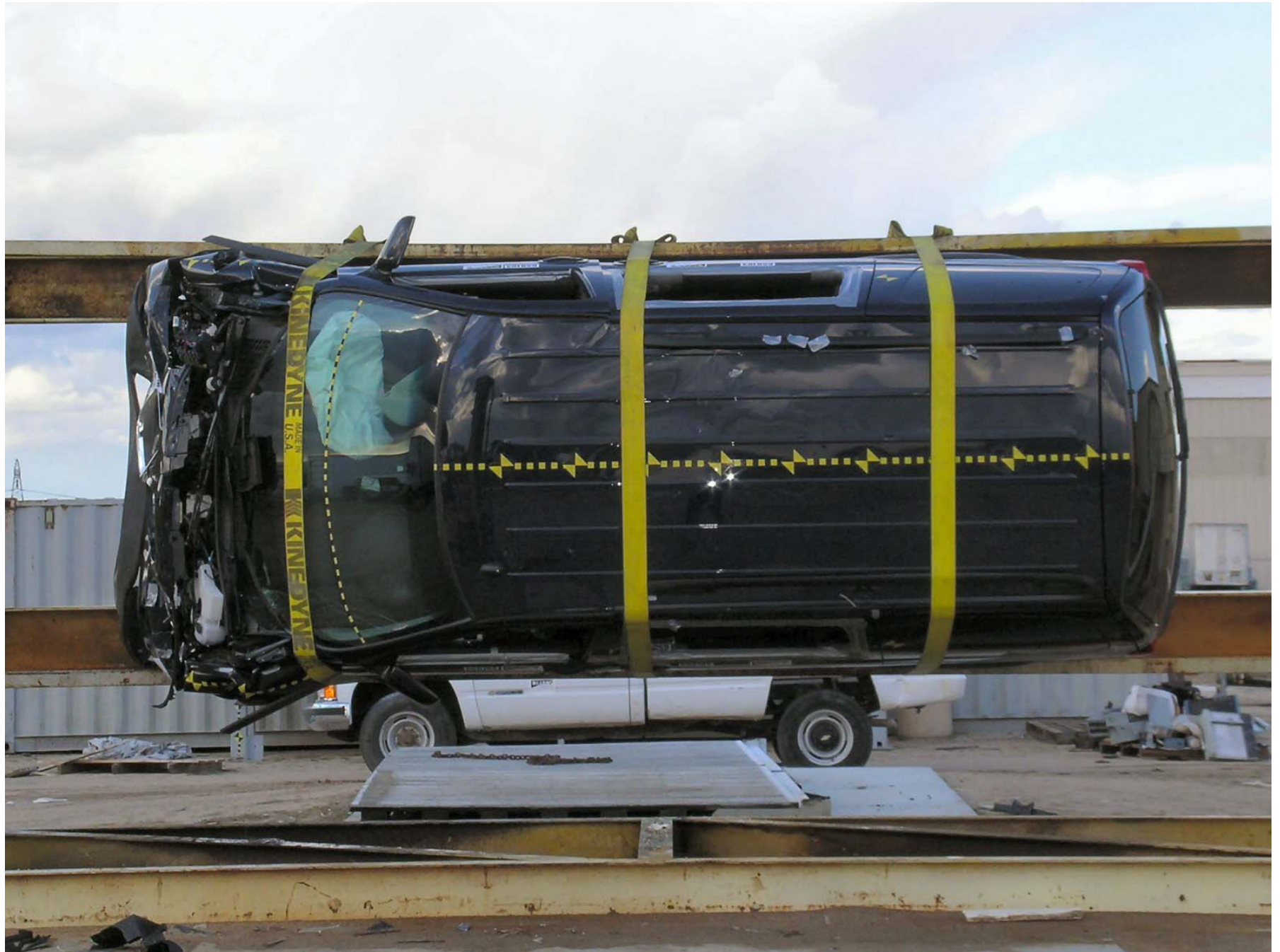
Figure A-59: Vehicle on Rollover Device (90°)
