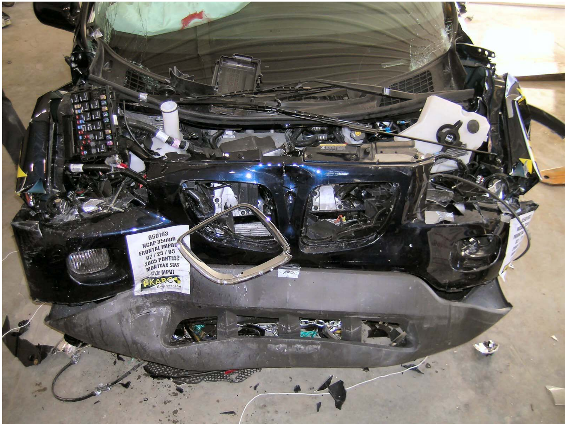
Figure A-21: Post-Test Engine Compartment (Vehicle Moved)
