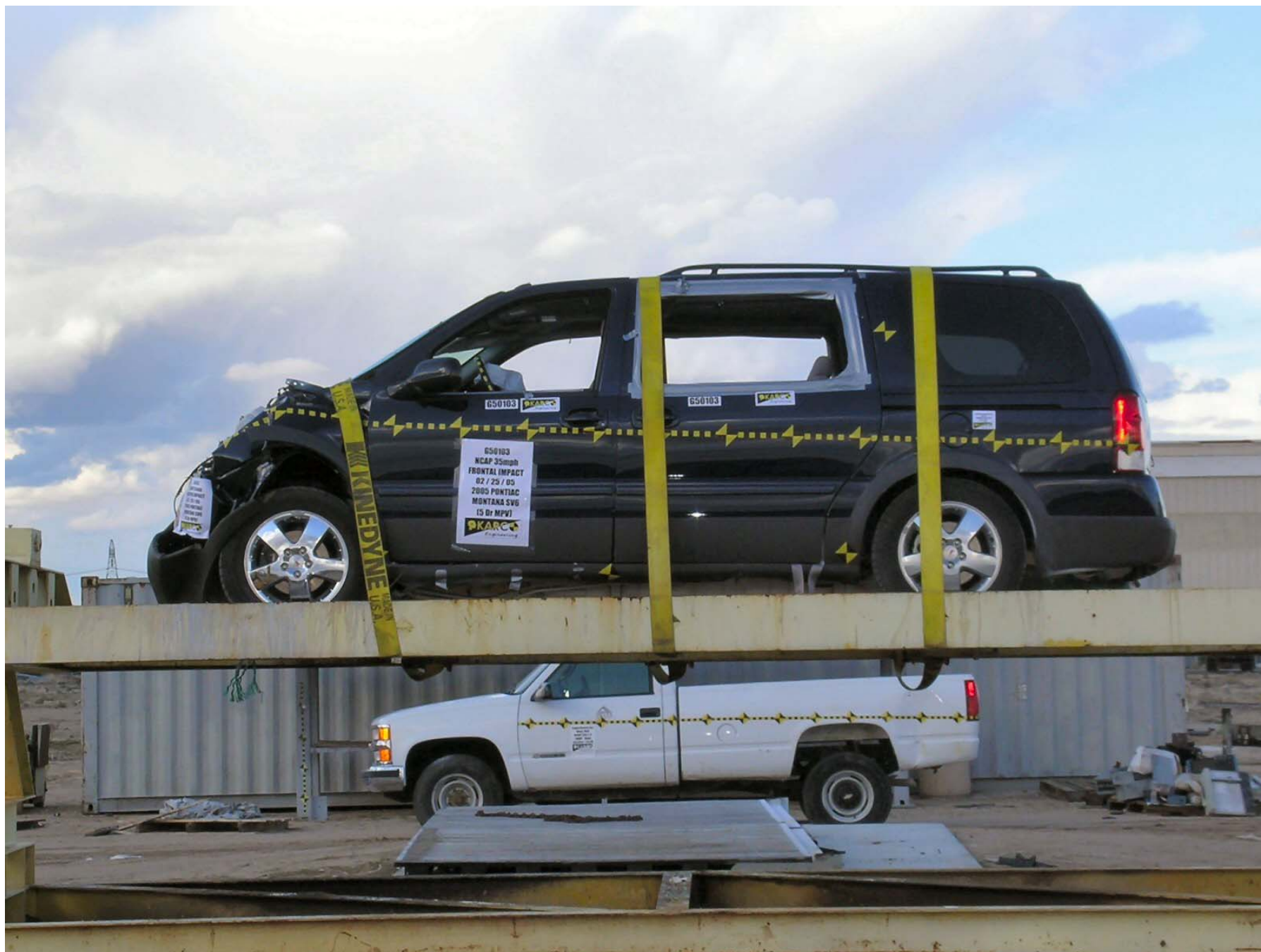
Figure A-58: Vehicle on Rollover Device (0°)
