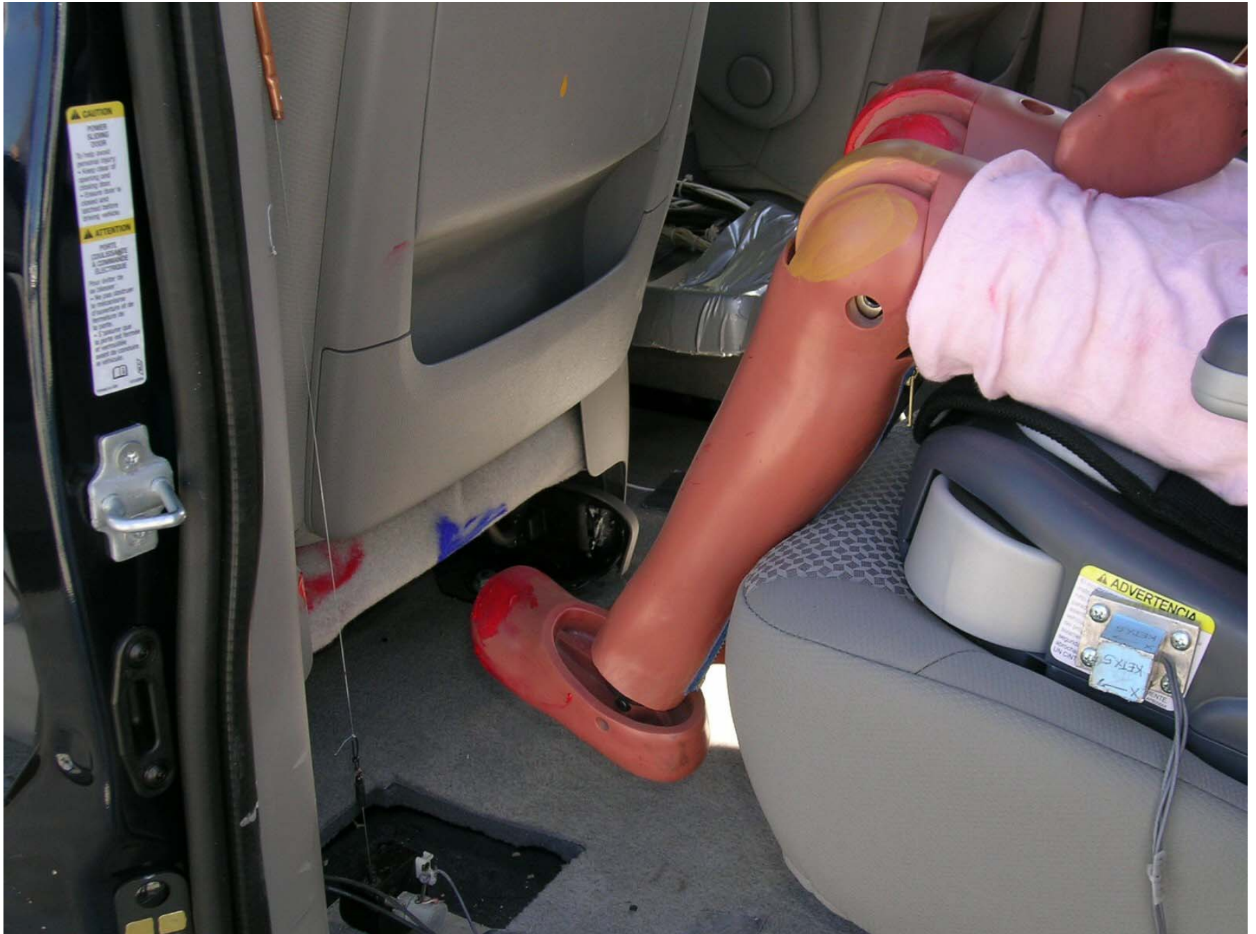
Figure F2-36: Post-Test Position 4 Dummy Feet Contacts
