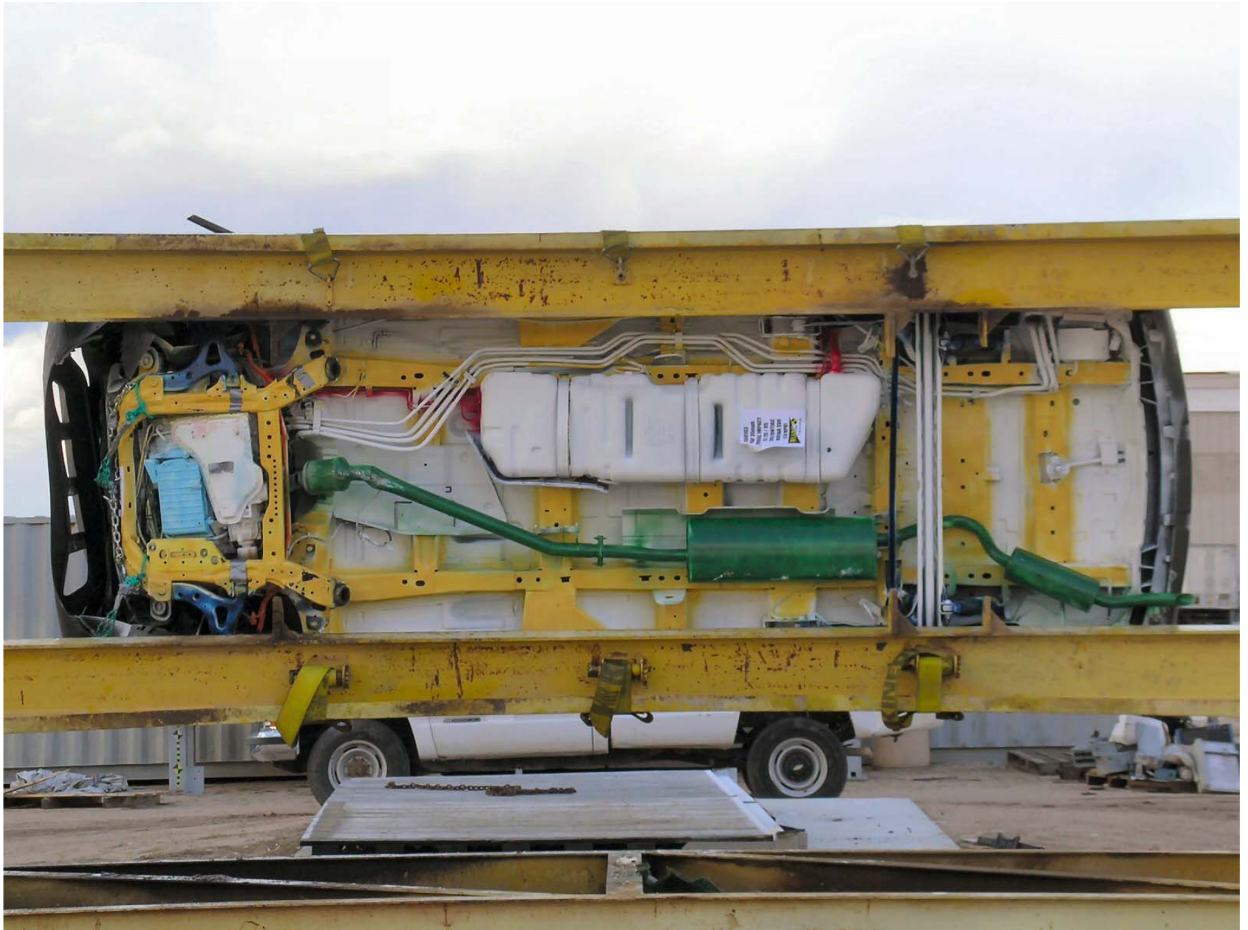
Figure A-61: Vehicle on Rollover Device (270°)
