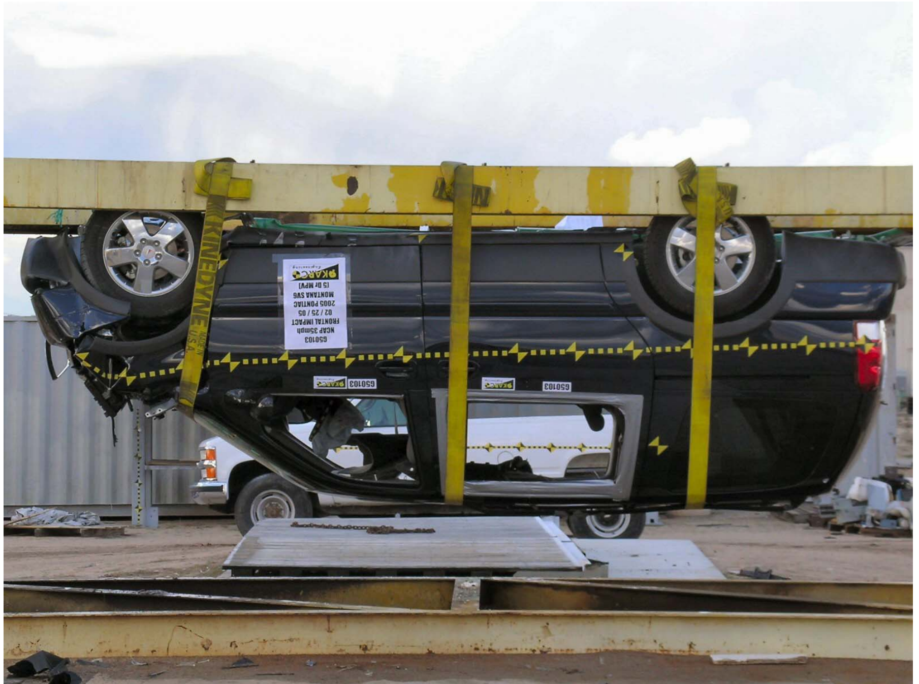
Figure A-60: Vehicle on Rollover Device (180°)
