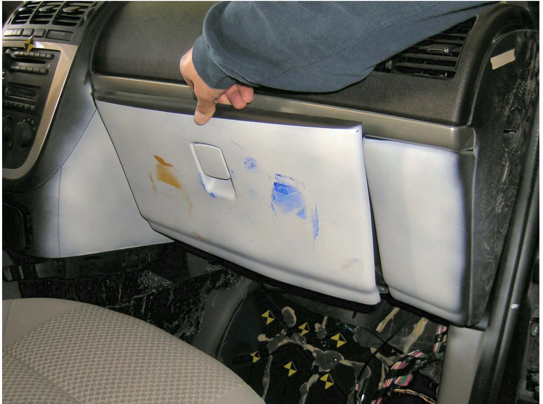
Figure A-53: Post-Test Passenger Side Glove Box
