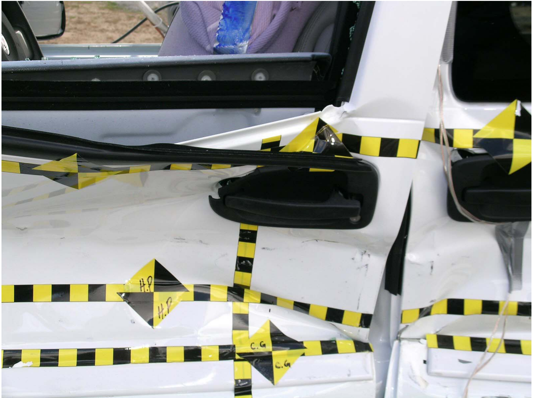
Figure A-32: Post-Test Left Front Door
