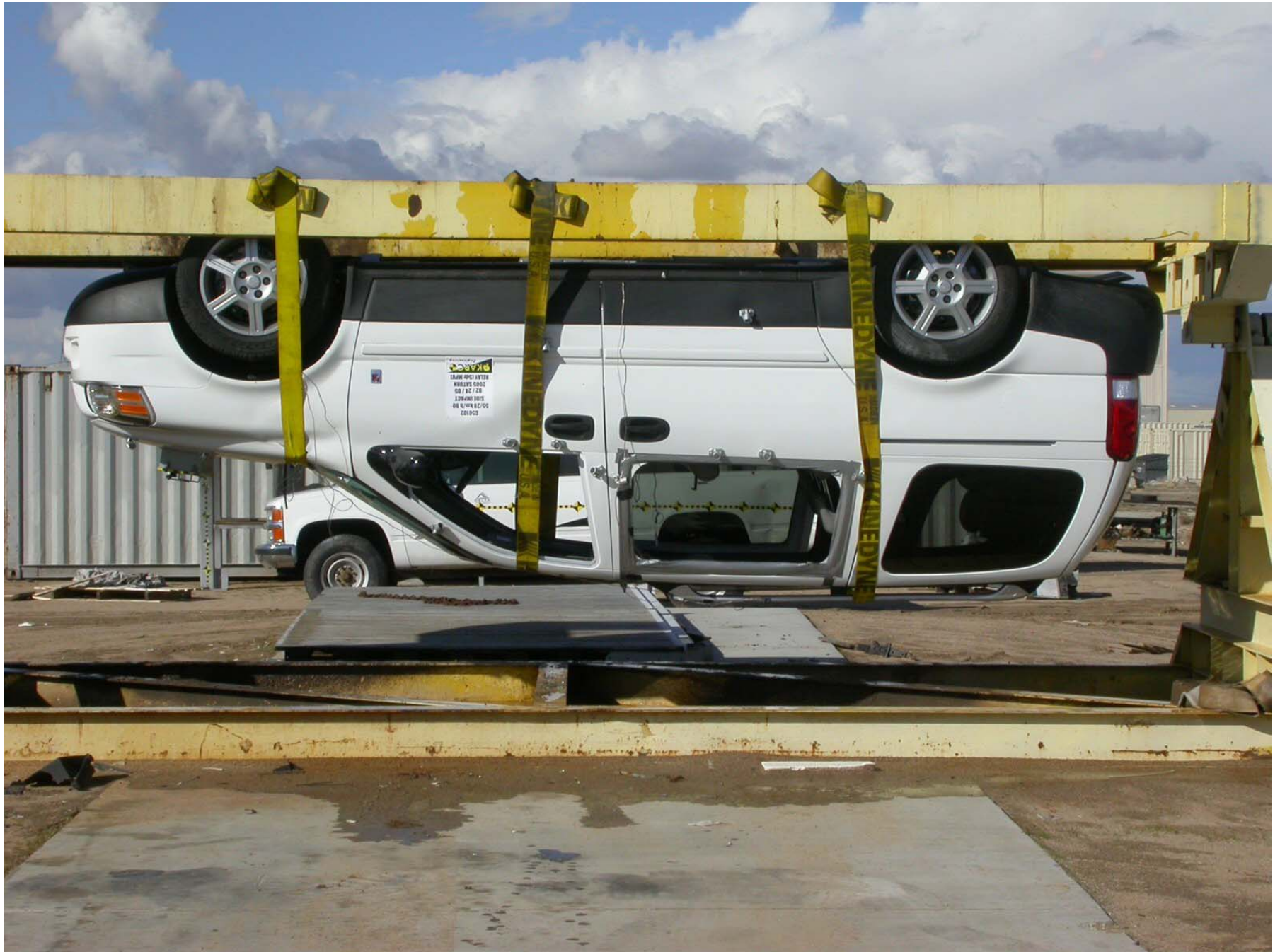
Figure A-63: Vehicle on Rollover Device (180°)
