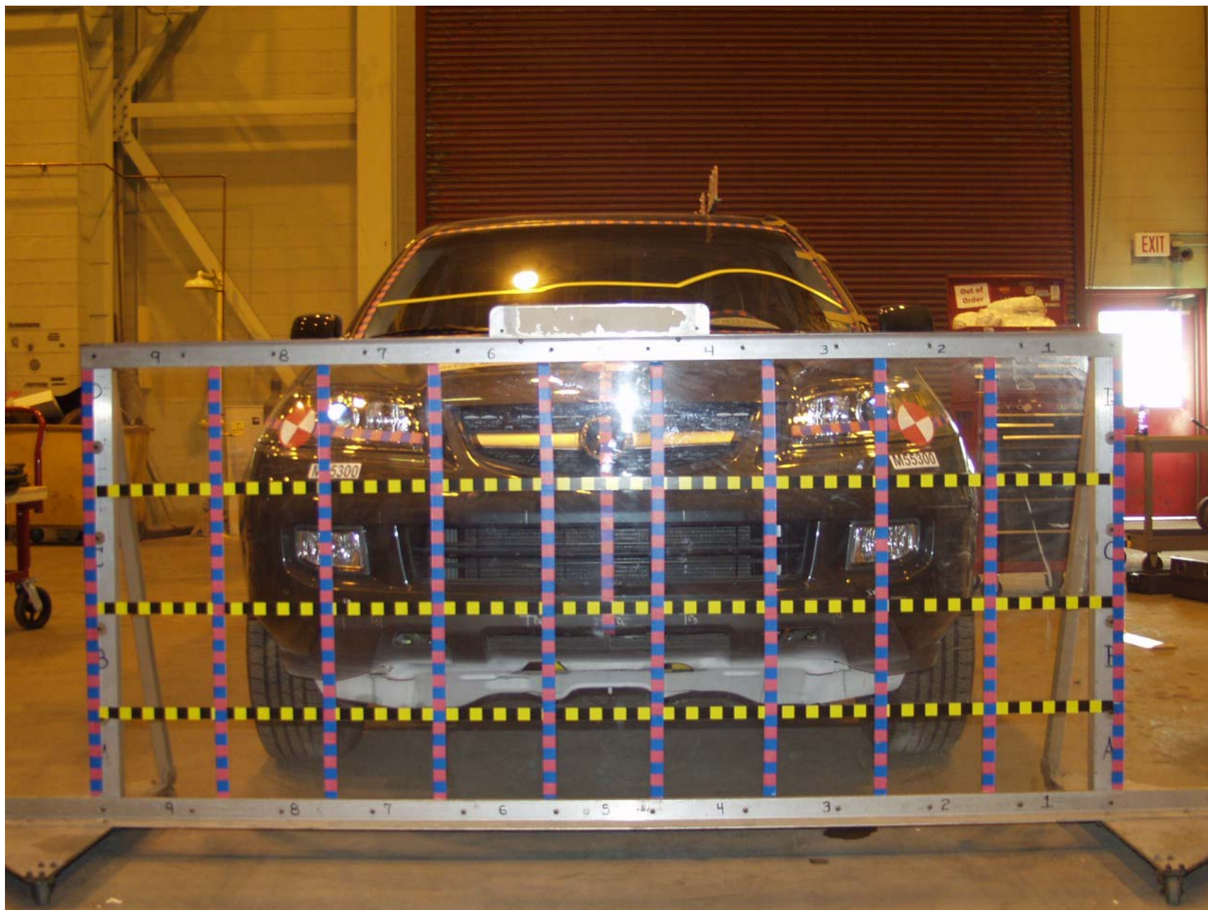
Figure A-1 LOAD CELL LOCATIONS
