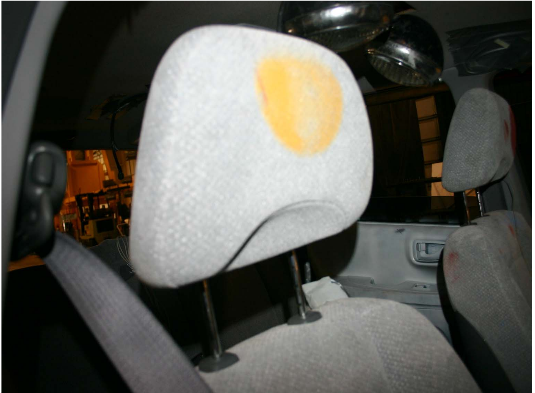
Post-Test Passenger Dummy Head Contact
