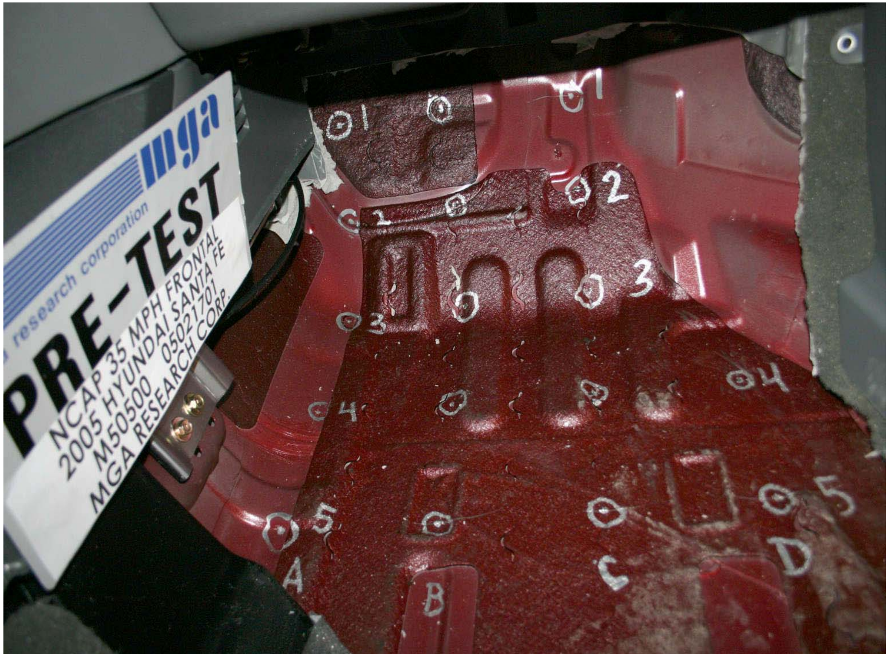
Pre-Test Passenger Side Floor Pan View
