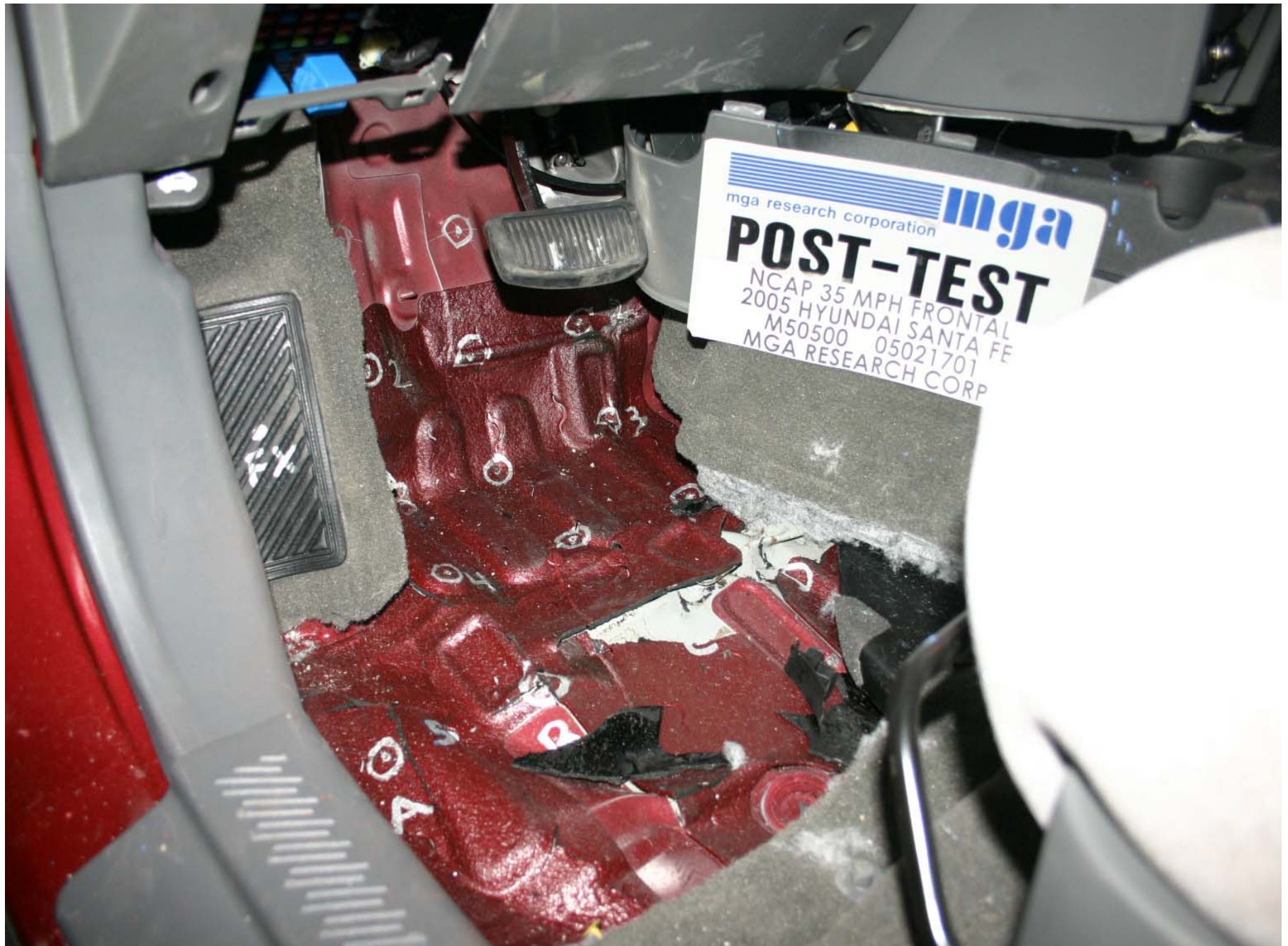
Post-Test Driver Side Floor Pan View
