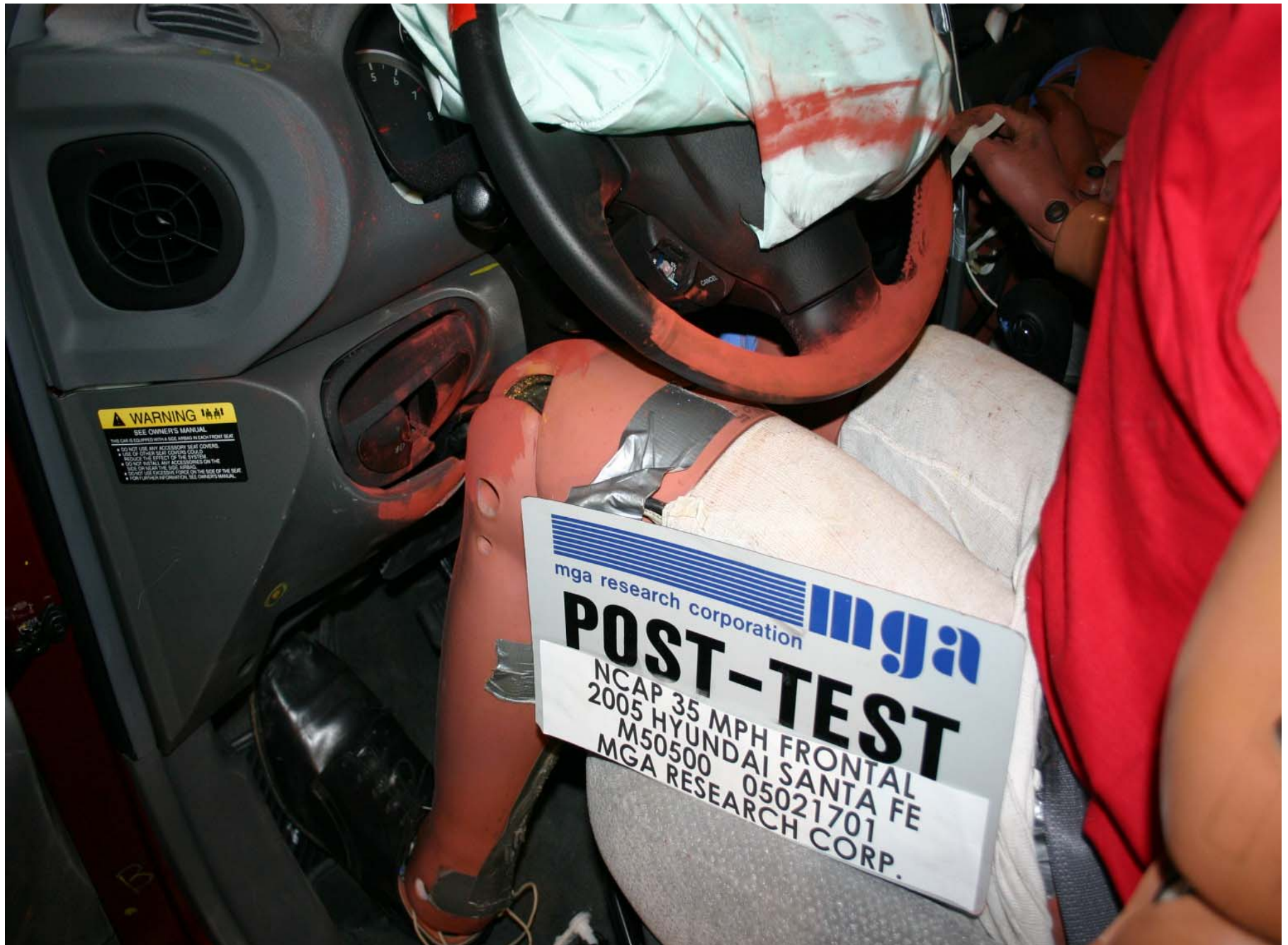
Post-Test Driver Side Knee Bolster View
