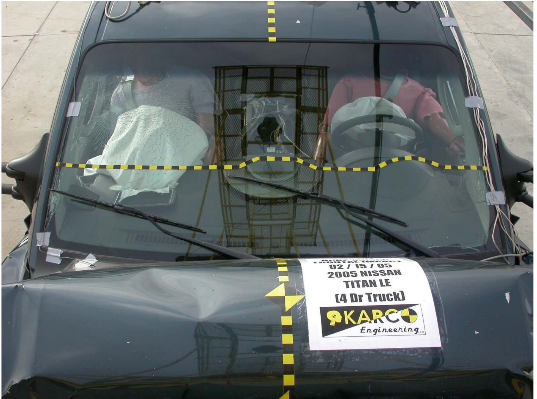
Figure A-18: Post-Test Windshield
