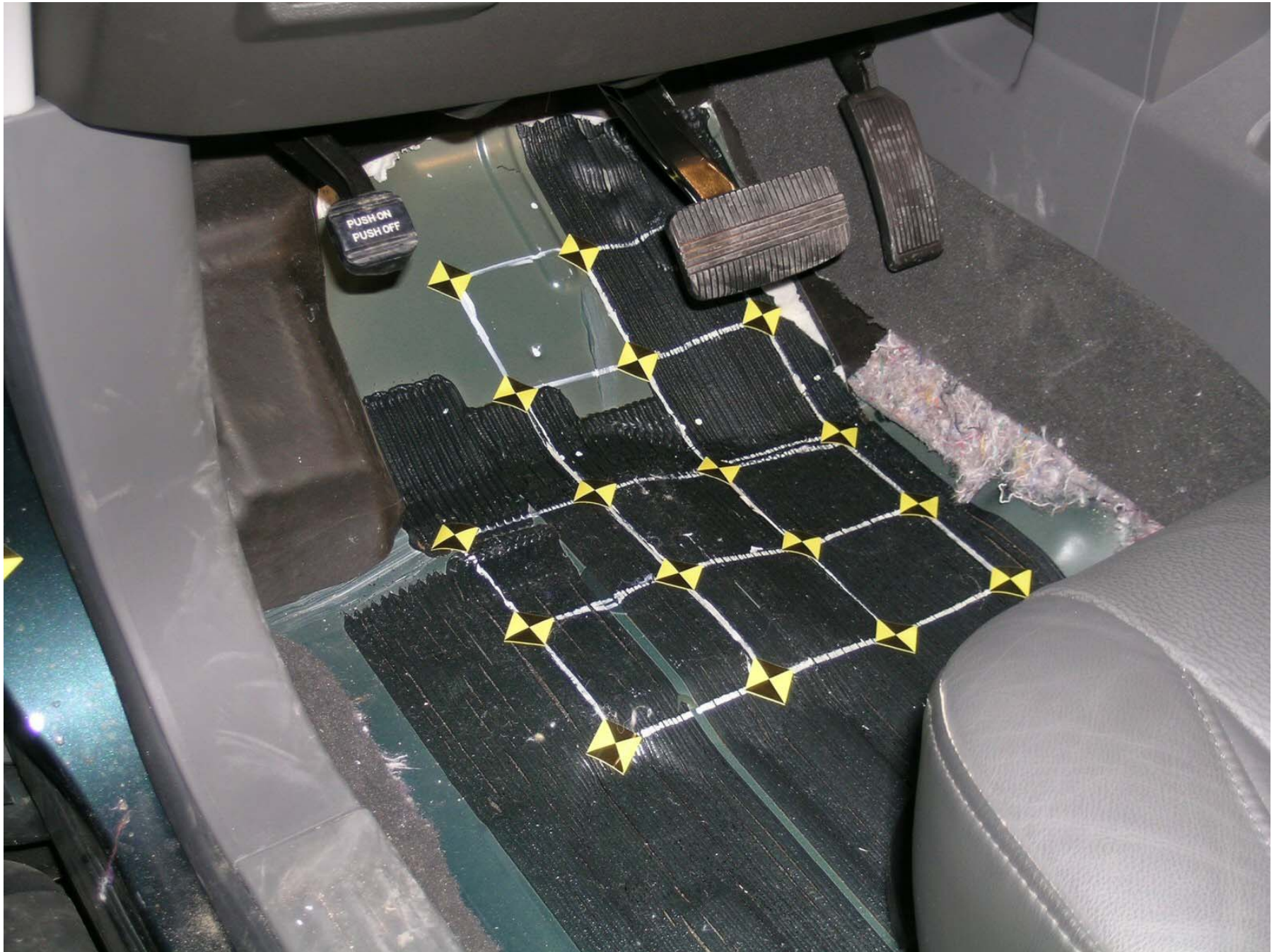
Figure A-39: Pre-Test Driver Side Floor Pan
