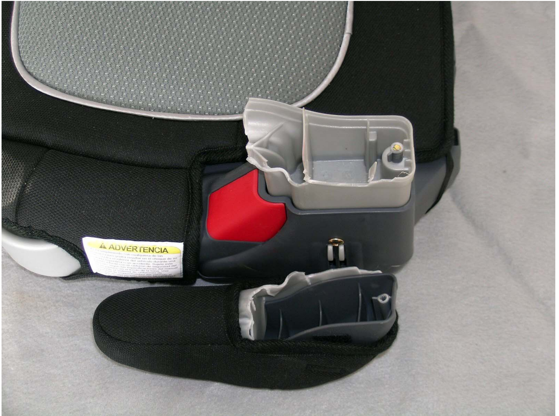
Figure F2-39: Post-Test Position 3 CRS Damage
