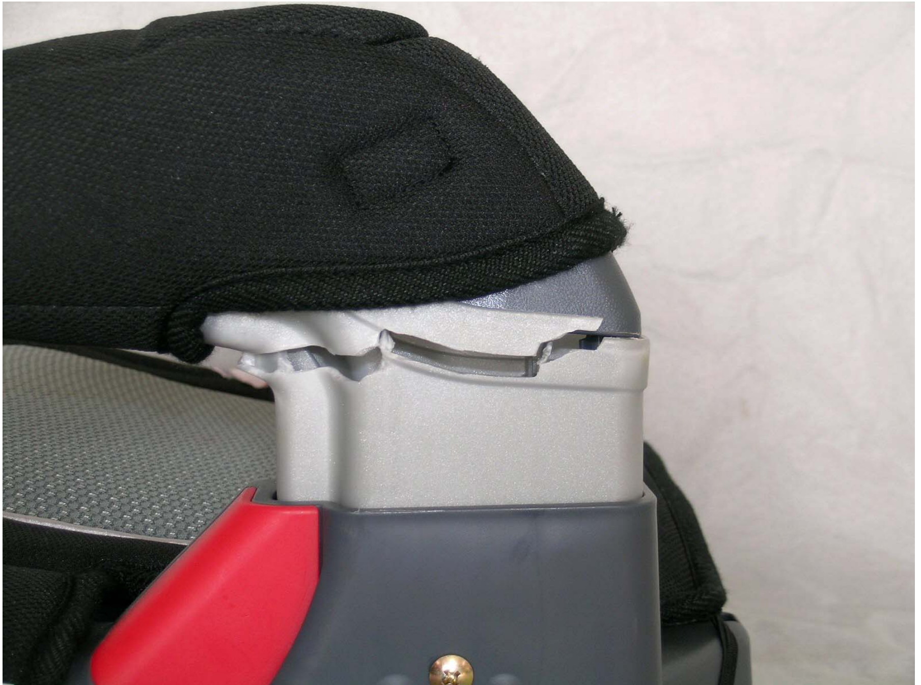
Figure F2-40: Post-Test Position 3 CRS Damage
