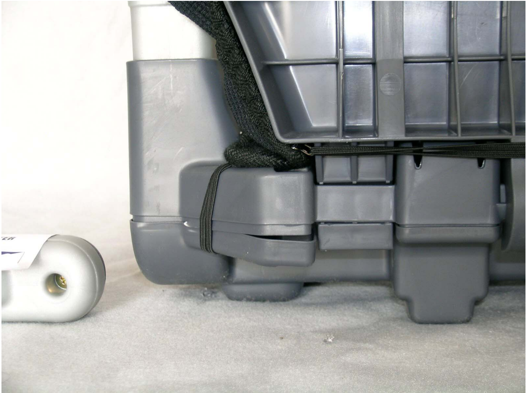
Figure F2-43: Post-Test Position 4 CRS (Base Separation at Left Rear)
