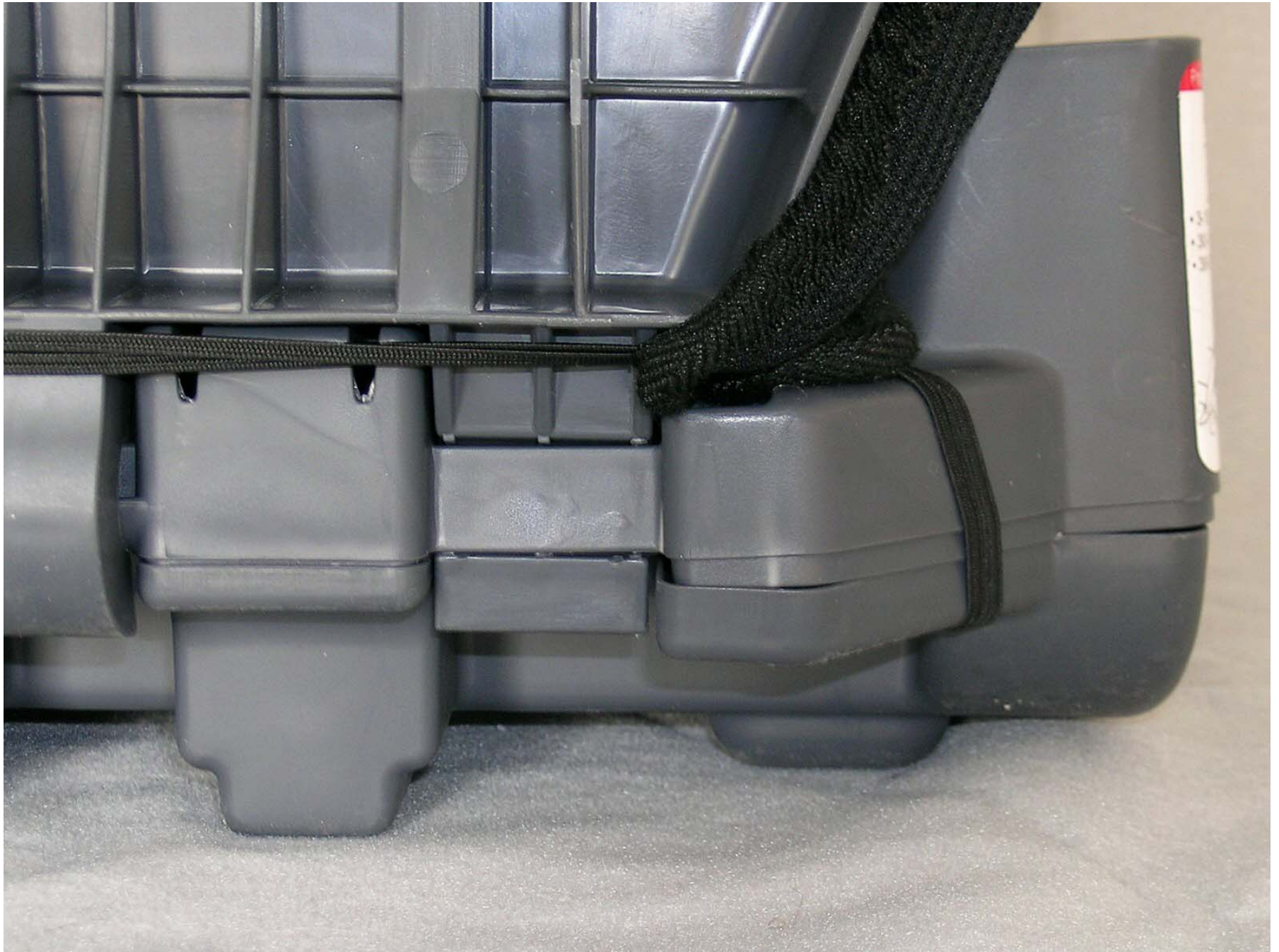
Figure F2-44: Post-Test Position 4 CRS (Base Separation at Right Rear)
