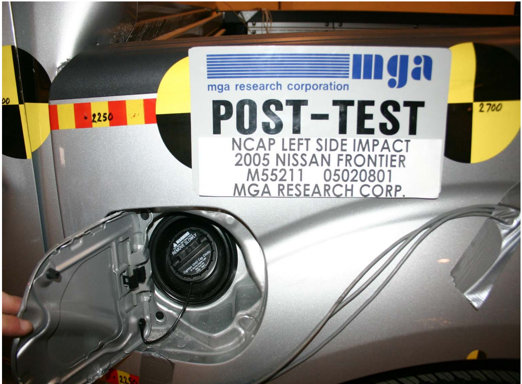
Post-Test Fuel Filler Cap View
