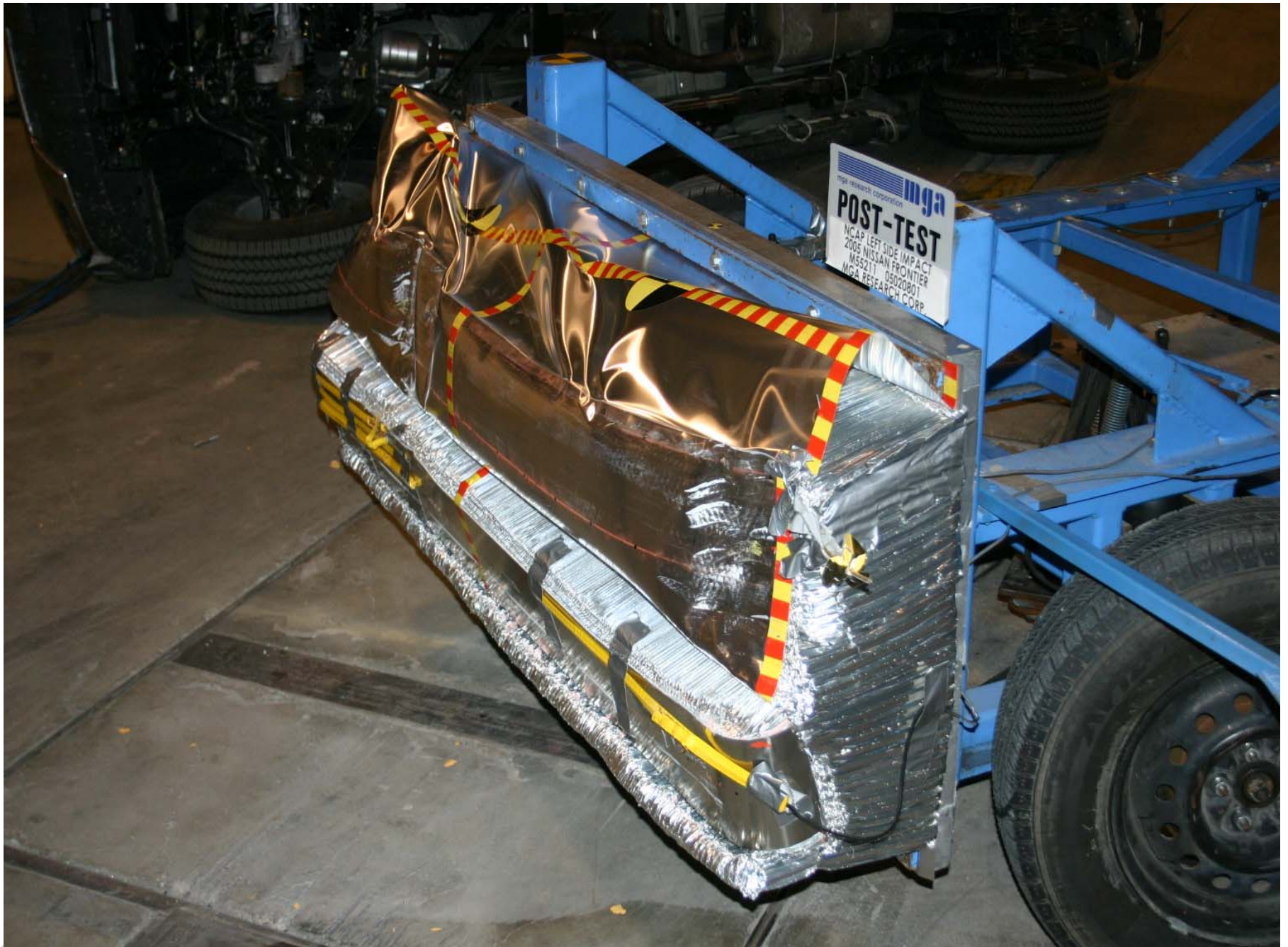
Post-Test MDB Left Side View
