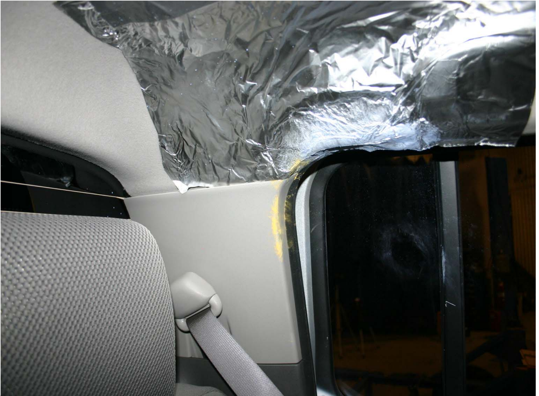
Post-Test Passenger Dummy Head Contact (side header)
