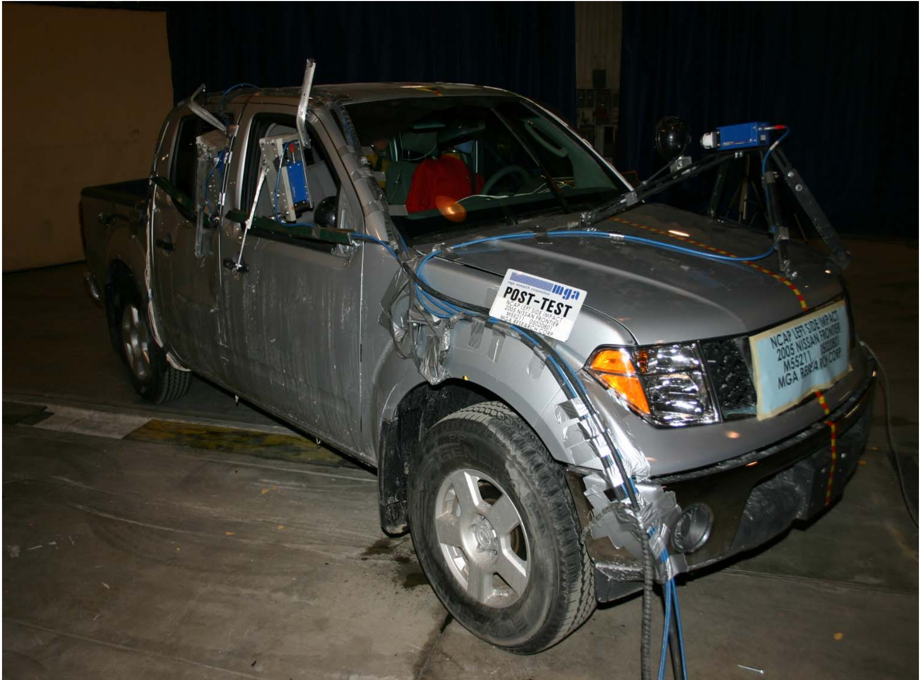
Post-Test Right Front ¾ View of Test Vehicle
