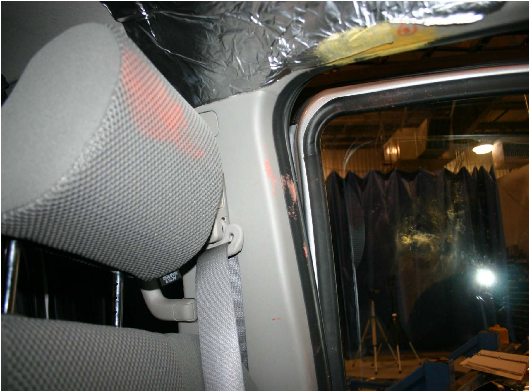
Post-Test Driver Dummy Head Contact (side header & headrest)
