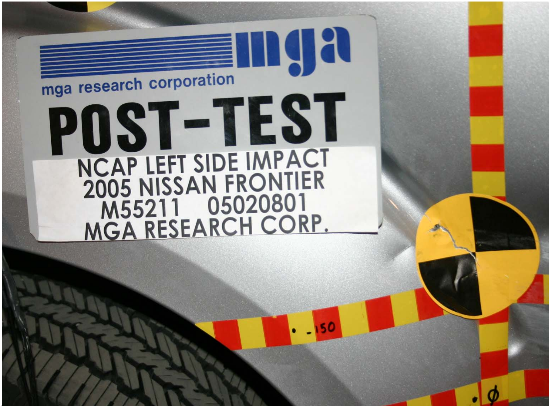
Post-Test Impact Point on Vehicle
