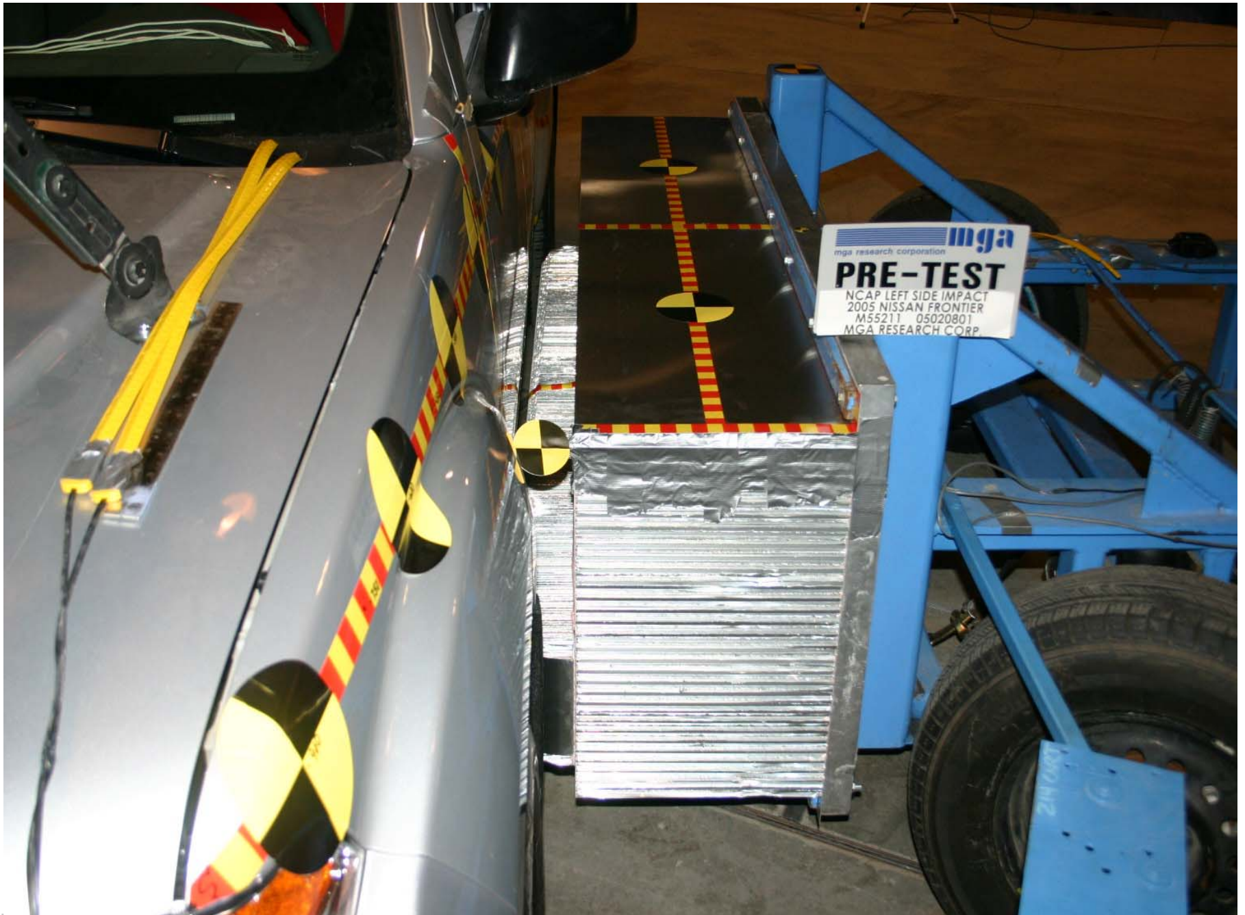
Pre-Test MDB (Left Side) Positioned Against Vehicle
