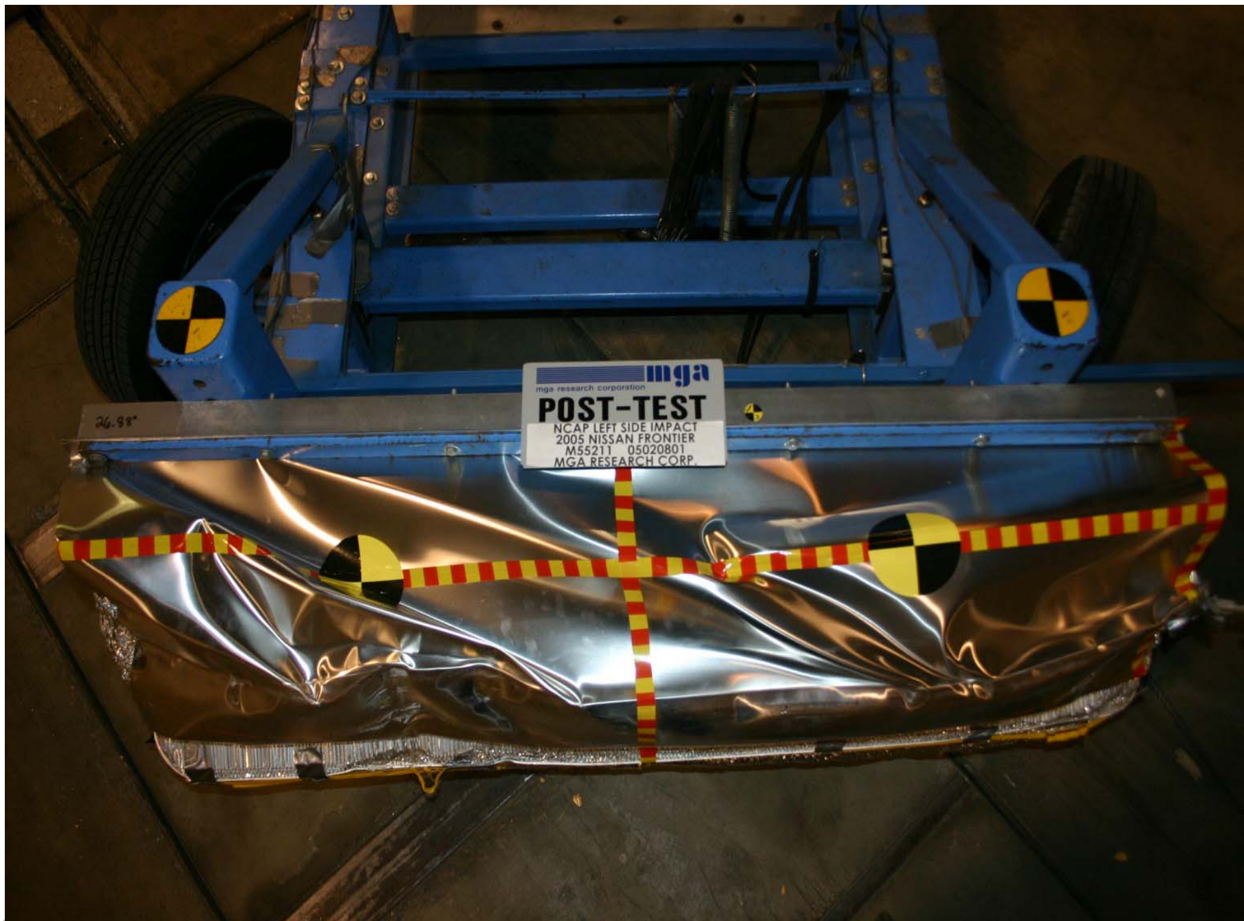
Post-Test MDB Top View
