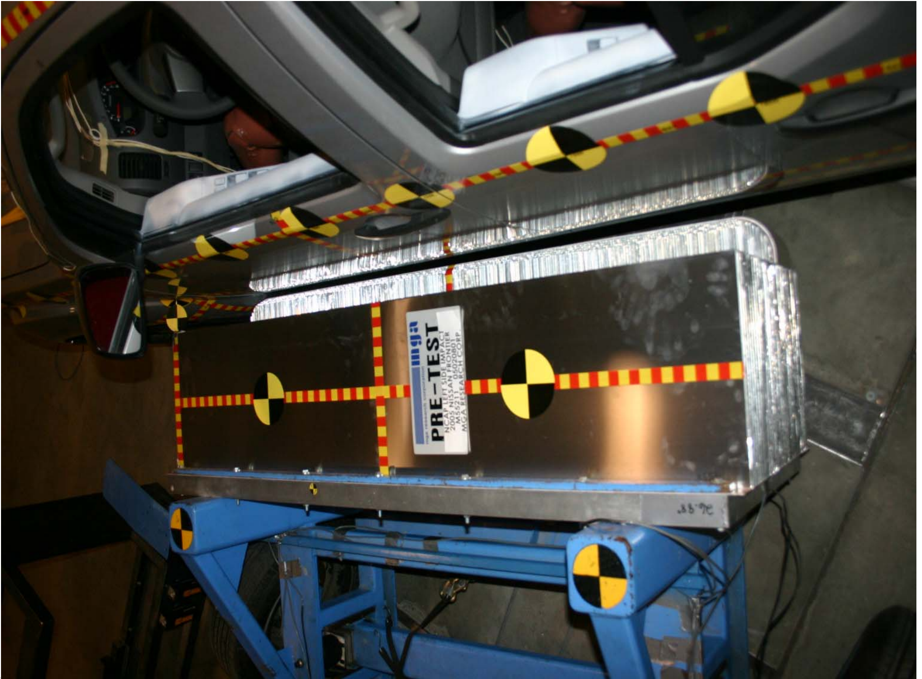
Pre-Test MDB Positioned Against Vehicle Overhead View
