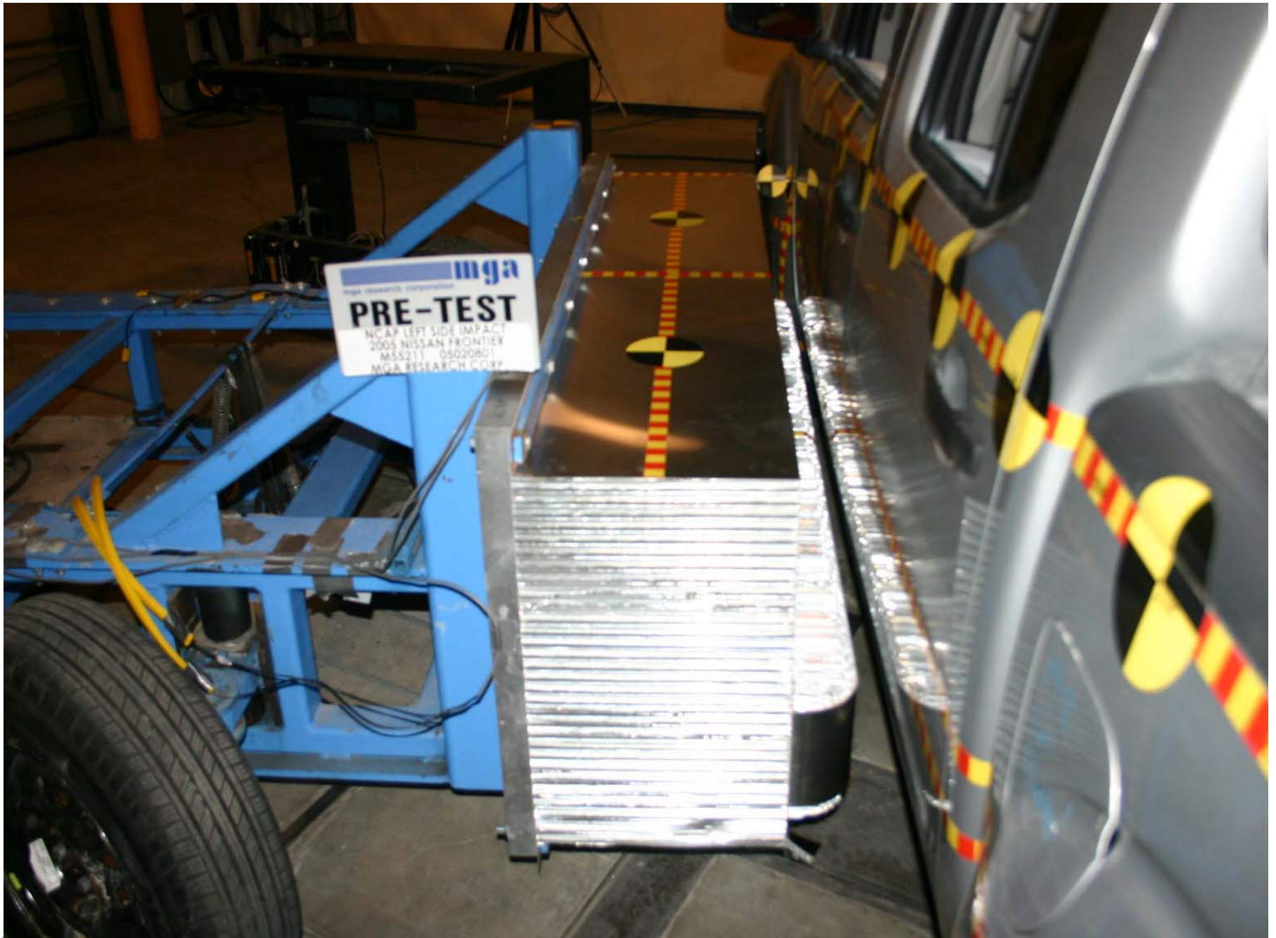
Pre-Test MDB (Right Side) Positioned Against Vehicle
