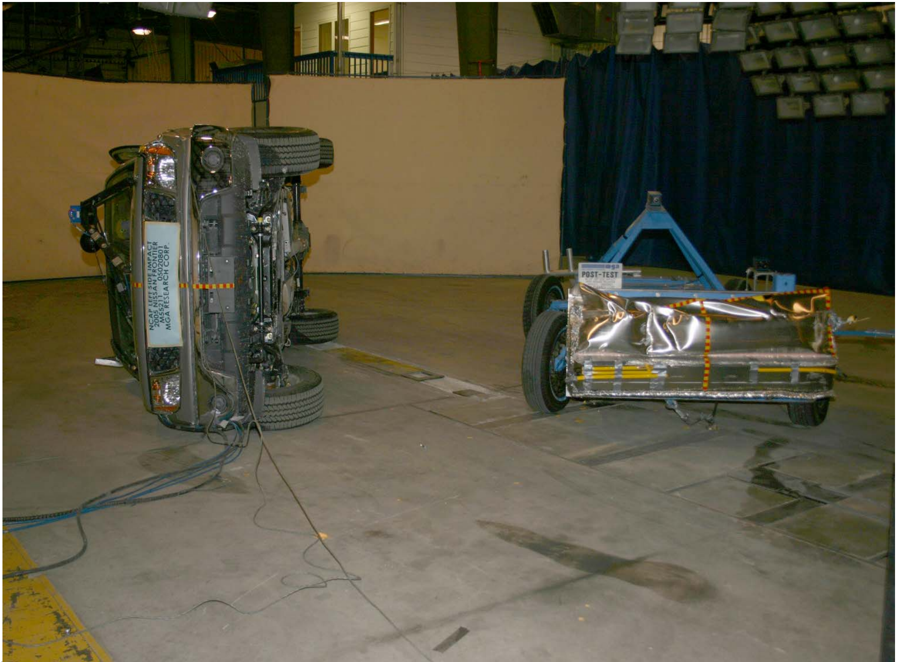
Post-Test MDB (Front) and Vehicle
