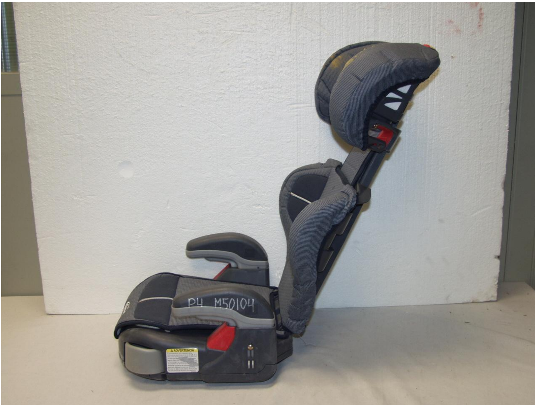
Figure 3-16 POST-TEST LEFT SIDE VIEW OF POSITION 4 CRS
