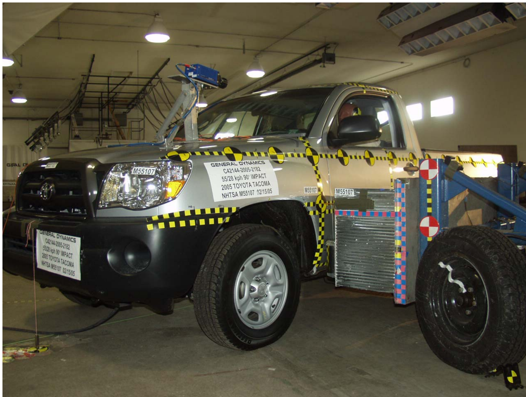
Figure A-31 PRE-TEST LEFT SIDE VIEW OF MDB WITH IMPACTOR FACE IN POSITION
