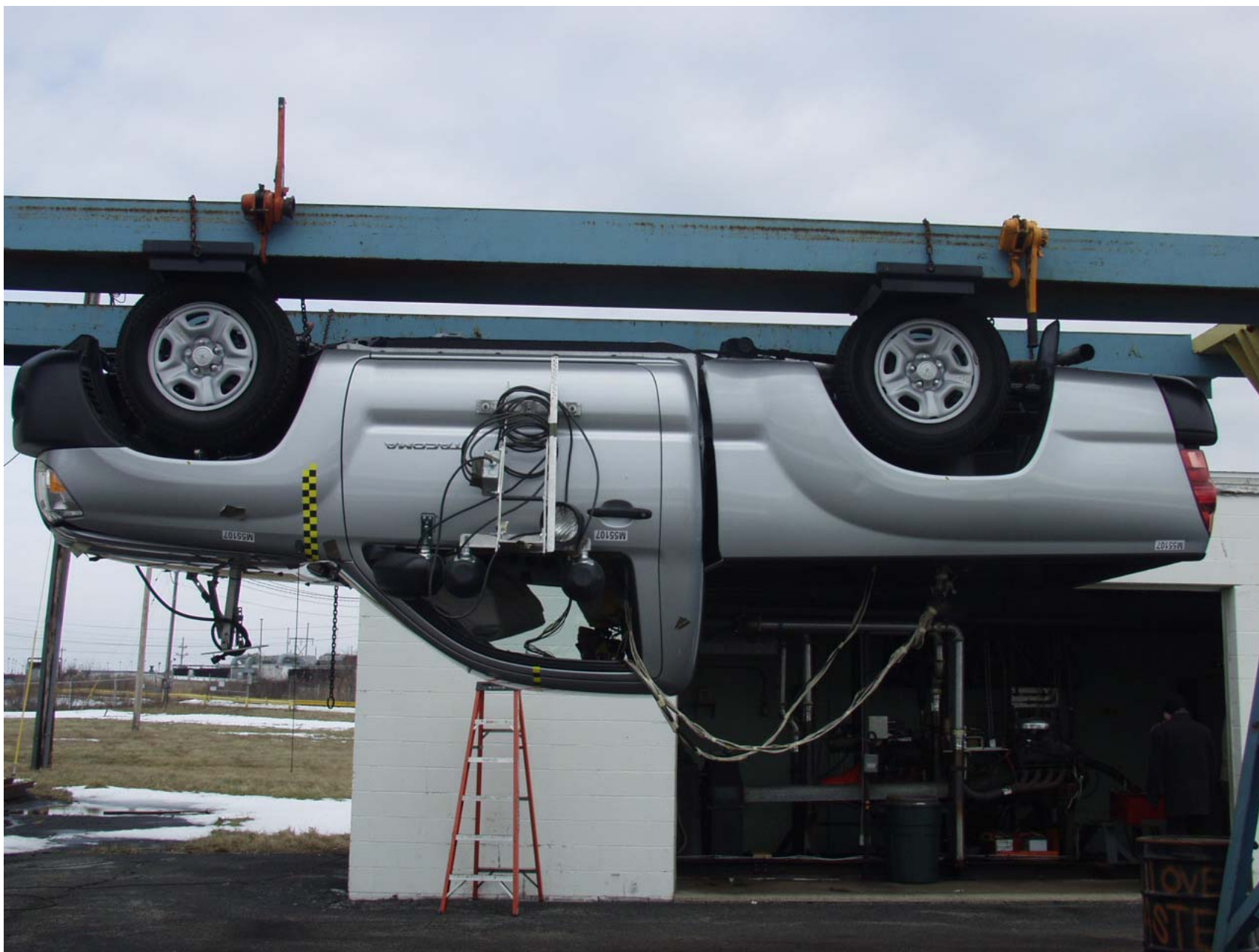
Figure A-38 ROLLOVER 180 DEGREES
