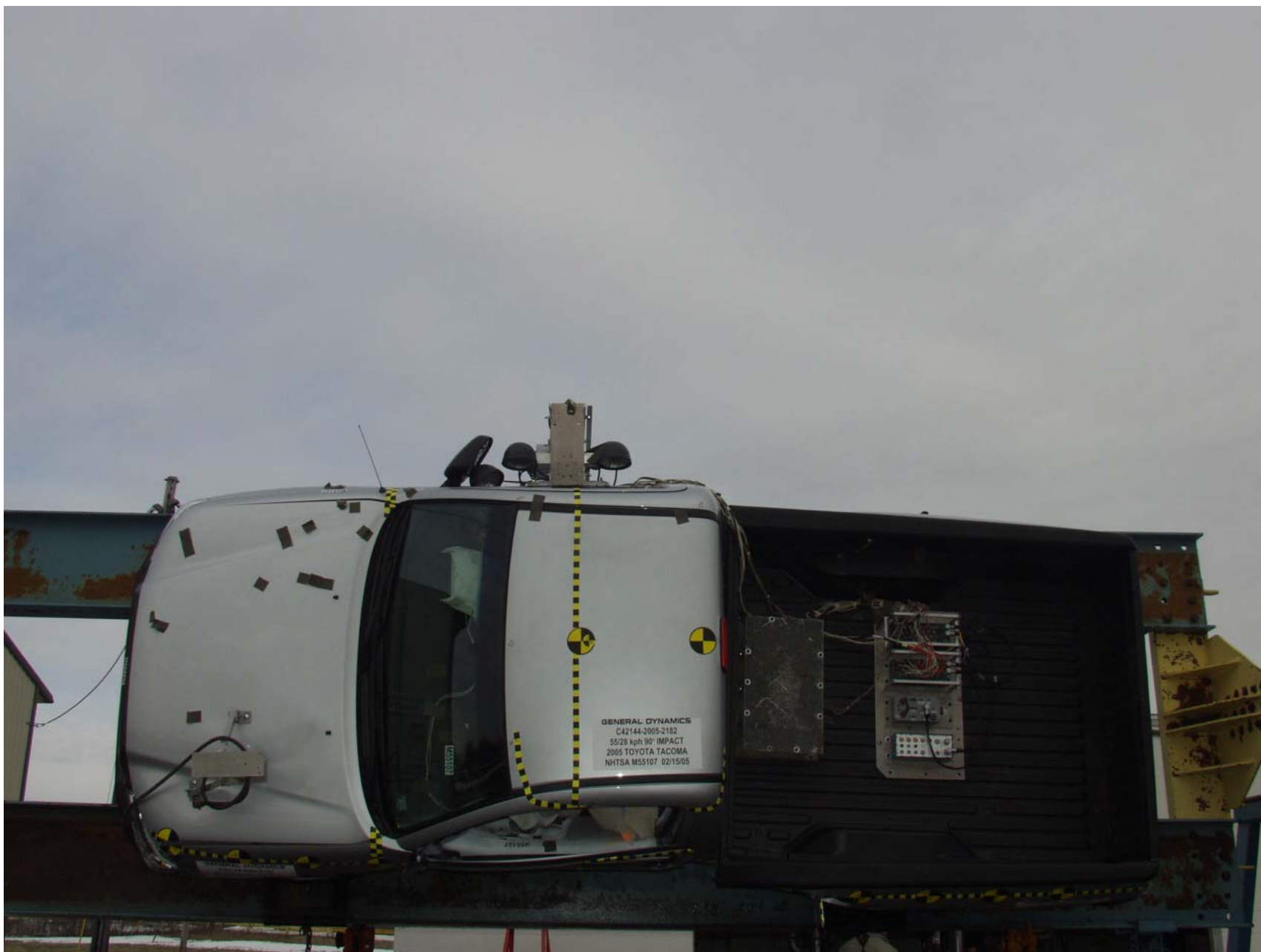
Figure A-37 ROLLOVER 90 DEGREES
