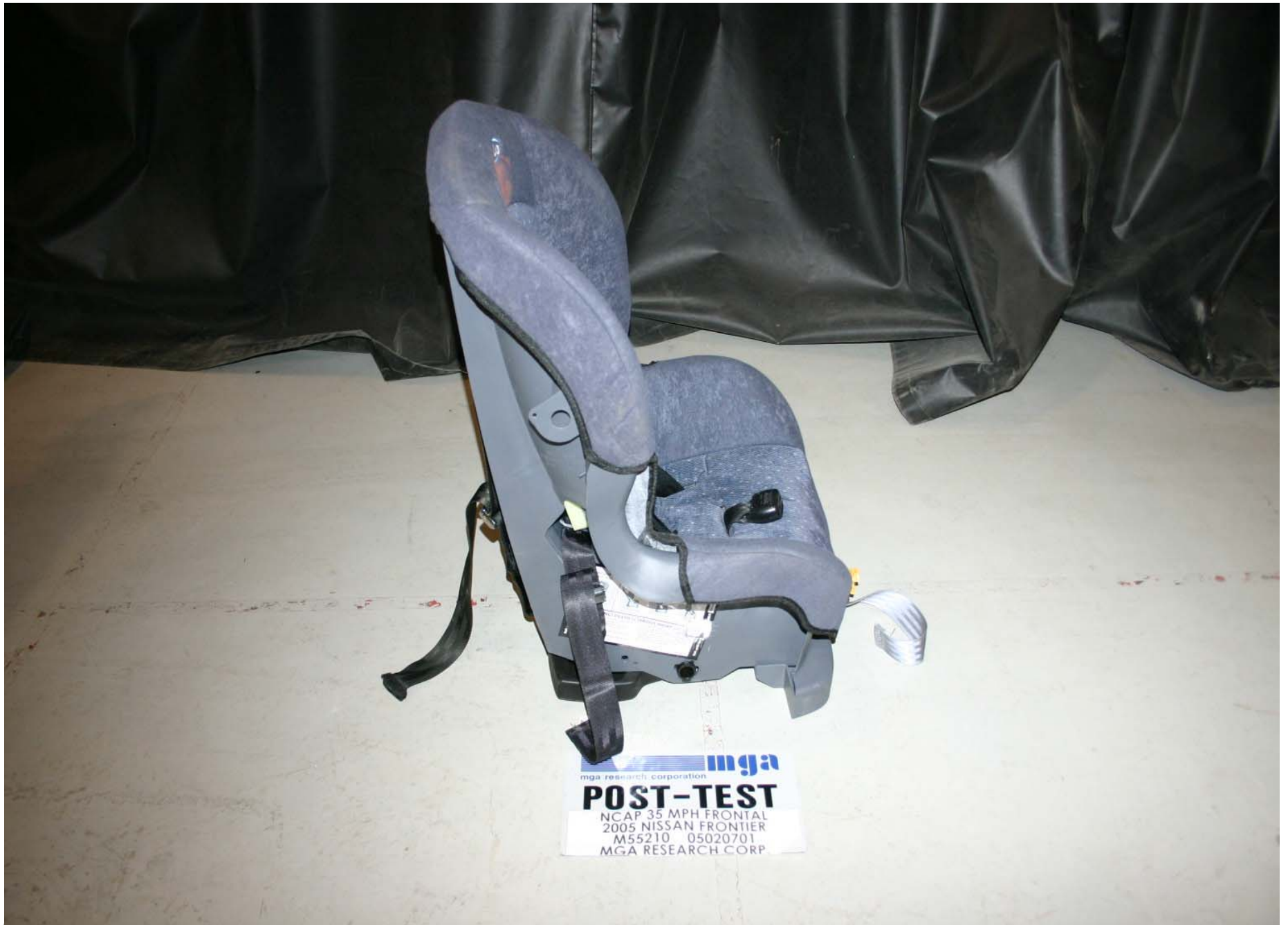
Post-Test Right Side View of Position 3 CRS
