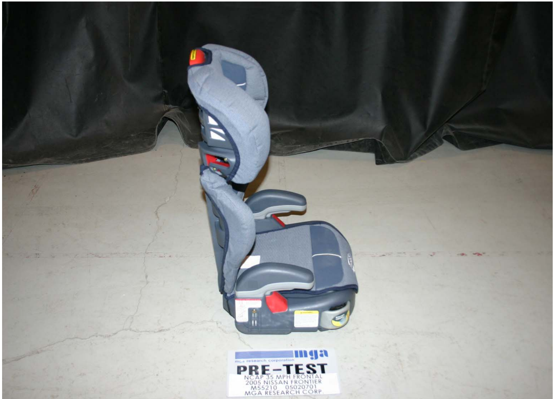
Pre-Test Right Side View of Position 4 CRS
