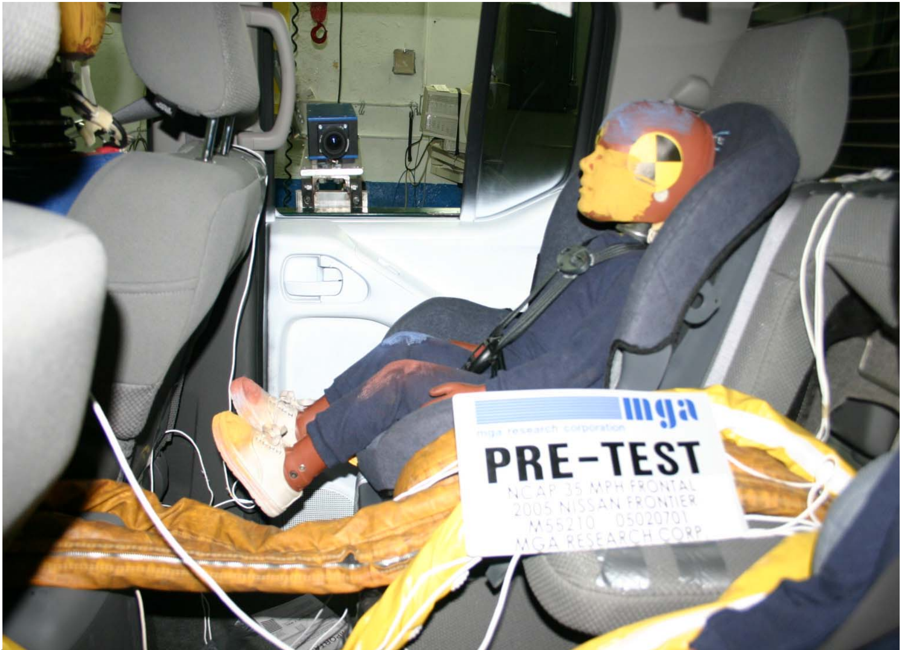
Pre-Test Position 3 Left Side View
