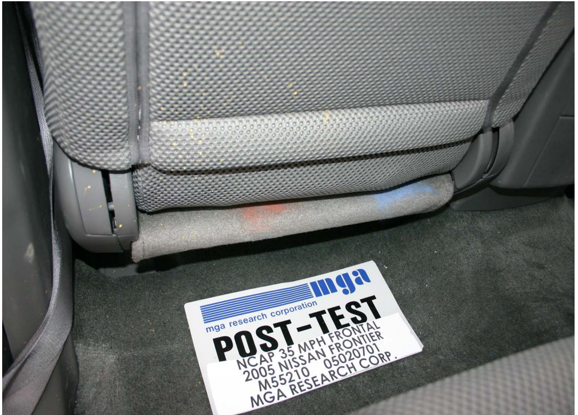
Post-Test Position 4 Feet Contact
