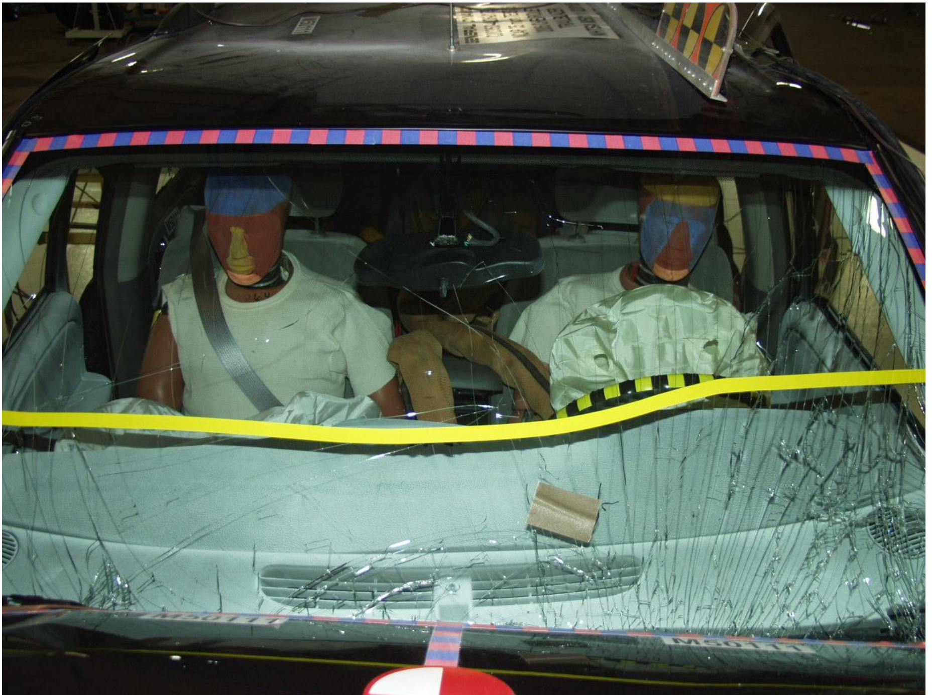
Figure A-19 POST-TEST WINDSHIELDVIEW
