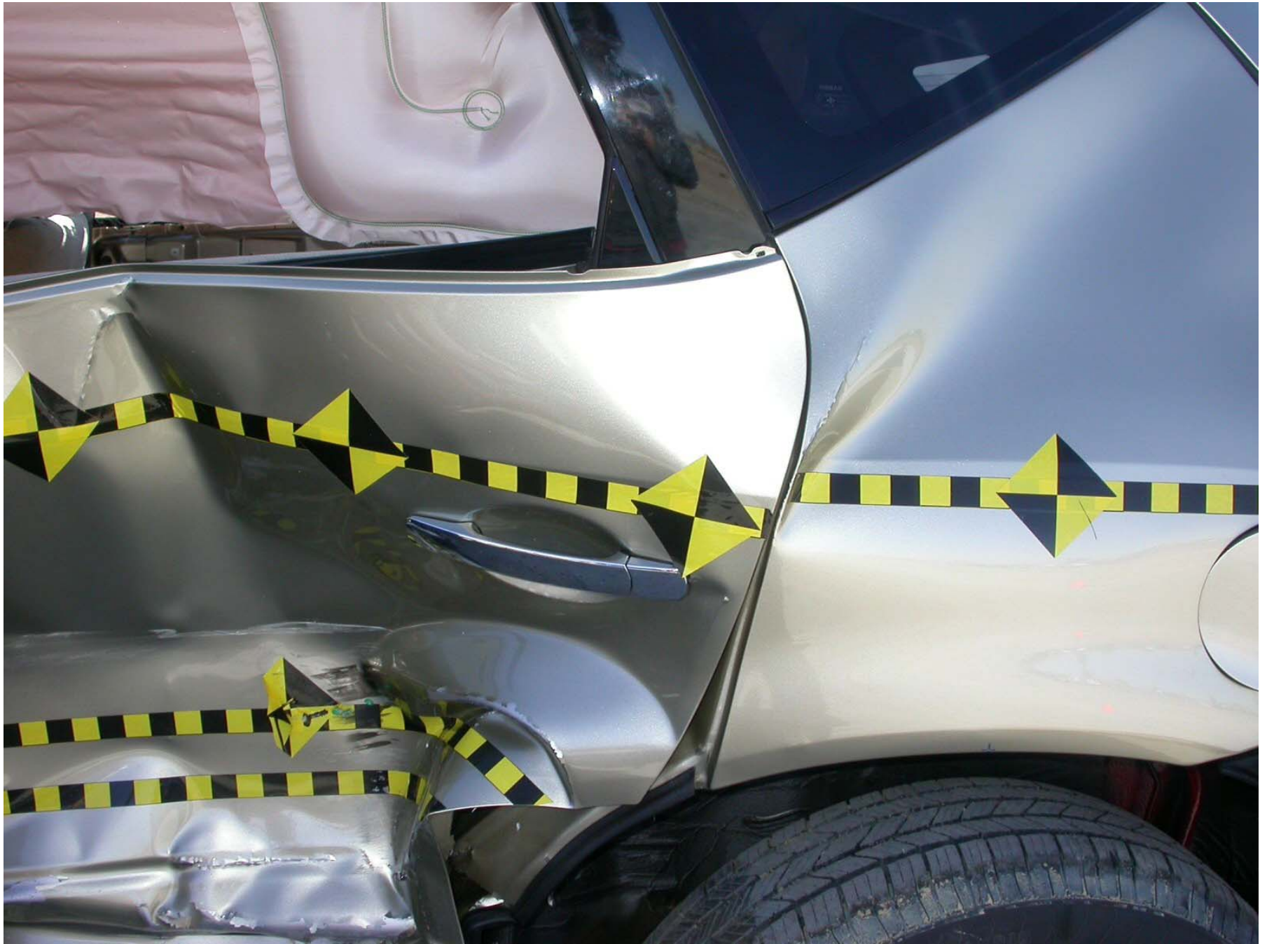
Figure A-34: Post-Test Left Rear Door
