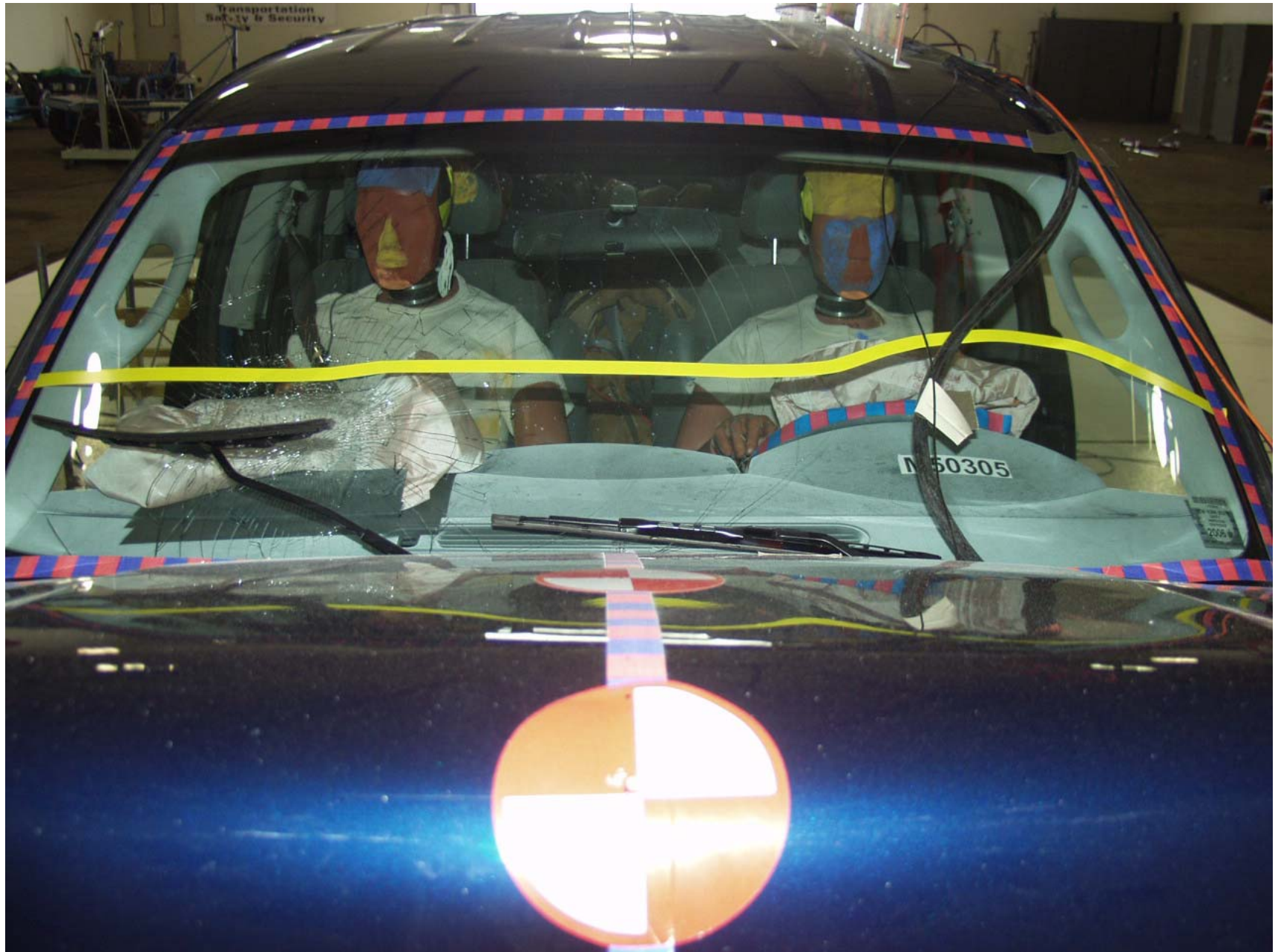
Figure A-19 POST-TEST WINDSHIELDVIEW
