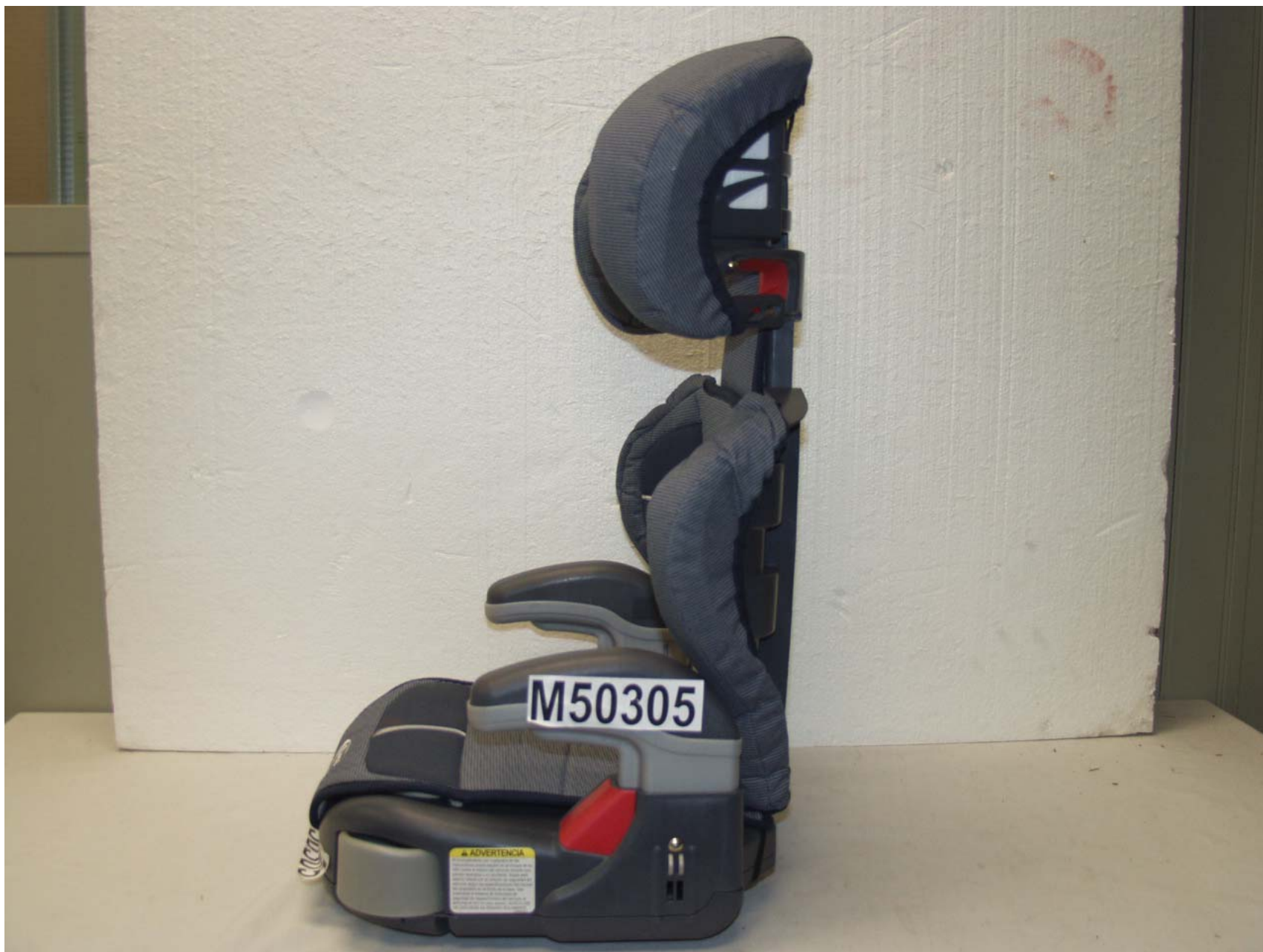
Figure 3-16 POST-TEST LEFT SIDE VIEW OF POSITION 4 CRS
