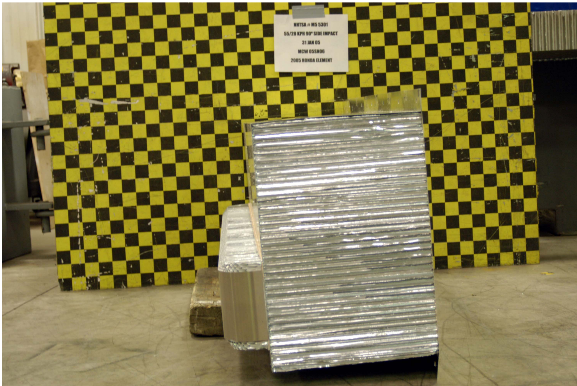
Figure A-49: PRE-TEST ALUMINUM BARRIER LEFT SIDE
