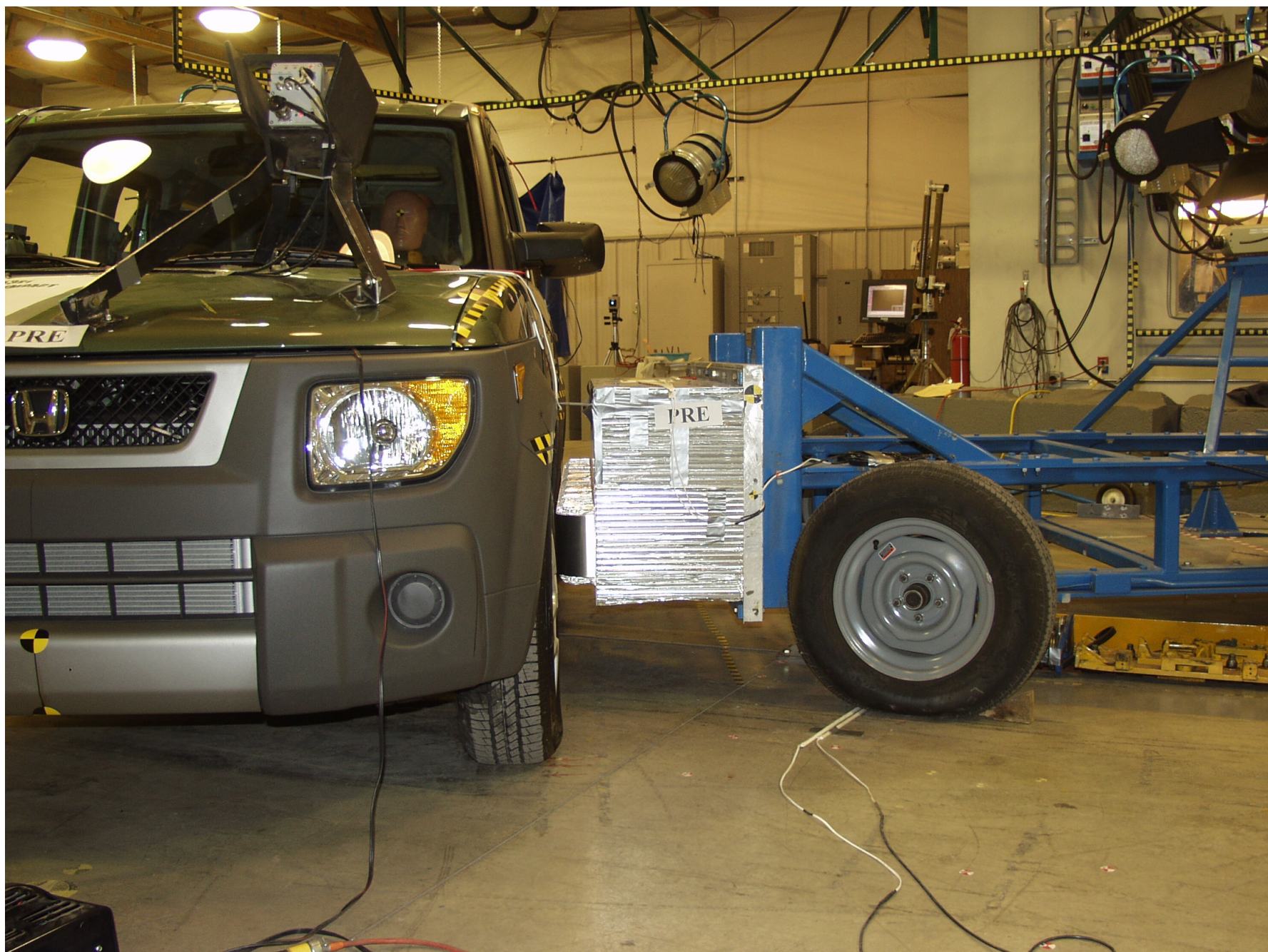
Figure A-31: PRE TEST LEFT SIDE VIEW OF MDB IN IMPACT POSITION
