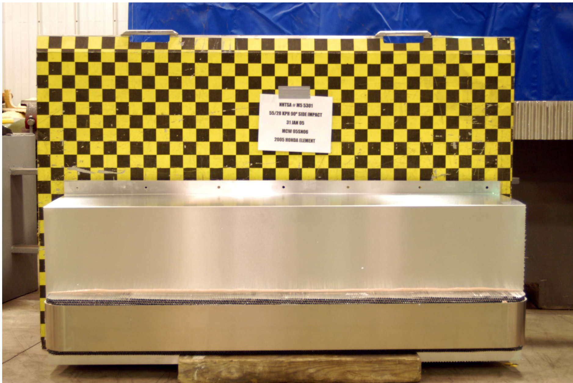
Figure A-47: PRE-TEST ALUMINUM BARRIER FRONT
