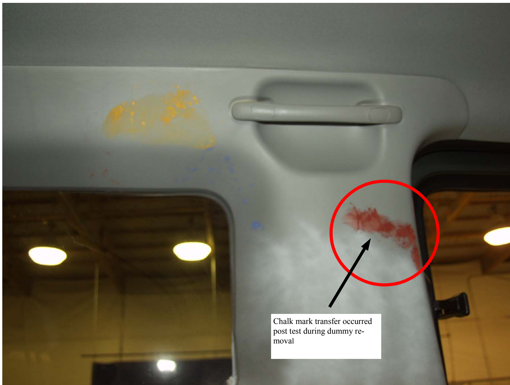
Figure A-30: POST-TEST INTERIOR OF REAR DOOR SHOWING SID H3 IMPACT LOCATIONS 2
