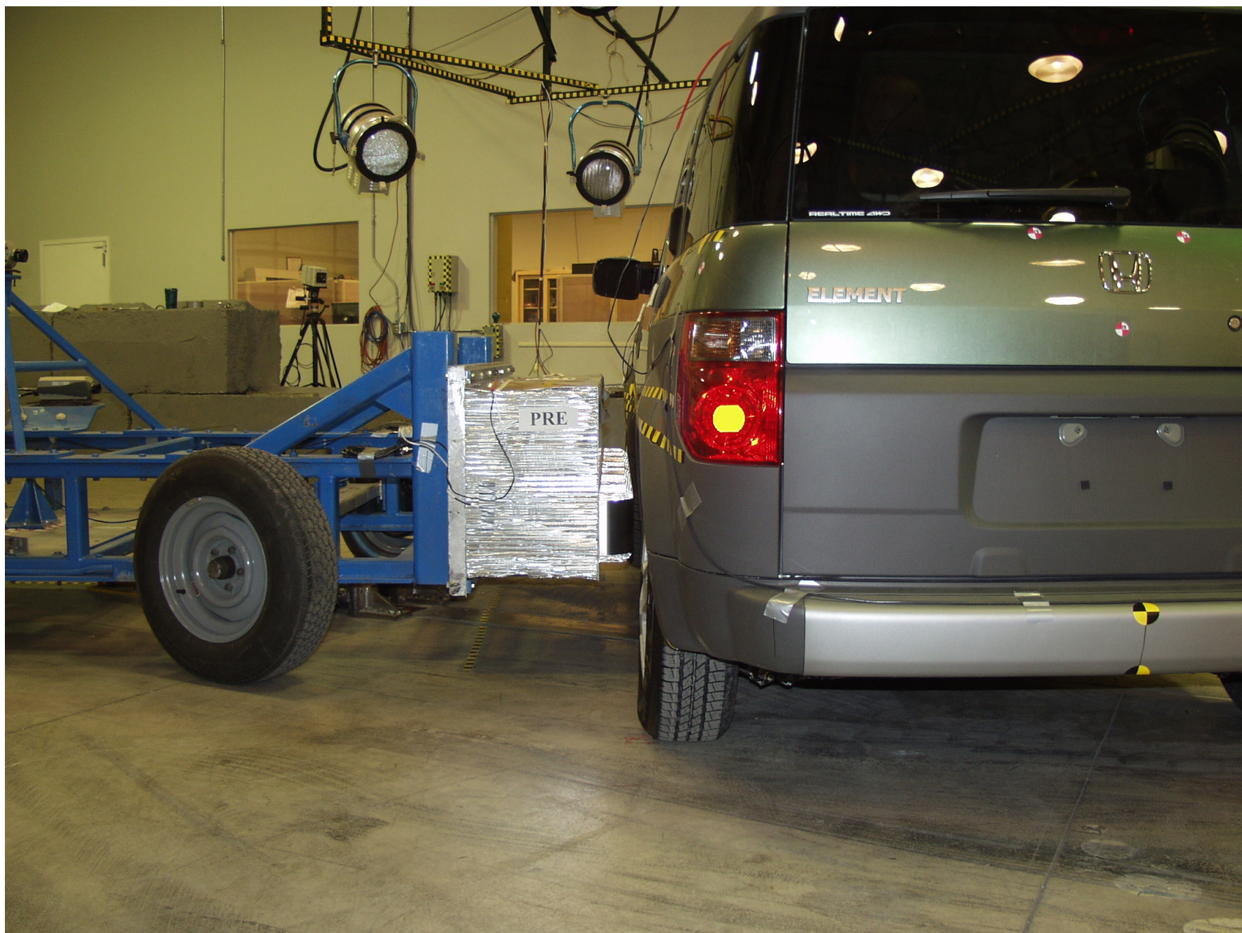
Figure A-33: PRE TEST RIGHT SIDE VIEW OF MDB IN IMPACT POSITION
