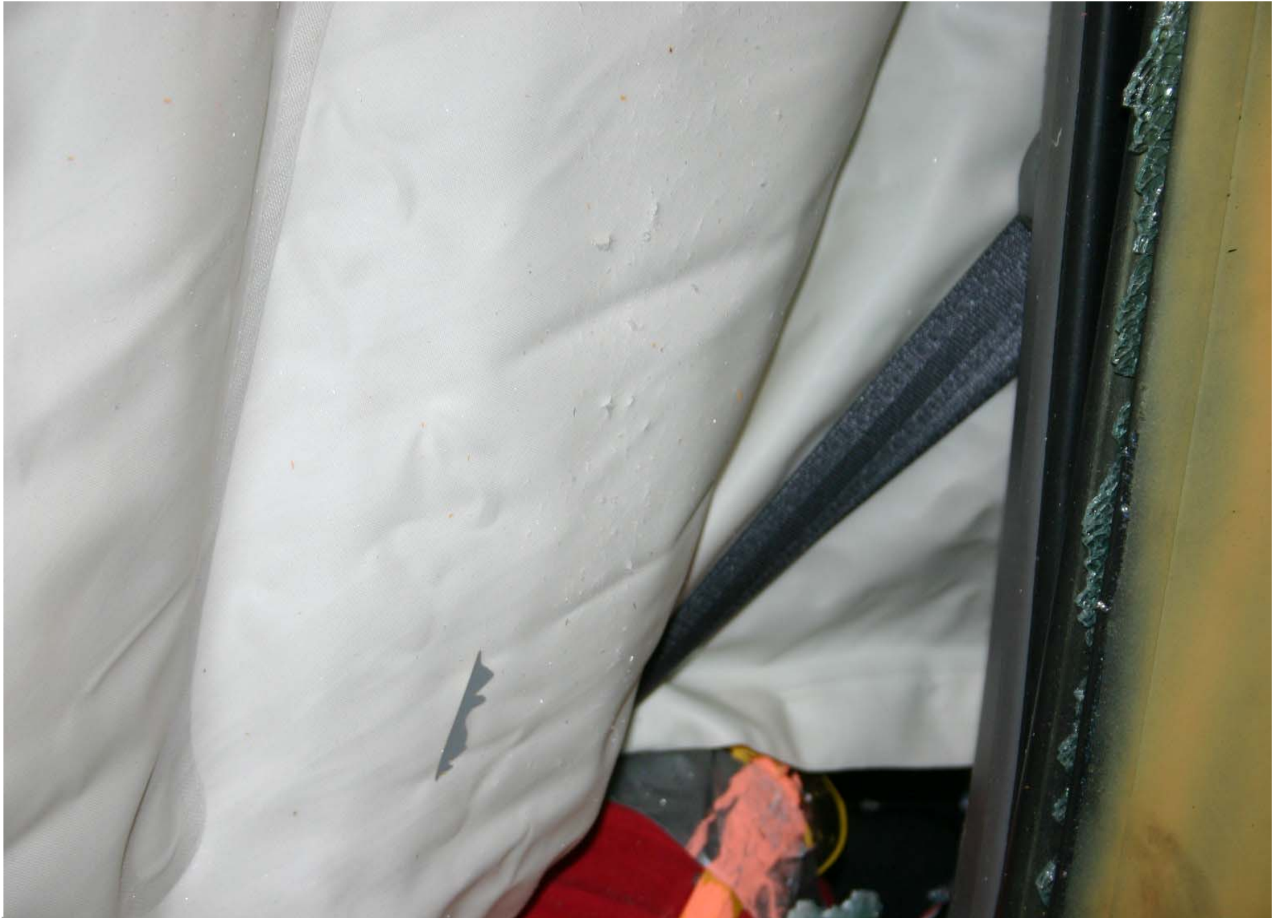
Post-Test Hole in Curtain Airbag
