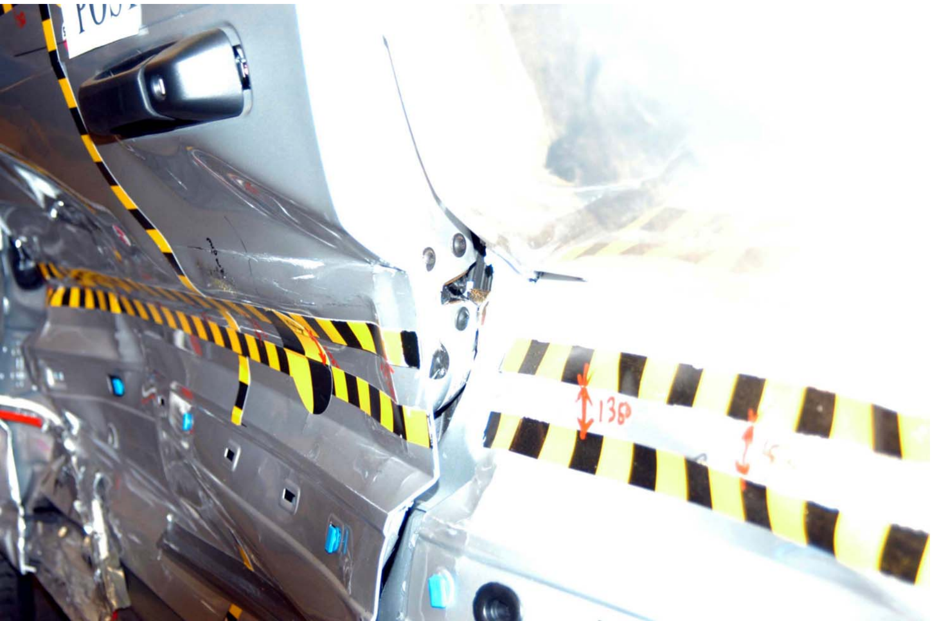
Figure A-18: POST-TEST UNLATCHED DRIVER DOOR 2
