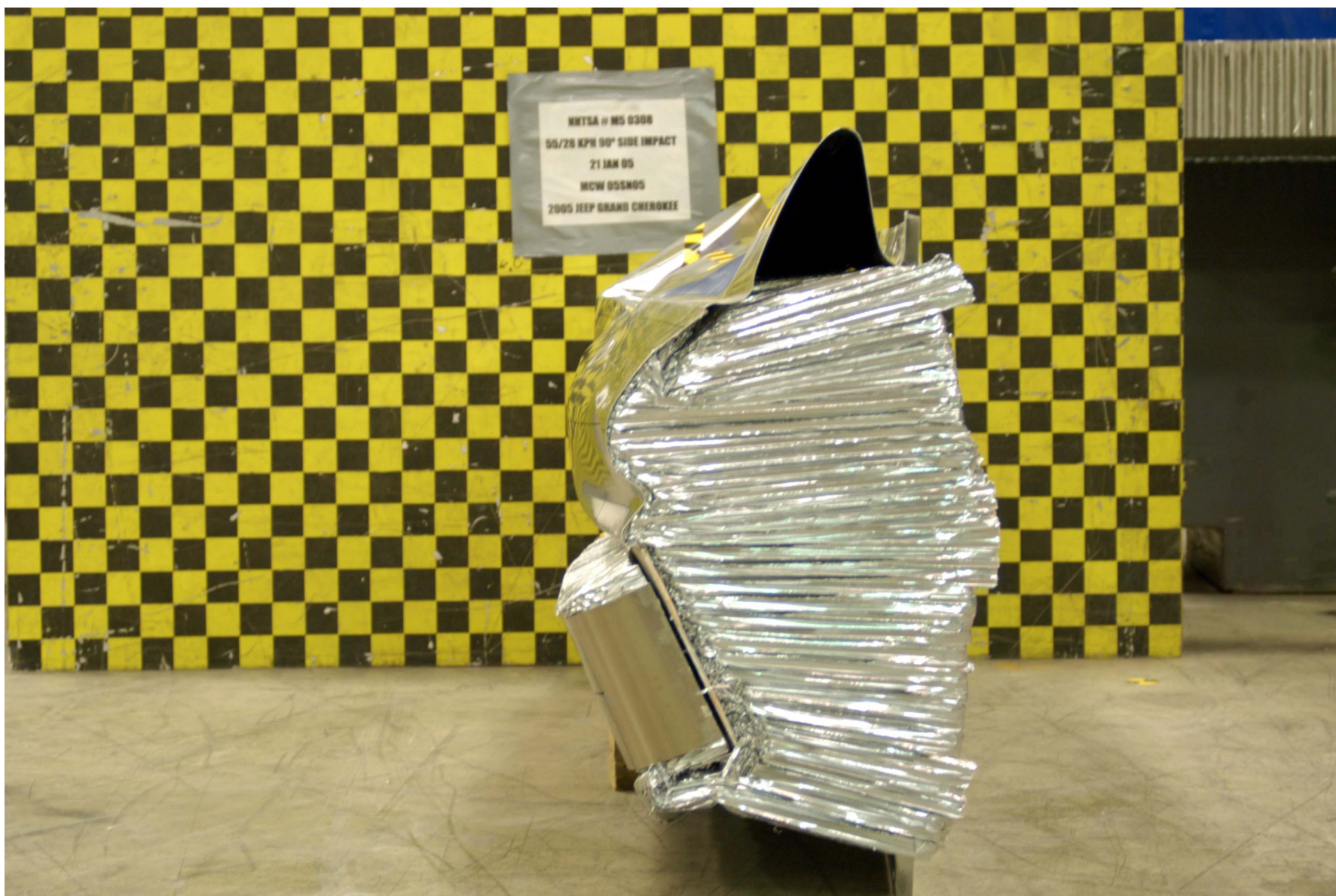
Figure A-52: POST-TEST ALUMINUM BARRIER LEFT SIDE
