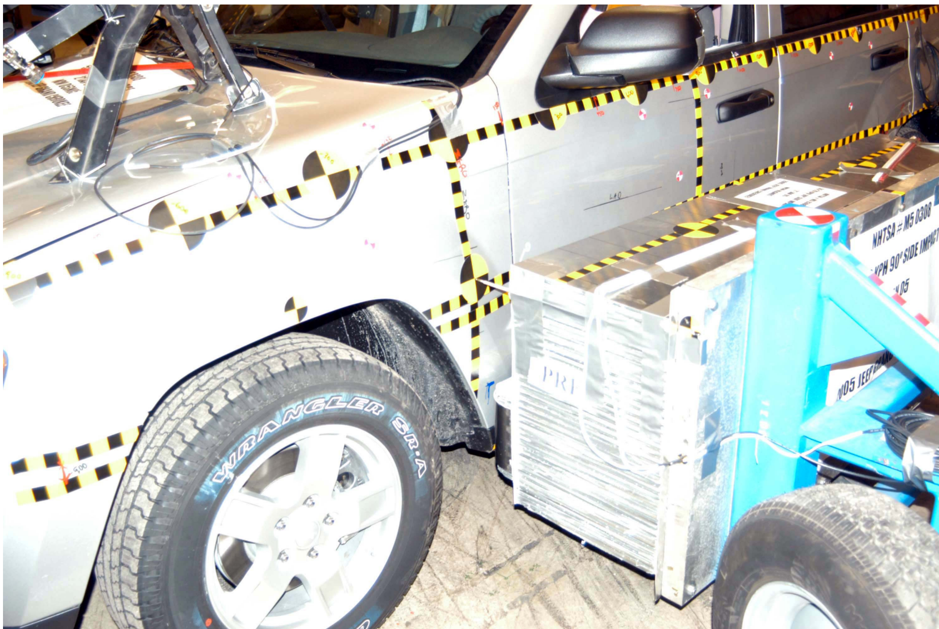
Figure A-39: PRE TEST CLOSE-UP OF IMPACT POINT TARGET SHOWING WELDING ROD
