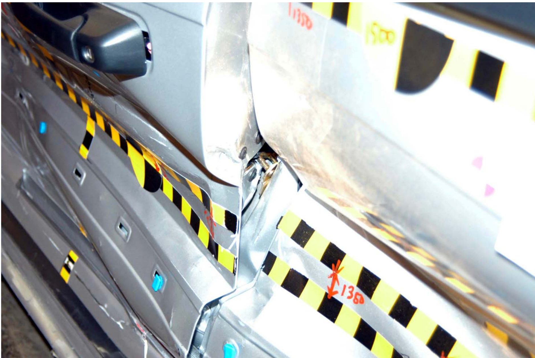
Figure A-17: POST-TEST UNLATCHED DRIVER DOOR
