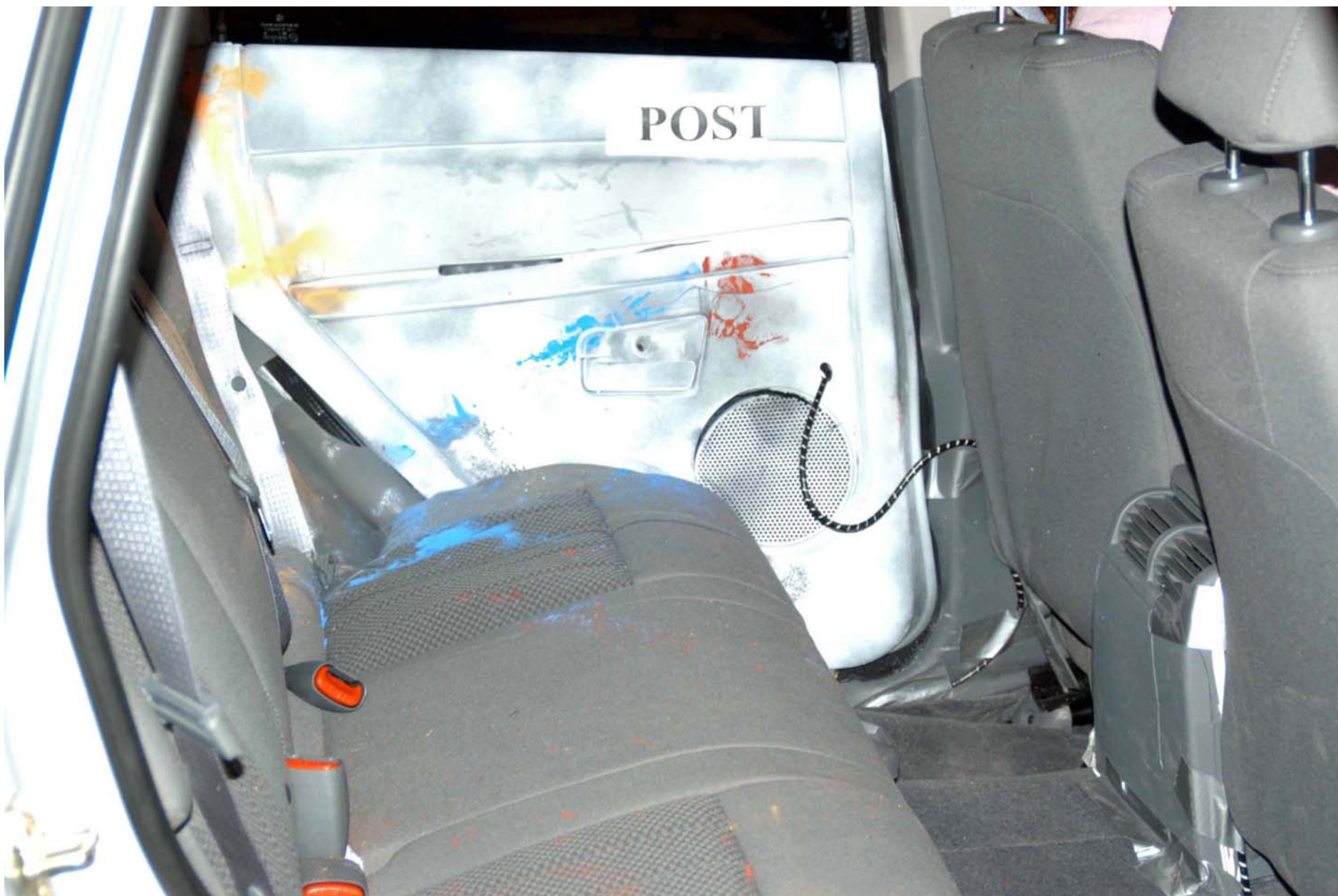
Figure A-32: POST-TEST INTERIOR OF REAR DOOR SHOWING SID H3 IMPACT LOCATIONS 2
