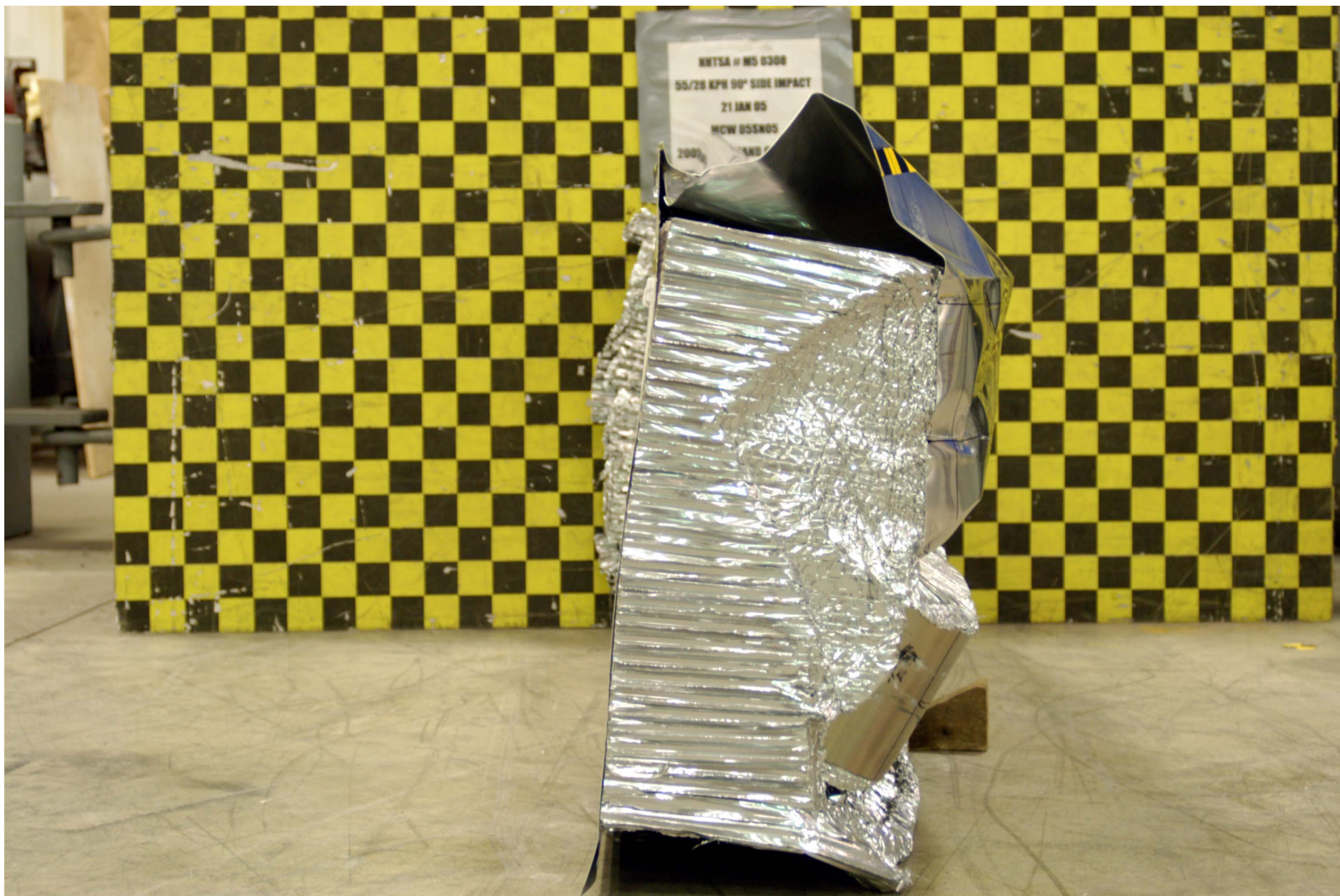
Figure A-54: POST-TEST ALUMINUM BARRIER RIGHT SIDE
