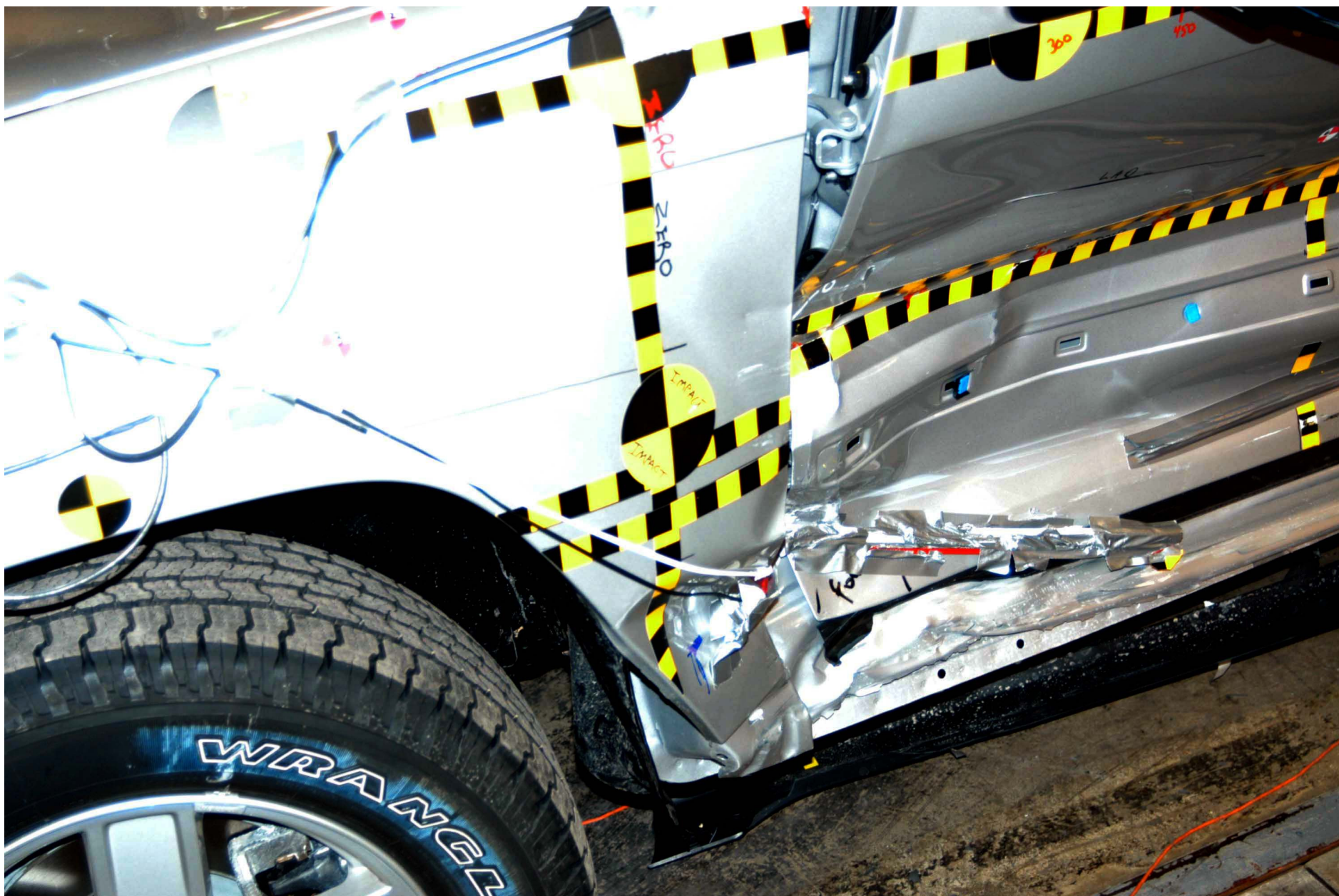
Figure A-40: POST TEST CLOSE-UP OF IMPACT POINT TARGET
