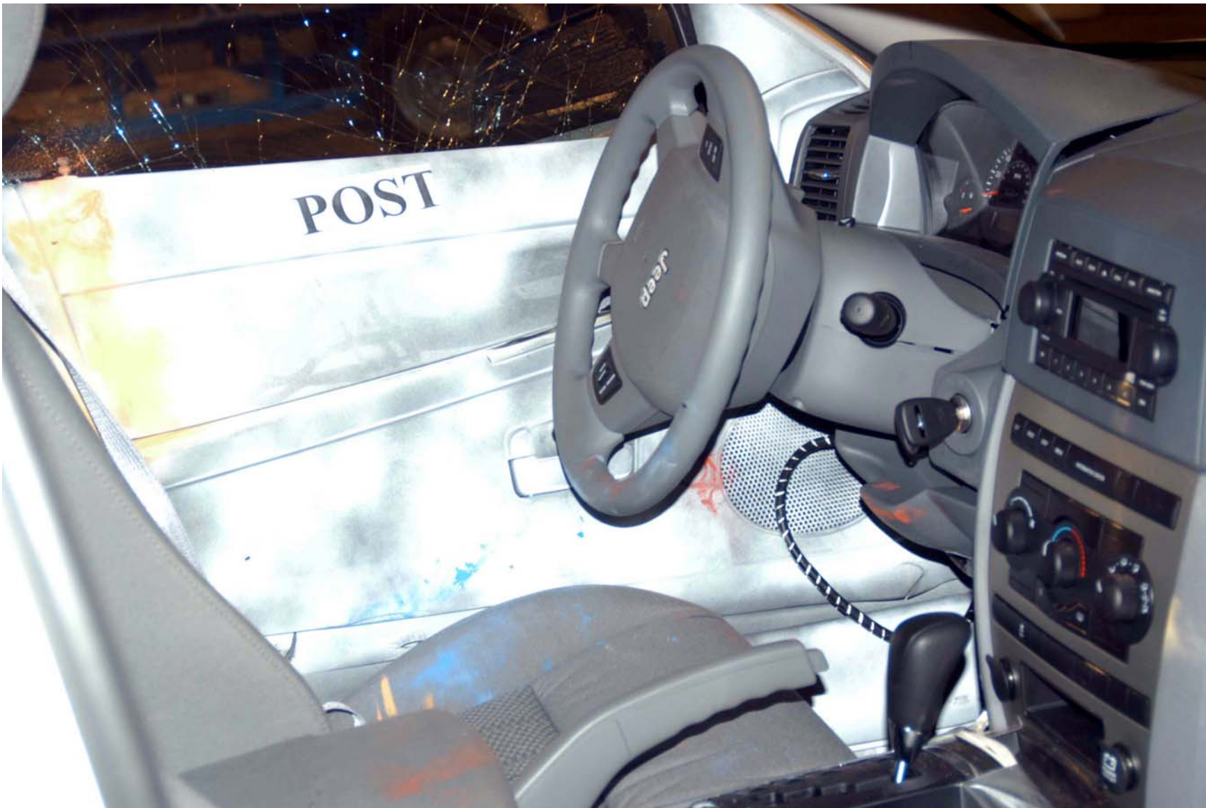
Figure A-29: POST-TEST INTERIOR OF FRONT DOOR SHOWING SID H3 IMPACT LOCATIONS 2
