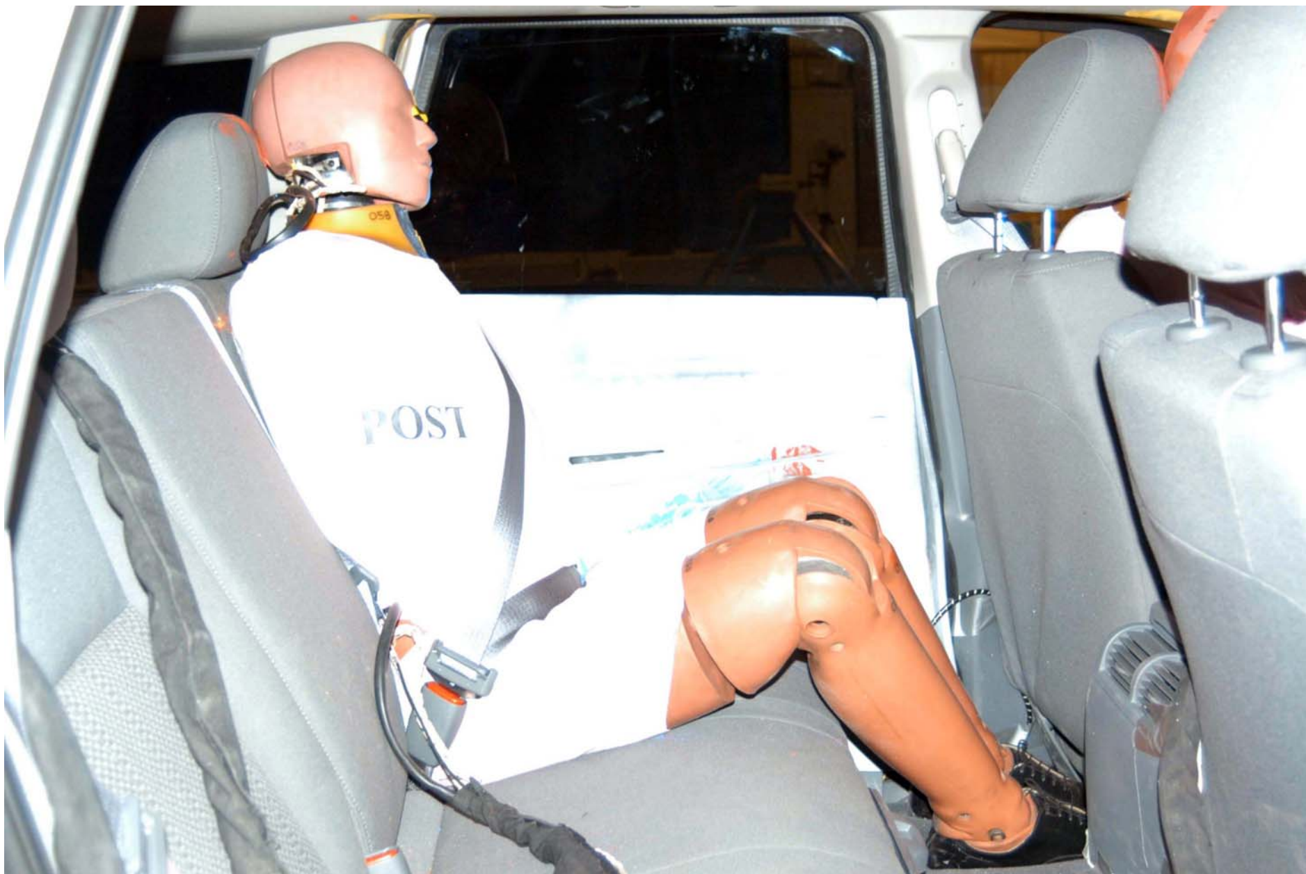
Figure A-22: POST-TEST RIGHT OCCUPANT COMPARTMENT VIEW OF REAR SID H3
