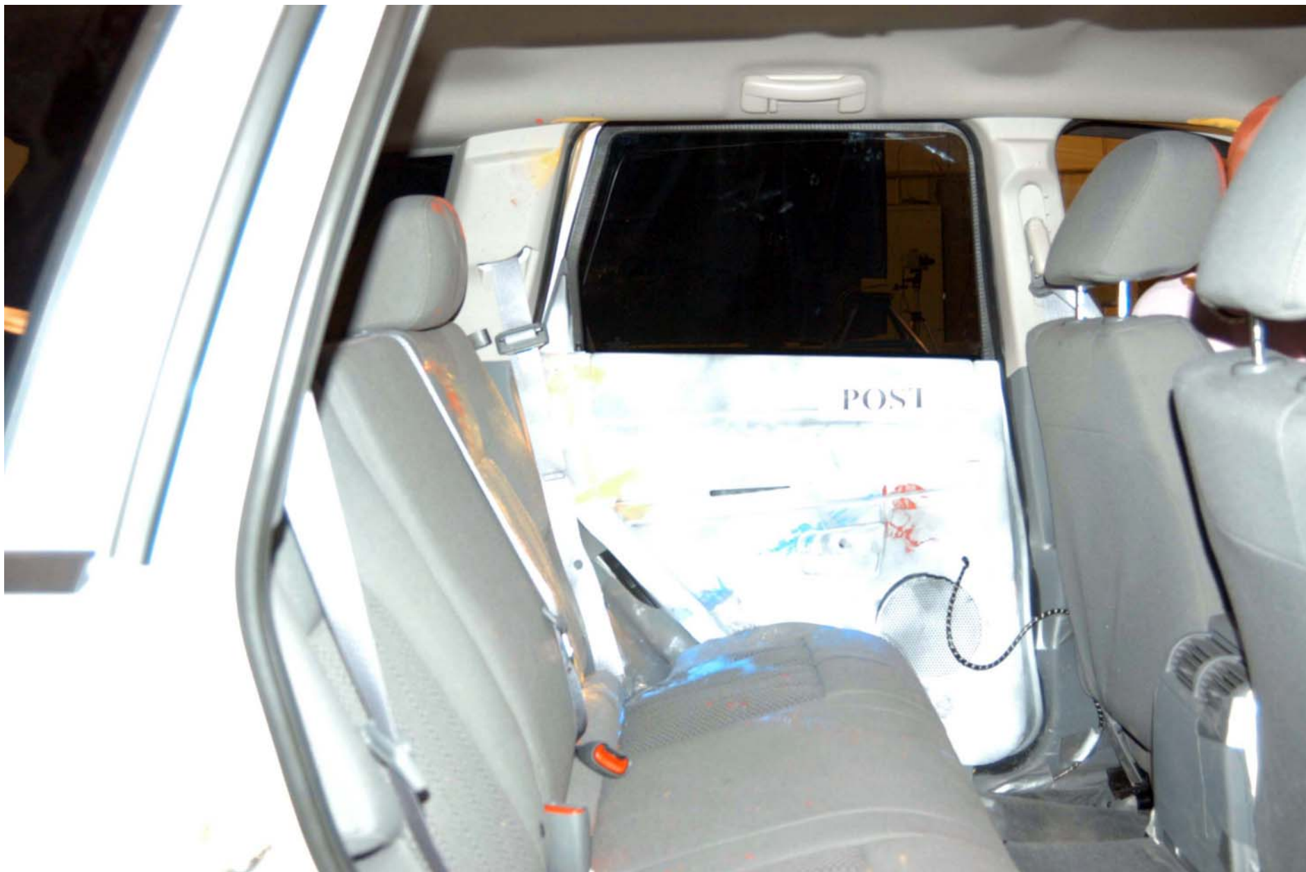
Figure A-31: POST-TEST INTERIOR OF REAR DOOR SHOWING SID H3 IMPACT LOCATIONS
