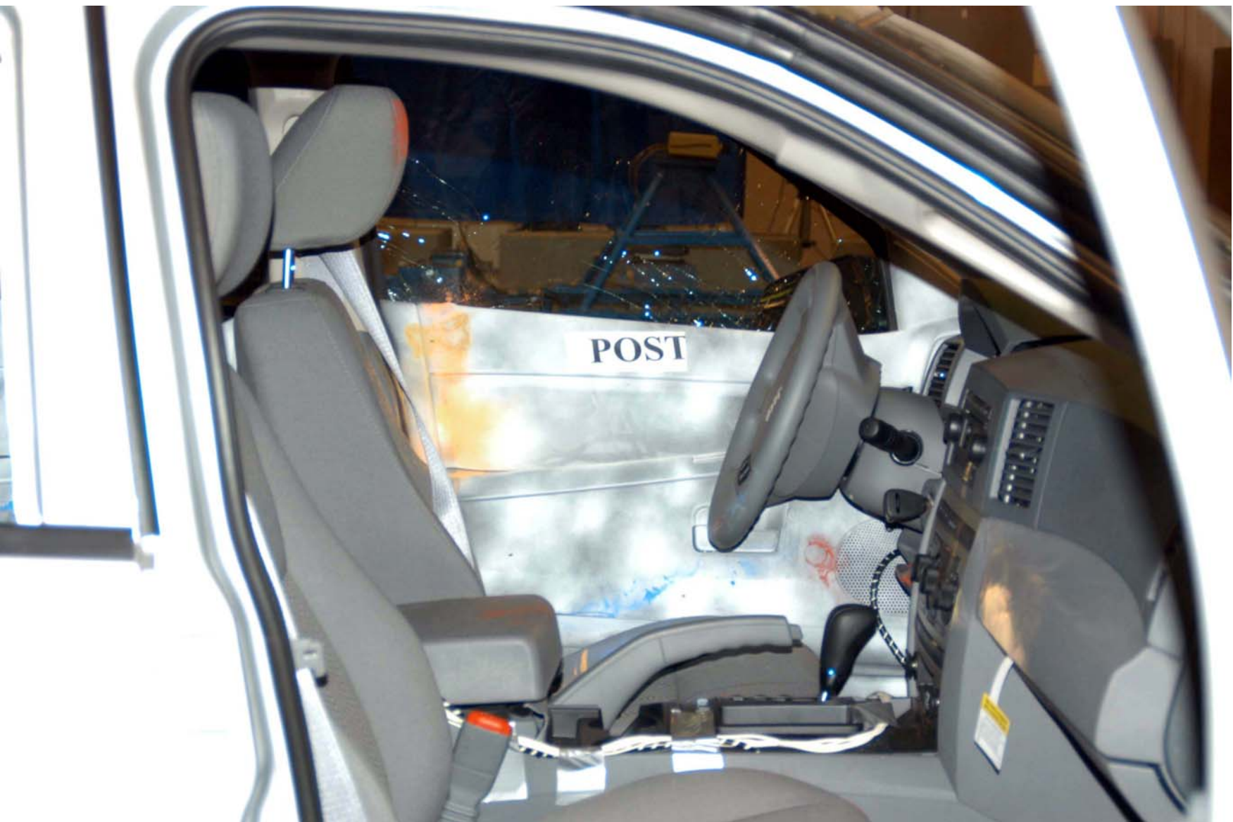
Figure A-28: POST-TEST INTERIOR OF FRONT DOOR SHOWING SID H3 IMPACT LOCATIONS
