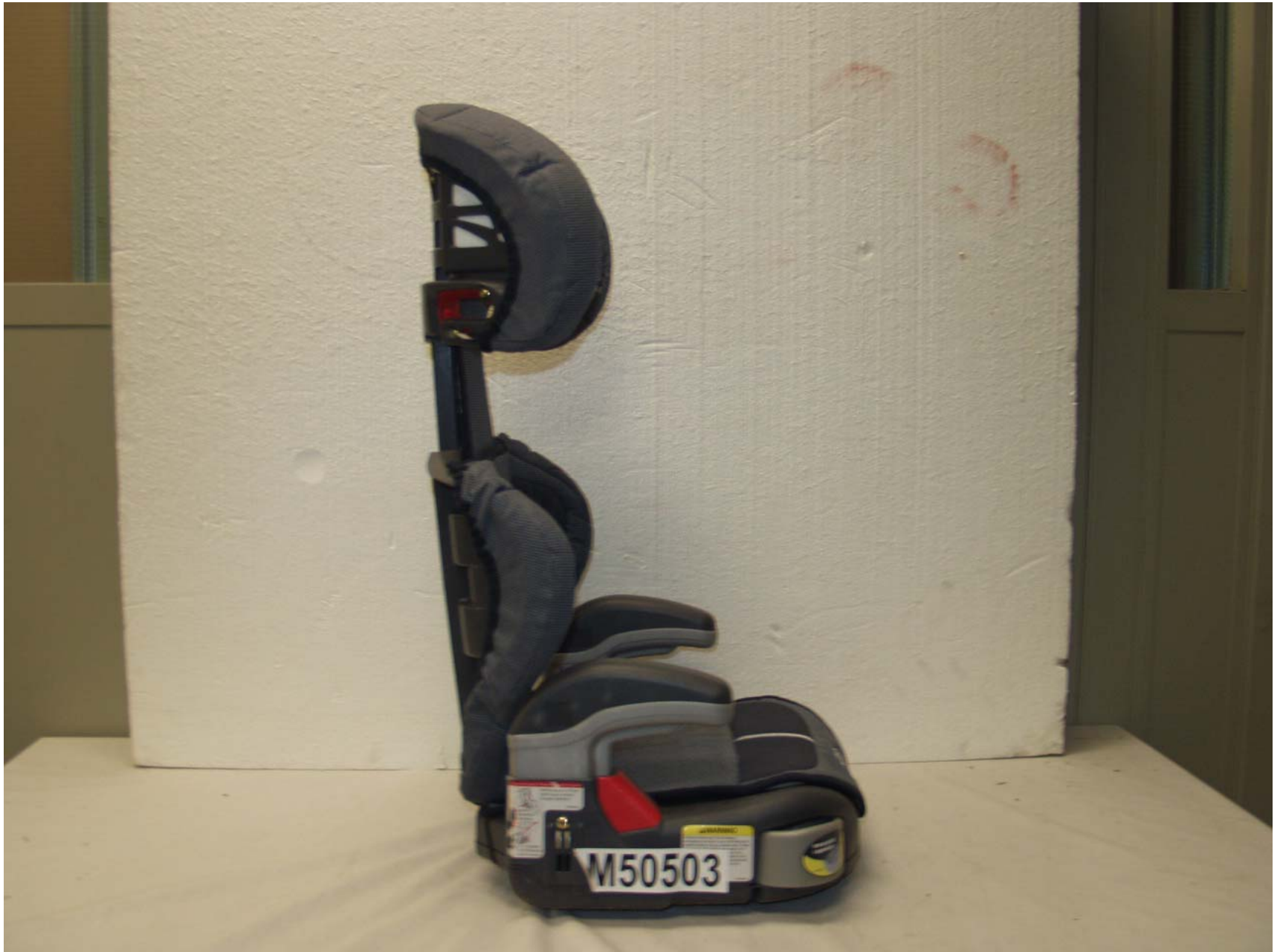
Figure 3-18 POST-TEST RIGHT SIDE VIEW OF POSITION 4 CRS
