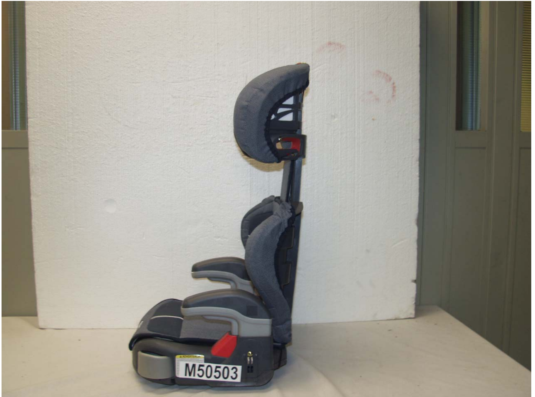
Figure 3-16 POST-TEST LEFT SIDE VIEW OF POSITION 4 CRS
