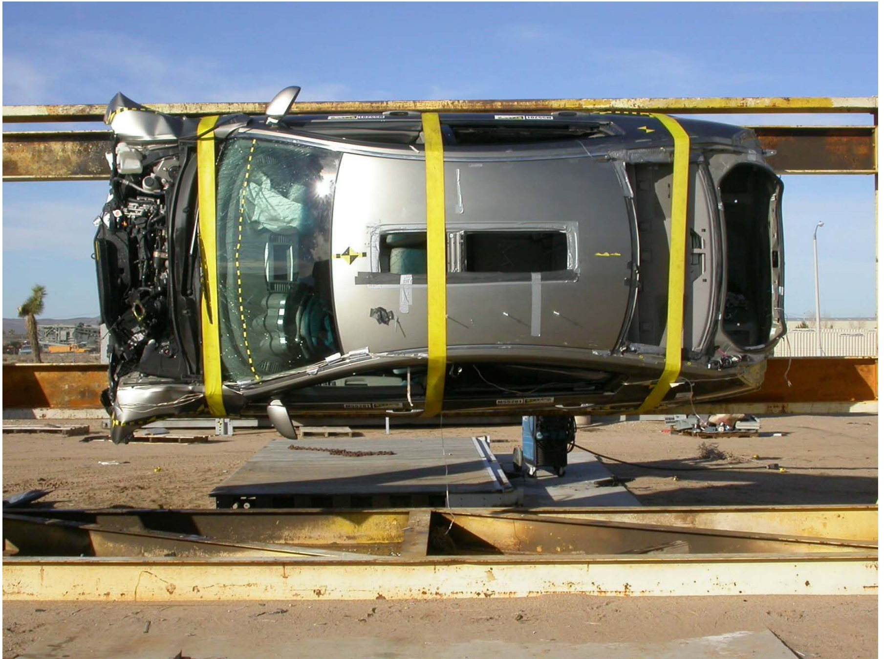
Figure A-59: Vehicle on Rollover Device (90°)
