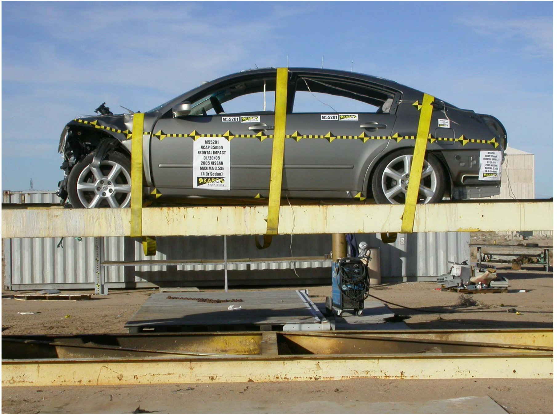
Figure A-58: Vehicle on Rollover Device (0°)
