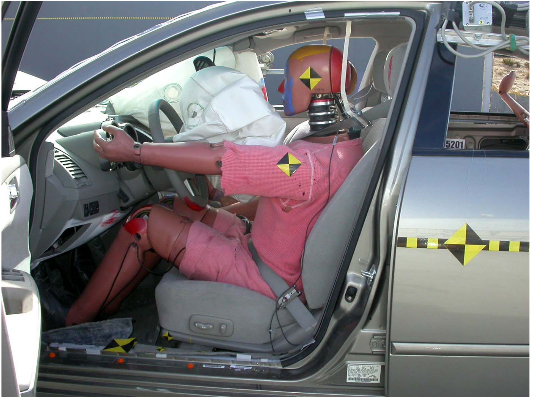
Figure A-35: Post-Test Driver Dummy (Door Open)
