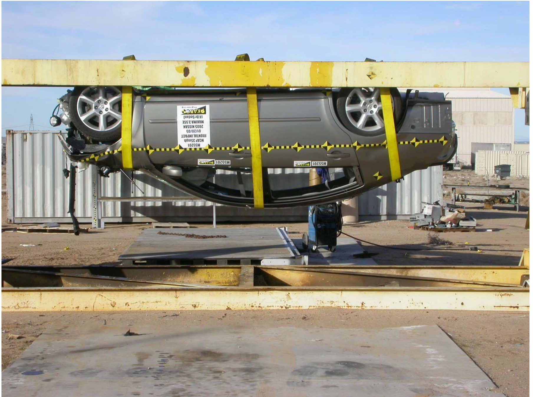
Figure A-60: Vehicle on Rollover Device (180°)
