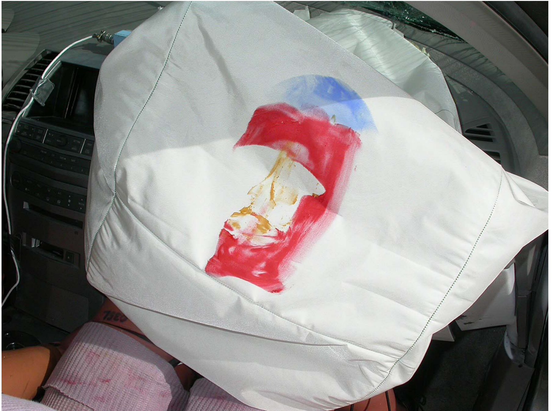
Figure A-57: Post-Test Passenger Dummy Airbag Contact
