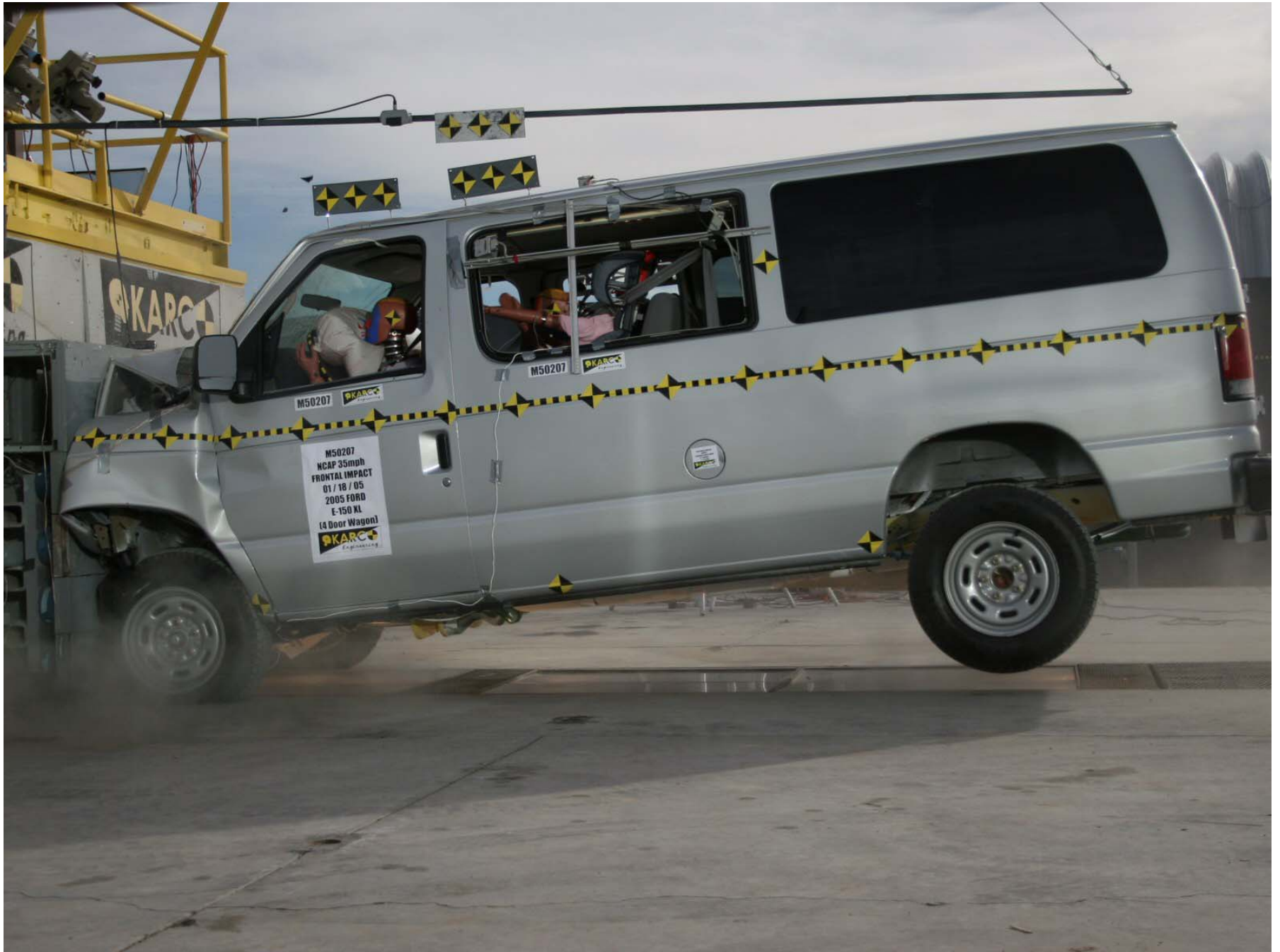
Figure A-62: Vehicle Impact
