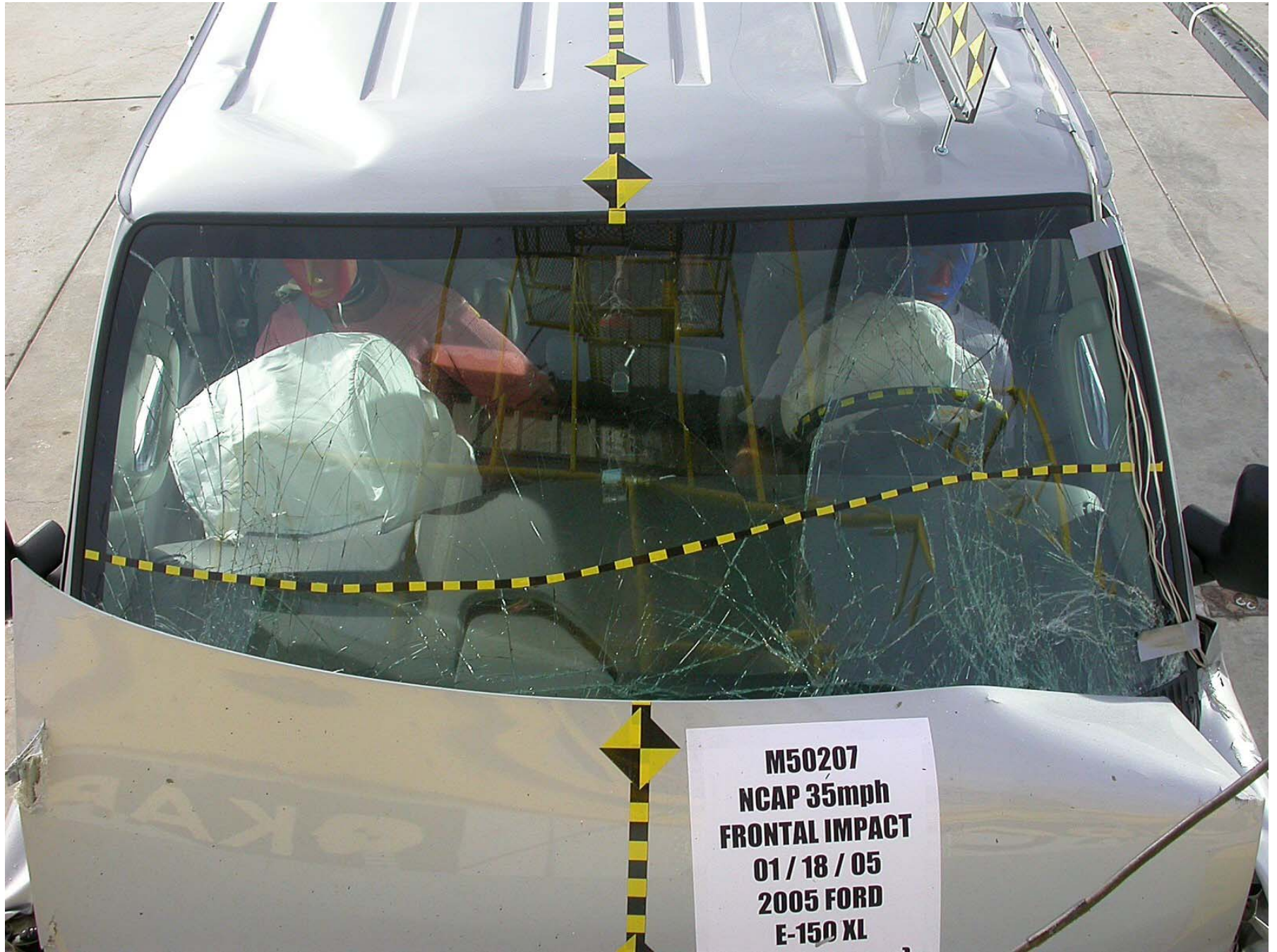
Figure A-19: Post-Test Windshield
