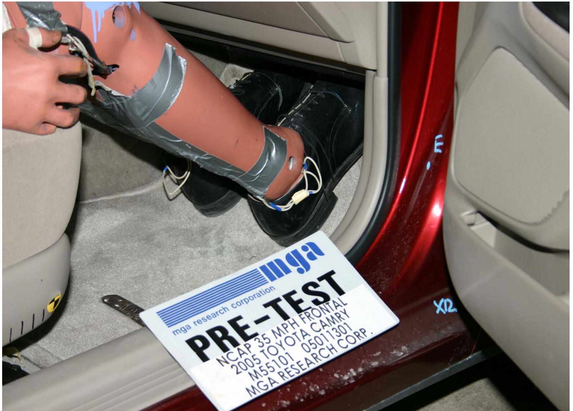
Pre-Test Passenger Dummy Feet Position
