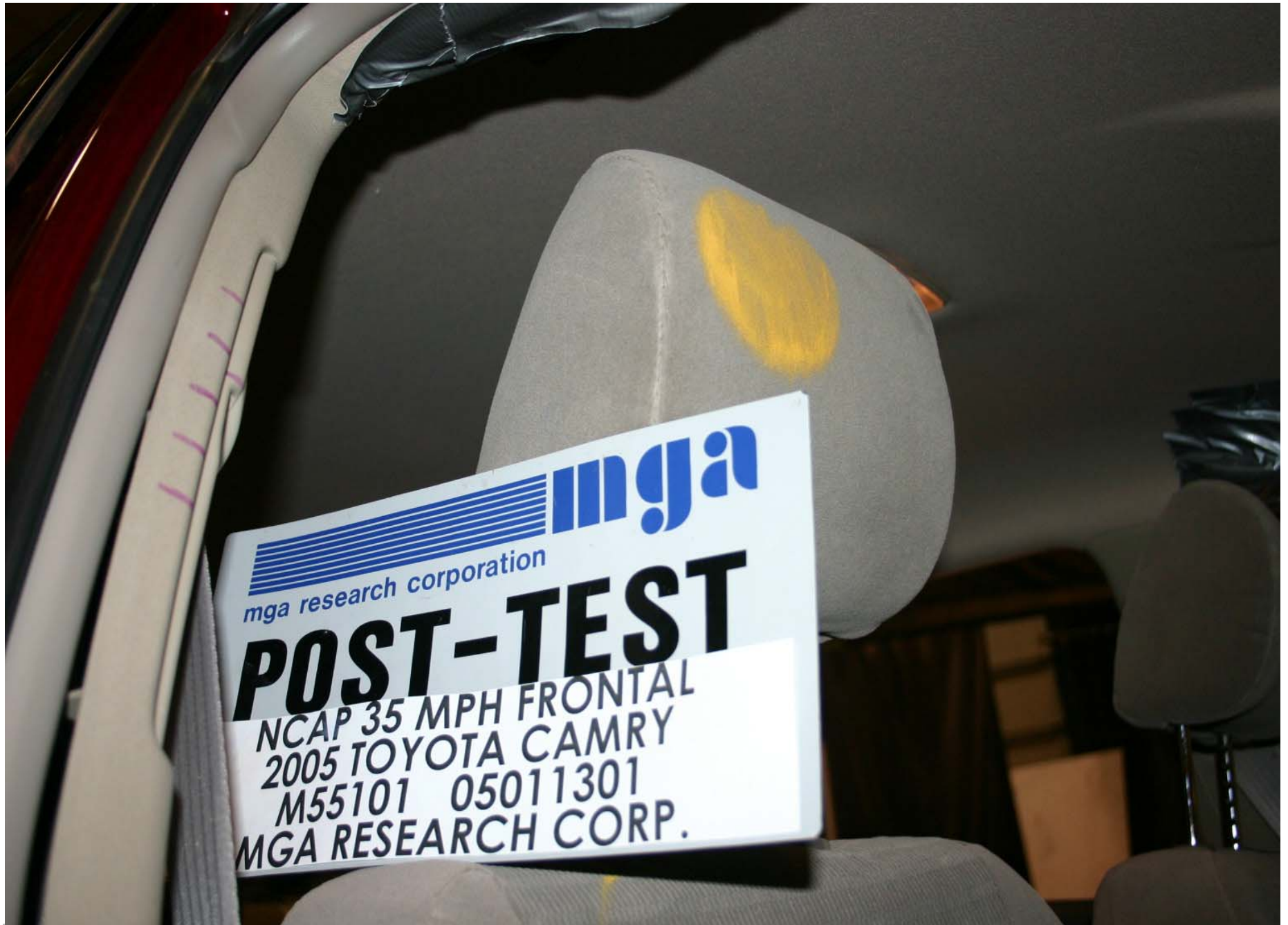
Post-Test Passenger Dummy Head Contact
