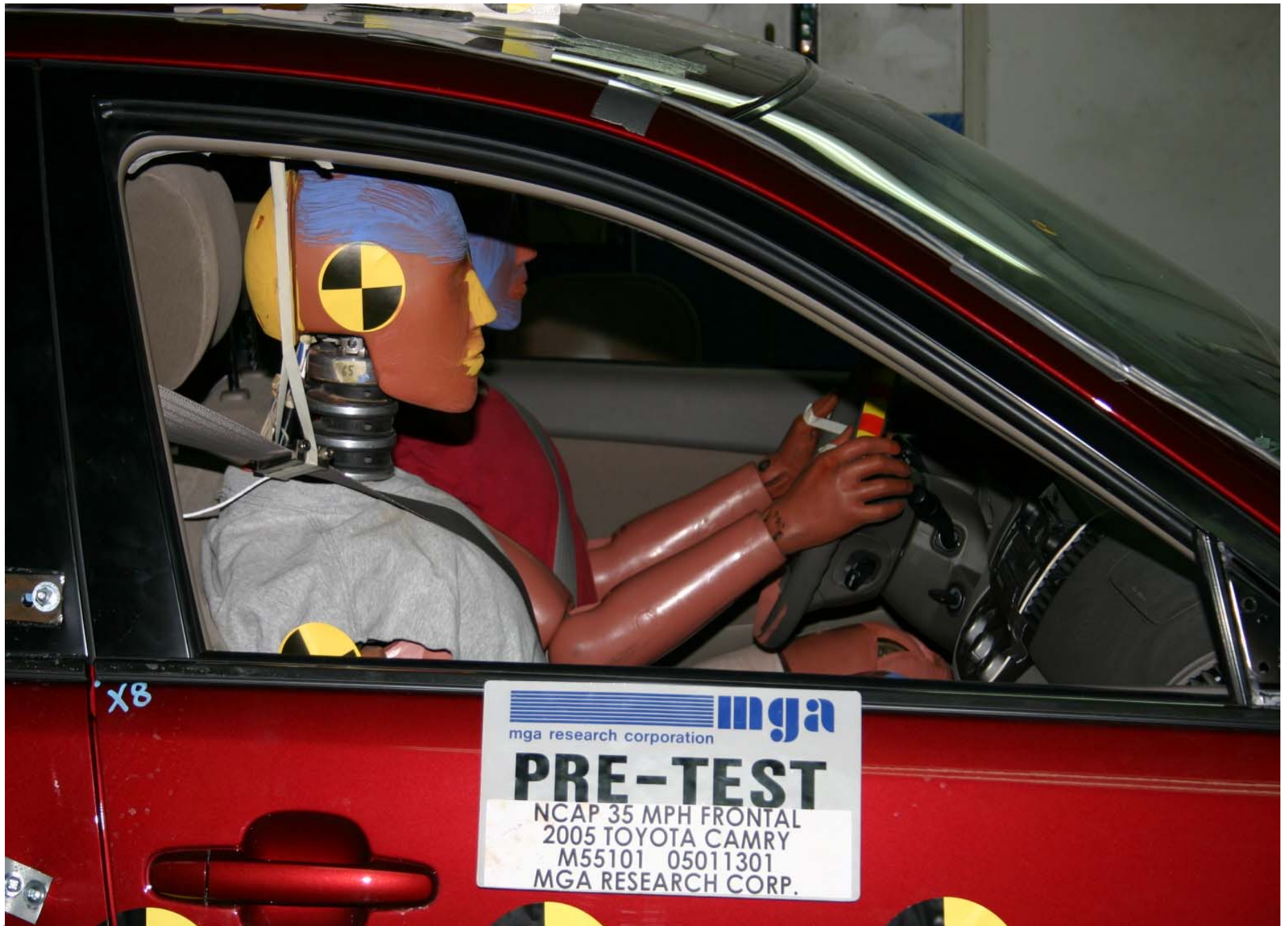
Pre-Test Passenger Dummy Position Right Side View
