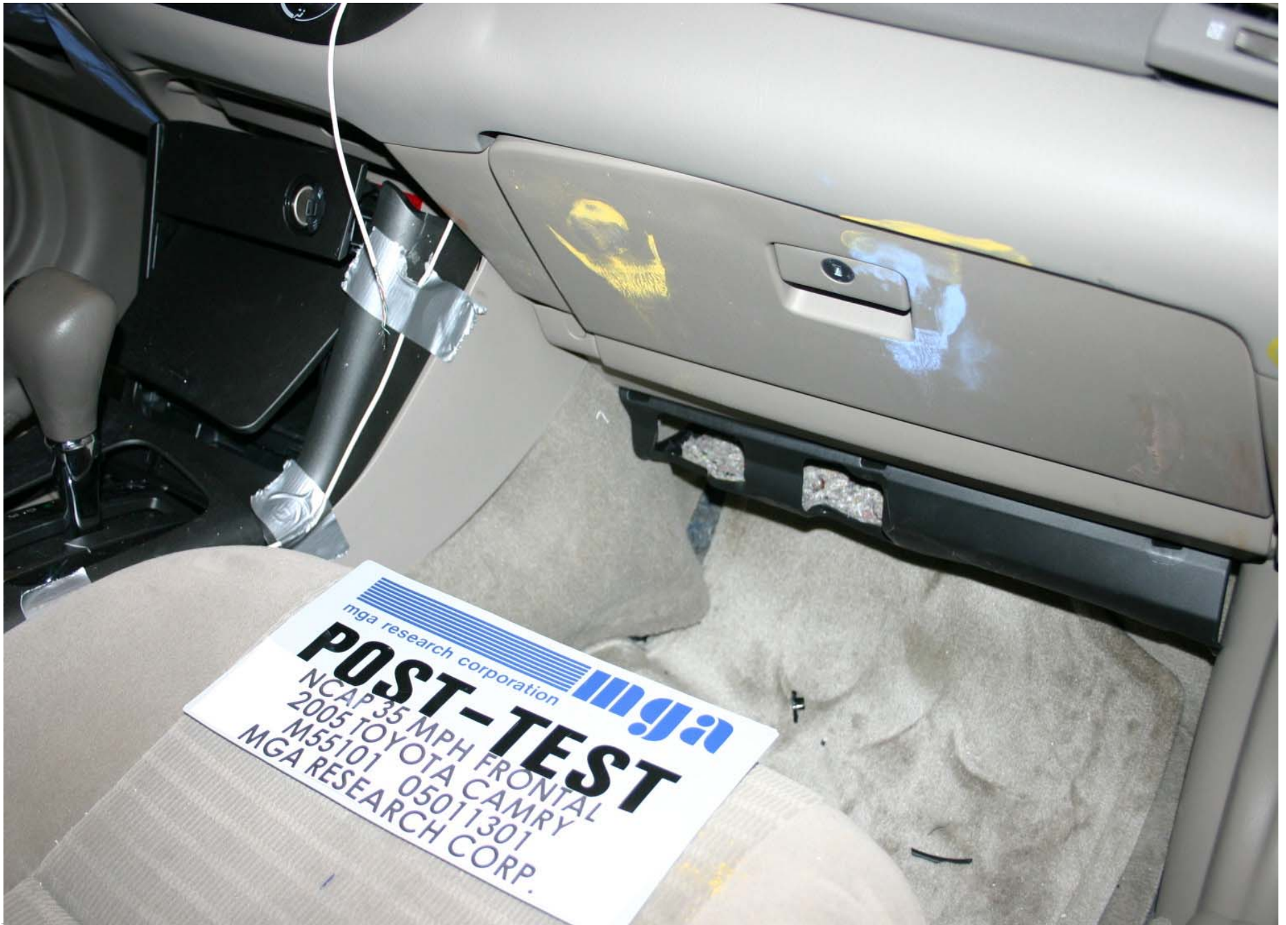
Post-Test Passenger Dummy Knee Contact
