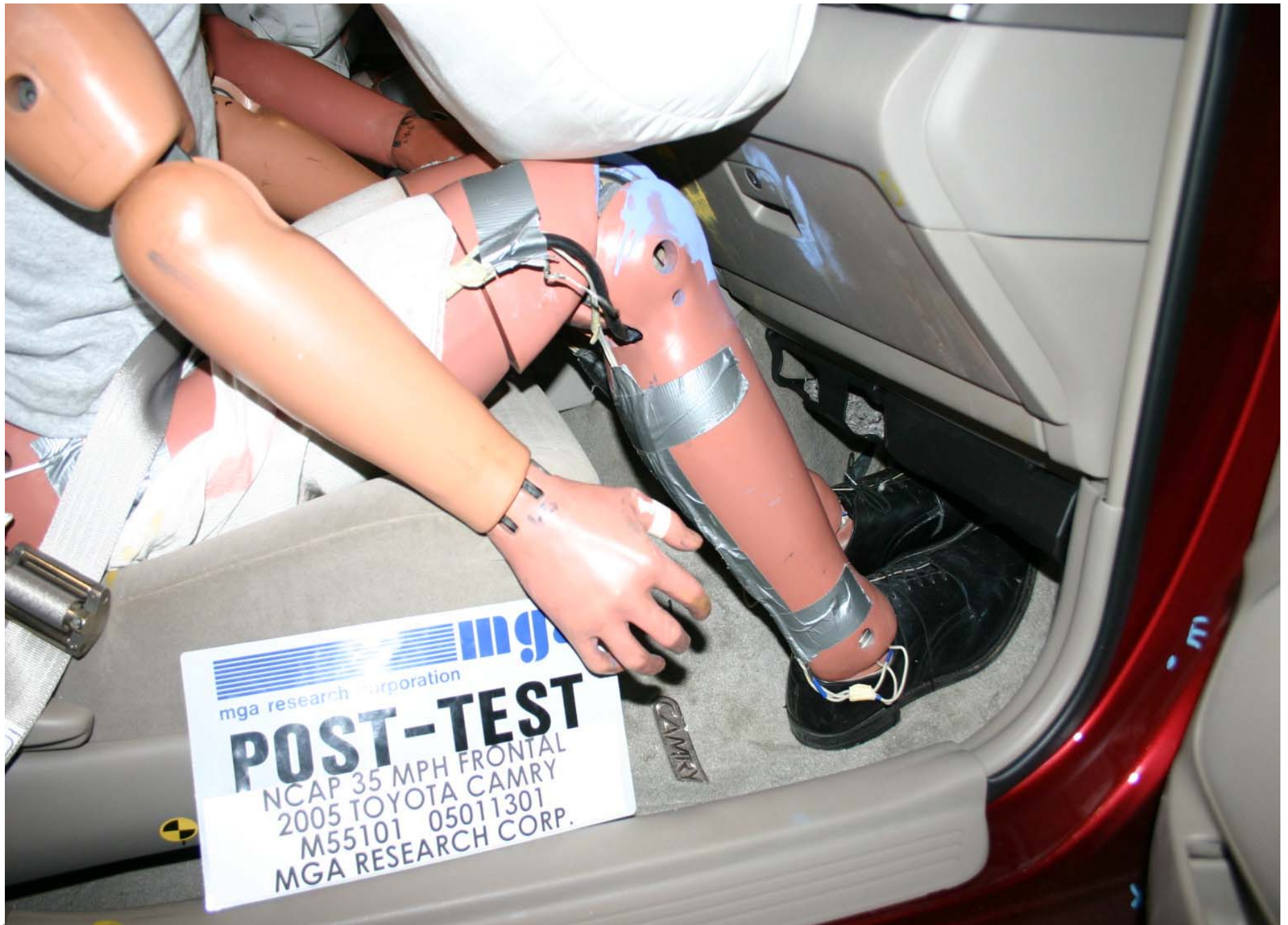
Post-Test Passenger Side Knee Bolster View
