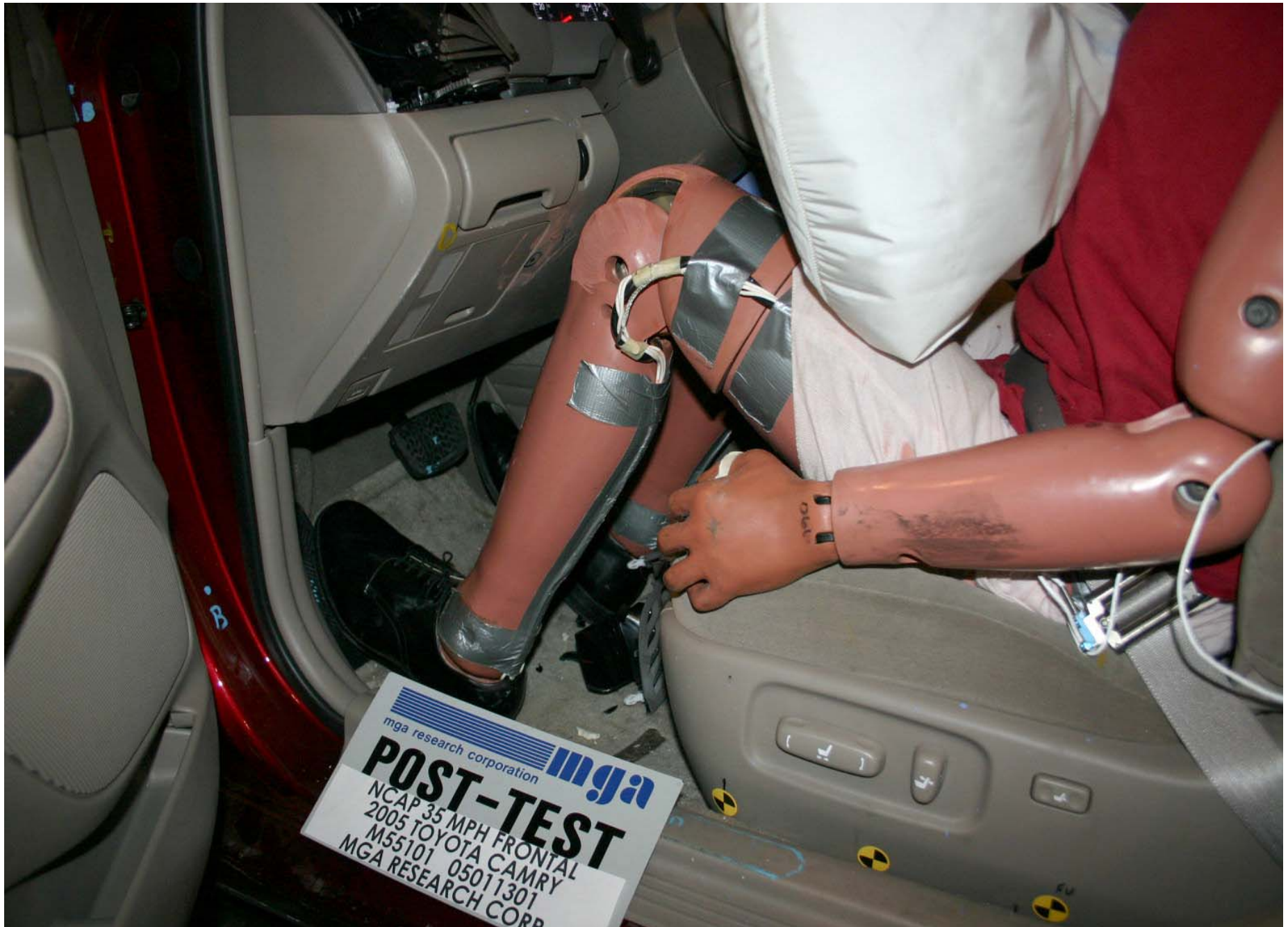
Post-Test Driver Side Knee Bolster View
