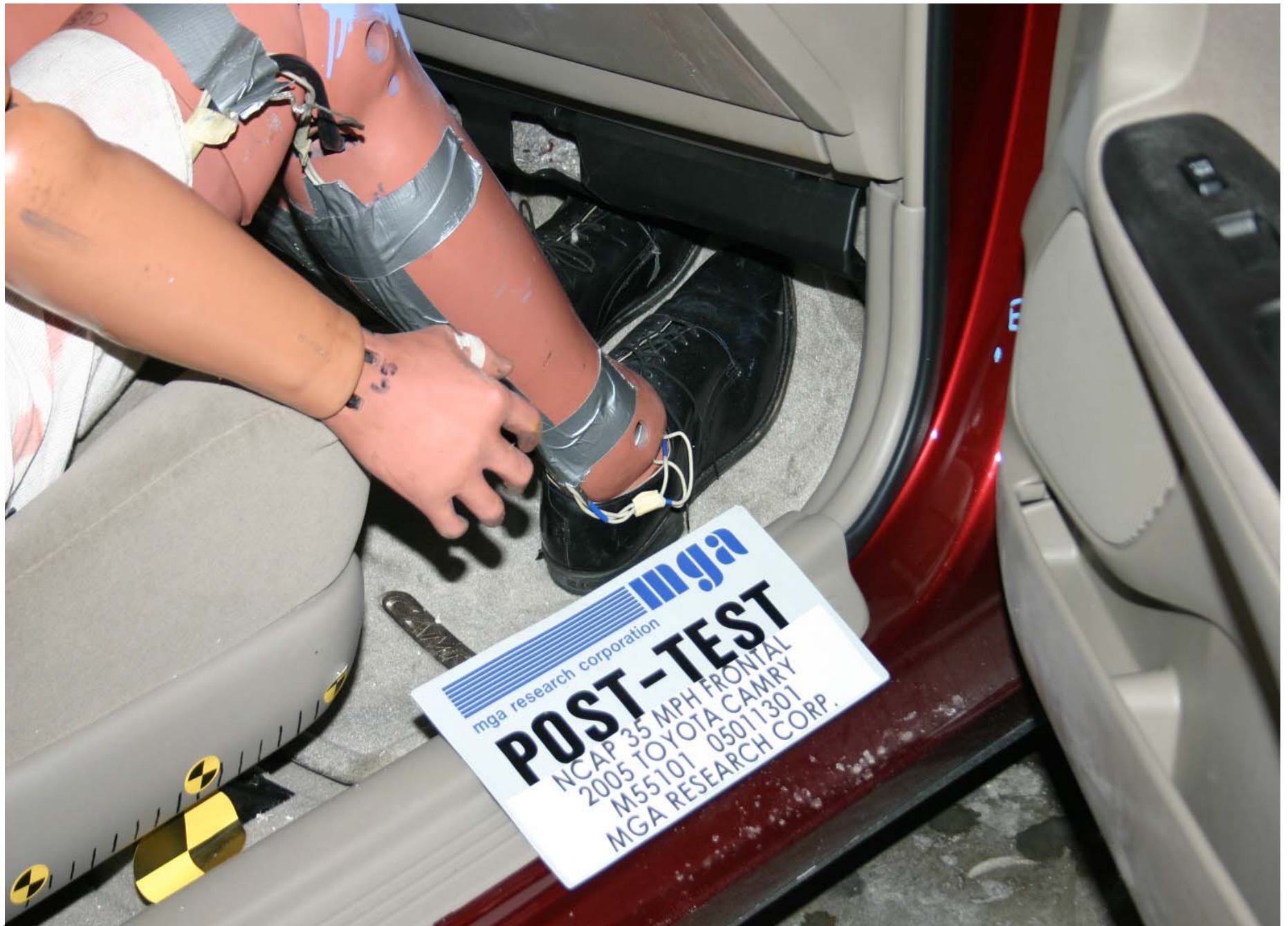
Post-Test Passenger Dummy Feet Position
