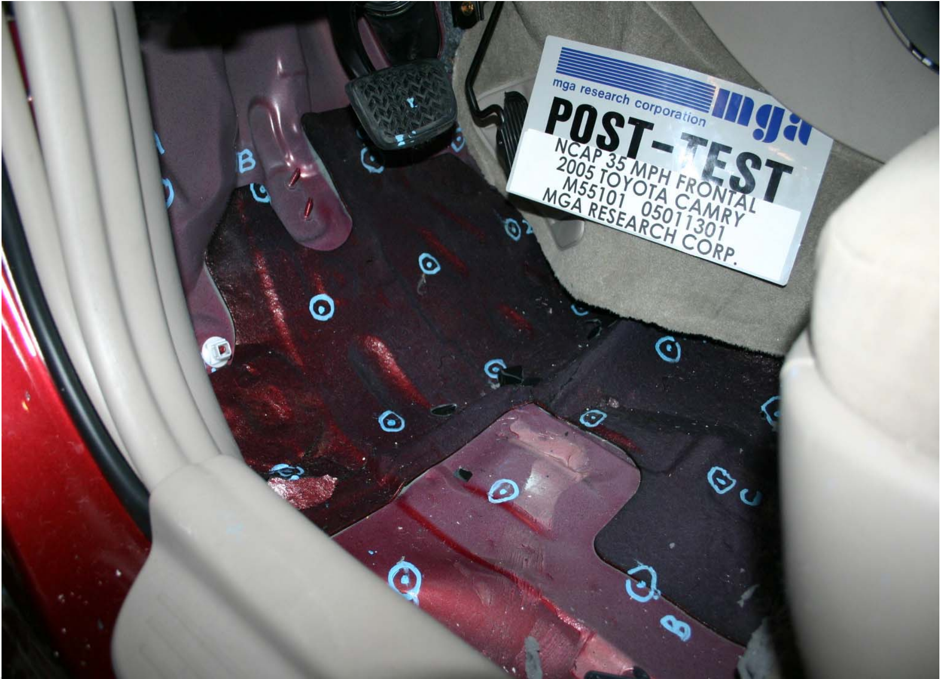
Post-Test Driver Side Floor Pan View
