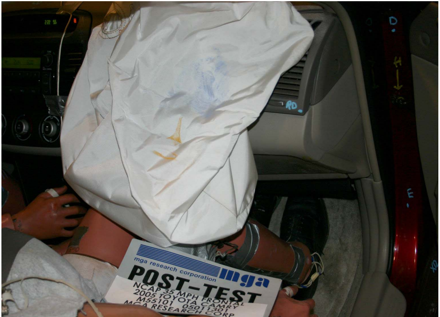
Post-Test Passenger Dummy Airbag Contact
