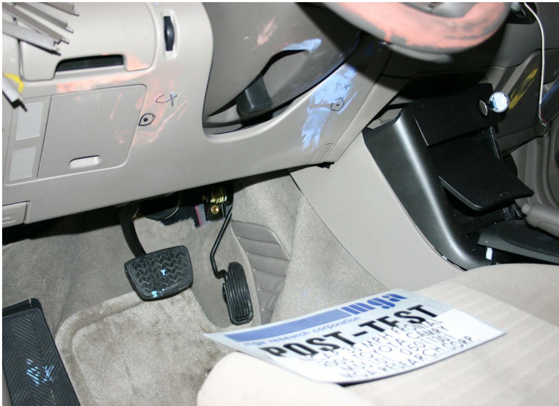
Post-Test Driver Dummy Knee Contact
