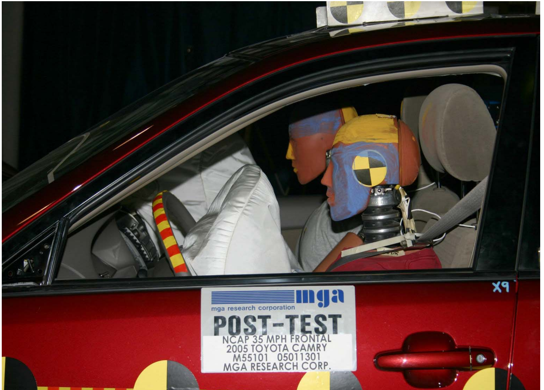
Post-Test Driver Dummy Position Left Side View
