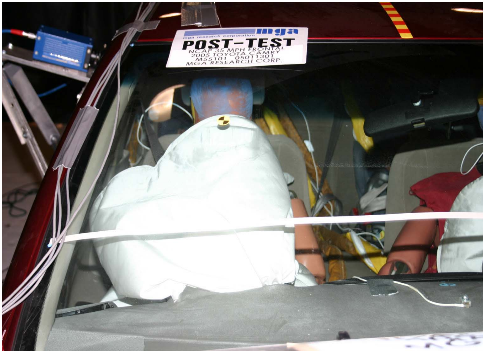
Post-Test Passenger Dummy Front View (head position)
