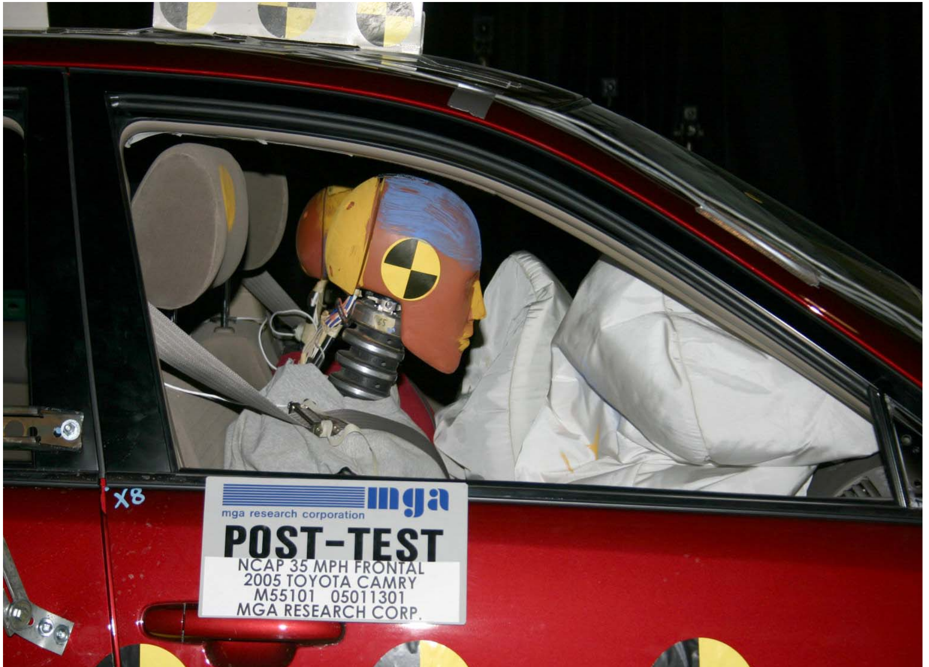
Post-Test Passenger Dummy Position Right Side View
