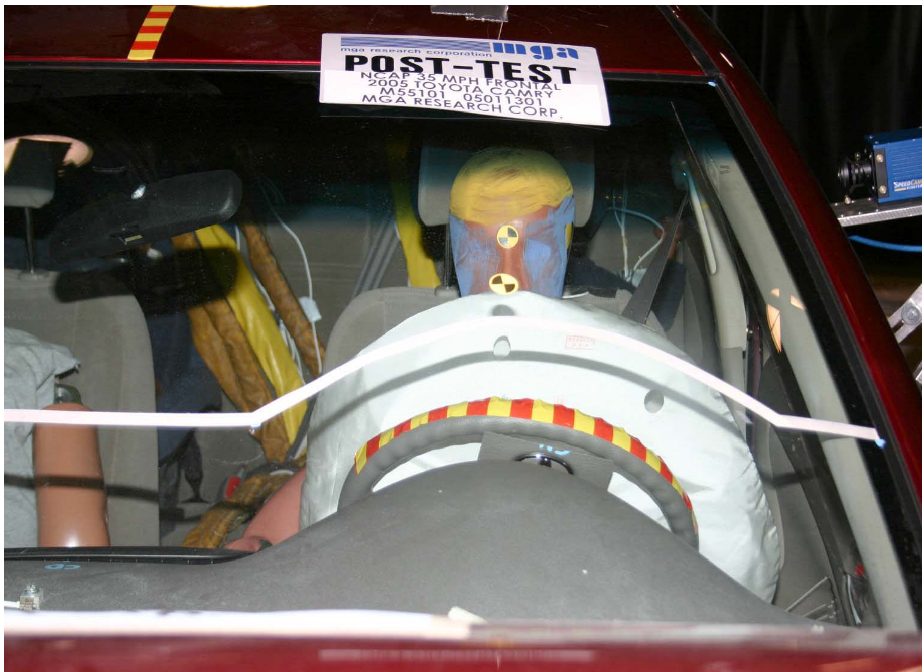
Post-Test Driver Dummy Front View (head position)
