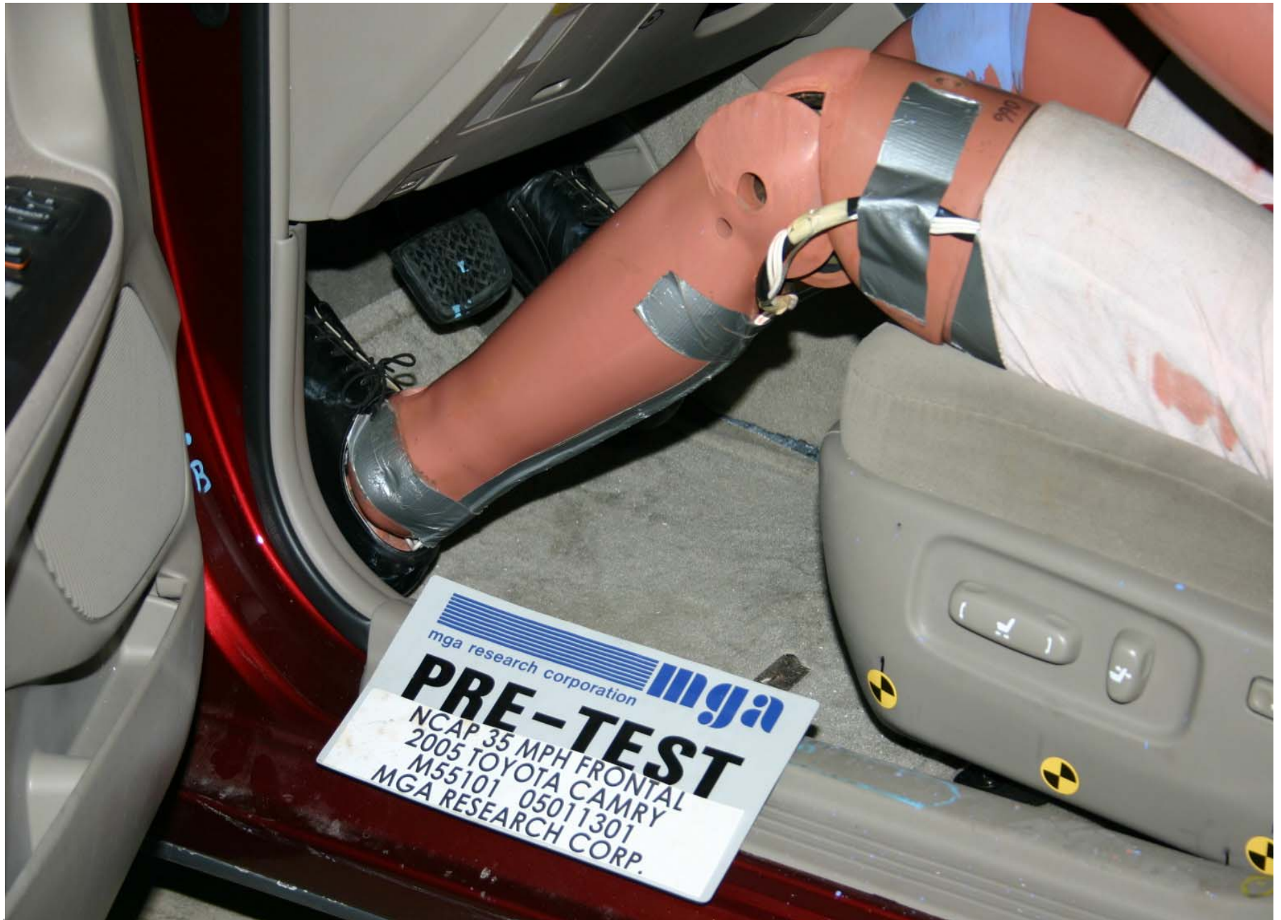
Pre-Test Driver Dummy Feet Position
