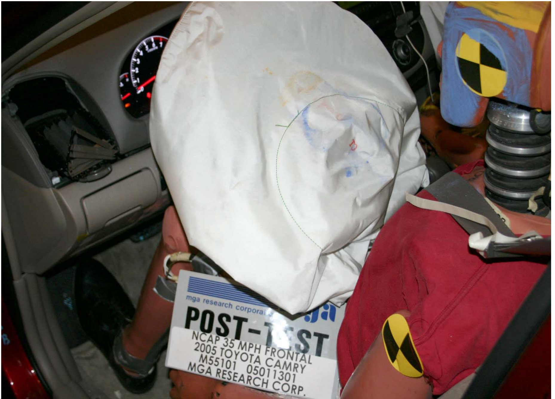
Post-Test Driver Dummy Airbag Contact
