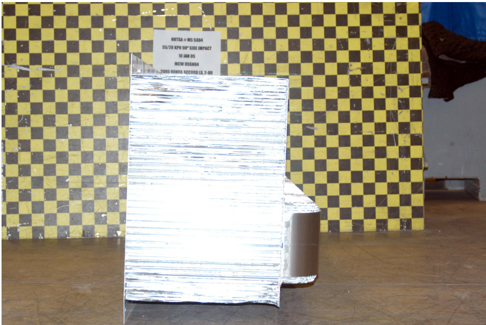
Figure A-51: PRE-TEST ALUMINUM BARRIER RIGHT SIDE
