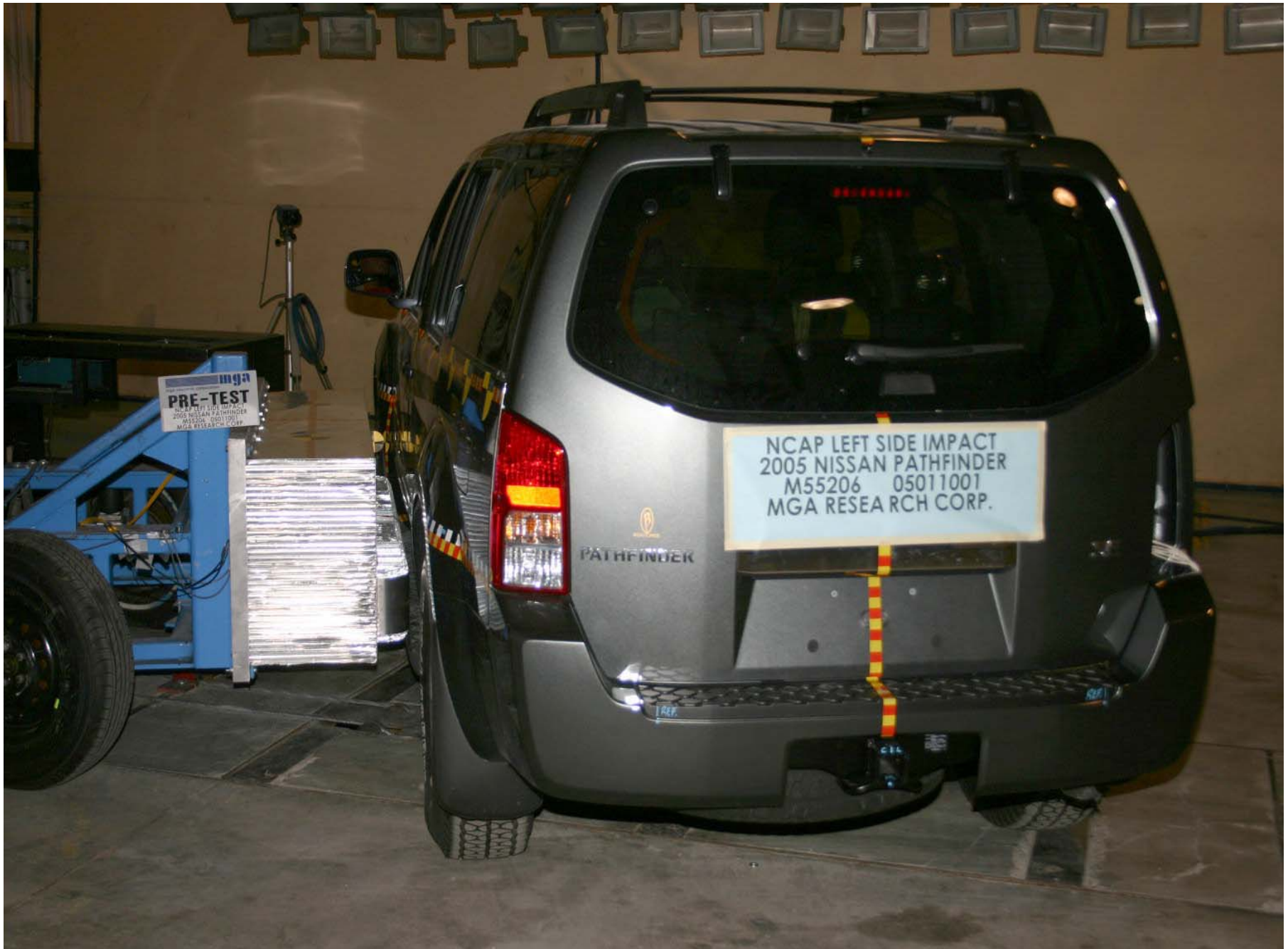
Pre-Test MDB (Right Side) Positioned Against Vehicle
