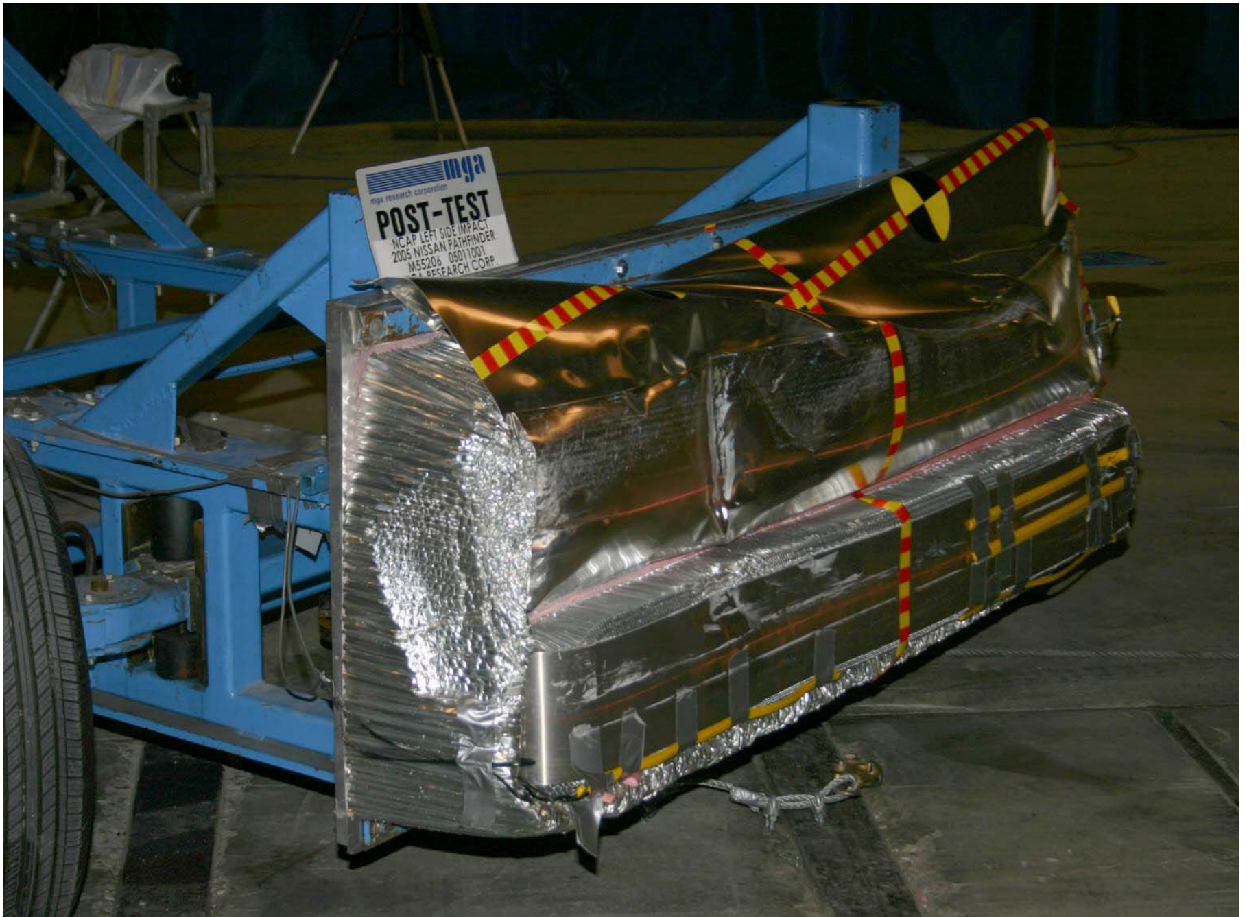
Post-Test MDB Right Side View
