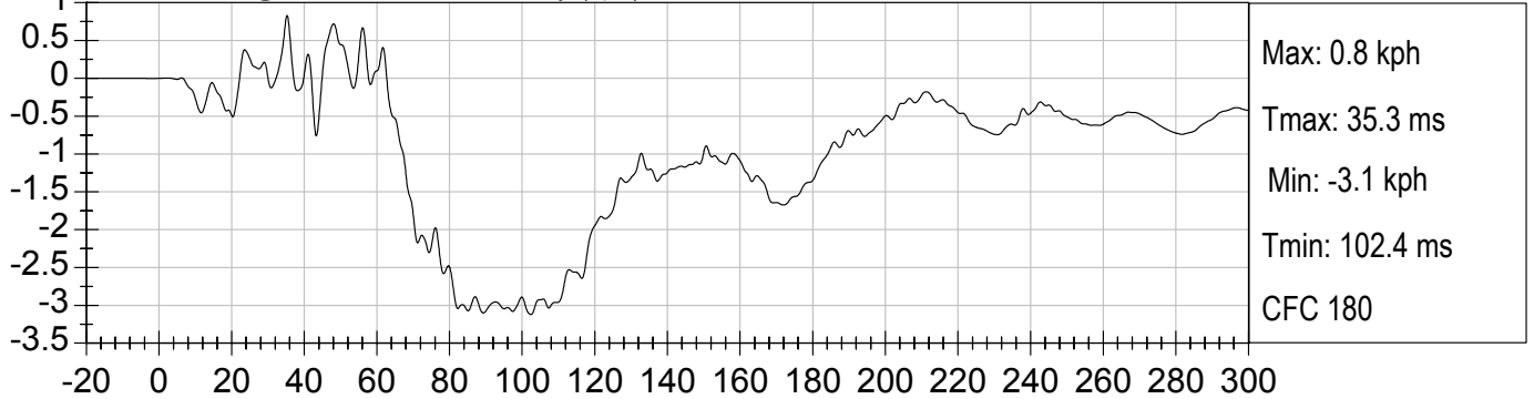
1 FLOORPAN @ REAR AXLE Z Velocity (kph) vs TIME (ms)
