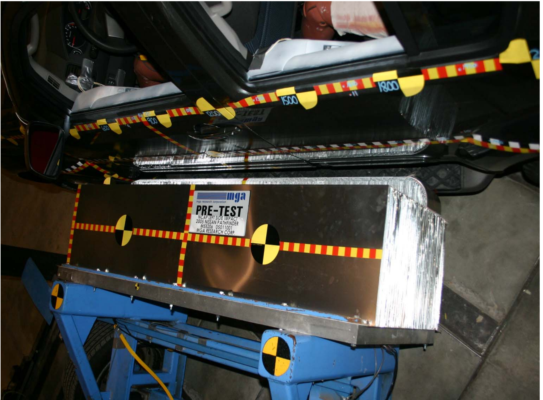
Pre-Test MDB Positioned Against Vehicle Overhead View
