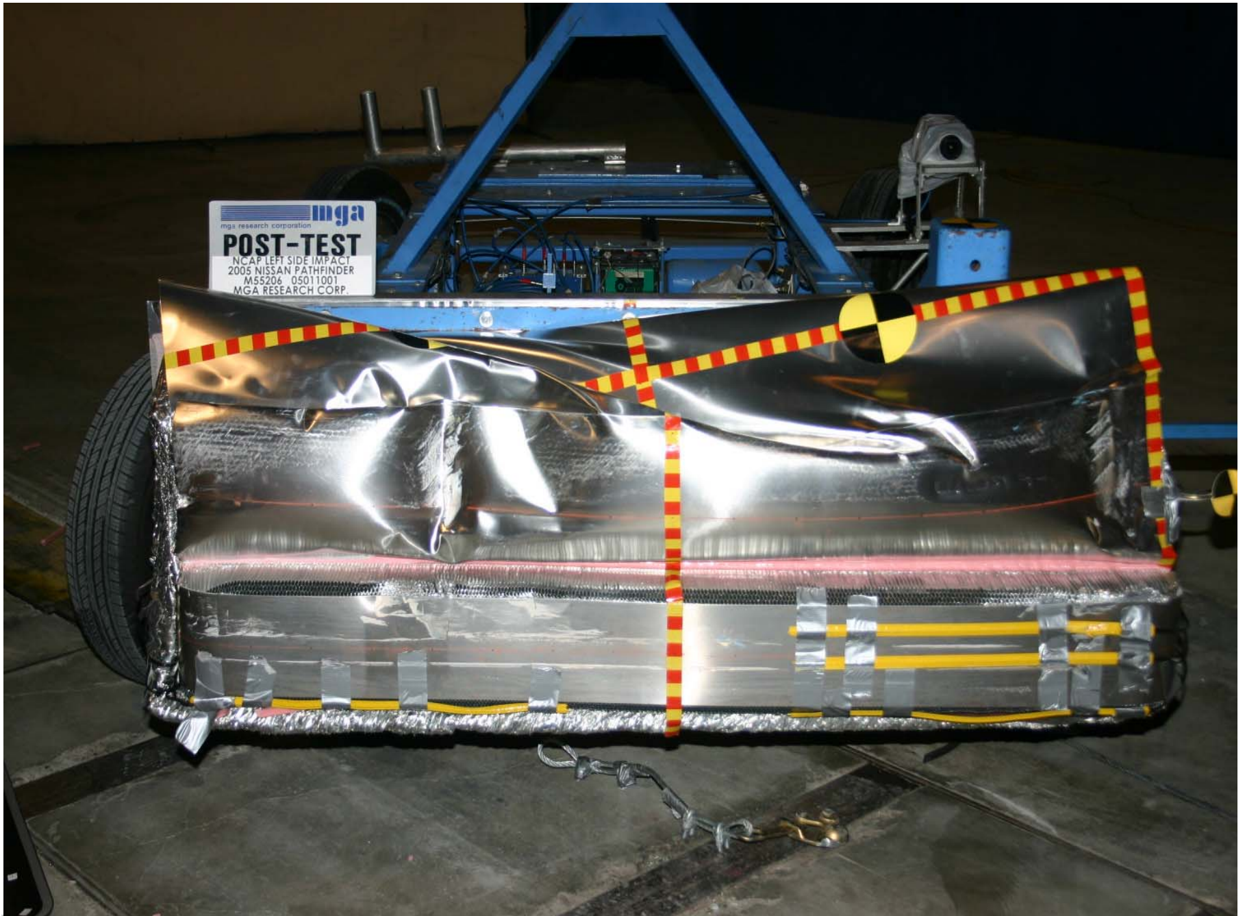
Post-Test MDB Front View
