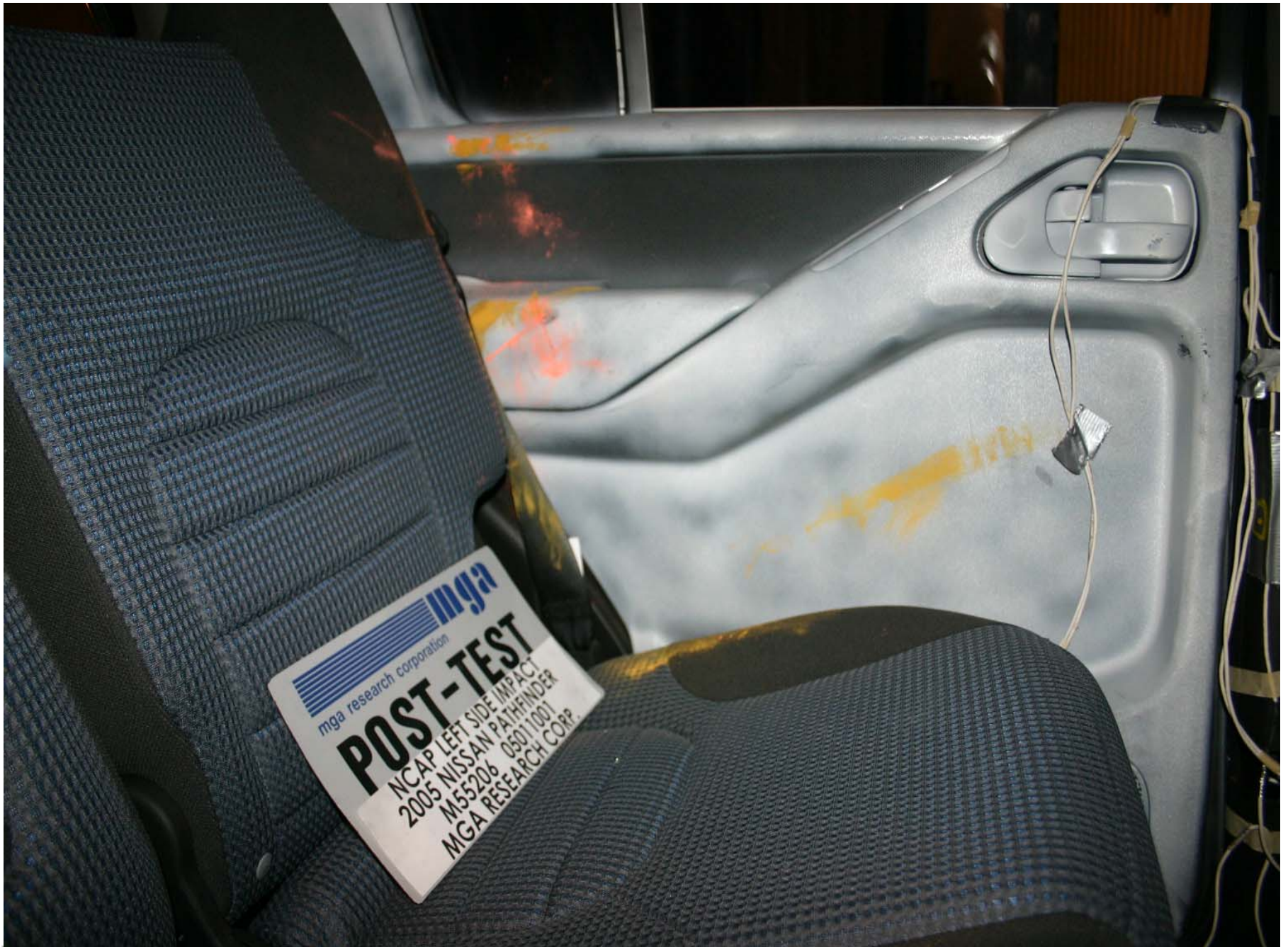
Post-Test Passenger Dummy Mid Contact
