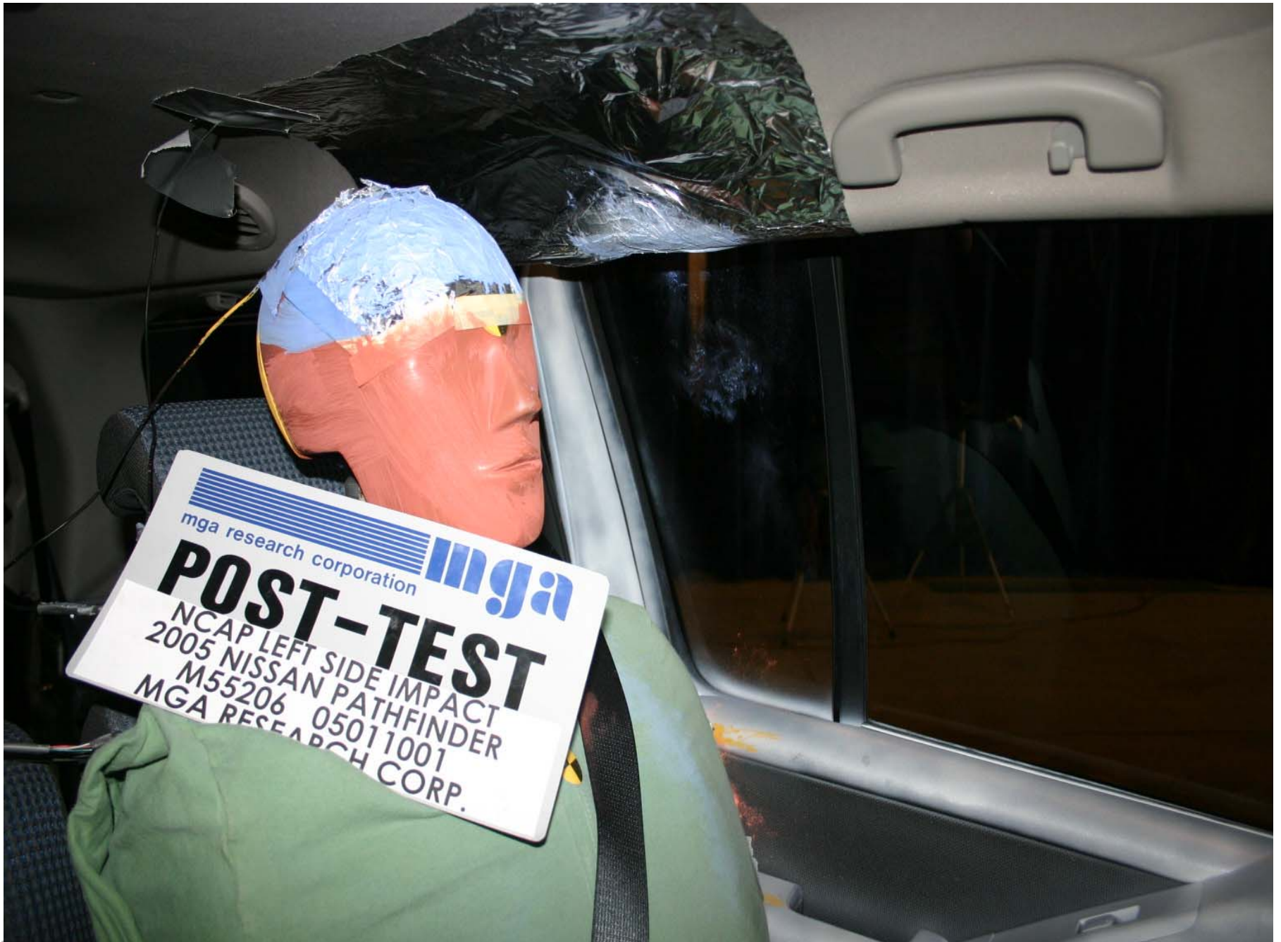
Post-Test Passenger Dummy Head Contact (side header)
