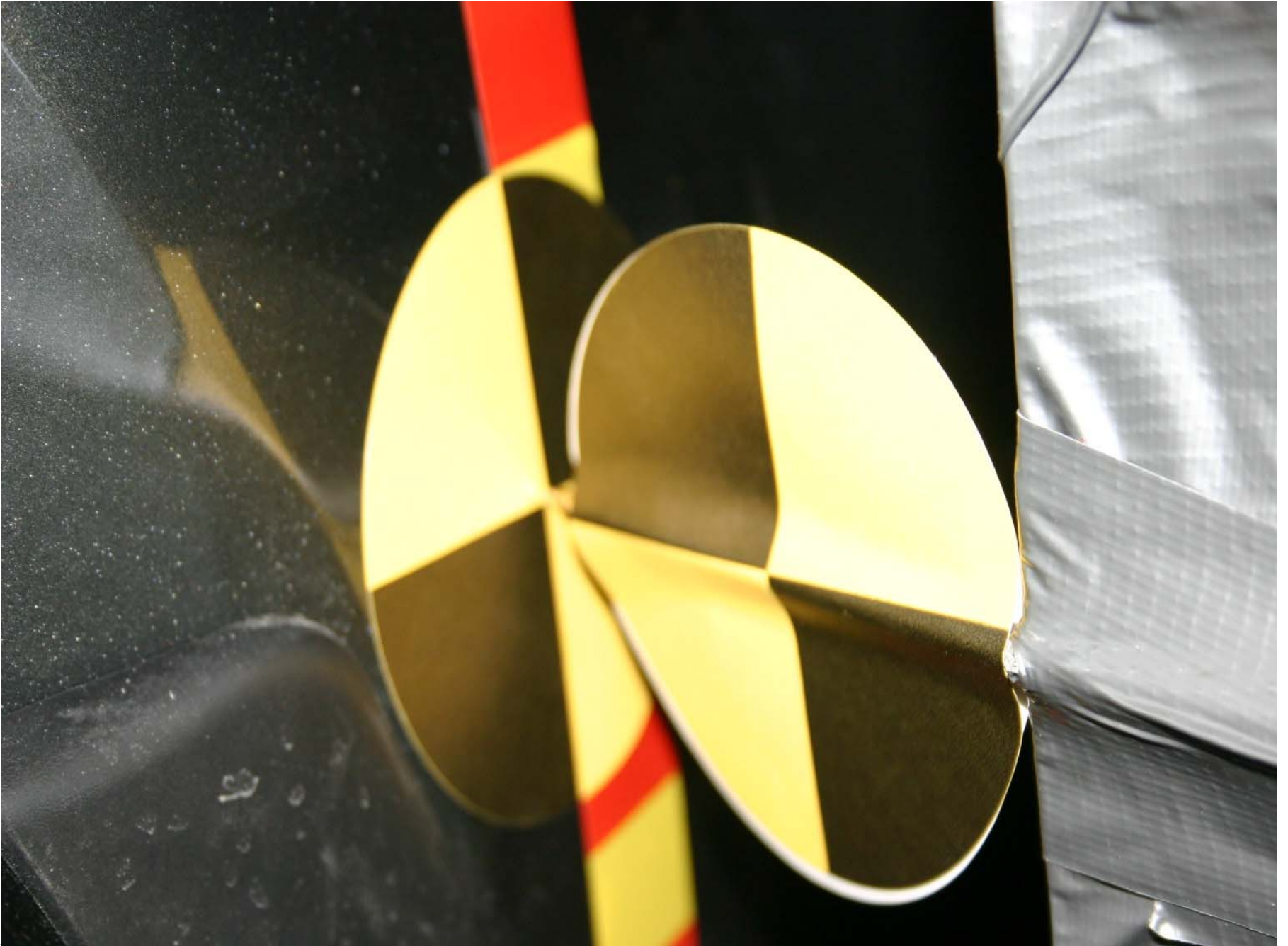
Pre-Test Impact Point on Vehicle
