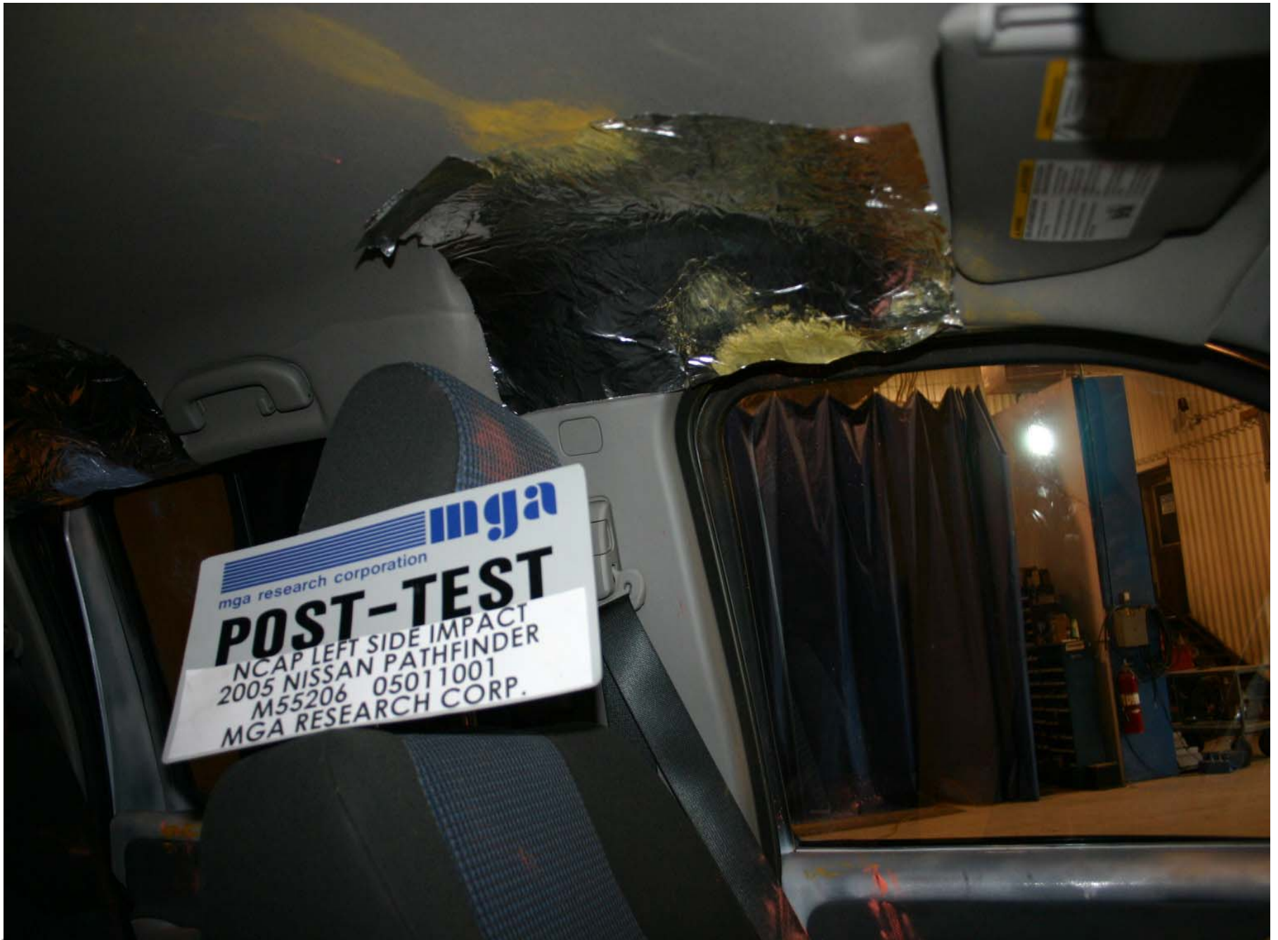
Post-Test Driver Dummy Head Contact (side header)
