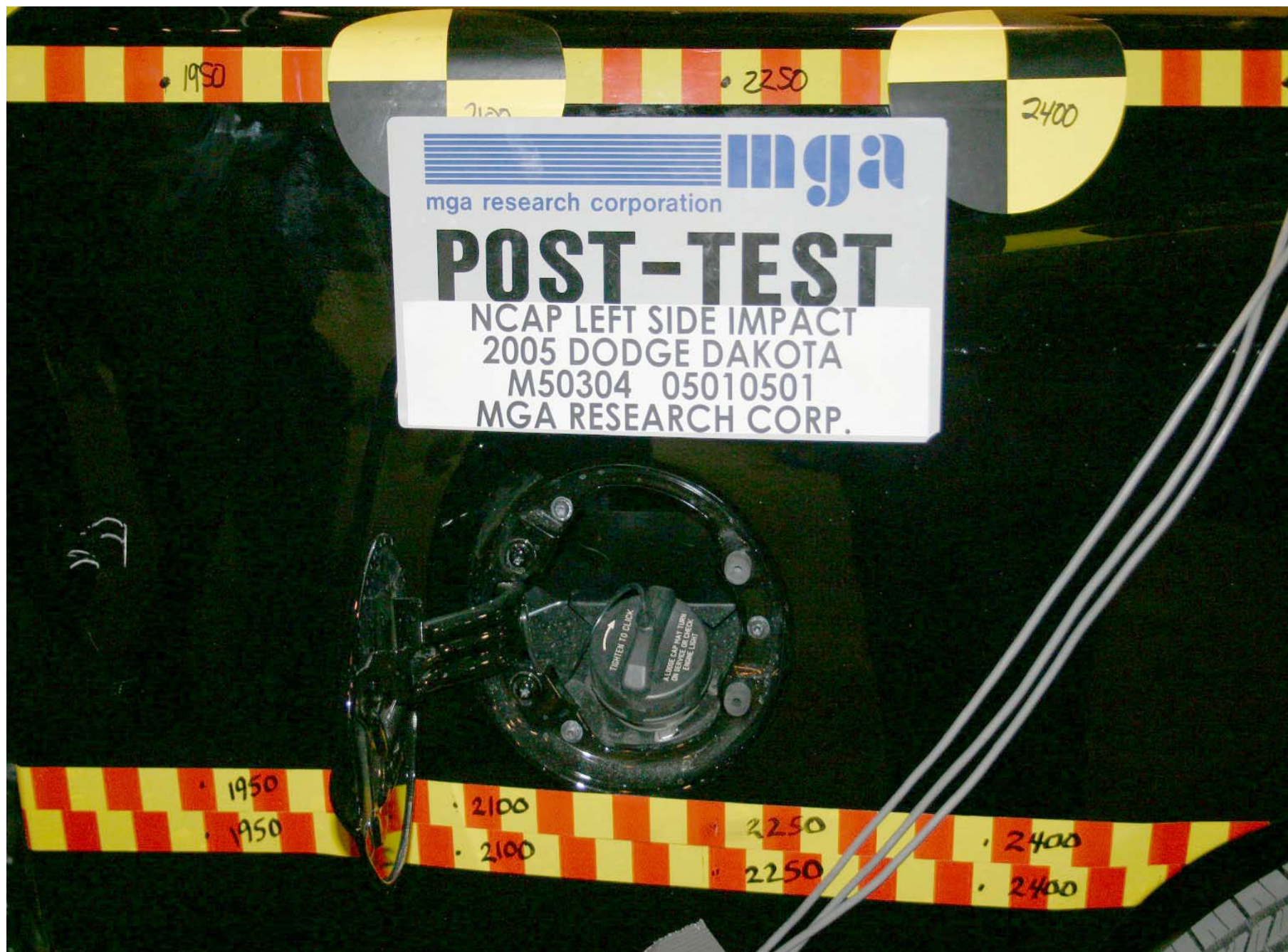
Post-Test Fuel Filler Cap View
