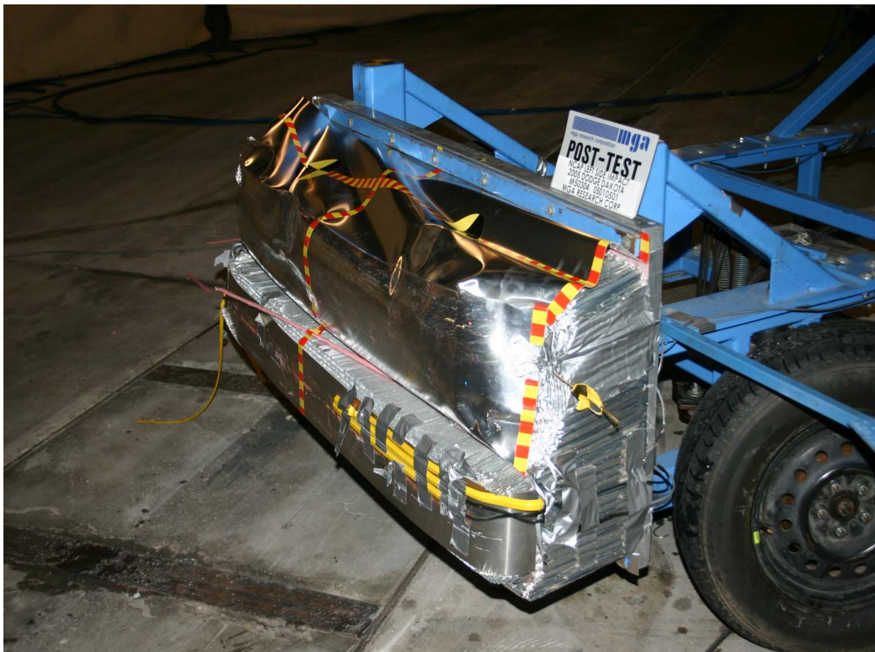
Post-Test MDB Left Side View
