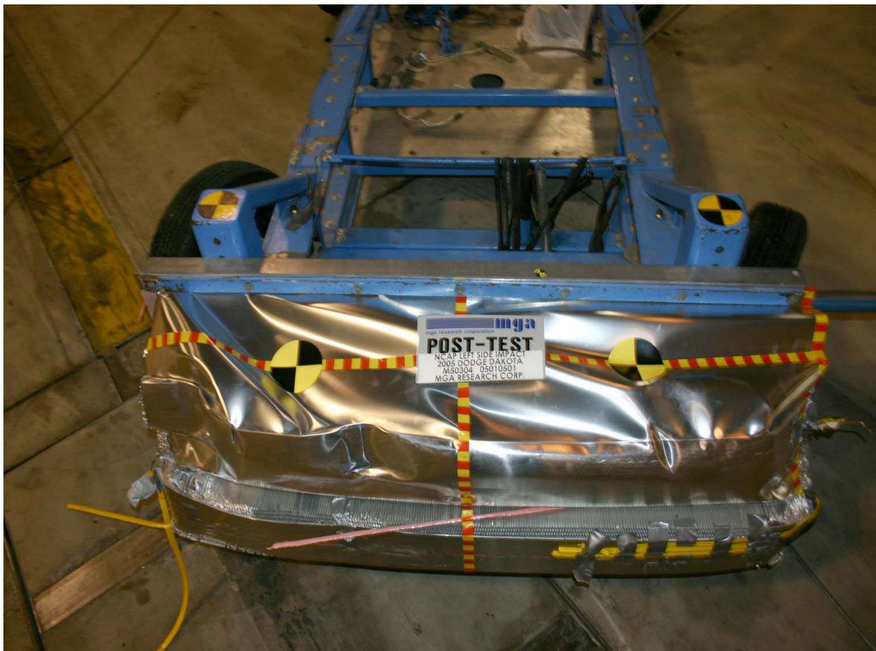
Post-Test MDB Top View
