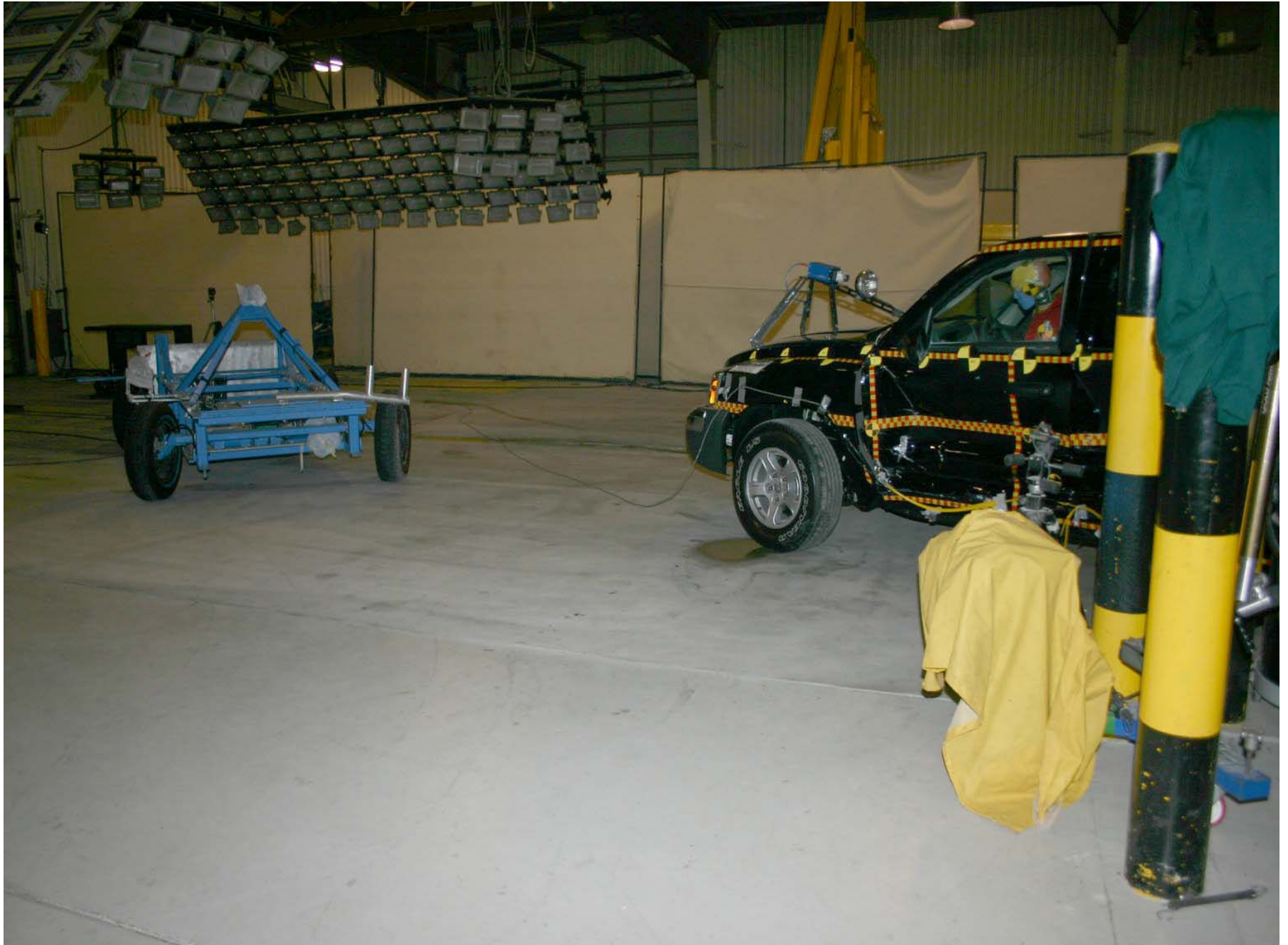
Post-Test MDB (Rear) and Vehicle
