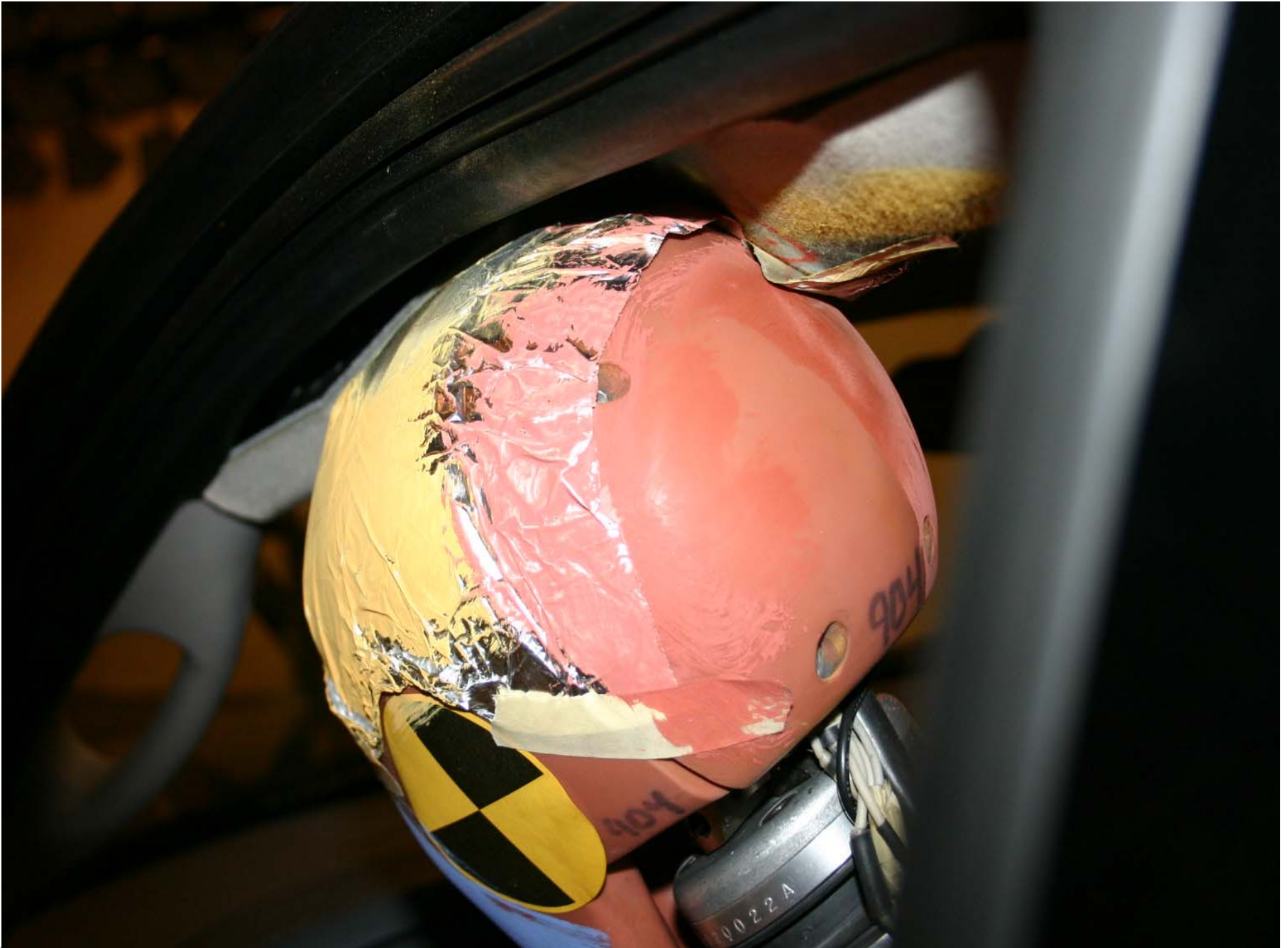
Post-Test Driver Dummy Head Contact
