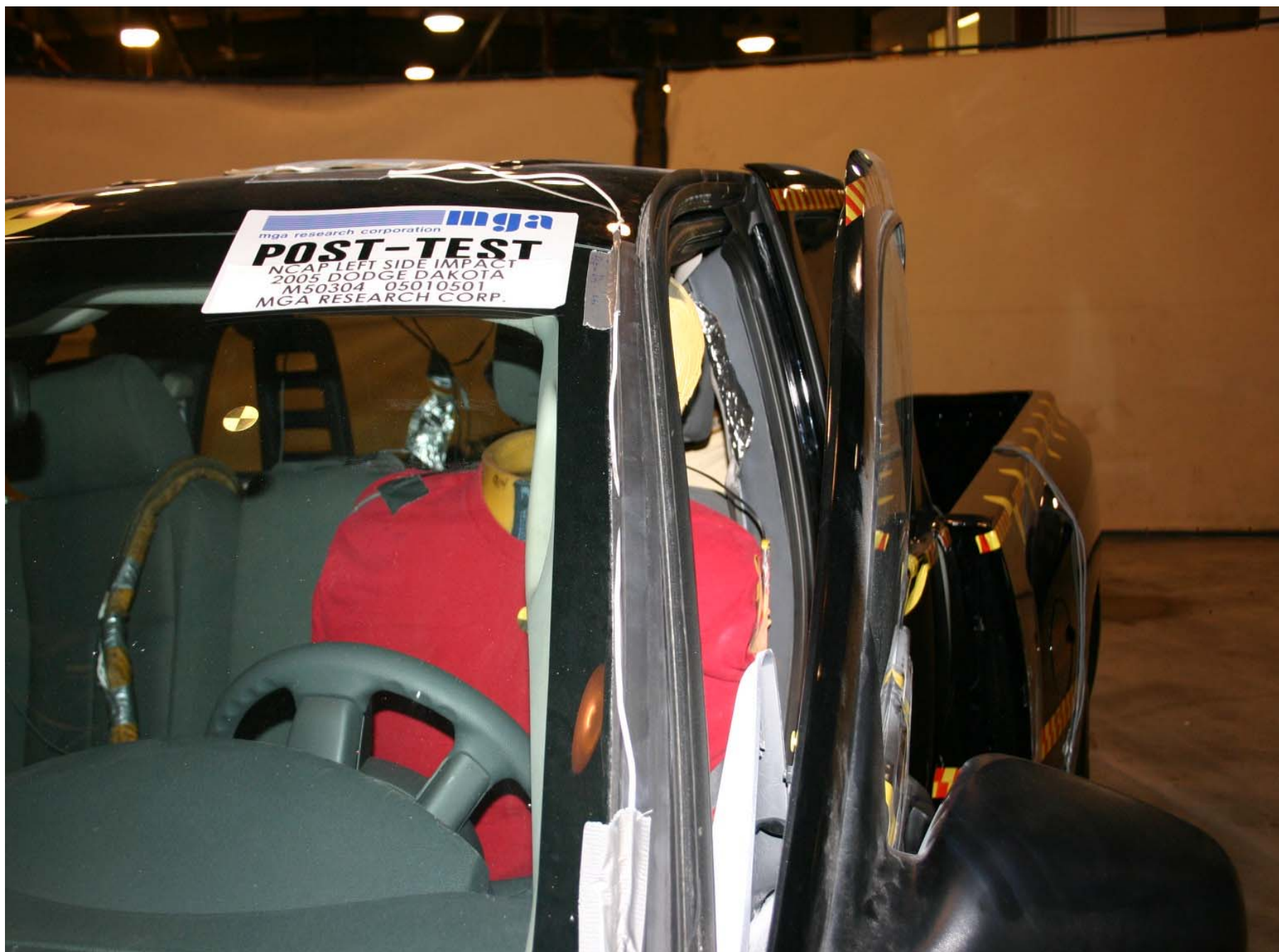
Post-Test Left Front Door Opening
