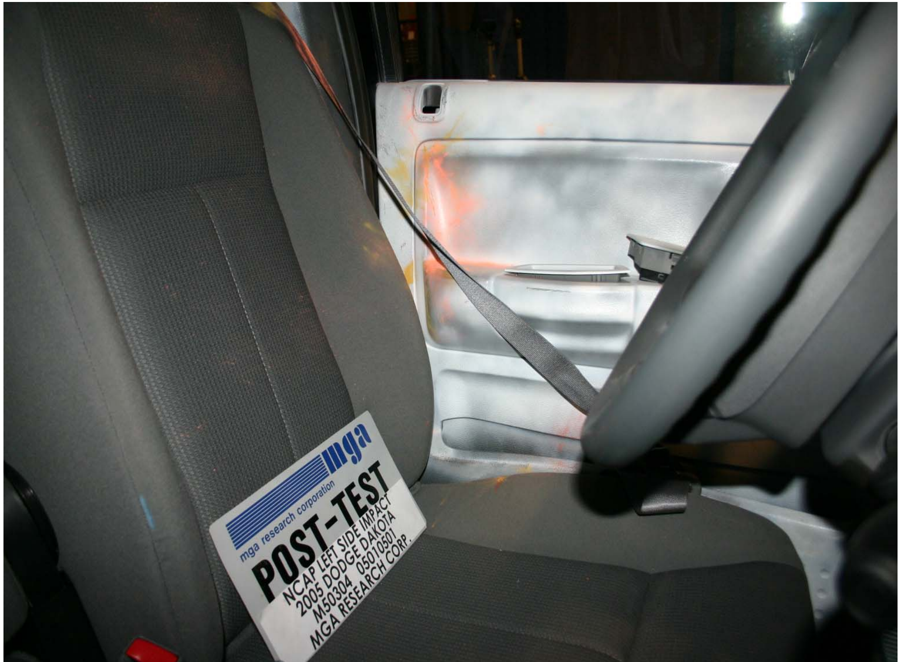
Post-Test Driver Dummy Mid Contact
