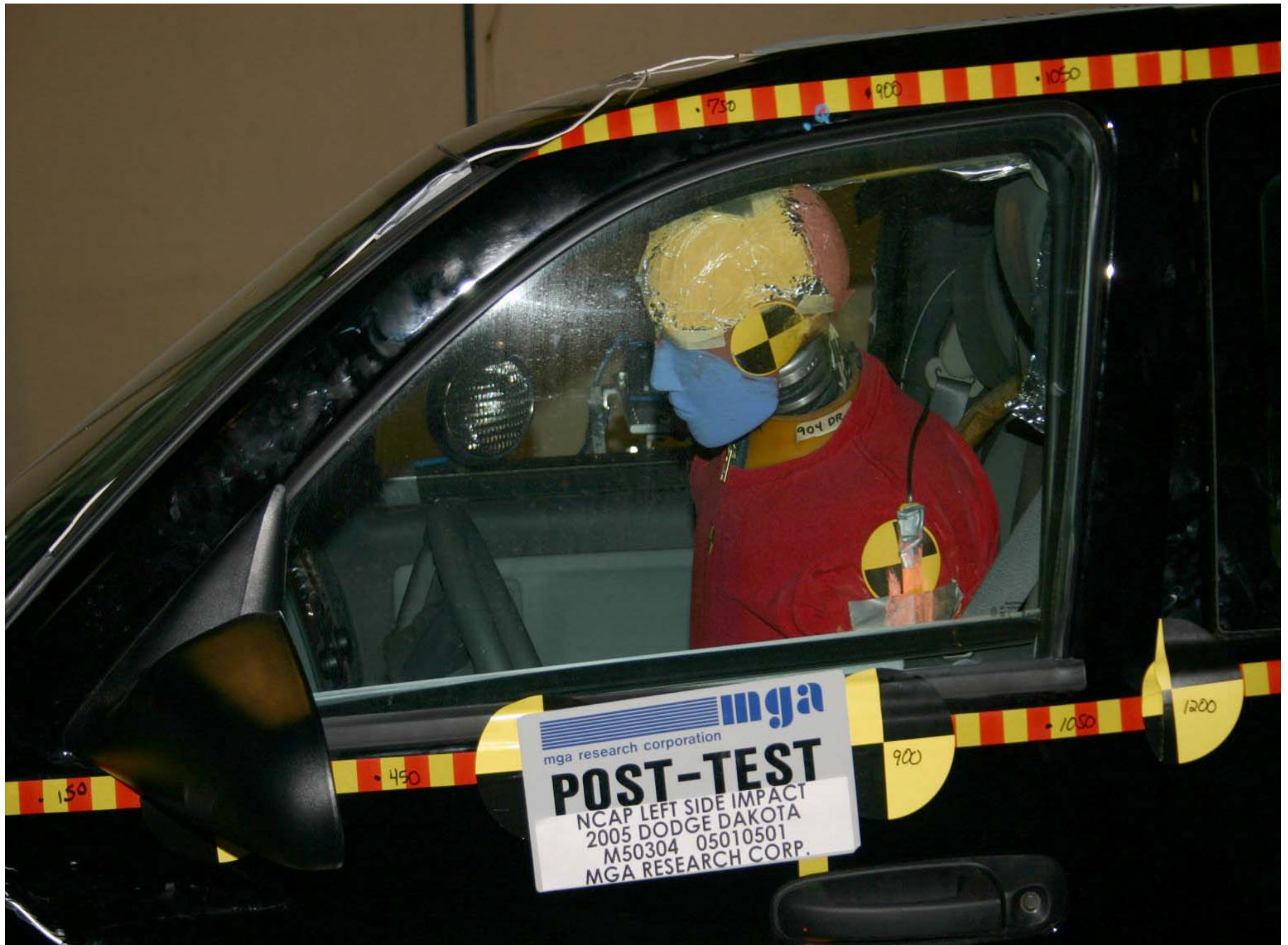
Post-Test Driver Dummy Left Side View
