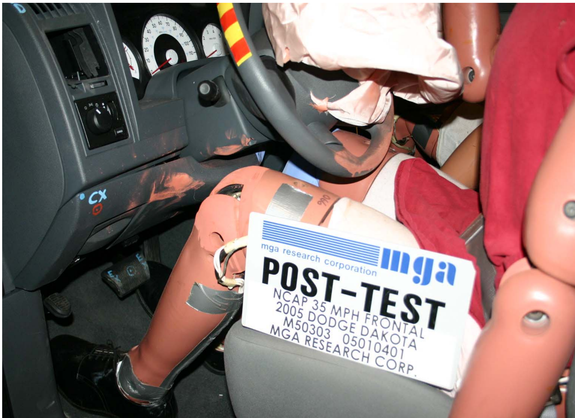
Post-Test Driver Side Knee Bolster View
