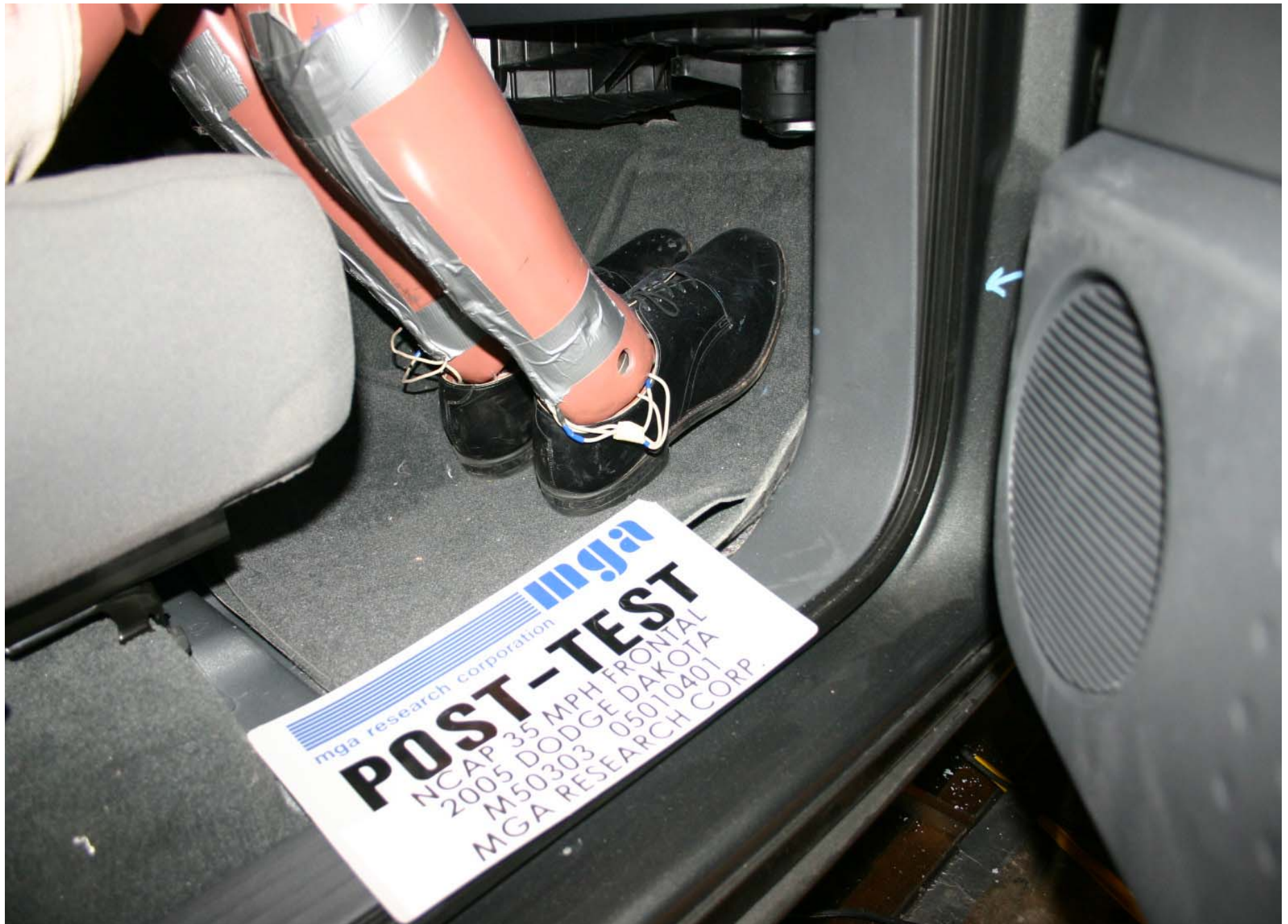
Post-Test Passenger Dummy Feet Position
