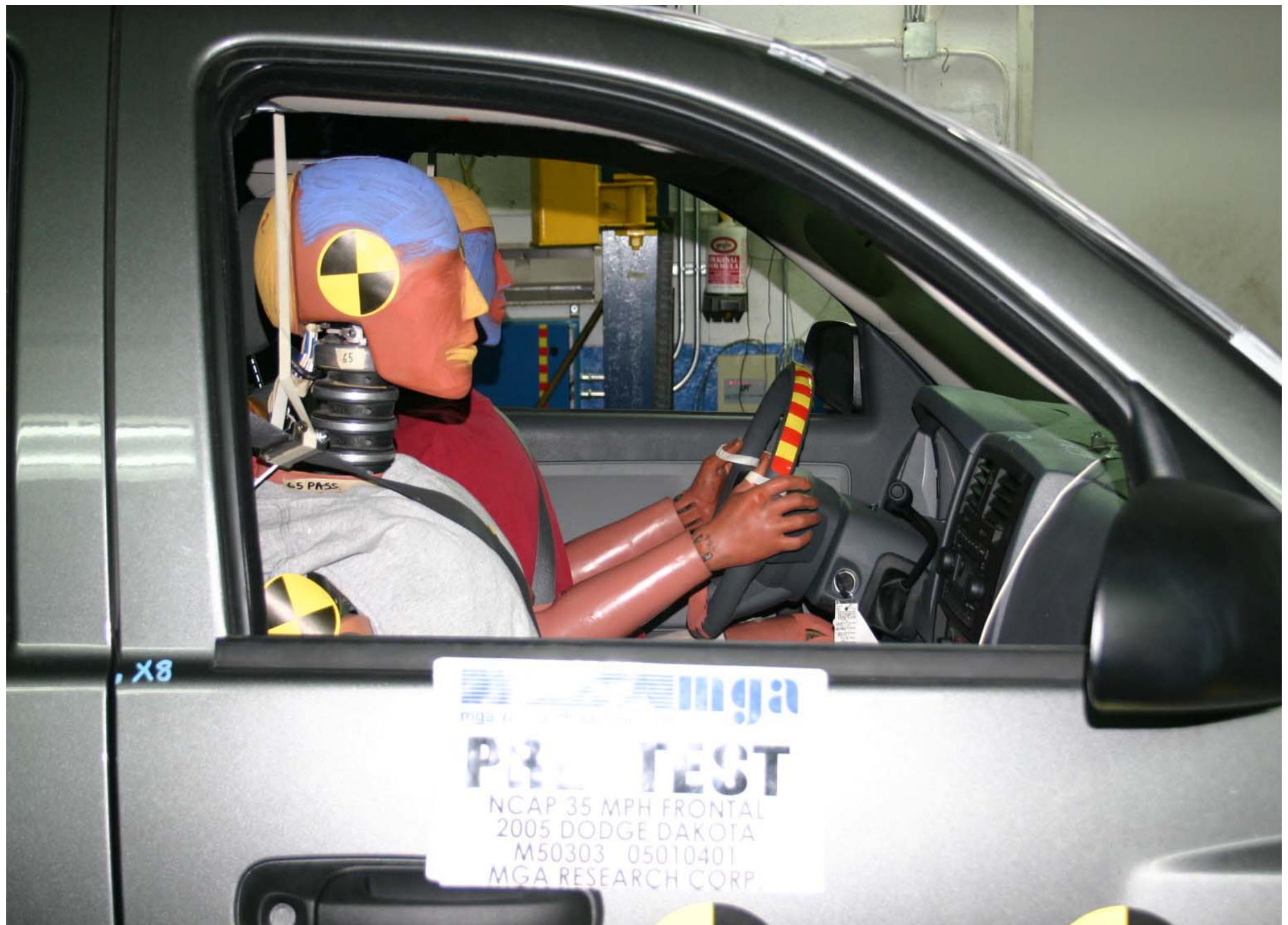
Pre-Test Passenger Dummy Position Right Side View
