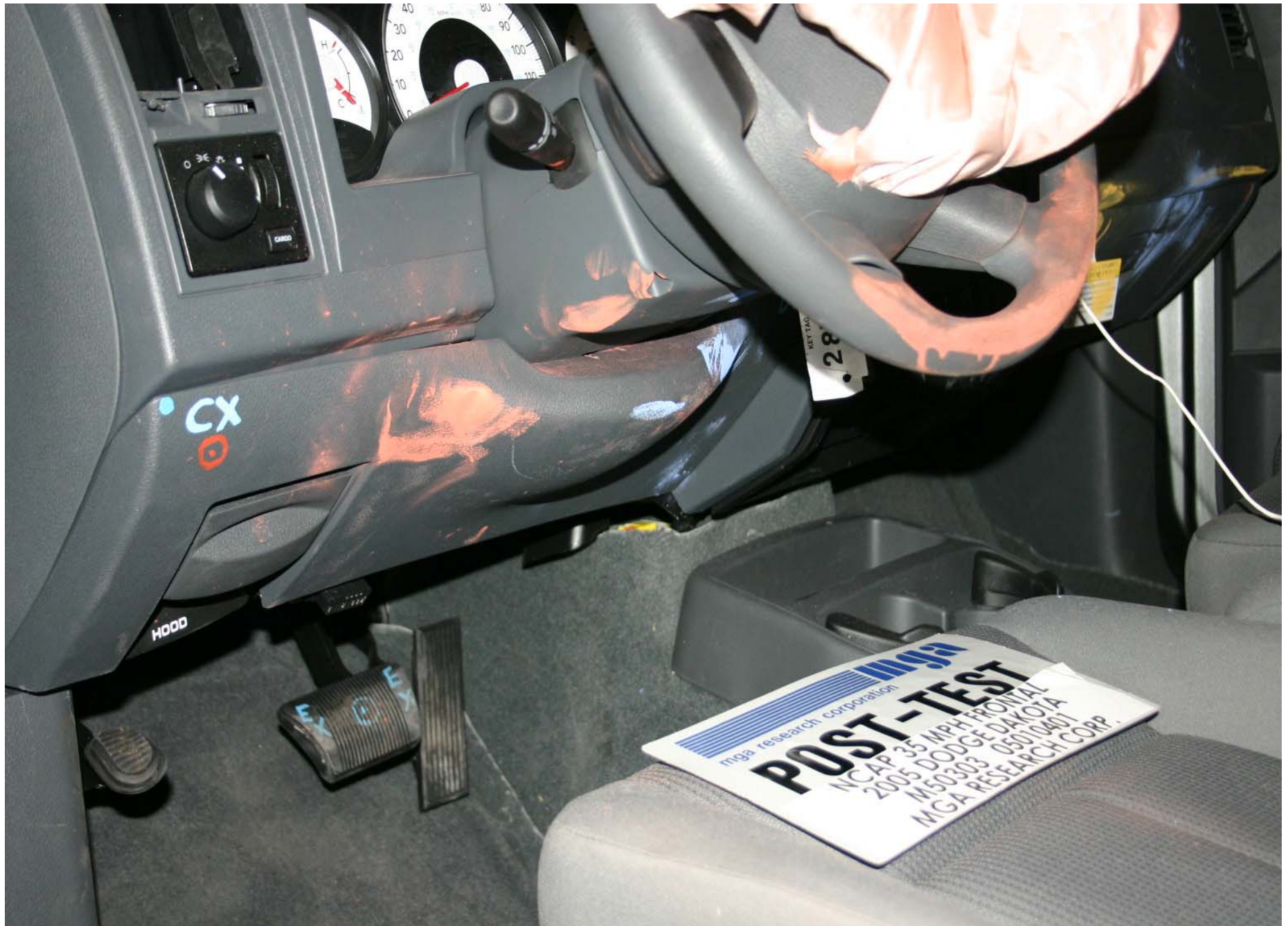
Post-Test Driver Dummy Knee Contact
