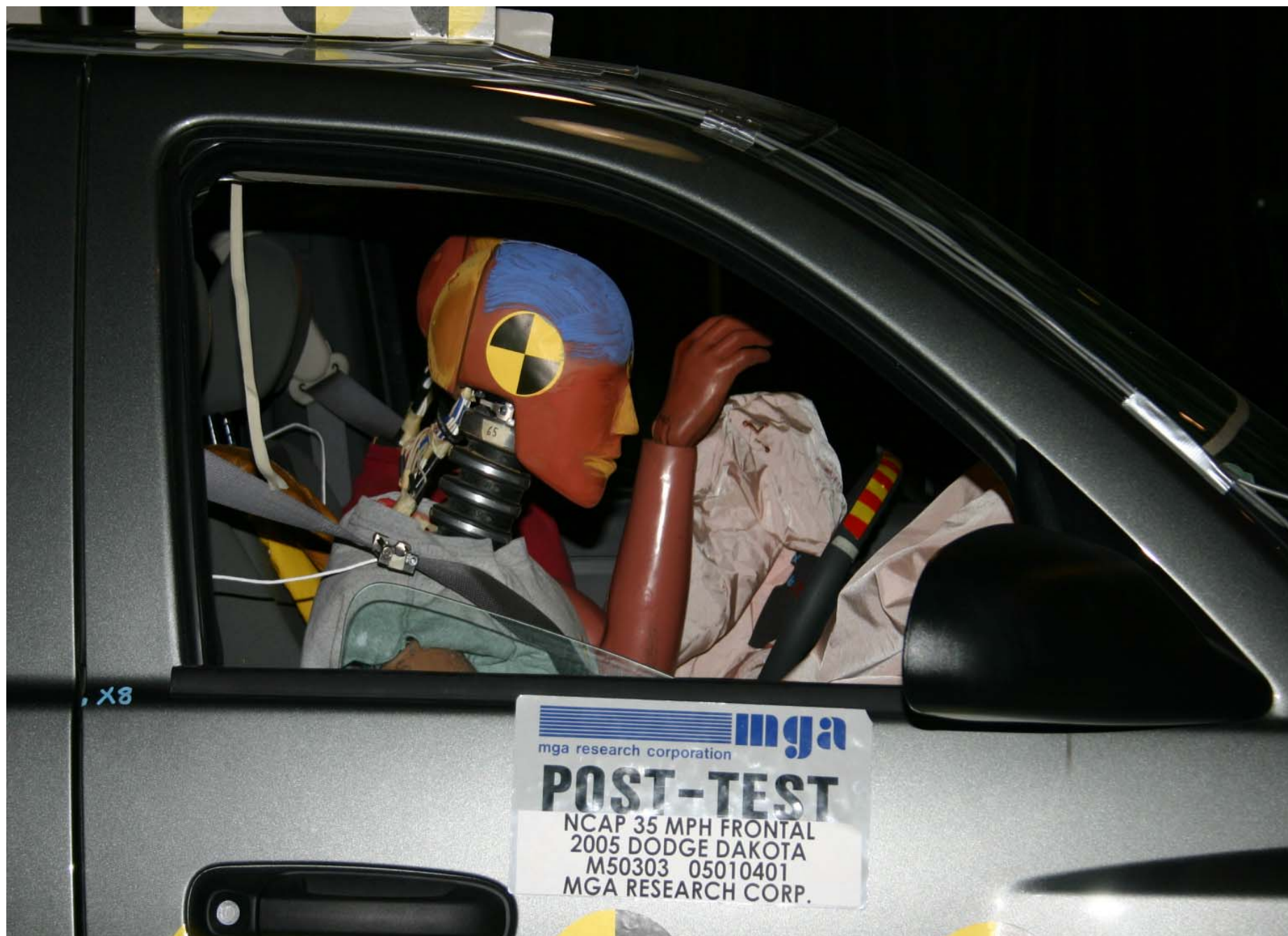
Post-Test Passenger Dummy Position Right Side View
