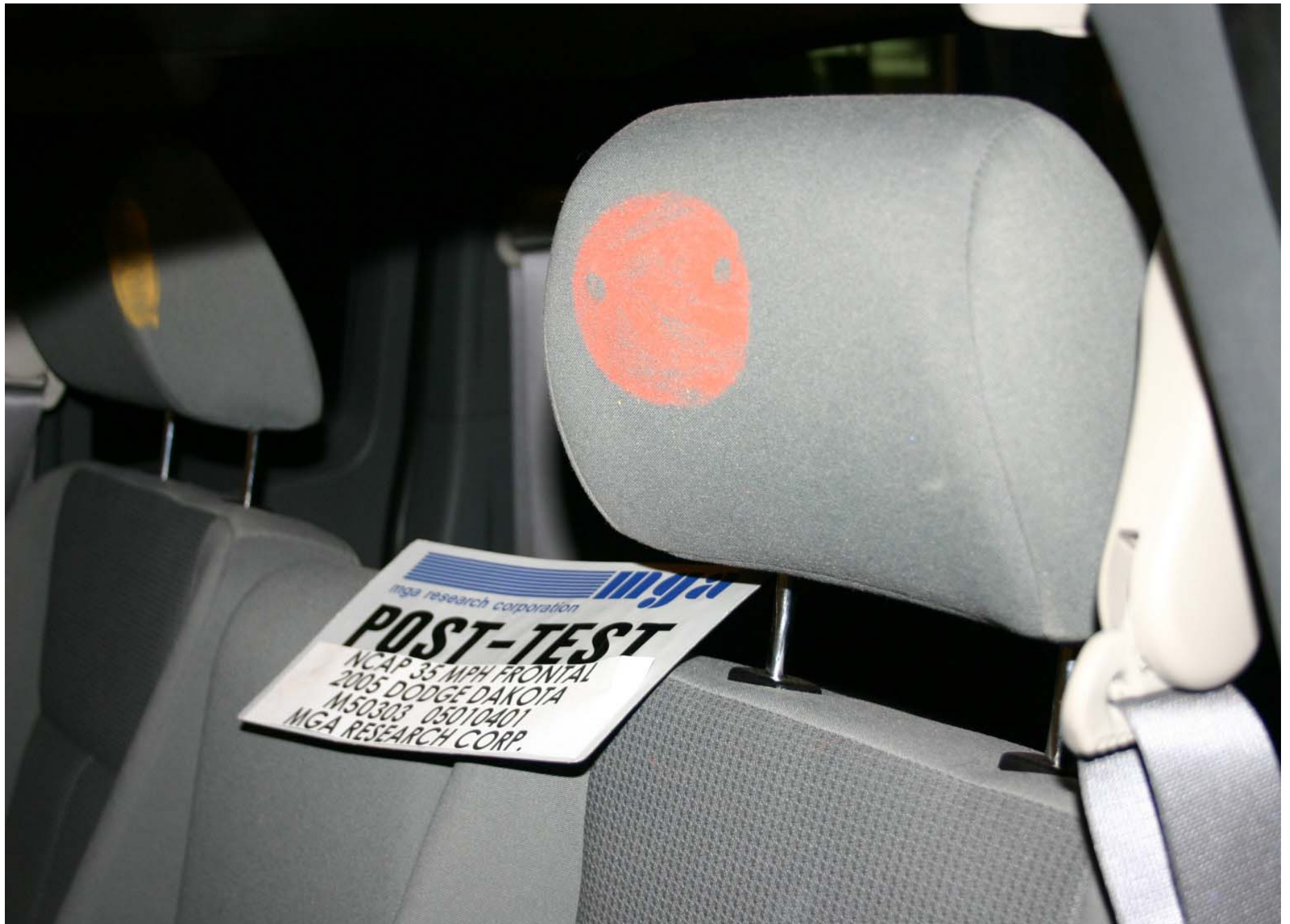
Post-Test Driver Dummy Head Contact
