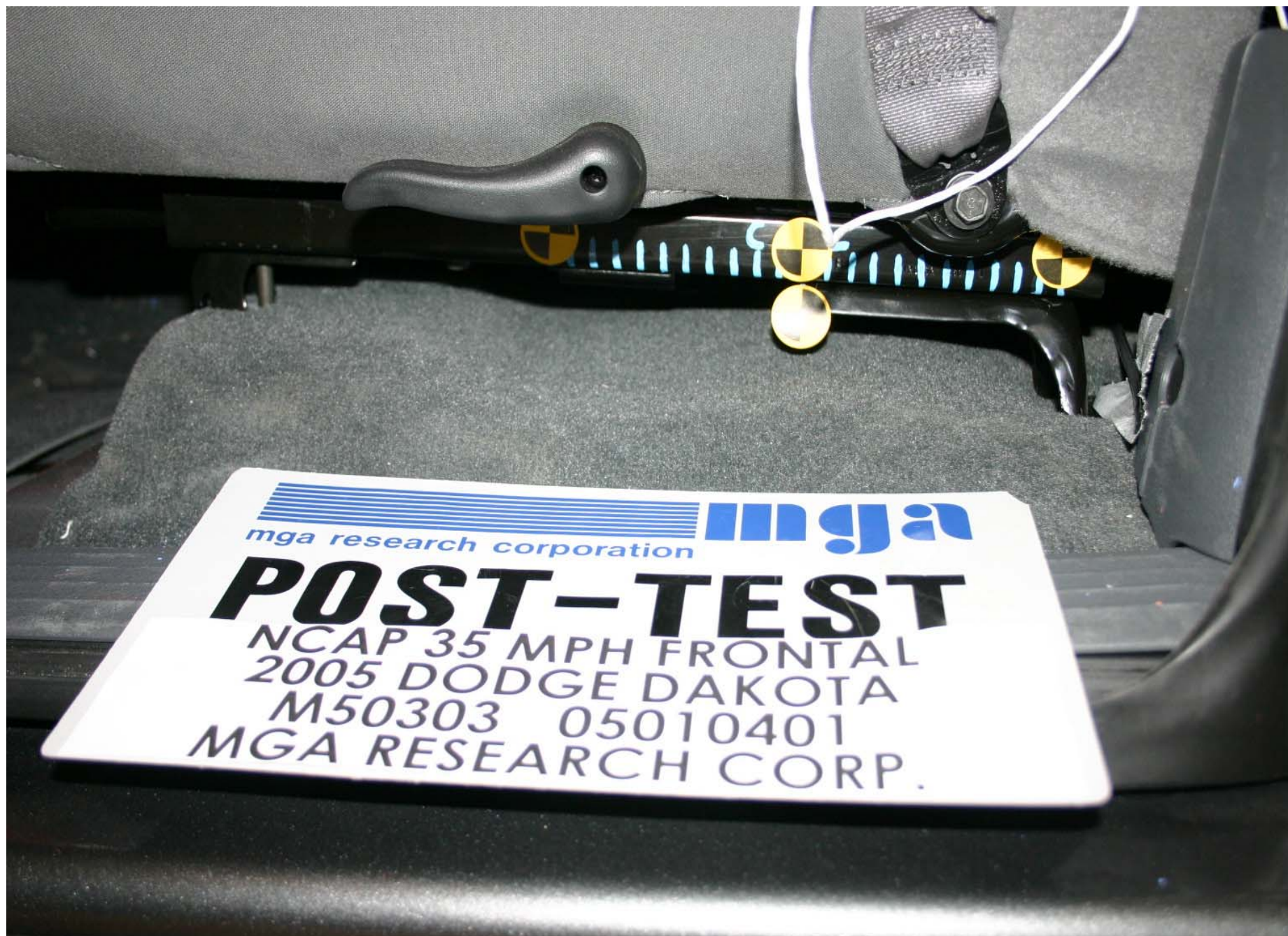
Post-Test Driver Dummy Seat Position
