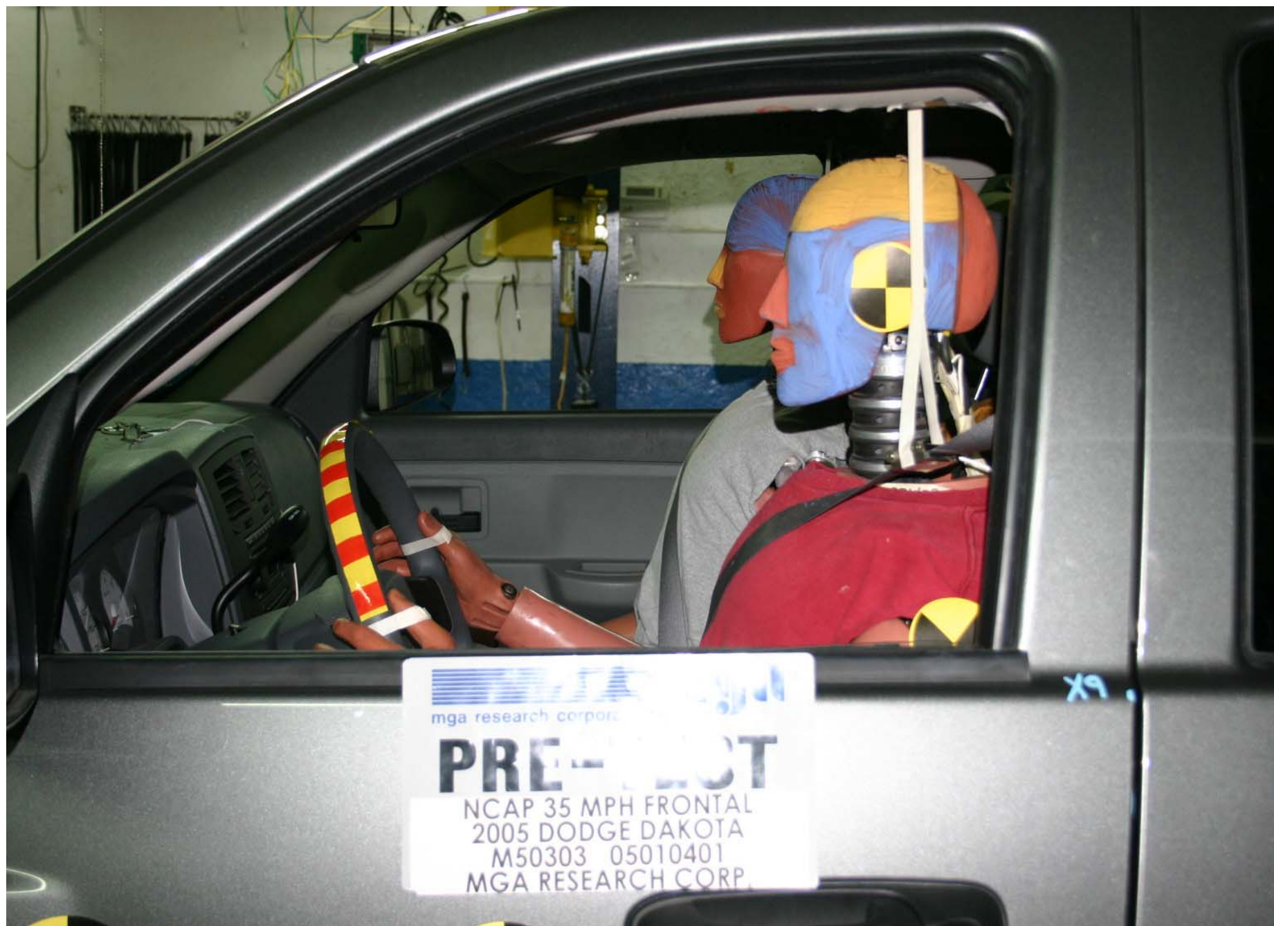
Pre-Test Driver Dummy Position Left Side View
