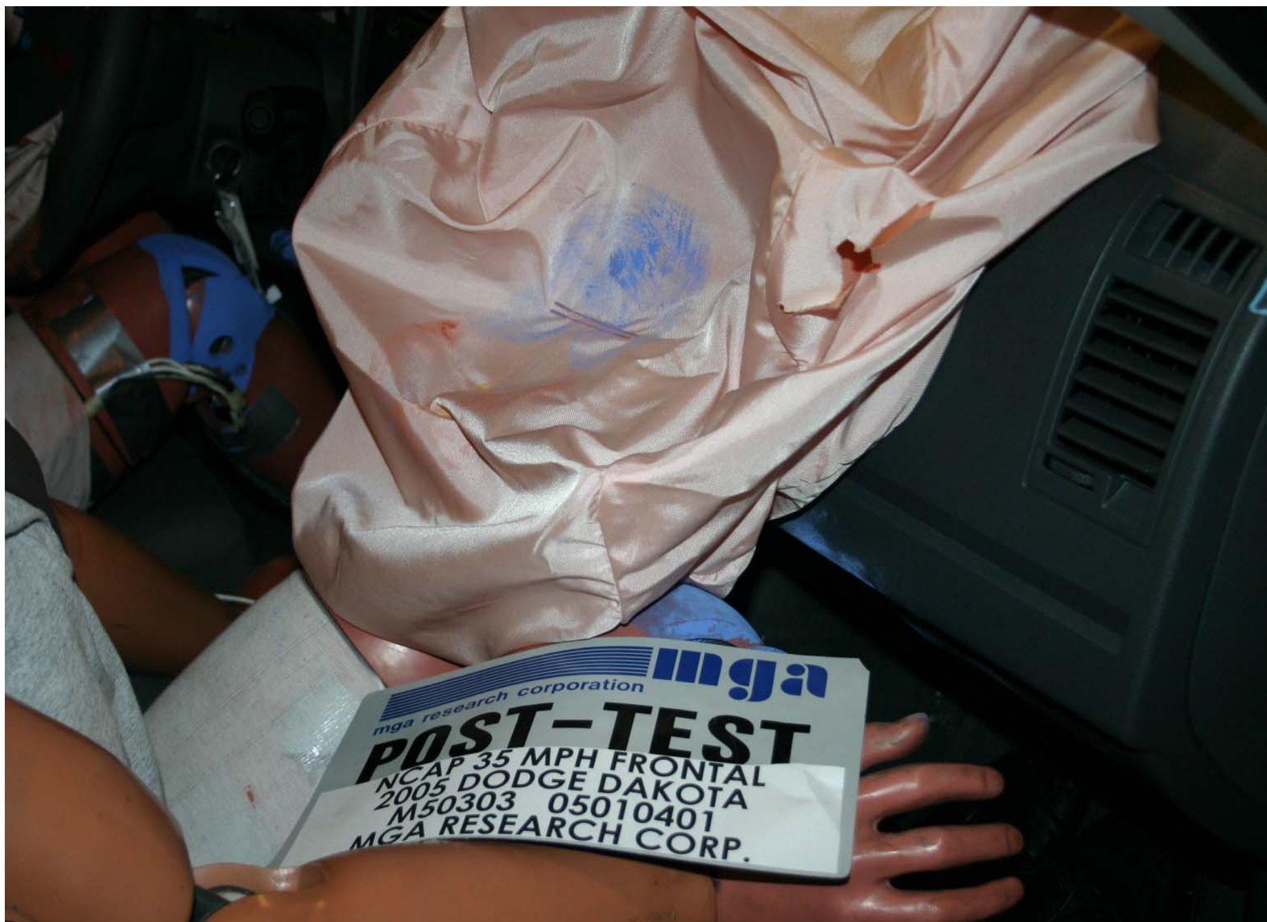
Post-Test Passenger Dummy Airbag Contact
