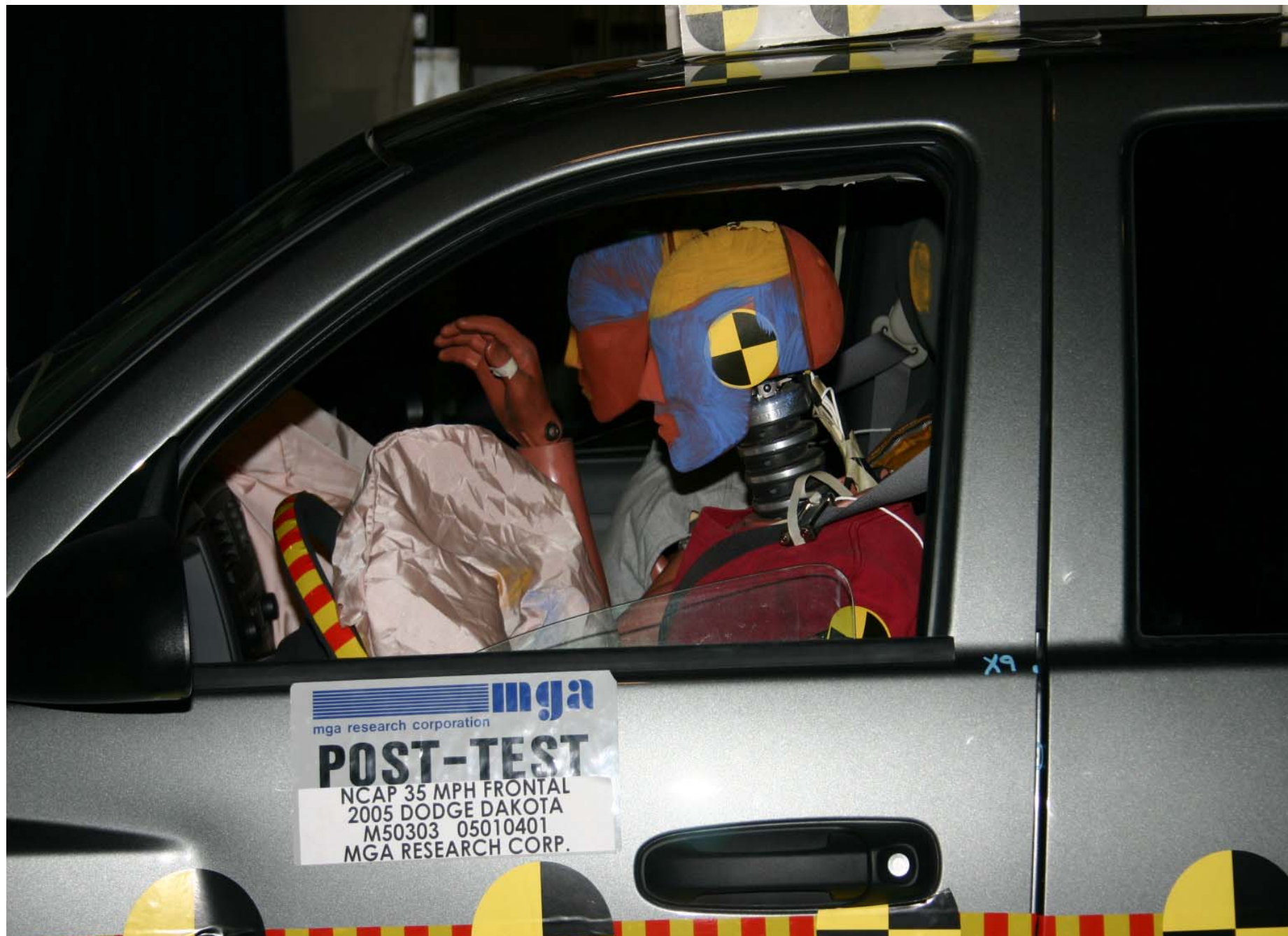
Post-Test Driver Dummy Position Left Side View
