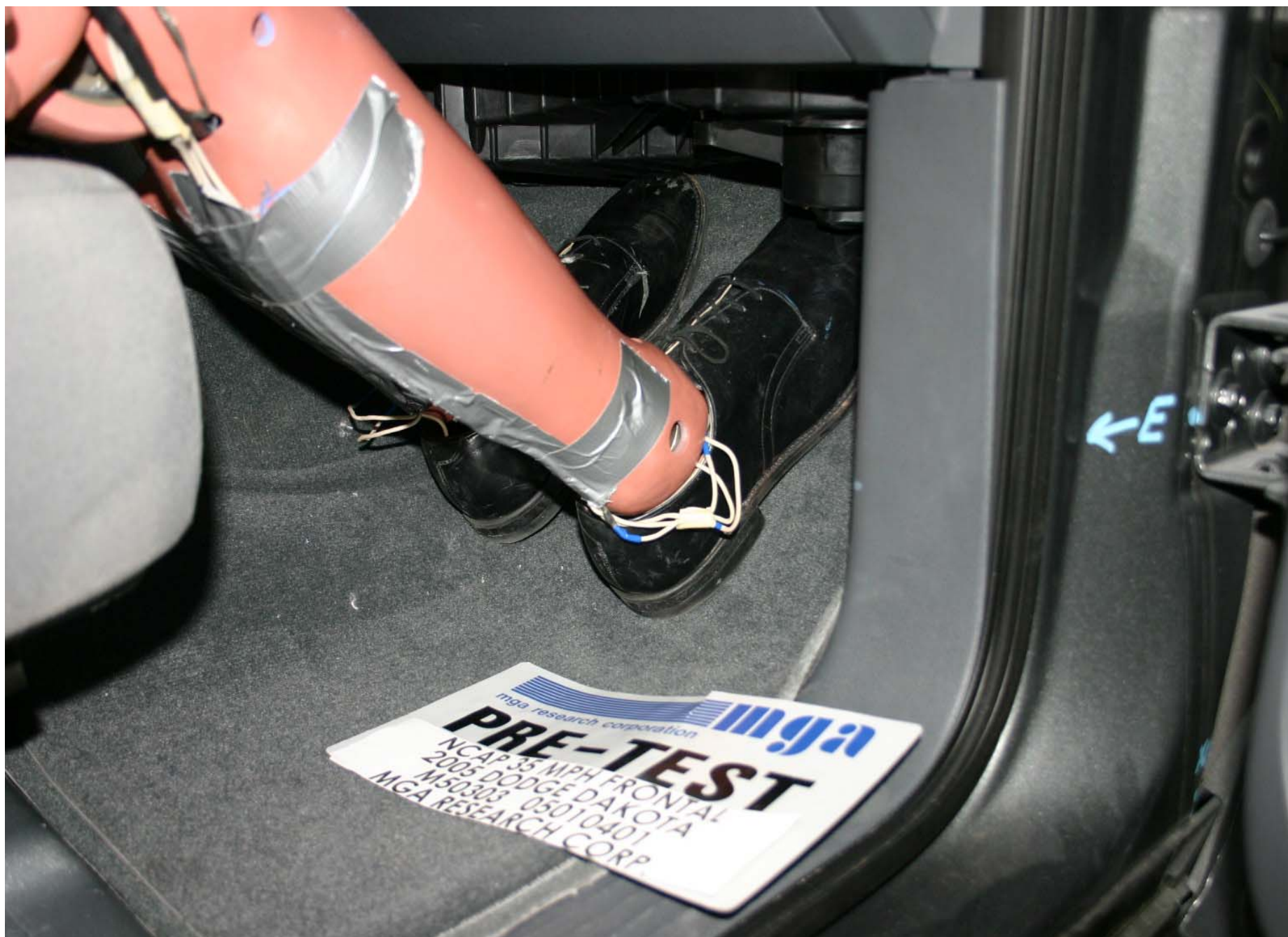
Pre-Test Passenger Dummy Feet Position
