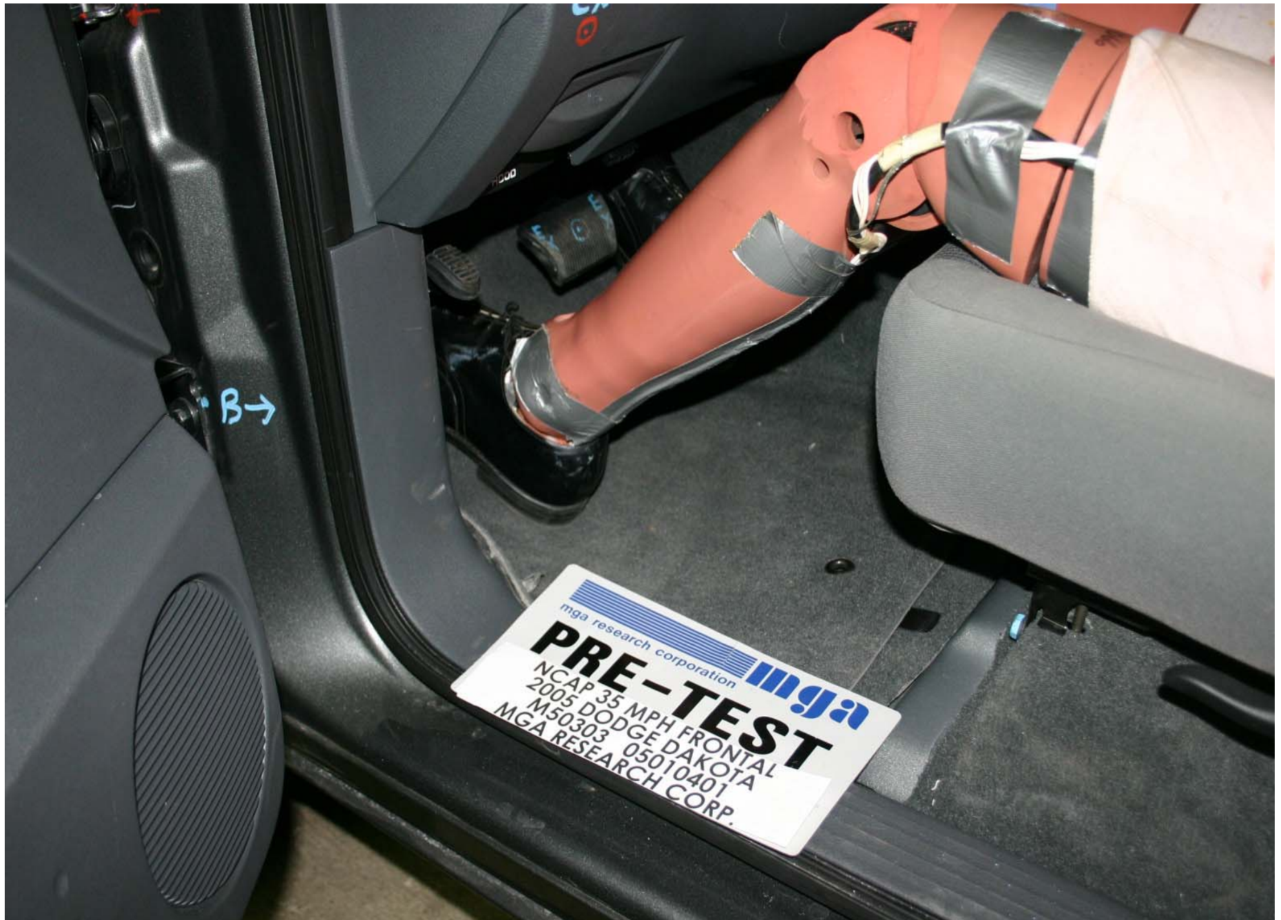
Pre-Test Driver Dummy Feet Position
