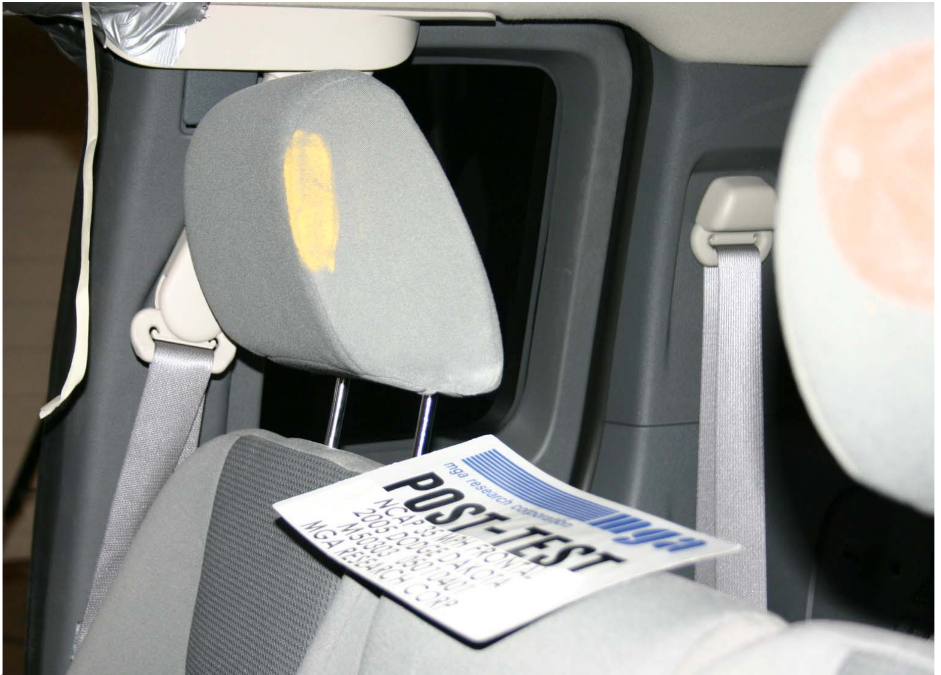
Post-Test Passenger Dummy Head Contact
