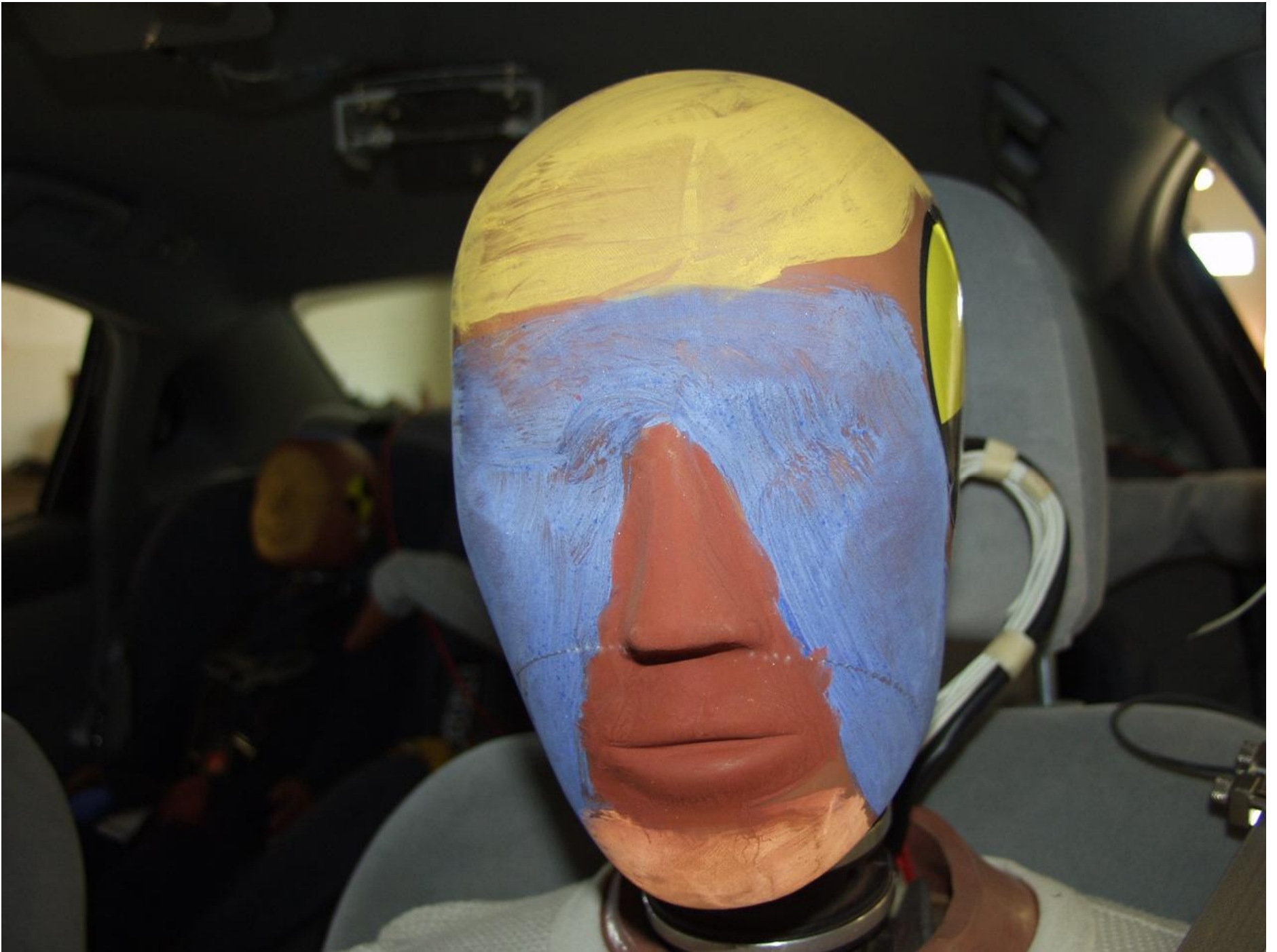
Figure A-42 POST-TEST DRIVER HEAD VIEW
