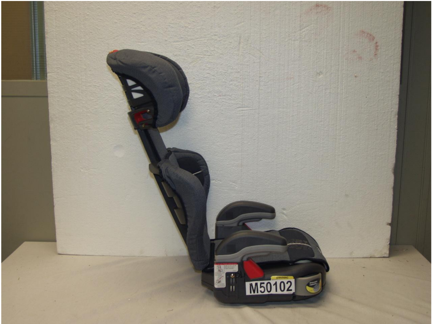
Figure 3-18: POST-TEST RIGHT SIDE VIEW OF POSITION 4 CRS
