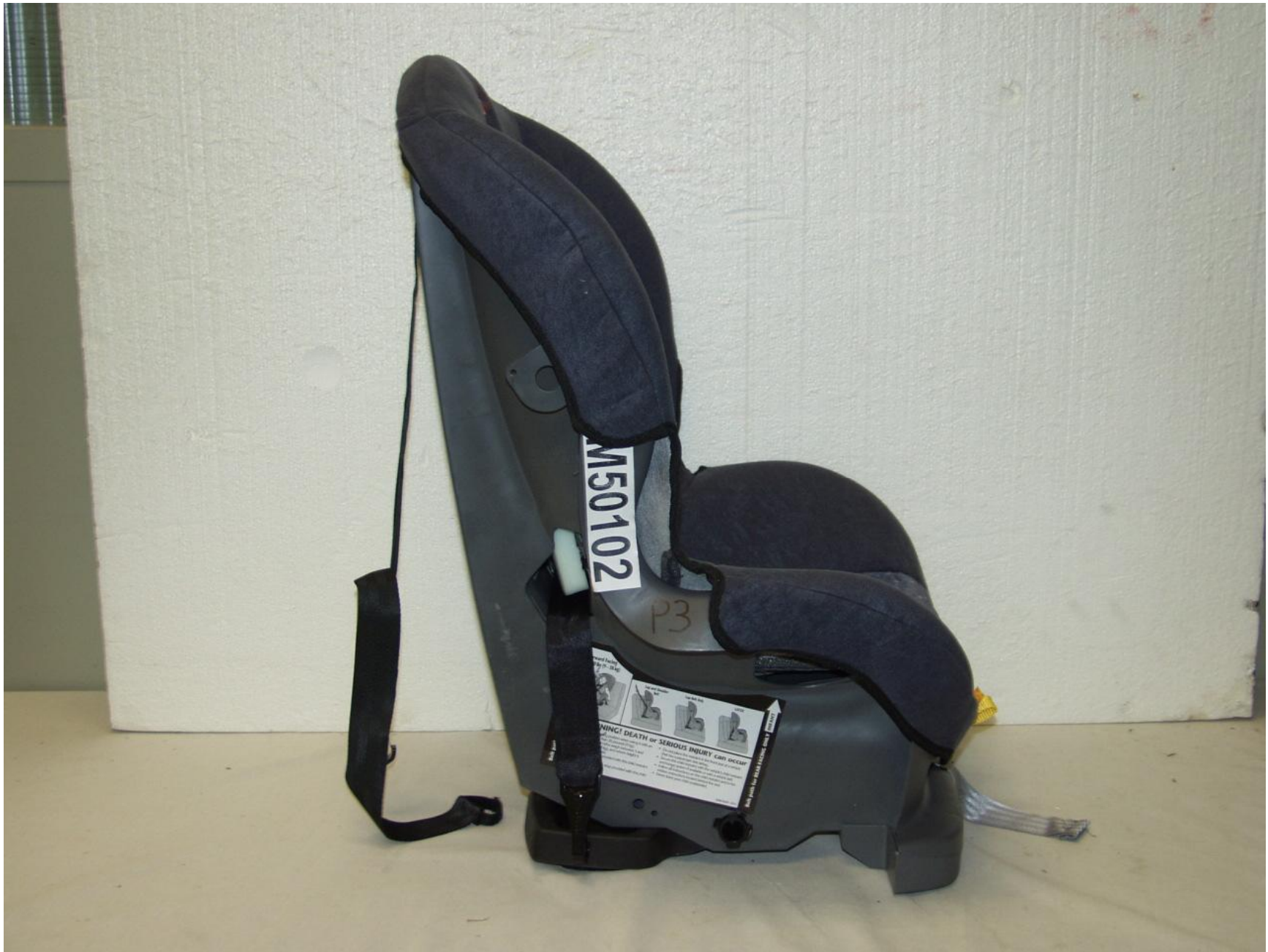
Figure 3-9: POST-TEST RIGHT SIDE VIEW OF POSITION 3 CRS
