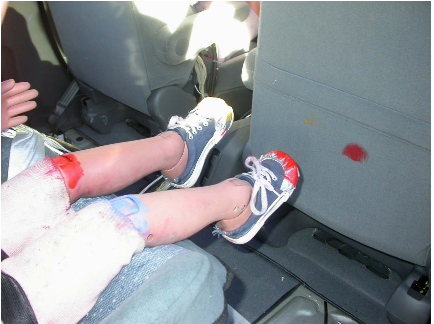
Figure F2-18: Post-Test Position 3 Dummy Leg Contacts
