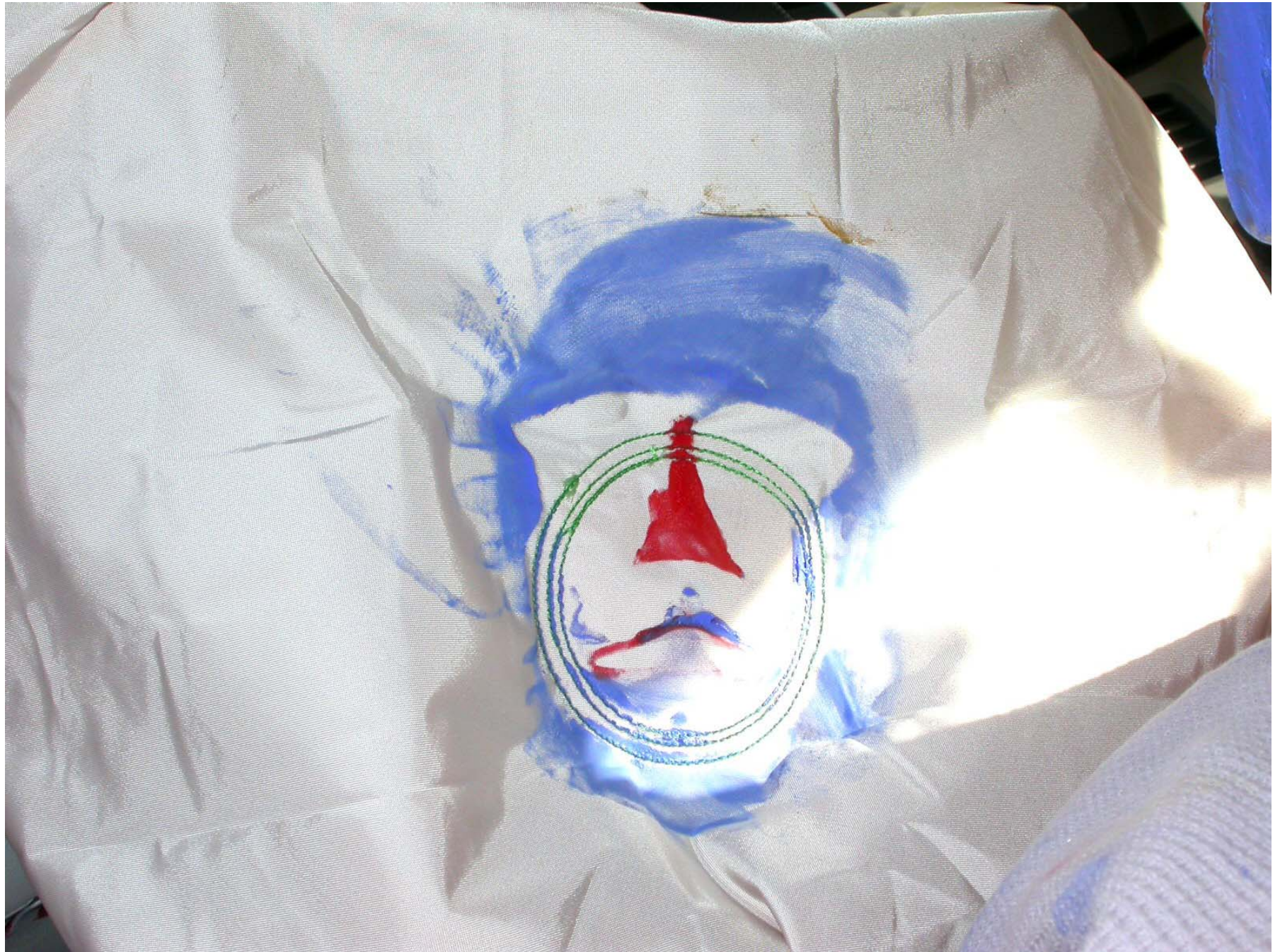
Figure A-43: Post-Test Driver Dummy Airbag Contact
