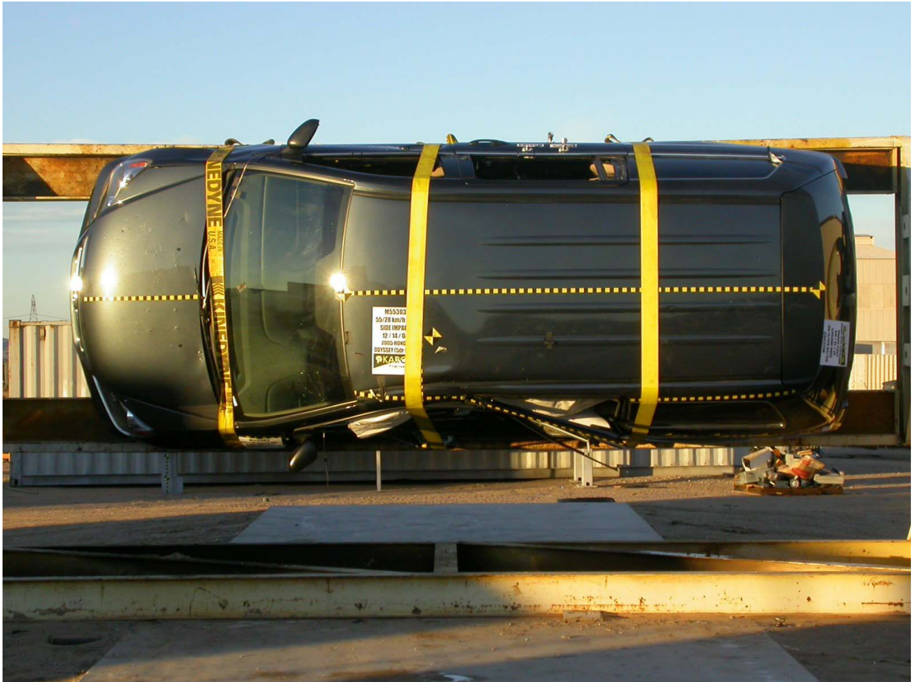
Figure A-64: Vehicle on Rollover Device (90°)
