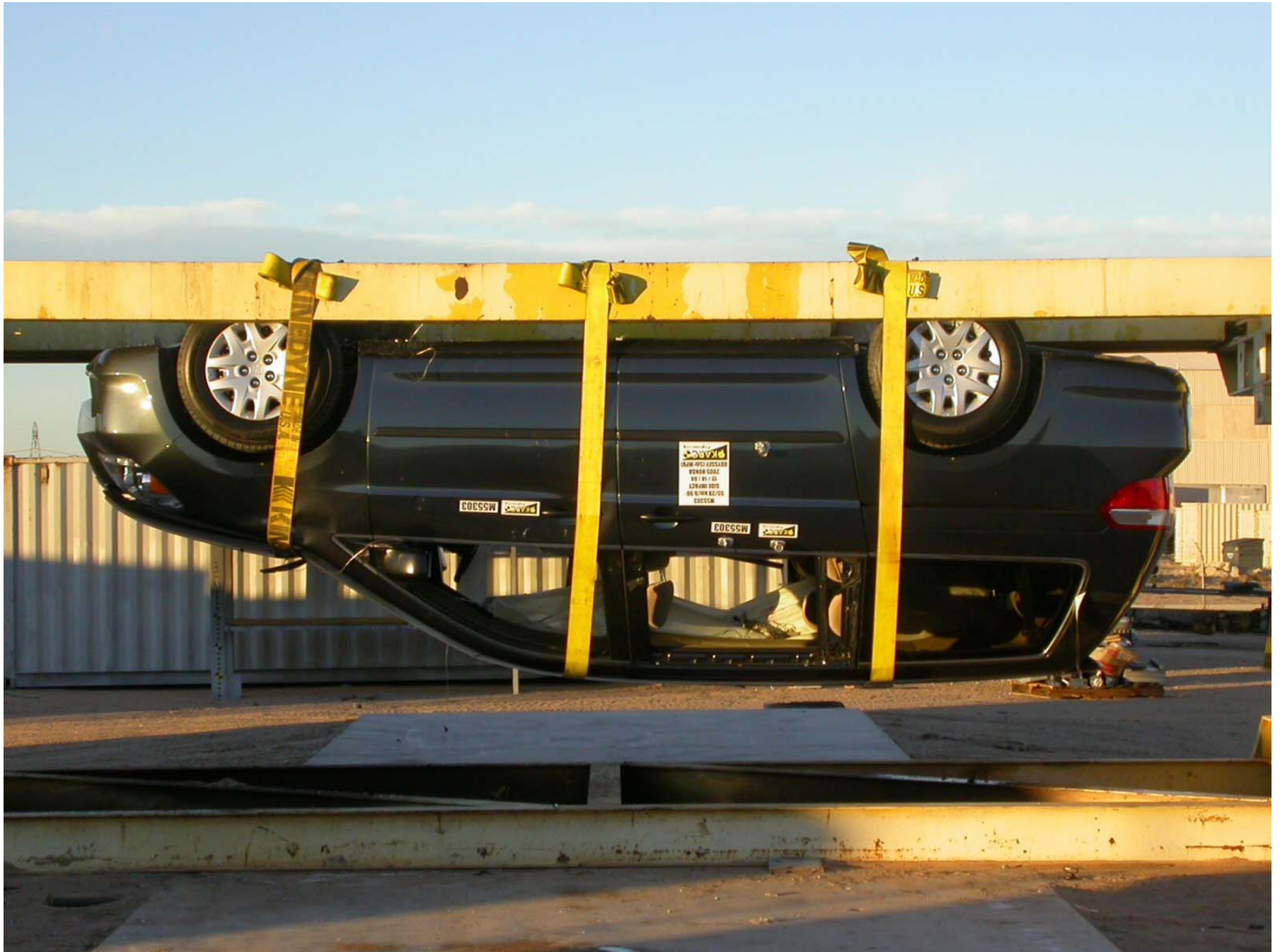
Figure A-65: Vehicle on Rollover Device (180°)
