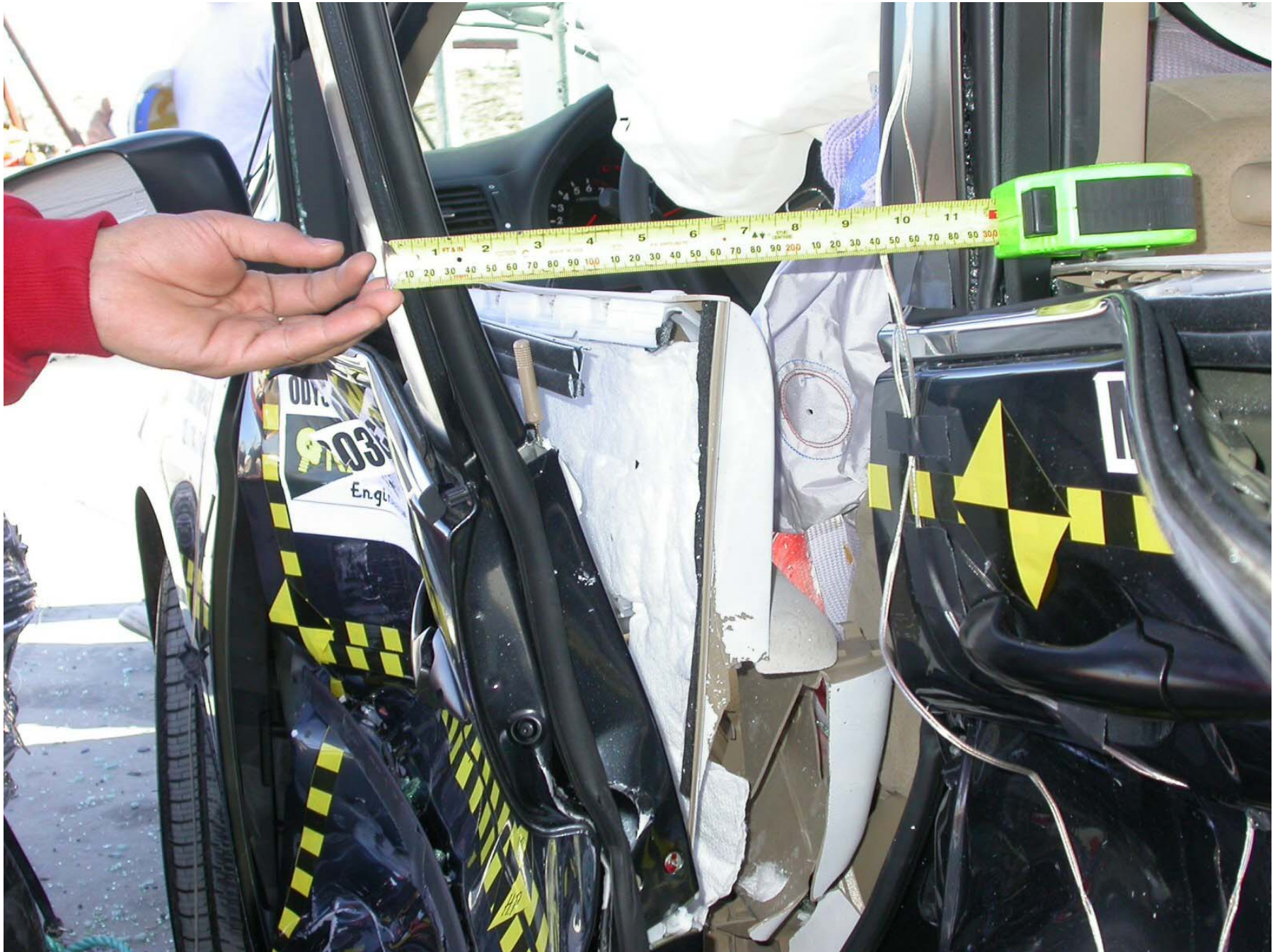
Figure A-70: Post-Test Driver Door (Unlatched)
