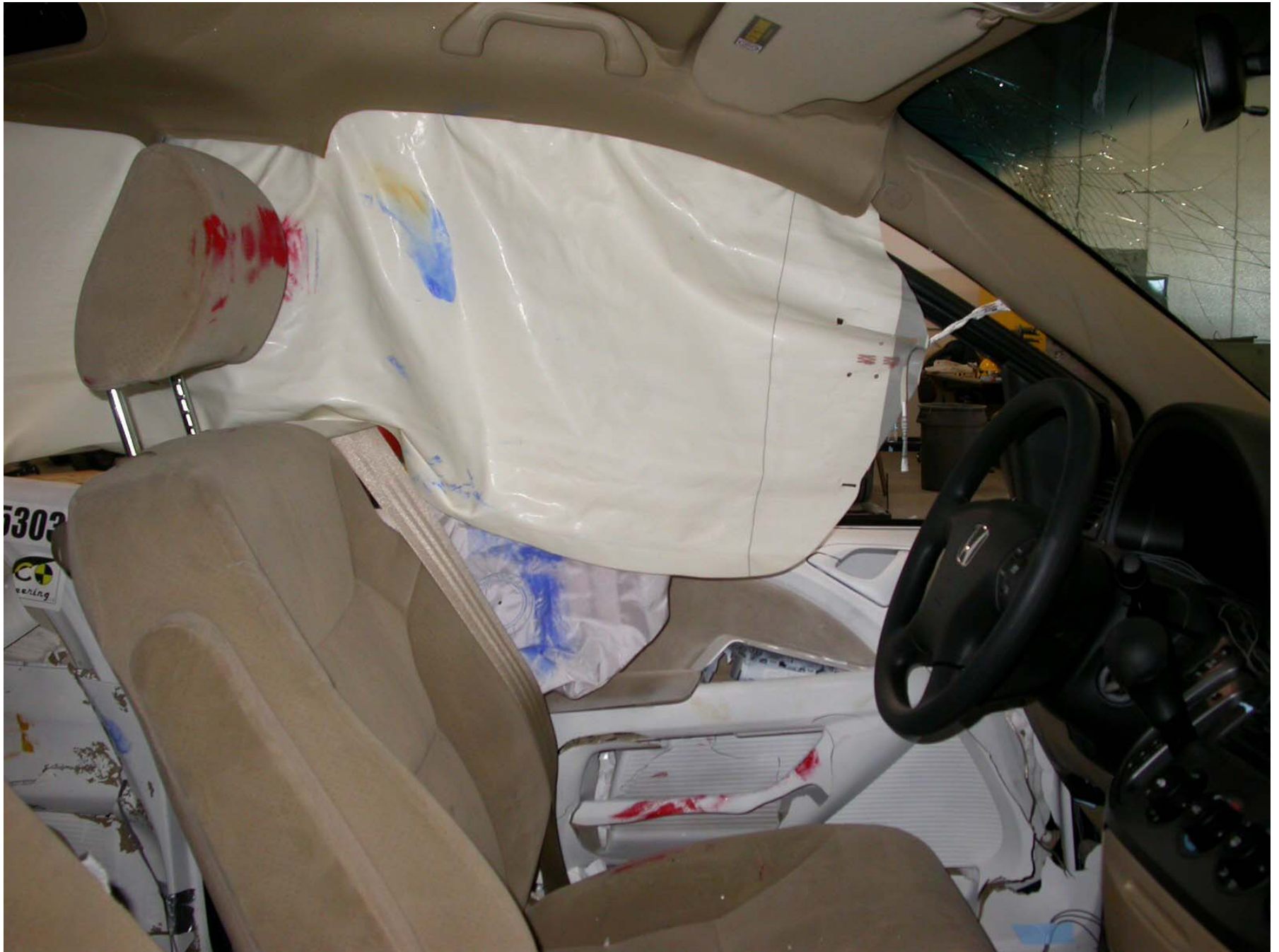
Figure A-45: Post-Test Front Door Panel (Interior)
