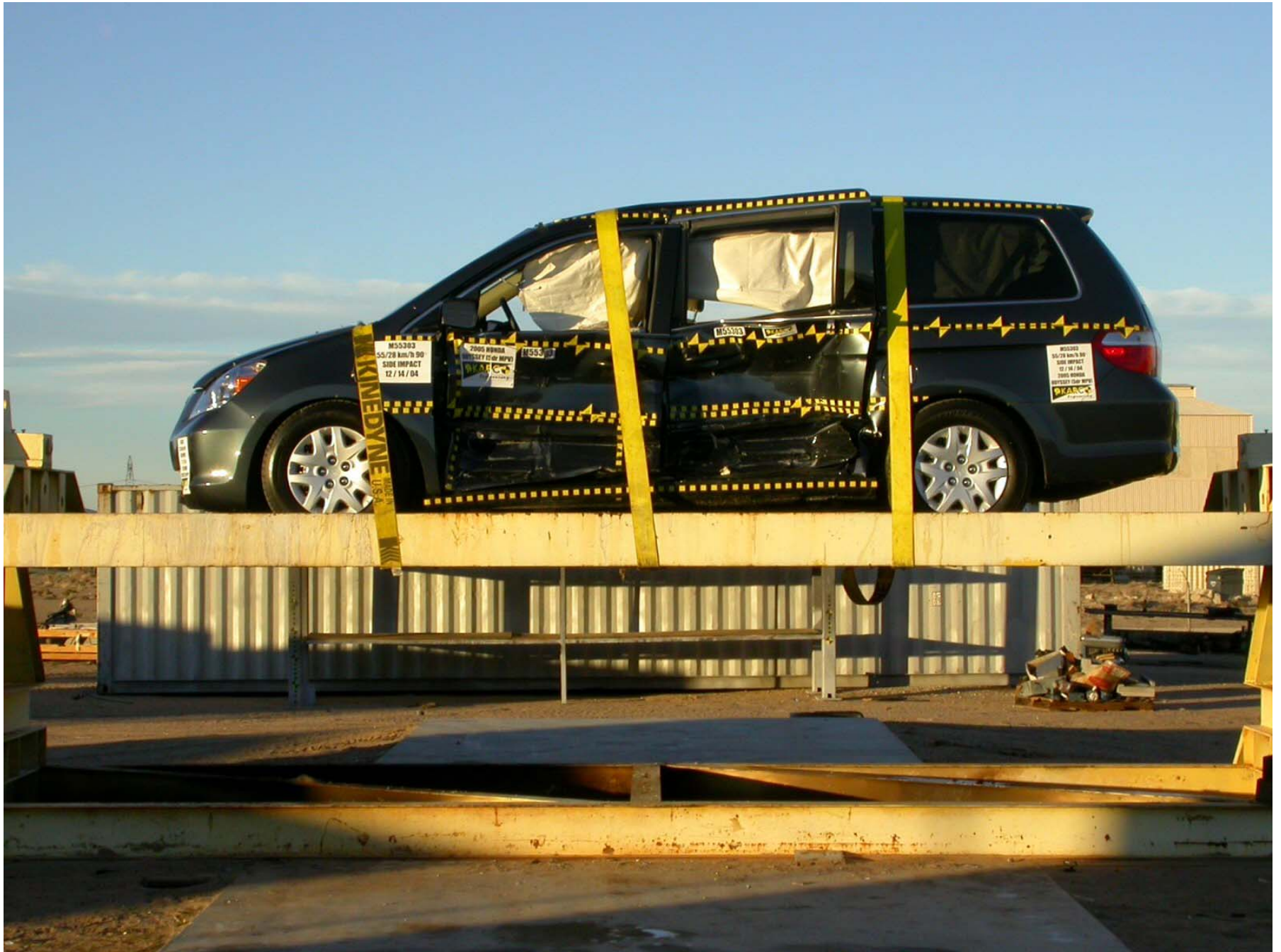
Figure A-63: Vehicle on Rollover Device (0°)
