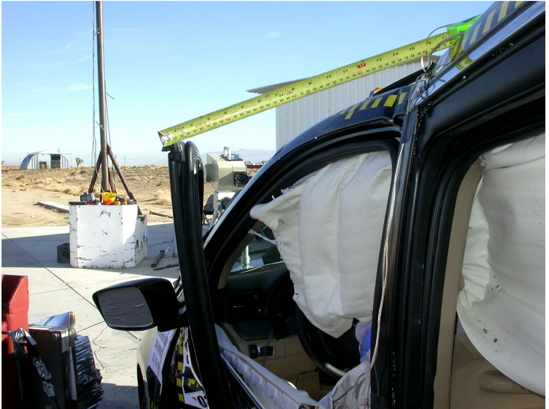
Figure A-69: Post-Test Driver Door (Unlatched)
