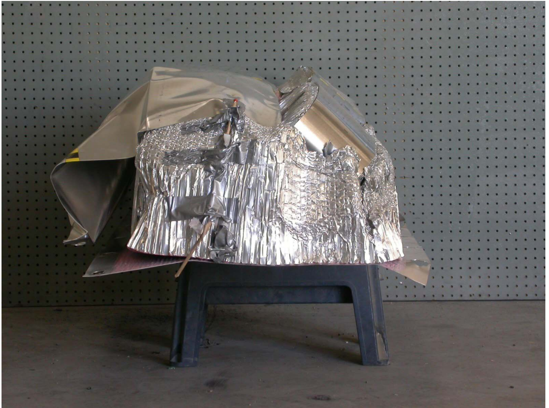
Figure A-60: Post-Test Right Side View of Deformable Barrier
