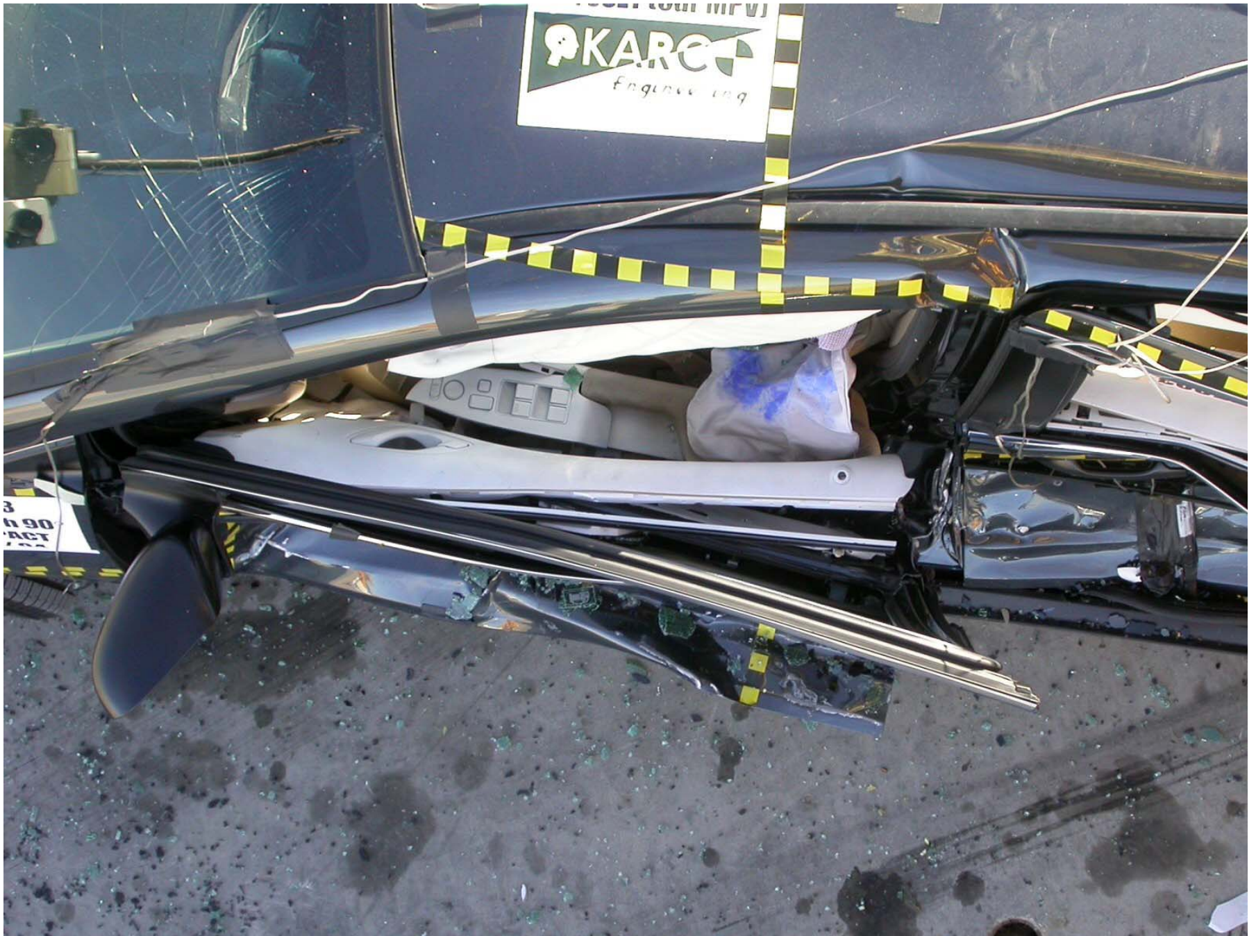
Figure A-41: Post-Test Driver Dummy Clearance From Door
