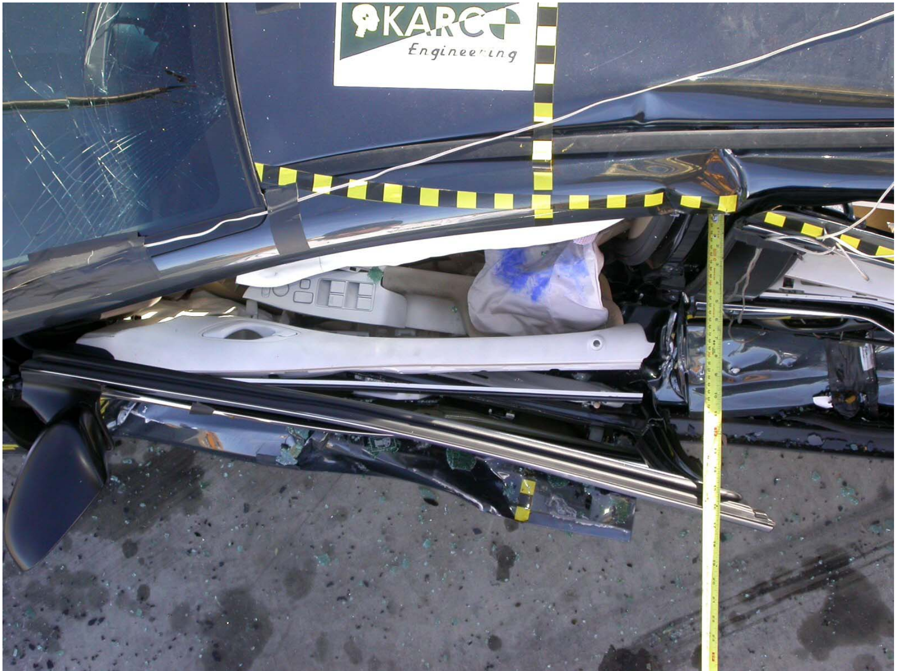
Figure A-68: Post-Test Driver Door (Unlatched)
