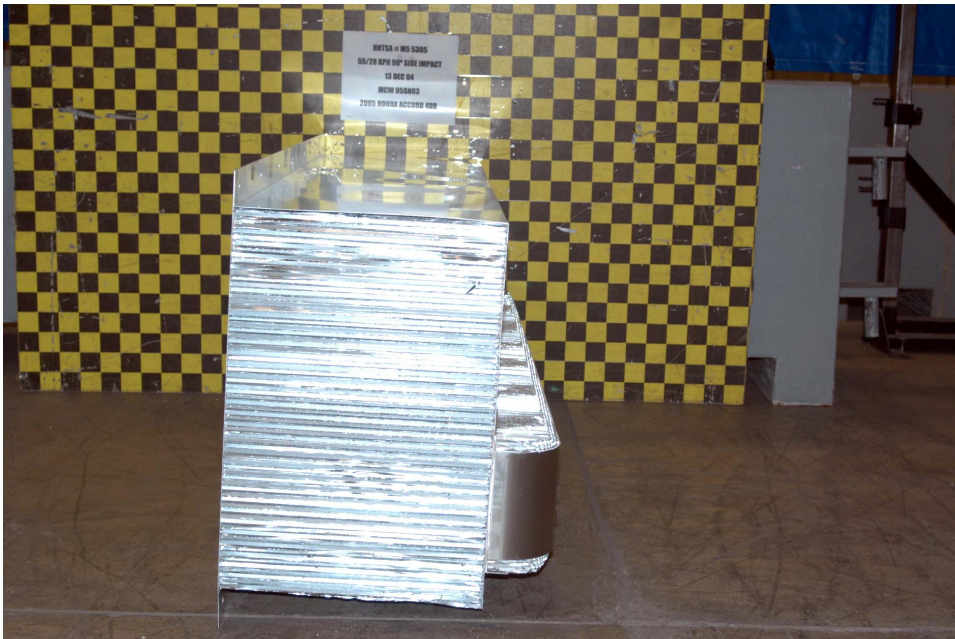
Figure A-51: PRE-TEST ALUMINUM BARRIER RIGHT SIDE
