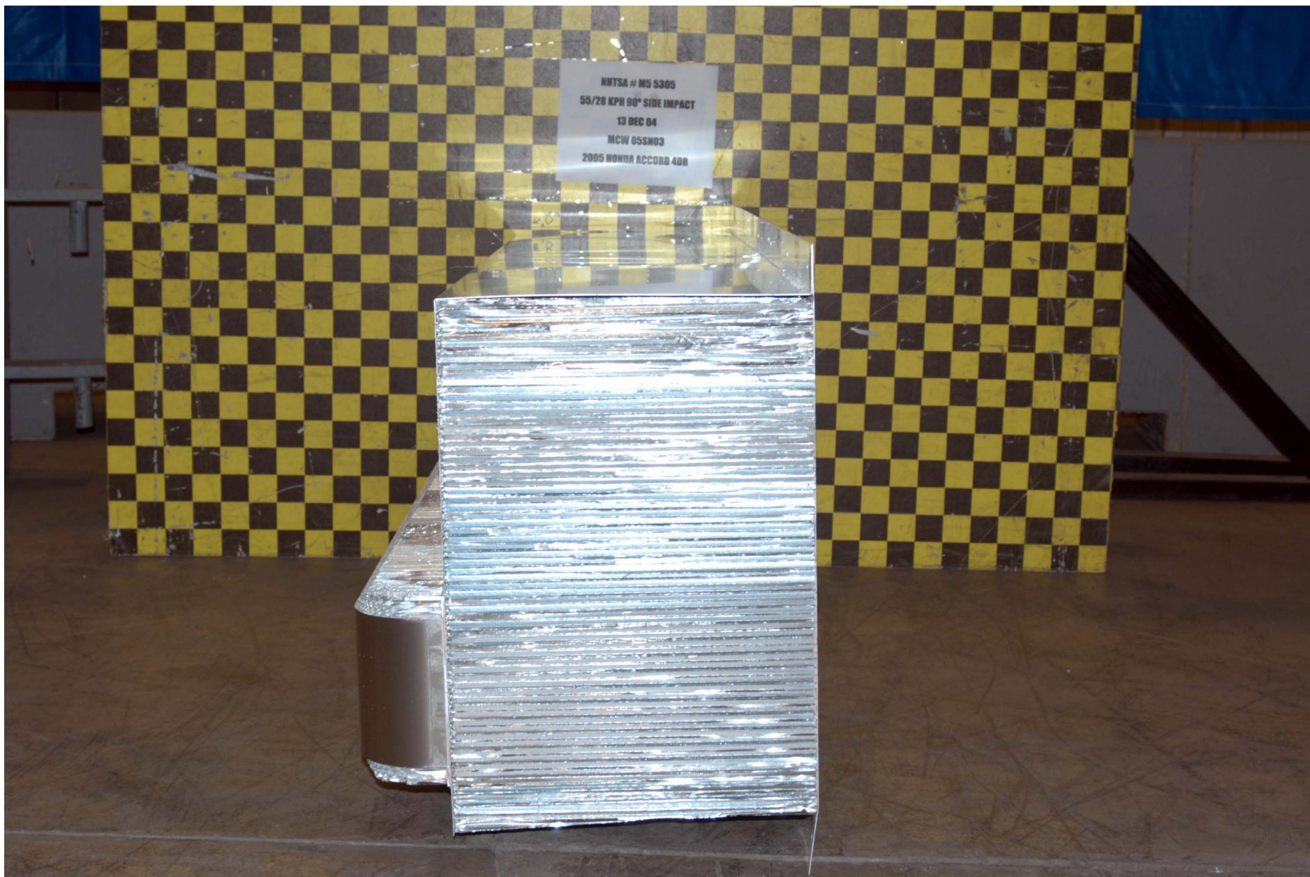
Figure A-49: PRE-TEST ALUMINUM BARRIER LEFT SIDE
