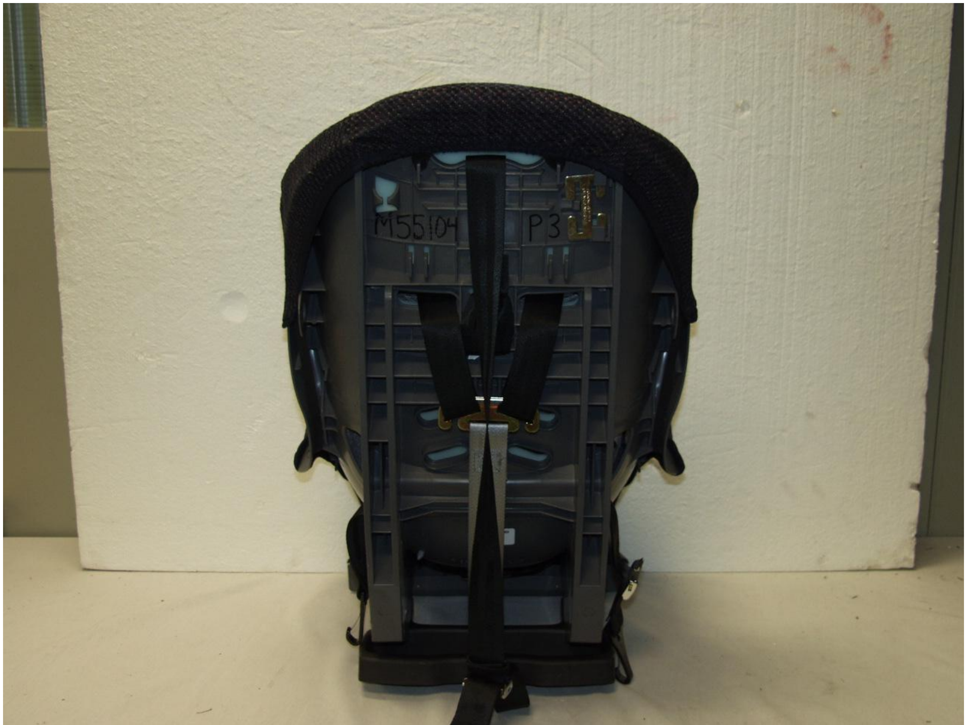
Figure 3-5 POST-TEST REAR VIEW OF POSITION 3 CRS
