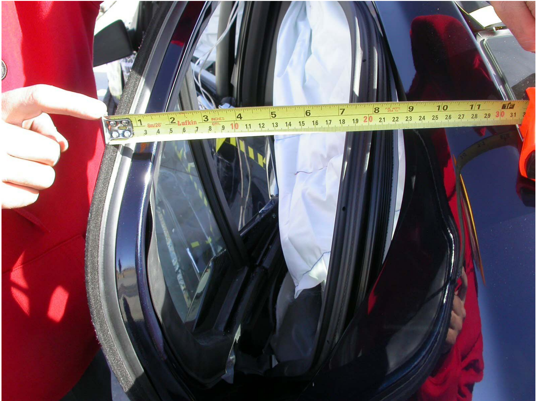
Figure A-68: Post-Test Impacted Rear Door
