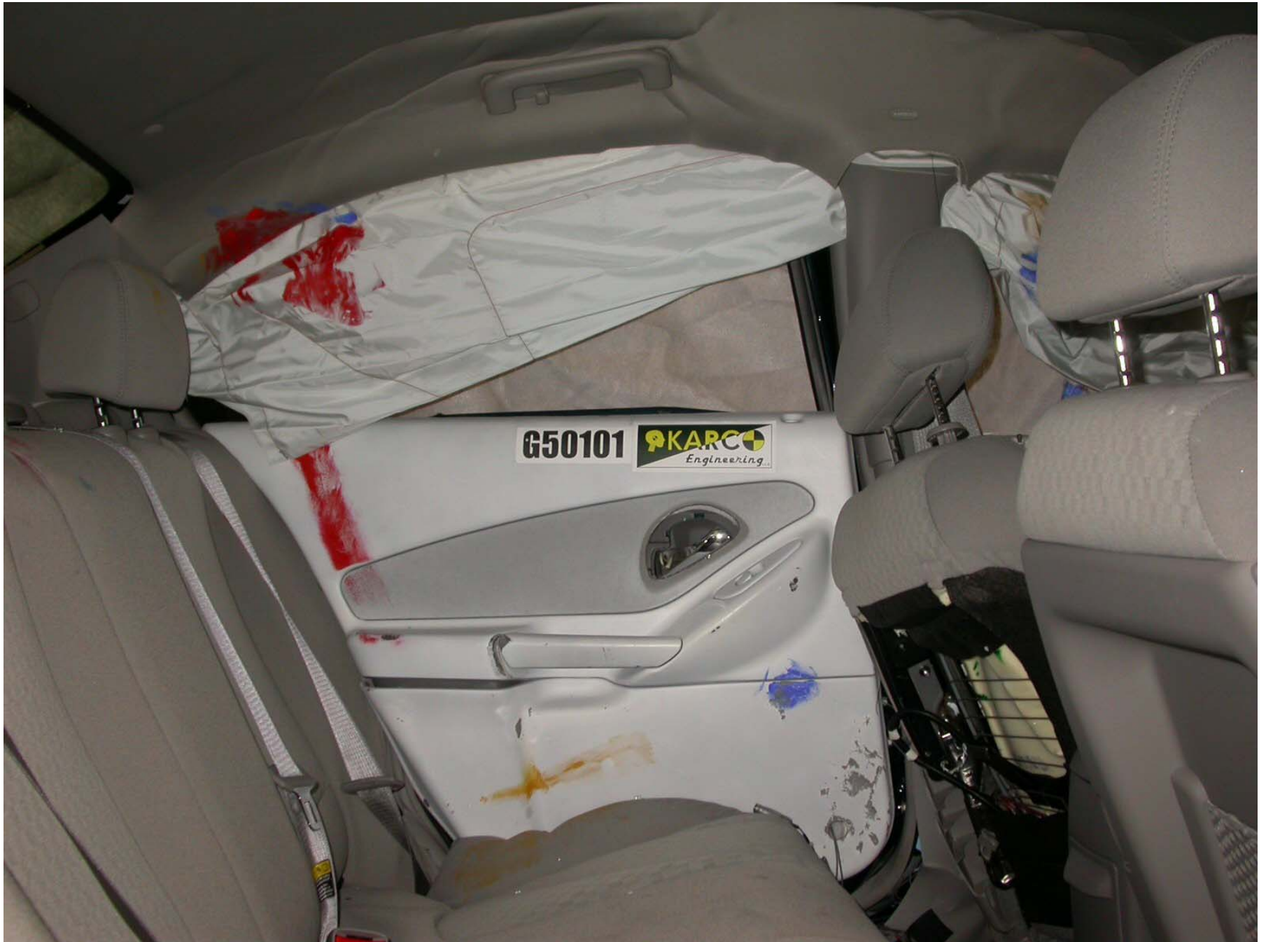
Figure A-54: Post-Test Passenger Door Panel (Interior)
