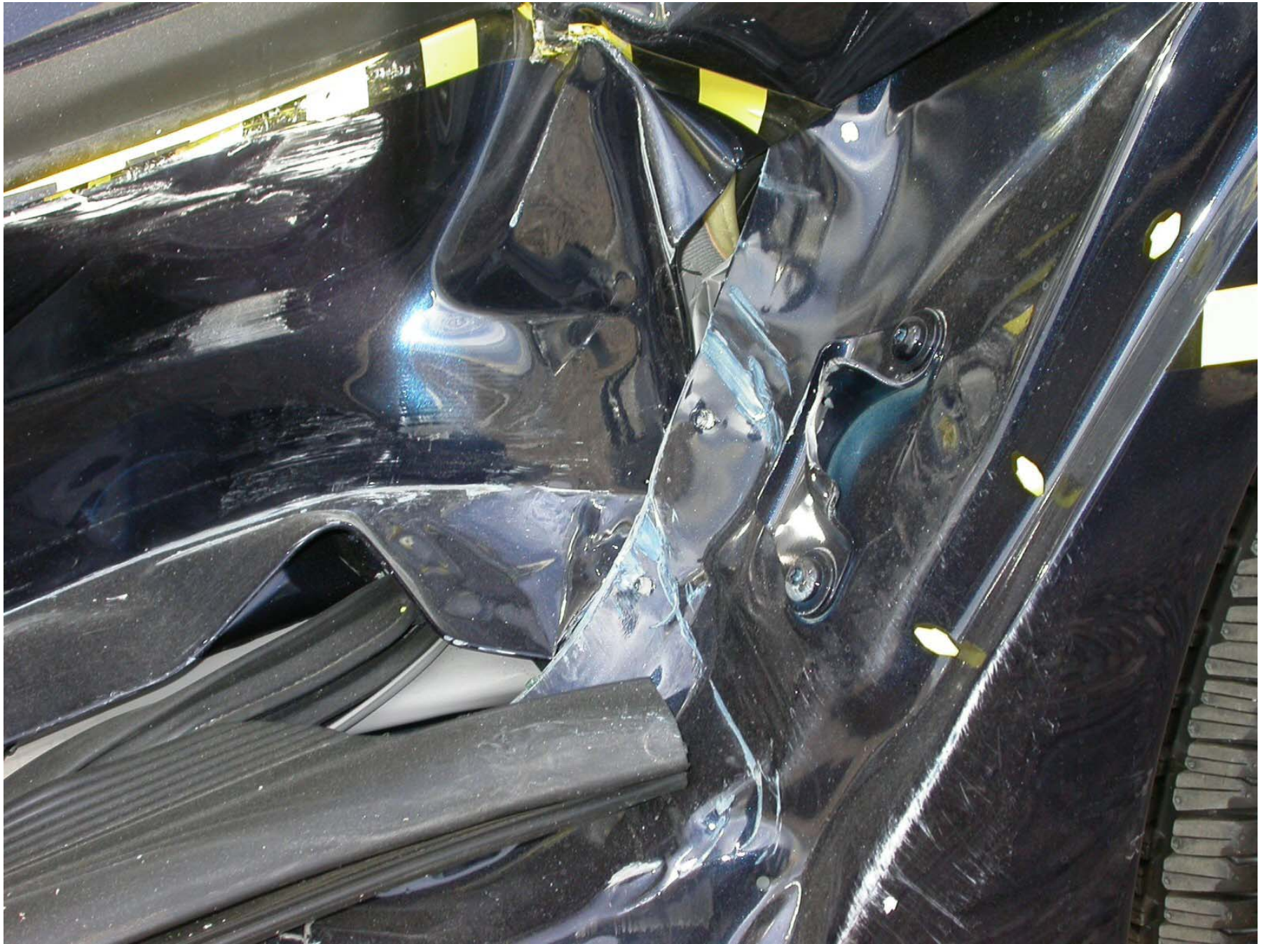
Figure A-69: Post-Test Impacted Rear Door Interlock
