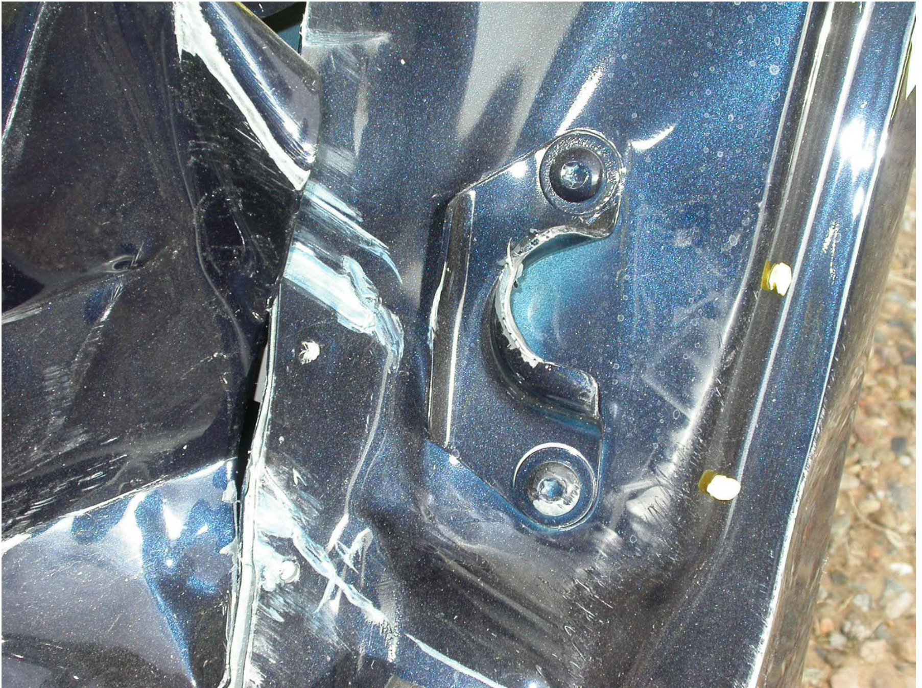
Figure A-70: Post-Test Impacted Rear Door Interlock
