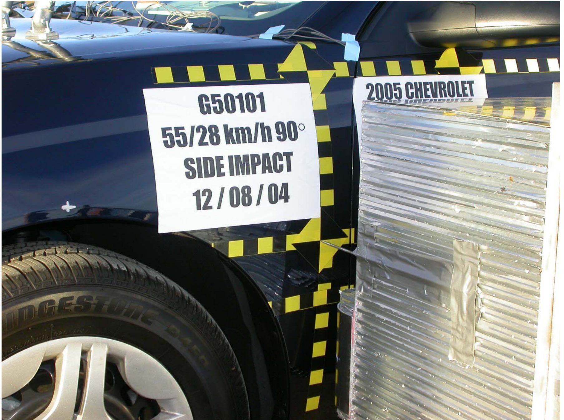
Figure A-25: Pre-Test Left Impact Point
