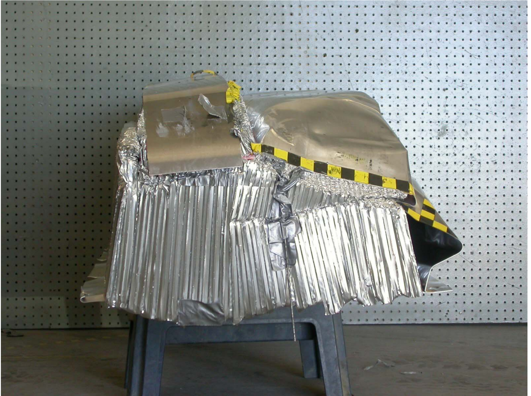
Figure A-62: Post-Test Left Side View of Deformable Barrier
