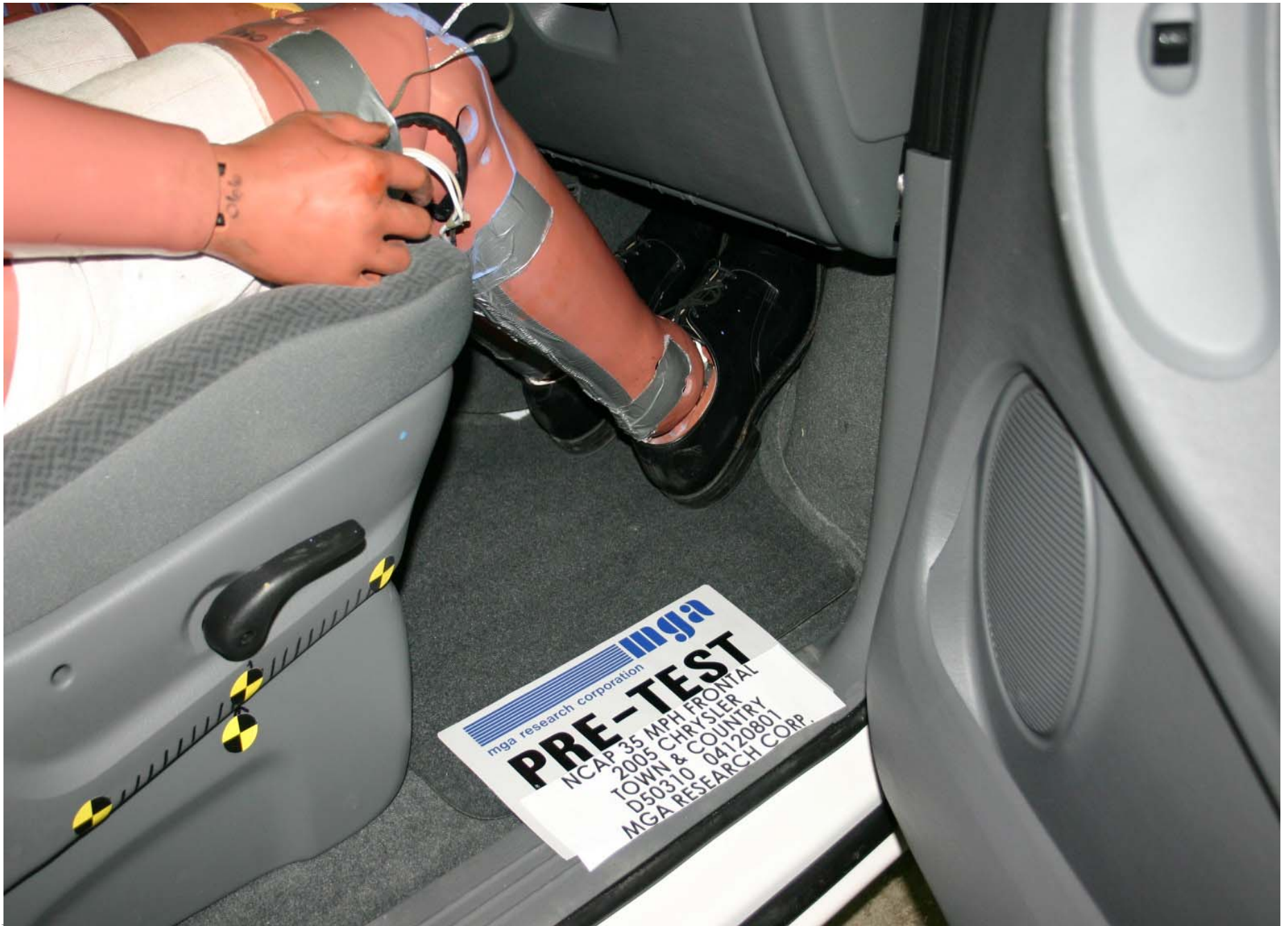
Pre-Test Passenger Dummy Feet Position
