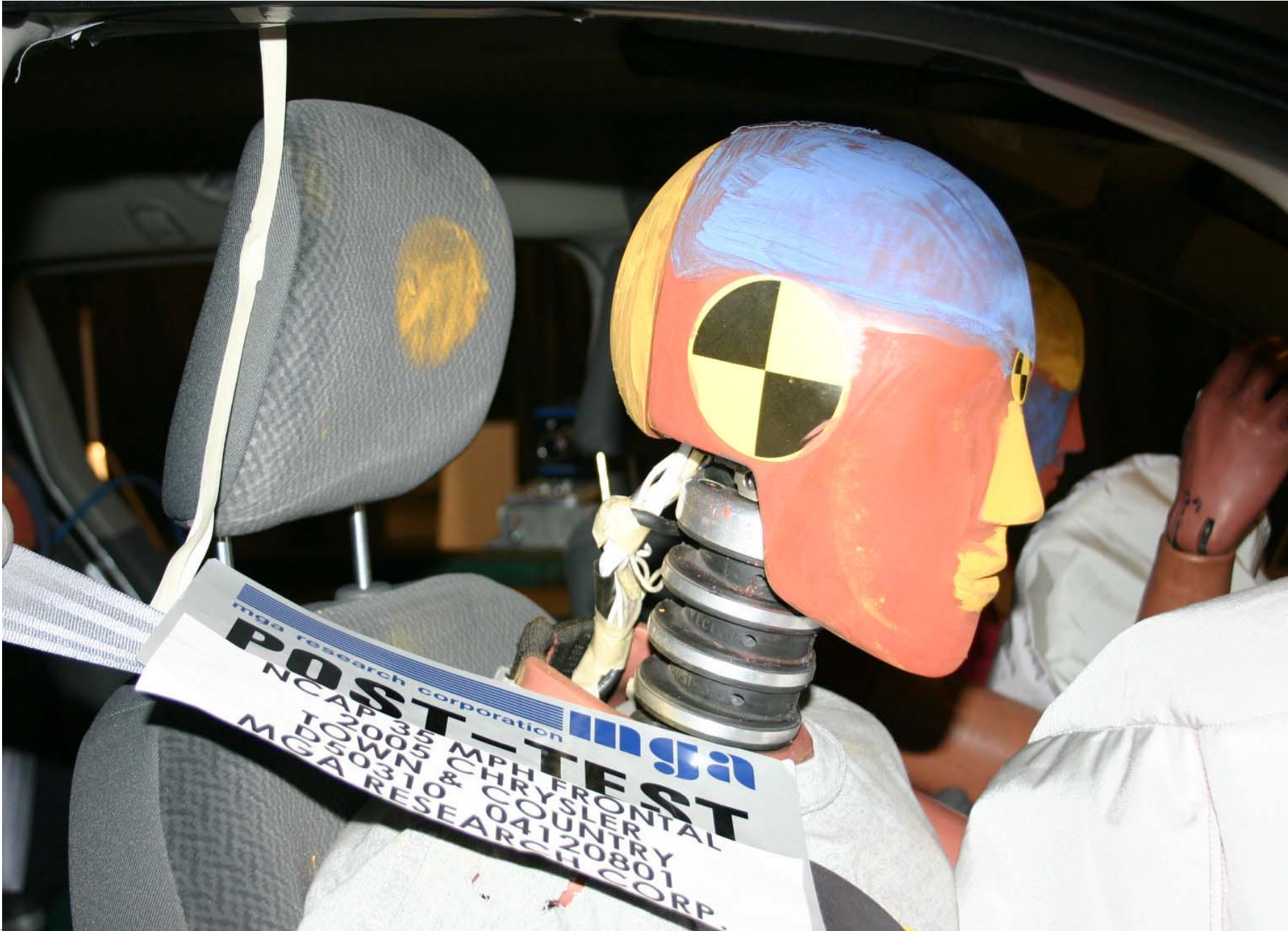
Post-Test Passenger Dummy Head Contact
