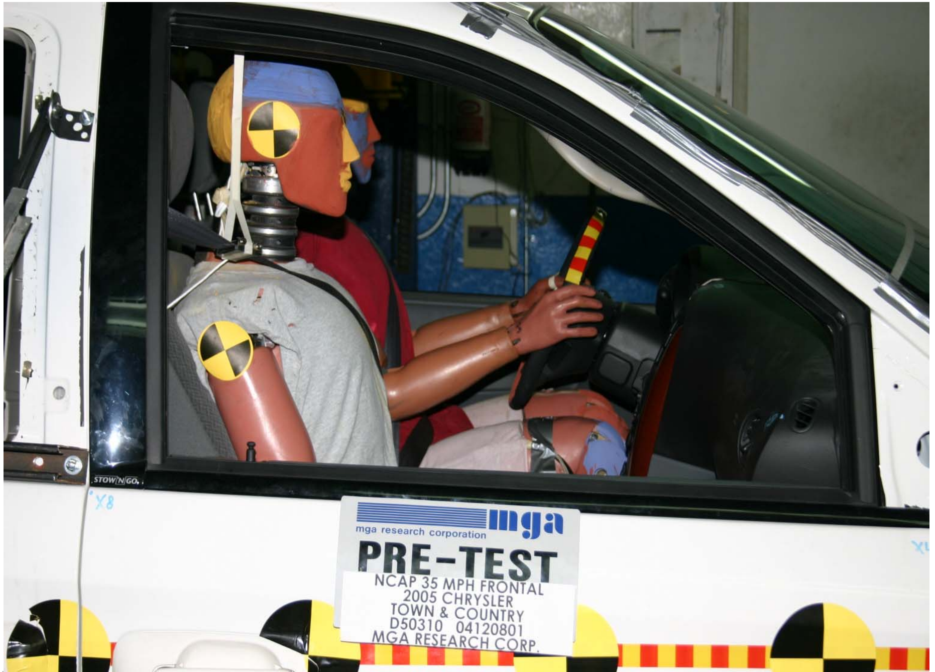
Pre-Test Passenger Dummy Position Right Side View
