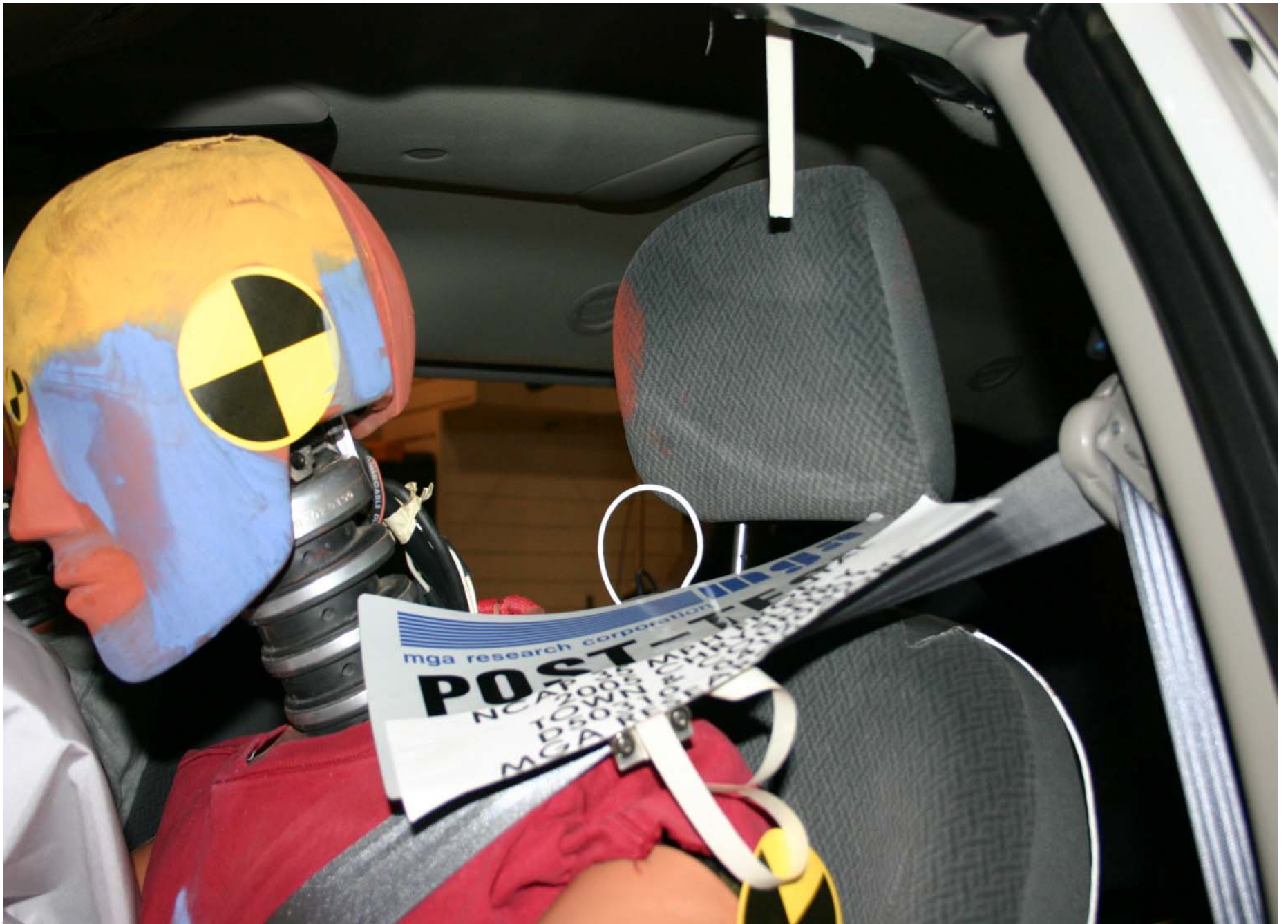
Post-Test Driver Dummy Head Contact
