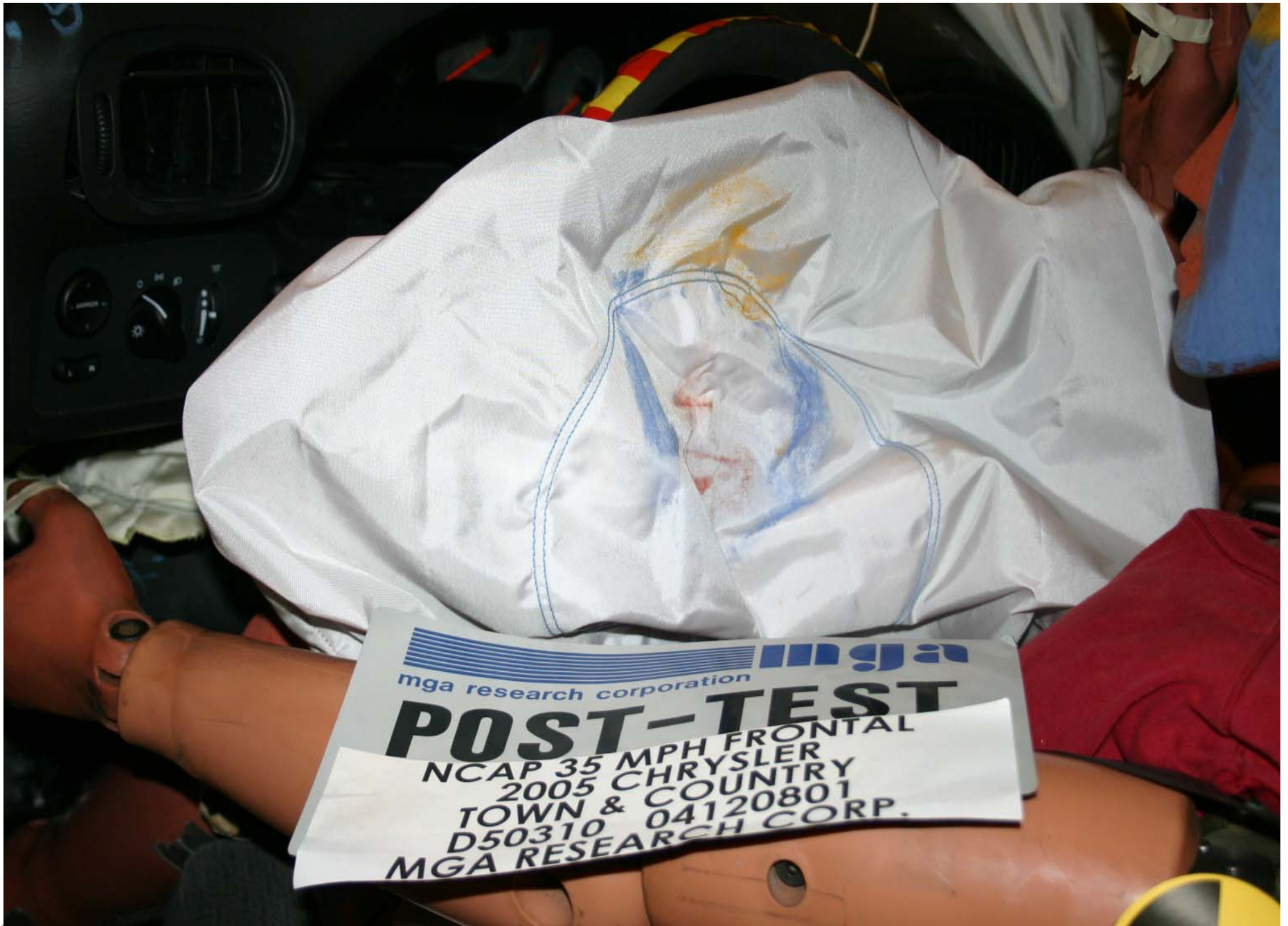
Post-Test Driver Dummy Airbag Contact
