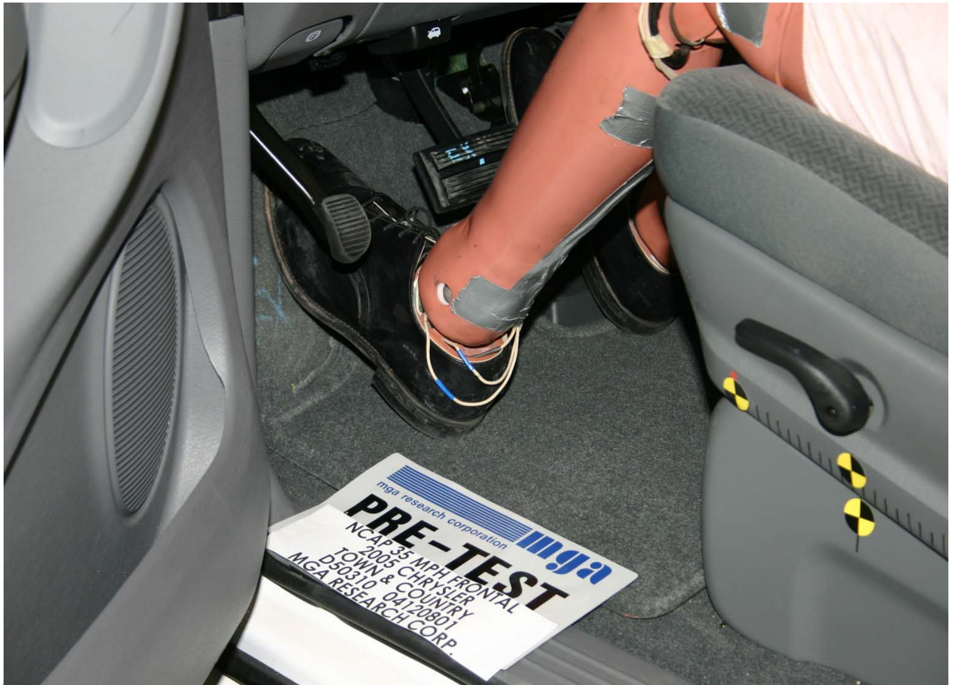
Pre-Test Driver Dummy Feet Position
