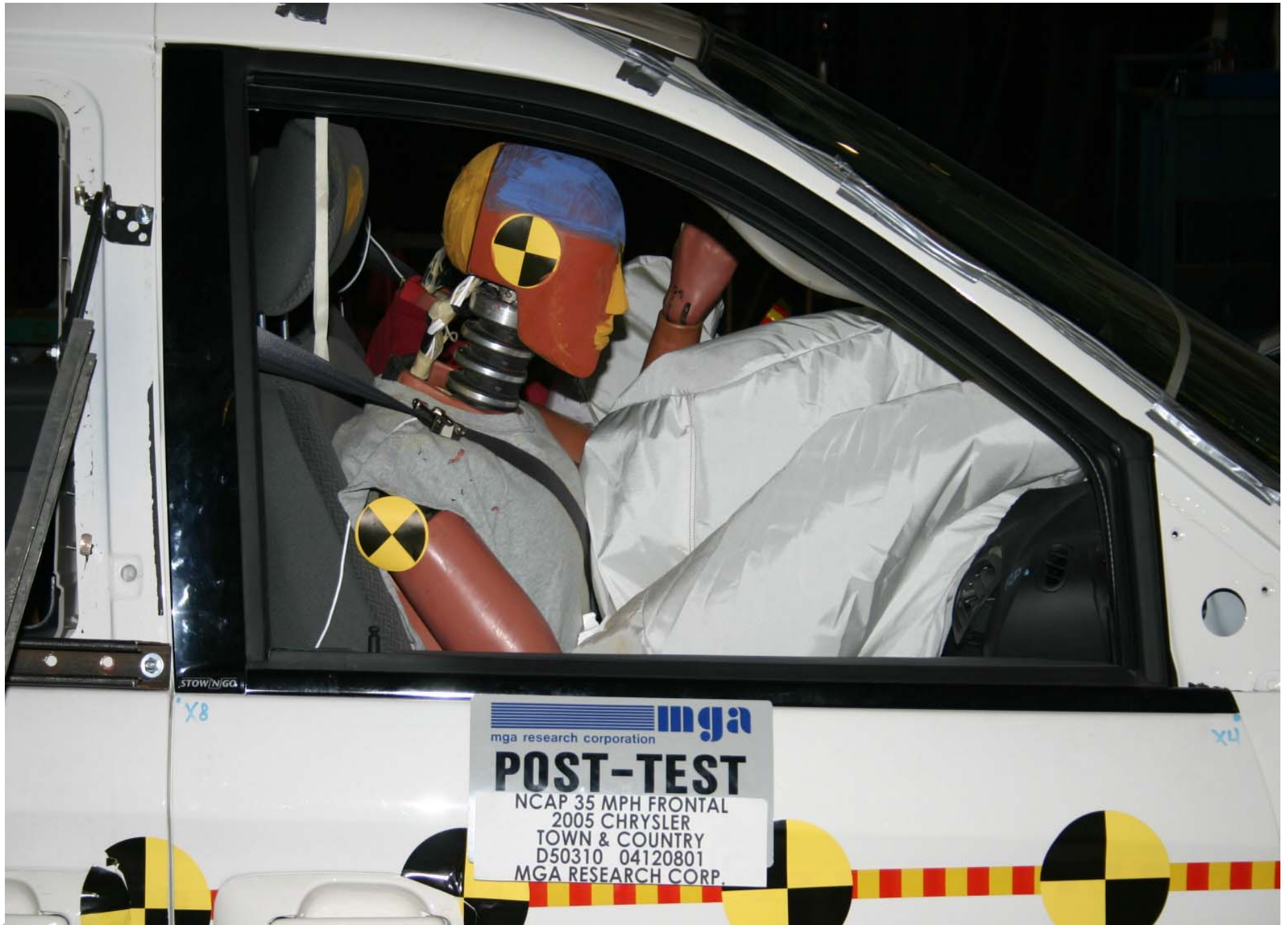
Post-Test Passenger Dummy Position Right Side View
