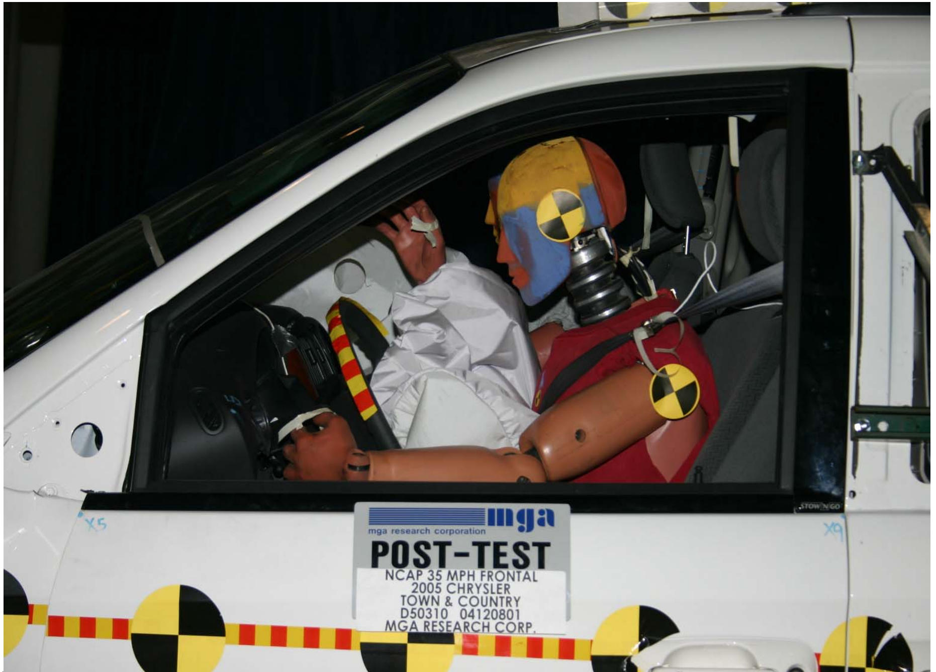
Post-Test Driver Dummy Position Left Side View
