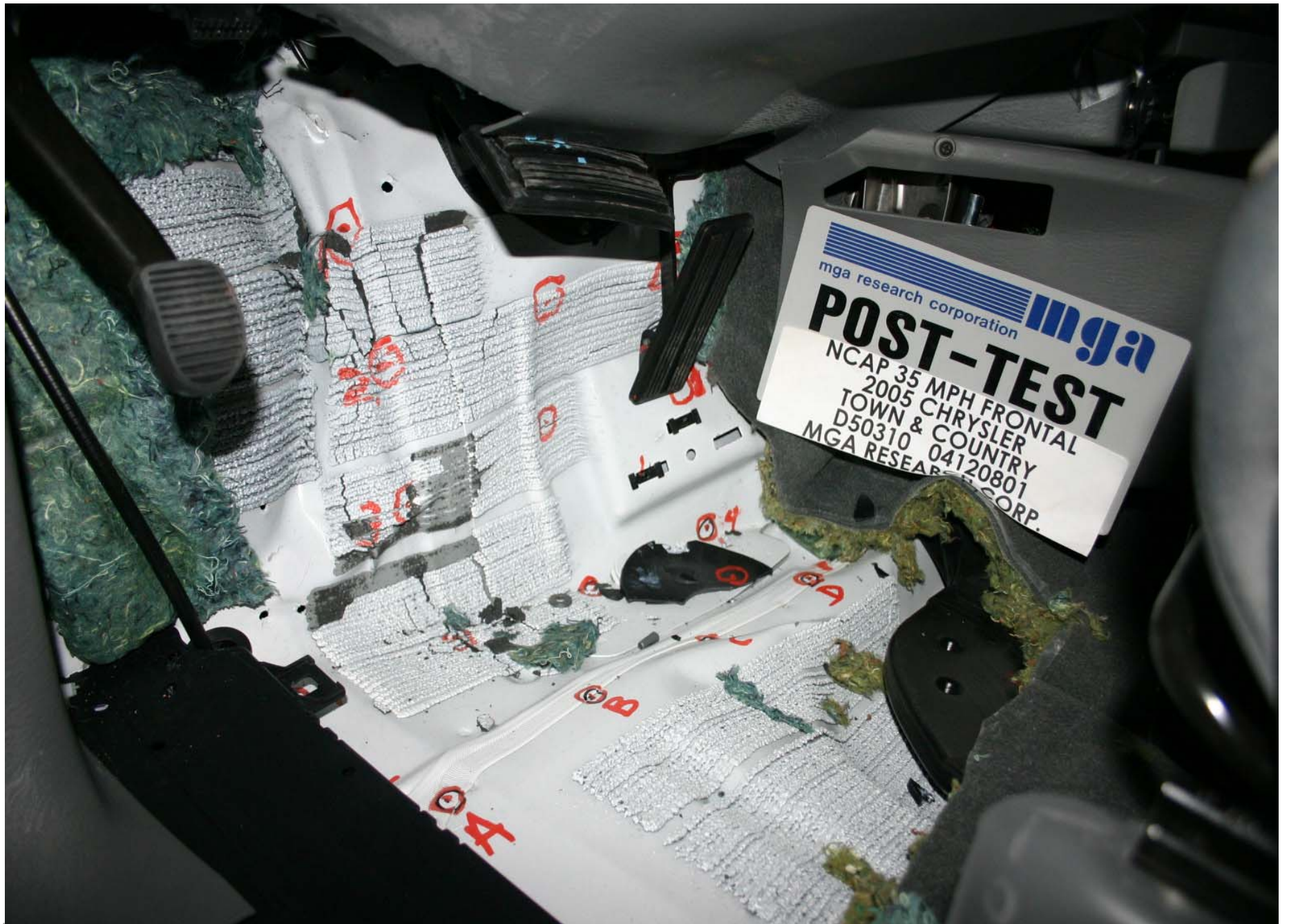
Post-Test Driver Side Floor Pan View
