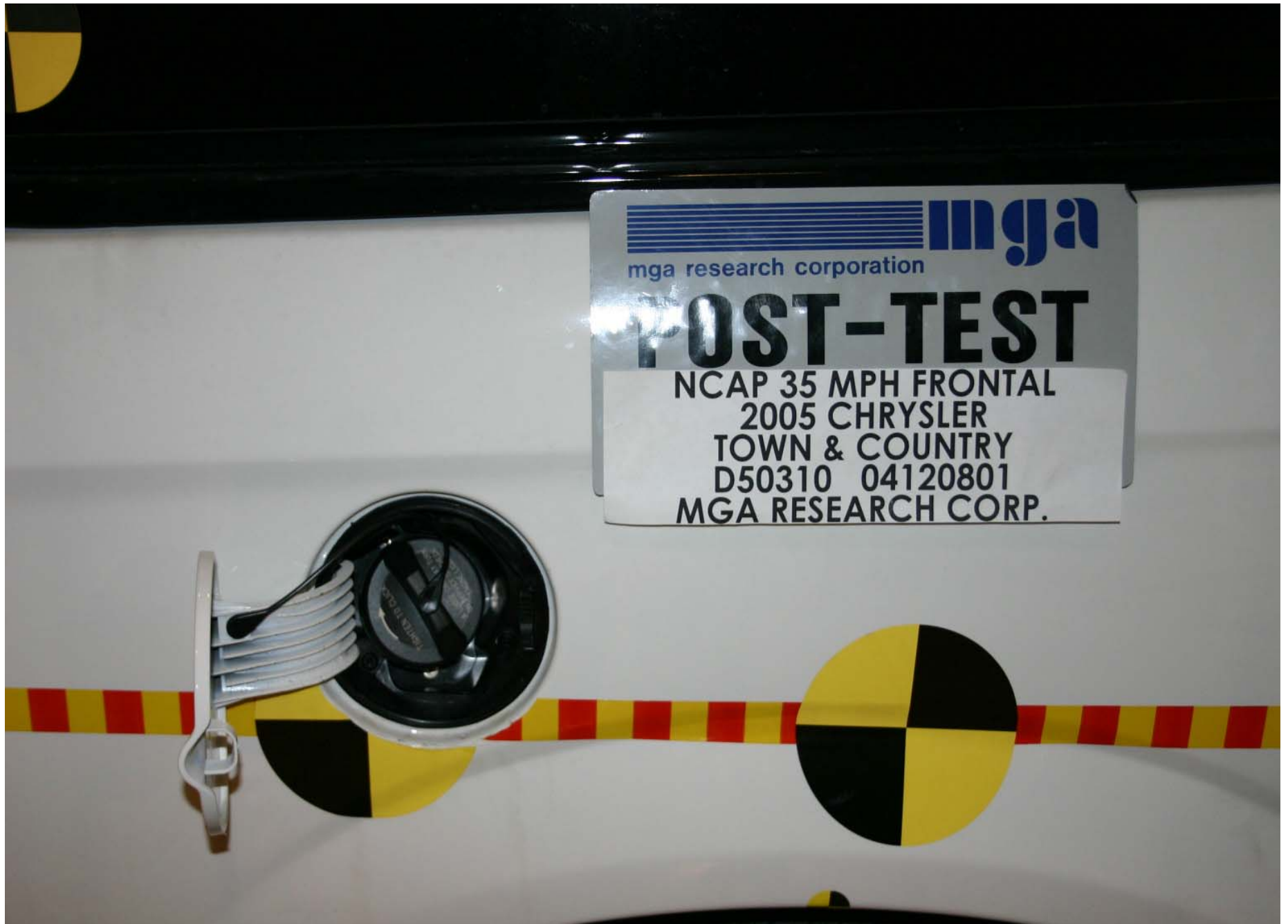
Post-Test Fuel Filler Cap View
