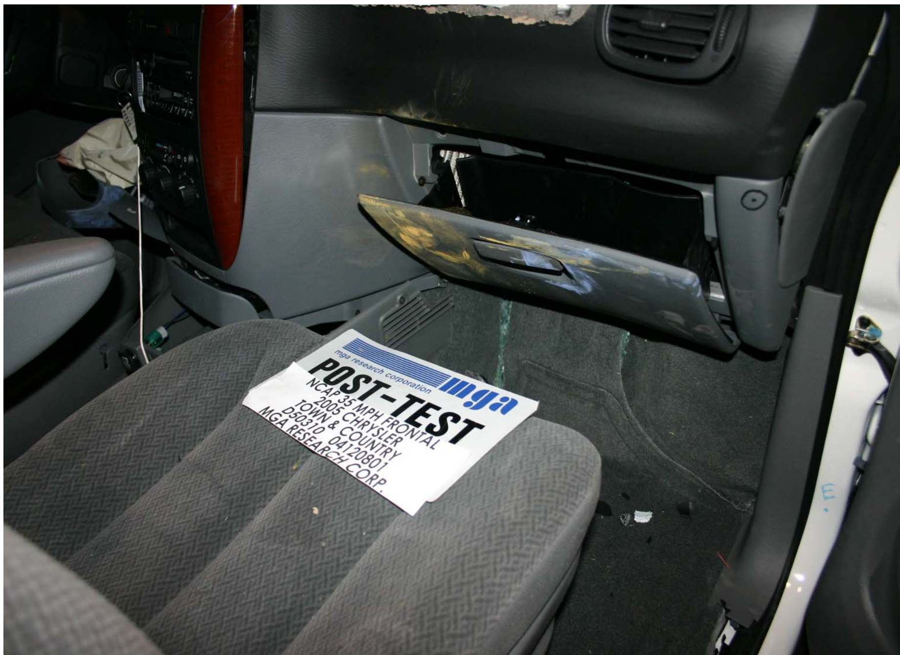
Post-Test Passenger Dummy Knee Contact
