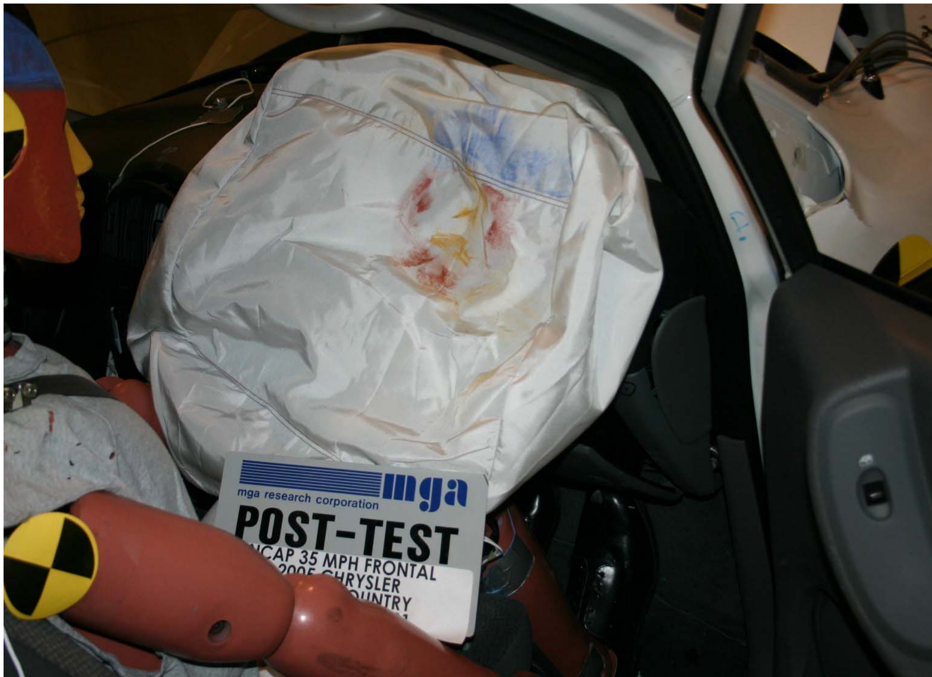
Post-Test Passenger Dummy Airbag Contact
