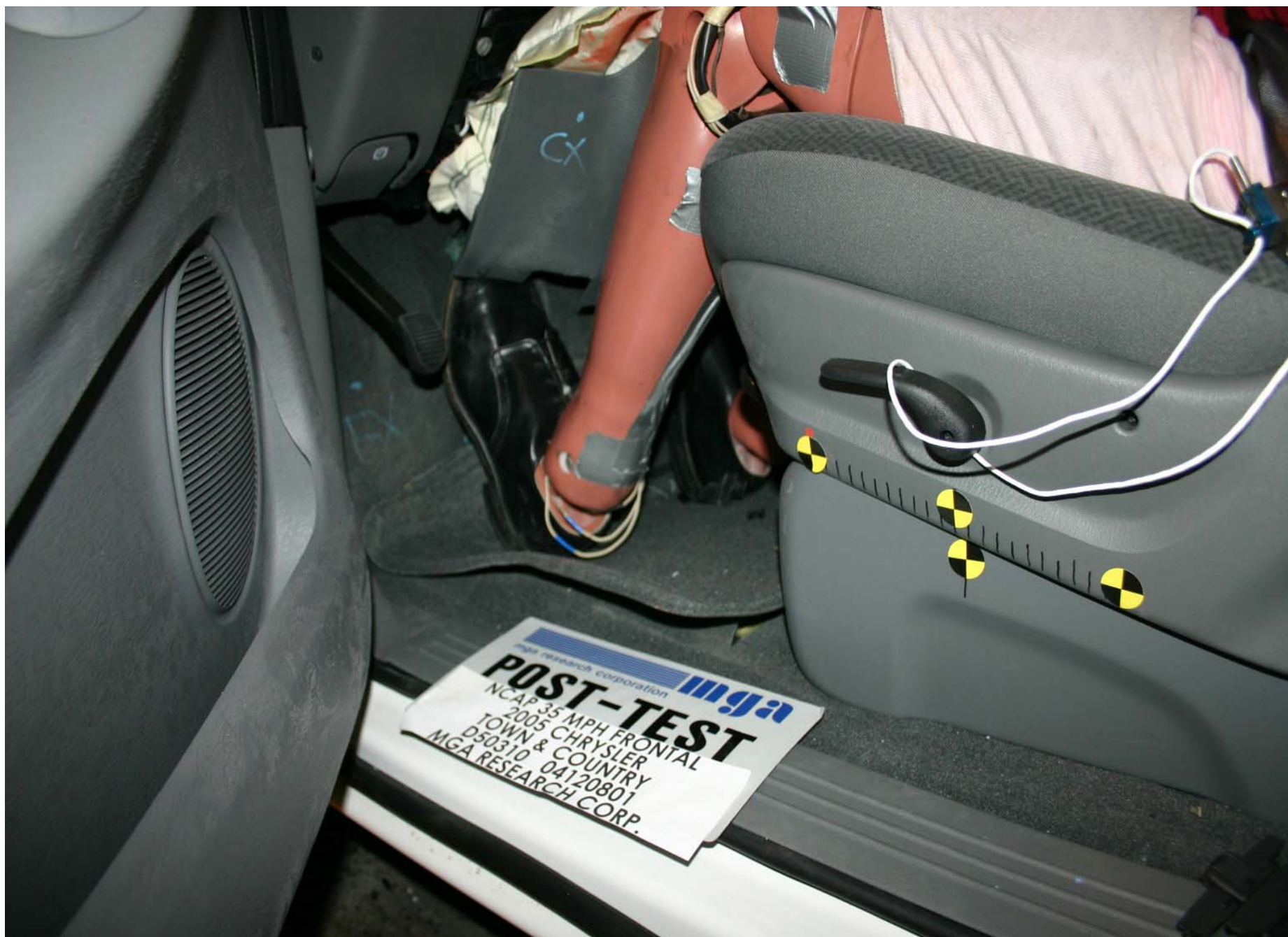
Post-Test Driver Dummy Feet Position
