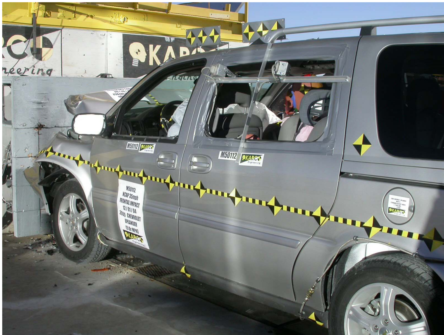
Figure A-17: Post-Test Left Side \frac{3}{4} View of Doors After Impact (Incorrect Placard: Placard Should Read 2005 Chevrolet Uplander)
